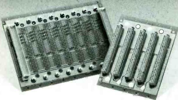
XIX<sup>IN</sup> VME Backplanes from Sarel are available to meet two functions. The XJI Backpanel is the main VME Bus, the XJ2 is the I/O Expansion Bus.
