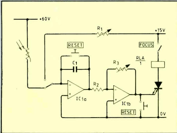
Fig. 2. Basic circuit of timer
