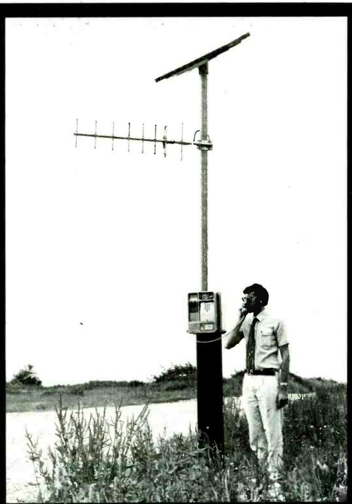
A telephone designed for use in the third world. It is solar powered and communicates by radio, with battery back-up. The equipment can also act as a relay to act as a local link so that remote villages can communicate with each other. Designed by Plessey Radio Systems.
