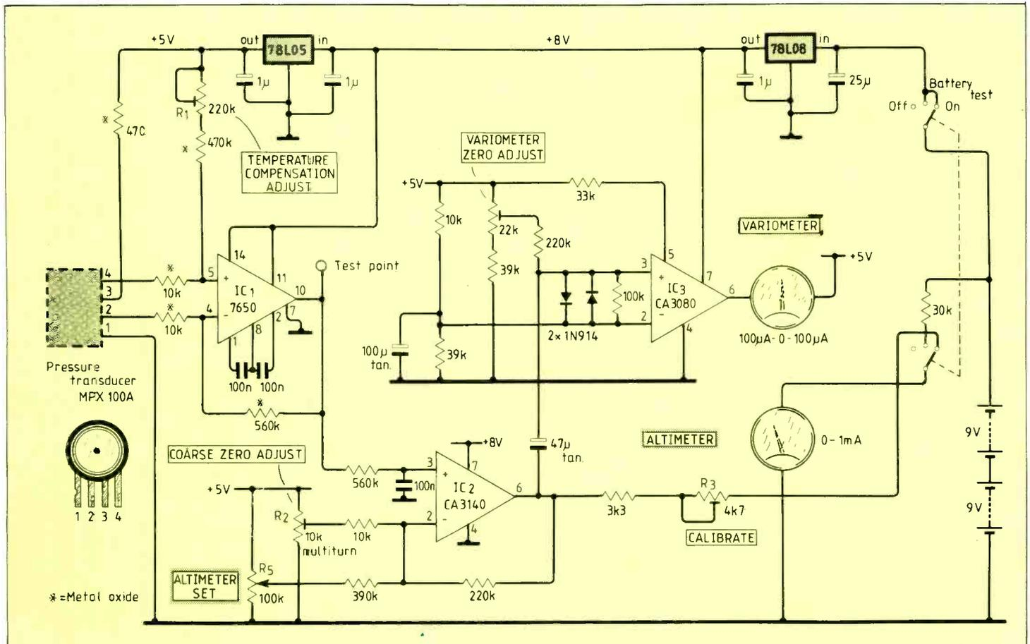
Pressure transducer is a low-cost device intended for the motor industry. Temperature compensation is achieved by the 7650 chopping op-amp and a Wheatstone bridge circuit.
