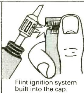
Flint ignition system built into the cap.
