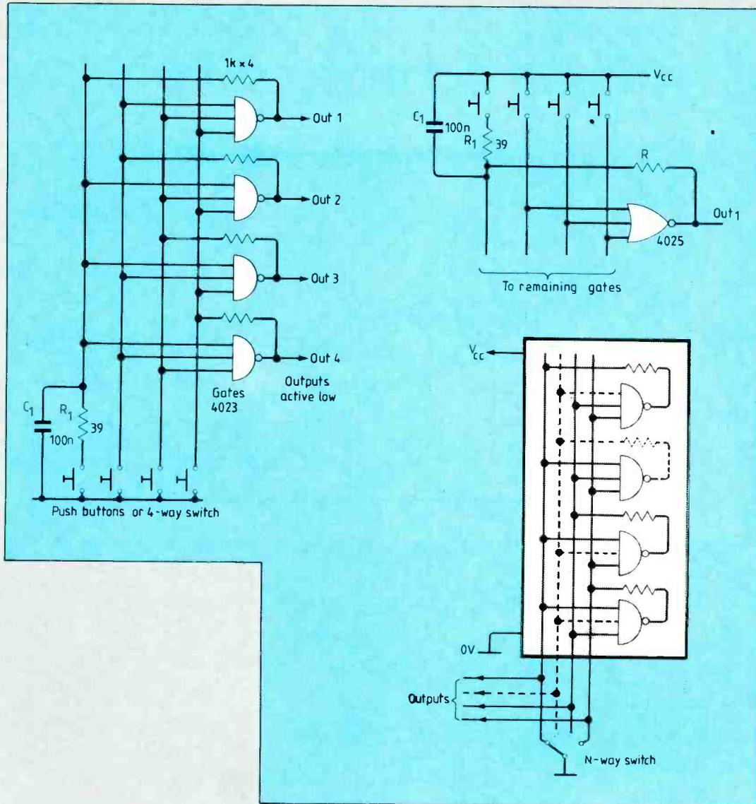
Contact debounce, a predetermined power-up setting and simplicity are features of this one-in-n-way push-button latch. When any button is pressed, its corresponding button line is taken low, forcing all others high. Only one line can be low at a time.
