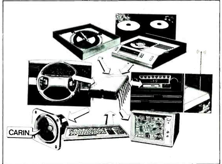
The elements, CD player, dashboard data, electronic compass and computer, that go together to make the Carin route information system, under development by Philips.
