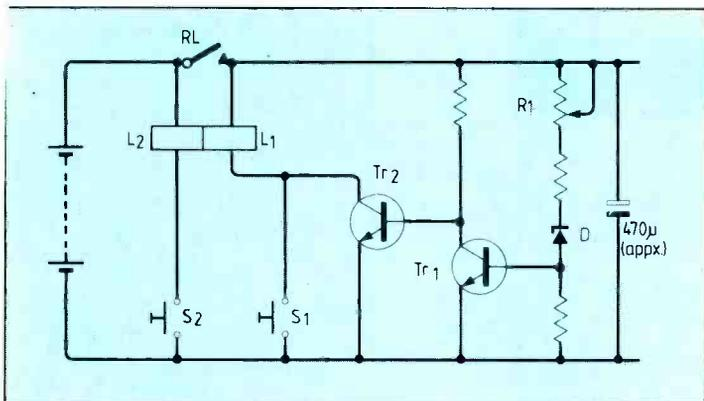
**Fig. 2. Low-voltage cut-out circuit is turned on by pressing push-button PB<sub>2</sub>. Relay closes, but Tr<sub>1</sub> clamps base of Tr<sub>2</sub> and holds off the coil L<sub>1</sub> of the relay. If voltage falls below that set by pre-set pot R<sub>1</sub> and zener, Tr<sub>1</sub> releases Tr<sub>2</sub>, the turn-off coil L<sub>1</sub> opens the relay and the load and circuit are switched off. Alternatively, the load may be turned off by pressing push-button PB<sub>1</sub>.**
