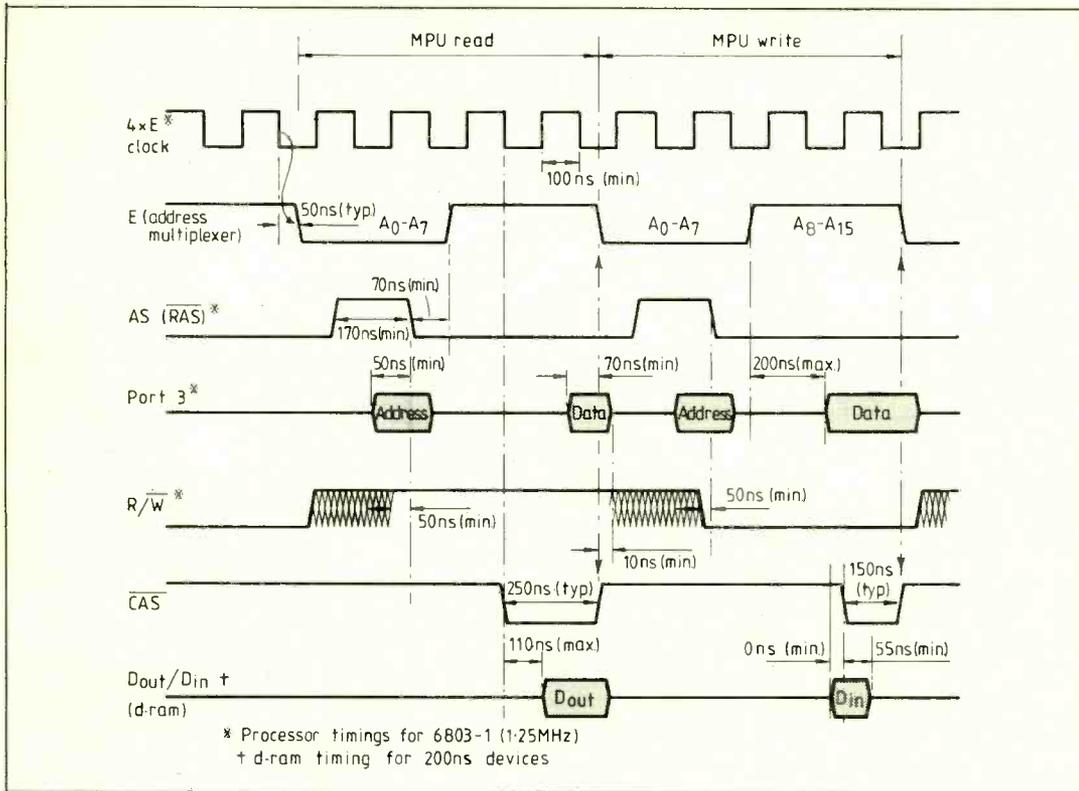
Fig. 5. Printer buffer timing required for dynamic rams.
