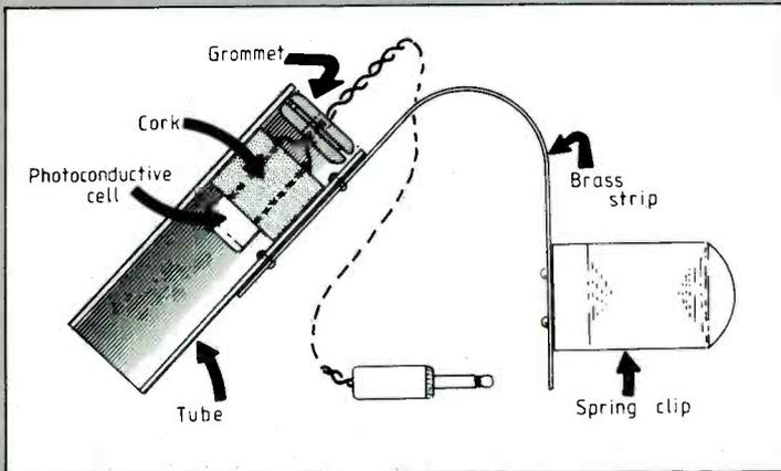
Fig. 5. Tubular holder for photosensitive cell giving a 30 degree viewing angle. Terry clip fixes to enlarger column.
