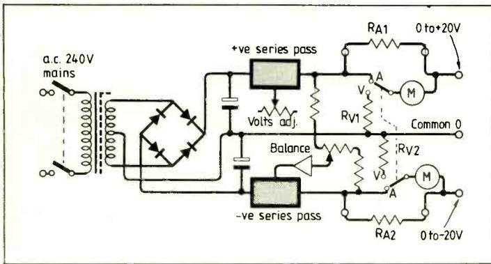
Fig. 1. The diagram shows how positive and negative lines can be obtained from a centre tapped transformer secondary in conjunction with a bridge rectifier. The negative line is referenced to the stabilised positive supply.
