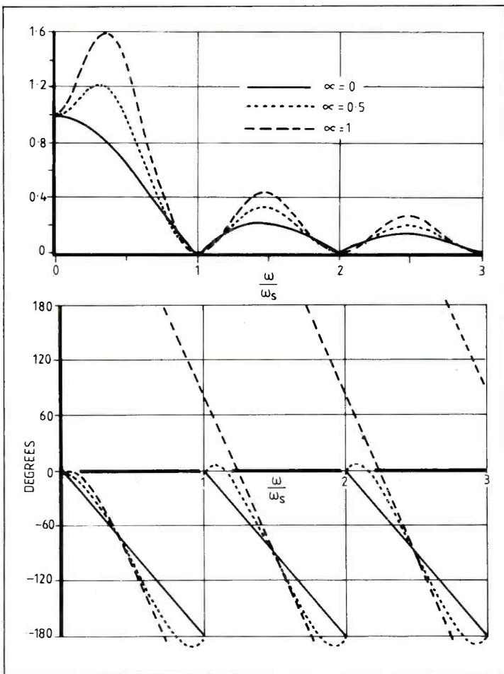
**Fig. 17. Gain characteristics of various hold circuits, amplitude above, phase below.**
