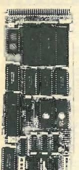
Based on the Intel 8052AH single component Microcontroller the CPU comes complete with a unique implementation of the BASIC language enabling direct access to the special function registers, timers and interrupts available on the 8051 device.
