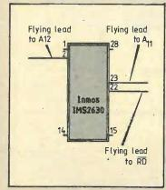
Remove the existing ram i.c. or i.cs and clear out the holes for the 28 pin package, preferably using a desoldering tool. Fit a 28-pin socket to the board and bend pins 2, 22 and 23 so that they do not fit in the socket when the IM 2630 is inserted. Finally, solder these pins to the circuit board as shown. K. Ball
