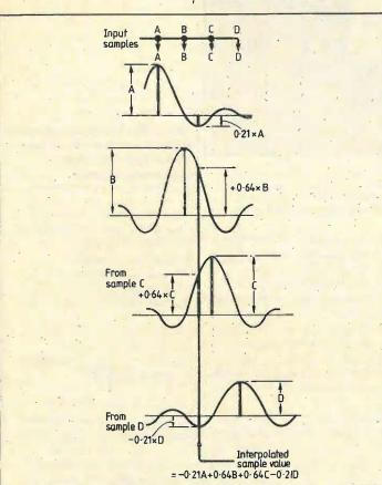
Fig. 8(a). To compute an intermediate smaple, the input samples are imagines to be sinx/x impulses, and the contributors from each at the point of interest can be calculated. In practice rather more samples either side need to be taken into account.
