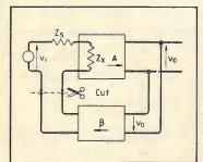
Fig.4. Practical amplifiers have impedances that load the network.
