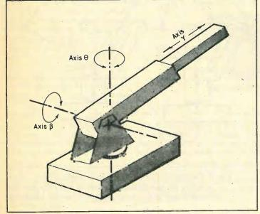
Fig. 4. Versatile yet basic configuration is capable of operation at any point inside the volume described by two concentric hemispheres whose maximum radius of operation is the length of the fixed arm plus y. This configuration is particularly suitable for robots of heavy load carrying capability.
