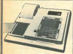
LOGS all tests and responses on PRINTER and ALPHA LCD Non-volatile memory retains test sequences CHECKSUMS, RAMTESTS, READS/WRITES MEMORY & I/O Reports location of SHORTS on ADDRESS and DATA busses Prints out memory contents n ASCIL HEX or SOURCE CODE
