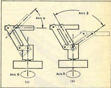
Fig. 6. Pantograph coupling on an articulated arm robot ensures the manipulator or power tool may remain perpendicular to the work station when the shoulder axis is moved.
