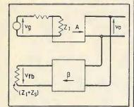
Fig.5. Loop gain for the circuit in Fig.4 is obtained by opening up the loop but maintaining the impedance levels shown.
