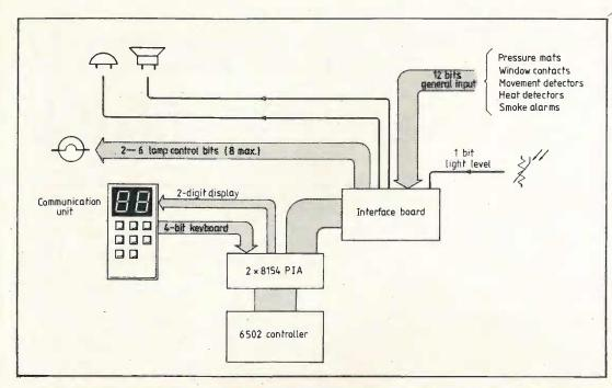
service up to eight mains lights, 12 inputs from various sensors, a five-tone internal sounder and special connections such as light level and auto reset prevention. Six port bits are used for user interface, allowing a reasonable length connection cable to the controller.
