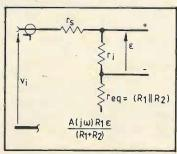
Fig. 7. Equivalent circuit of Fig.6 for straightforward circuit analysis.
