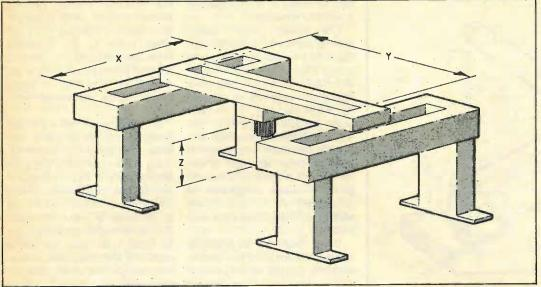
Fig. 2. Further example of the solid rectangle configuration. Manipulator covers area xy with the manipulator height over work area variable between zero and z. Uses include machine tools, heavy plant assembly and transferring parts within workcells normally outside the reach of the more conventional robot.
