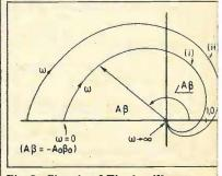
Fig.2. Circuit of Fig.1 will not oscillate if it has characteristic (i): oscillations occur
