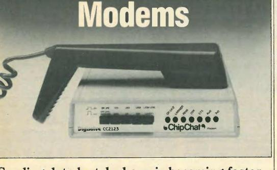
This microprocessor-based low-speed modem covers speeds of up to 1200 bit/s. Special features include an auto-dialler and a speed conversion buffer for access to viewdata from terminals (such as the IBM p.c.) which cannot send and receive at different rates.
