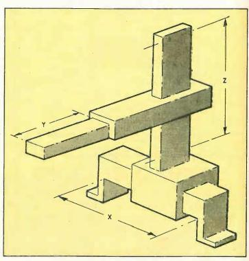
Fig. 1. Three sliding members are tightly confined to their respective freedoms-of-movement x, y and z. This gives an operating envolope which is a solid rectangle. The manipulator can be positioned at any distance between zero and y from the rectangle x\*z. Applications include automated
