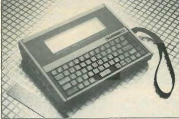
Display is through an eight line, 40-character liquid crystal which can be used for graphics. The screen memory allows for an 80-character by 24-line screen and the l.c.d. acts as a window on this larger virtual
