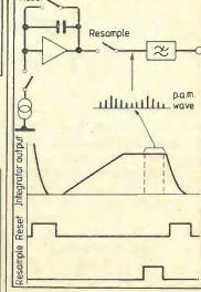
Fig. 6. In an integrator, the output level is only stable when the ramp finishes. An analogue switch is necessary to isolate the ramp from subsequent circuits. The switch can also be used to produce pulse amplitude modulated signal which has a flatter frequency response than a zero-order hold (staircase) signal.
