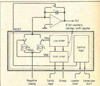
Fig. 3. Simpified diagram of sony CX-20017 having the high and low order current sources and associated timing circuits. The necessary integrator is external. Output needs to be resampled at peak of ramp (see Fig. 6).
