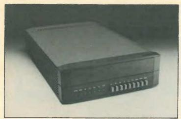
Duplex operation at 9600 baud over a two-wire telephone line is possible using a modem such as this one, the DM4962X from BT. Such a communication speed over a standard line requires a little more than frequency-shift keying circuits, though. This unit uses quadrature amplitude modulation.
