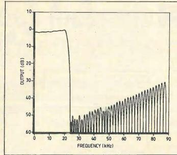
opposite errors at  $F_s = 176 \text{ kHz}$  Fig. 11. Amplitude response of digital filter in Philips produce a signal at 88 kHz, which oversampling system. The small rise to 20kHz offsets oversampling system. The small rise to 20kHz offsets the sinx/x aperture effect of zero-order hold d.a.c. Ripple in the stop band is due to truncation of coefficients. (Diagram courtesy of Philips Technical Review).
