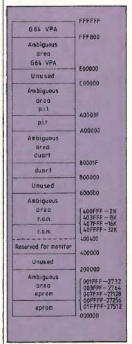
Fig. 2. Kavcomp system memory map. Simple address decoding means a cheap system allowing sufficient memory for most computer-
