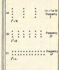
Fig. 9. Information rate can be held constant when frequency doubles by removing one bit from each word. In all cases here it is 16F. Bit rate of (c) is double that of (a). Data storage in oversampled form is inefficient.
