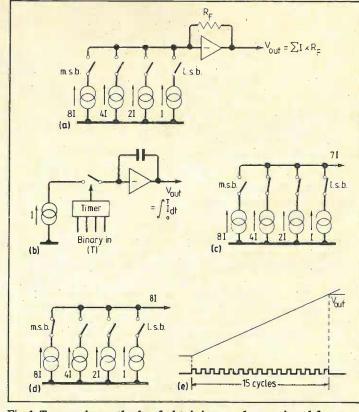
Fig. 1. Two main methods of obtaining analogue signal from binary data are the weighted current converter (a), and the timed integrator (b). In (c) the binary input is 0111 while in (d) it has increased by one bit, so a minimum accuracy is 1 in 16 for this four-bit converter, and would need to be 1 in 65,536 for a 16-bit converter. In the integrator technique (e), 15 clock cycles are counted for 1111 input and for a 16-bit device the clock rate would need to be 216 times sampling
