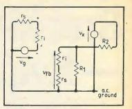
Fig. 8. Redrawn version of circuit of Fig. 6 opened-up by making a 'cut' at the inverting input terminal. Resistor r<sub>i</sub>+r<sub>s</sub> connected across R<sub>1</sub> takes into account power fed back into the circuit.
