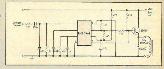
engine to idle correctly. The circuit is connected to the ignition side of the positive
