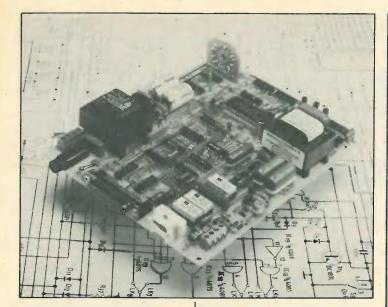
Wireless World modem: this low-speed two-wire modem, based on the Am7910 i.c., covers the V.21, V.23 and corresponding Bell modes and costs around £70 to make (E&WW, May-July and December 1984; the p.c.b. is still available). A series by Martin Allard describing a personal electronic mail system for the constructor began in the August issue. And a microprocessor-based multi standard terminal unit was described by John Walker in October's issue.
