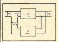
Fig.1.Conventional idealized feedback amplifier system. Arrows in boxes A and B show the direction of unilateral signal flow.
