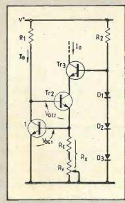
Now, large changes in V+ cause only small changes in VBE1 because of the logarithmic dependence of  $V_{BE1}$  on  $I_B$ . It can be shown that for
