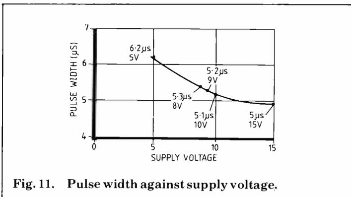
Fig. 11. Pulse width against supply voltage.
