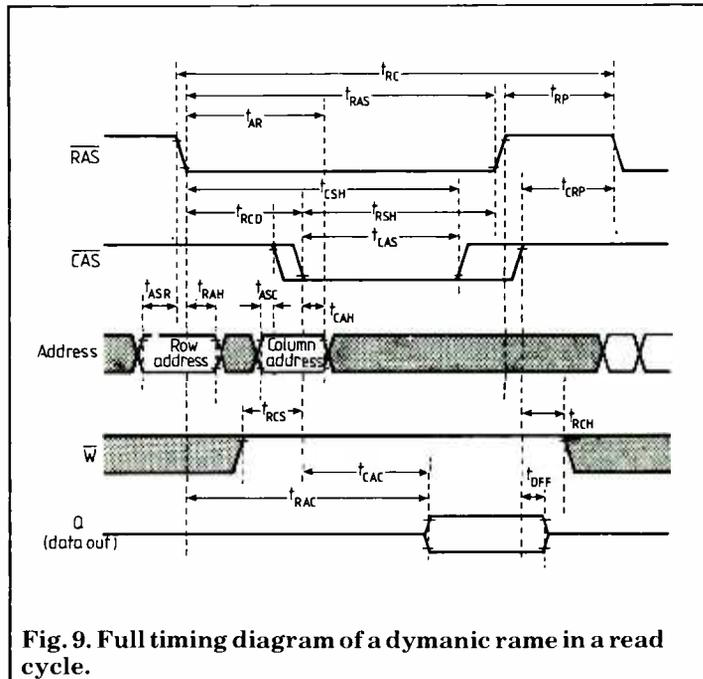
**Fig. 9. Full timing diagram of a dynamic RAM in a read cycle.**
