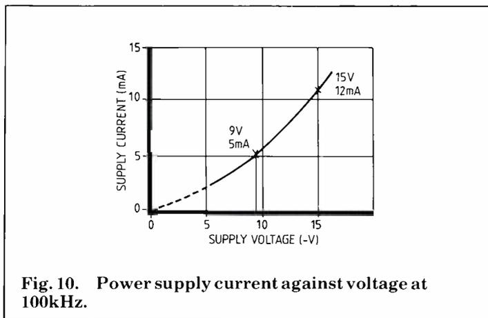
Fig. 10. Power supply current against voltage at 100kHz.
