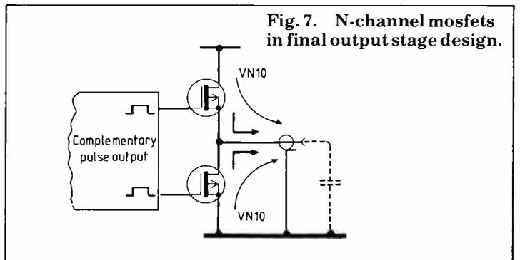
Fig. 7. N-channel mosfets in final output stage design.
