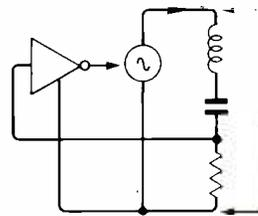
Fig. 5. Skeleton series-resonant self-oscillator in one possible form. The resistor would be a very low-value component, just enough to develop a useful feedback signal in phase with the current.
