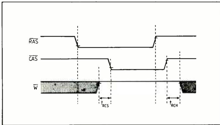
**Fig. 7. In a read cycle, there are no complex restrictions on the  $\bar{w}$  (write enable) input. It must be high at least  $t_{RCS}$  seconds before the falling edge of  $\bar{CAS}$  and remain high until after the rising edge of  $\bar{CAS}$ .**
