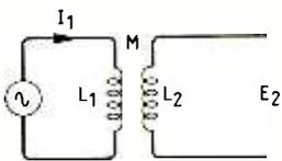
Fig. 1. Radio-frequency link in the form of a loosely coupled transformer
