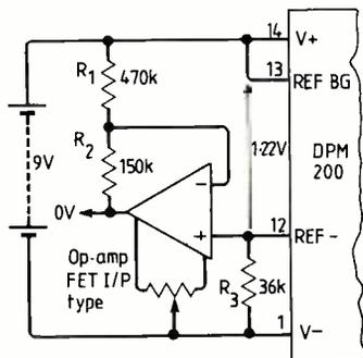
The voltage between Ref BG and Ref - is 1.22V nominal. Resistors R<sub>1</sub> and R<sub>2</sub> should be low-drift types. The advantage of this circuit is that it avoids the temperature coefficient of D<sub>5</sub> and the V<sub>be</sub> and H<sub>fe</sub> coefficient of the BC212 transistor.
