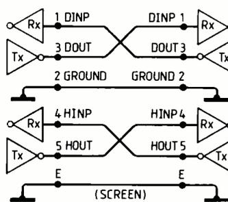
Fig. 7 (left). Standard S5/8 interconnecting cable. This one type will satisfy nearly every requirement.
