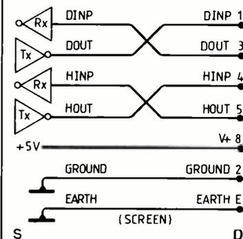
Fig. 8 (above). S5/8 captive lead for s-devices, which are those with no built-in power supply.
