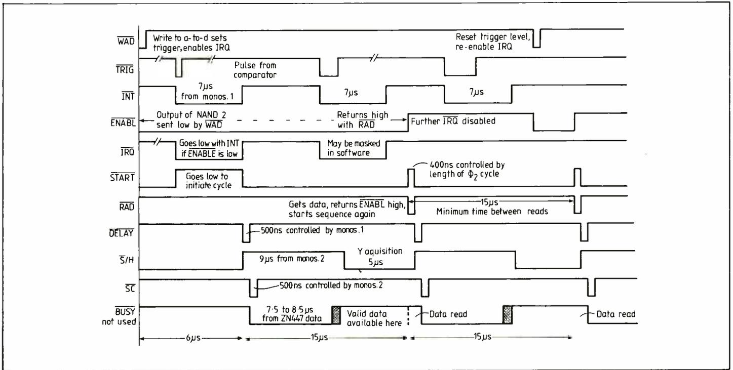
The rear edge of DELAY is used to produce  $\overline{SC}$  which is also about  $0.5\mu s$  long (100ns is all that is required).
