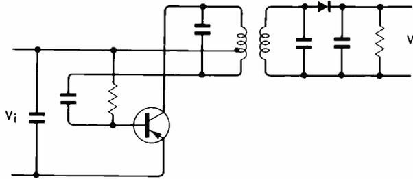
Fig. 4. Fig. 3 developed into a self-oscillating transmitter/receiver with a direct-current output.
