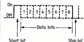
Fig. 10. Frame composition of S5/8 data. No parity bit is included because error-correction is intended to be done block-by-block. Sending rate is normally fixed at 9600 bit/s.
