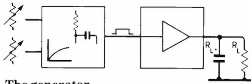
**Fig. 1. The generator comprises two functions, generation and power output.**
