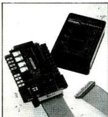
Interpack 1 includes an eight-channel a-to-d converter.
