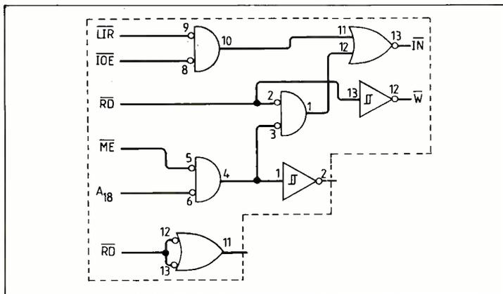
**Control logic for the 64180 computer board.** Signals MUX, RAS and CAS are for the d-rams and ROM selects the eeprom for reading at switch on or after reset. Link 4 determines whether the rom is switched out of the memory map following an i/o operation or following occurrence of an external signal through connector pin 22c. Part of the gating is shown in intentional logic (top).
