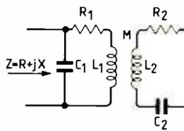
Fig. 9. Coupled circuits, Shunt-resonant primary.  $R_1$  and  $R_2$  are the r.f. resistance of  $L_1$  and  $L_2$  respectively.
