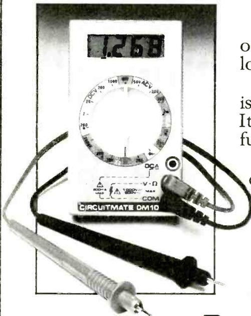
This 3½ digit multimeter has a basic DC accuracy of 0.8%, compared with 3% of full scale on most low-cost analogue instruments. For around £32.
