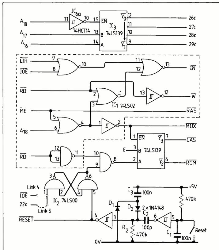
64180 computer board main circuit. Because the microprocessor has integrated peripheral functions, a computer with memory management unit, two d.m.a. channels, three serial channels with programmable bit-rate generator, two-channel
