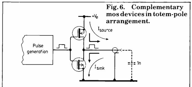
Fig. 6. Complementary mos devices in totem-pole arrangement.
