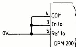
Although COM will sink a large amount of current to maintain its level below V<sub>+</sub>, it cannot source more than 10-20μA and can easily be pulled down to the lower potential.
