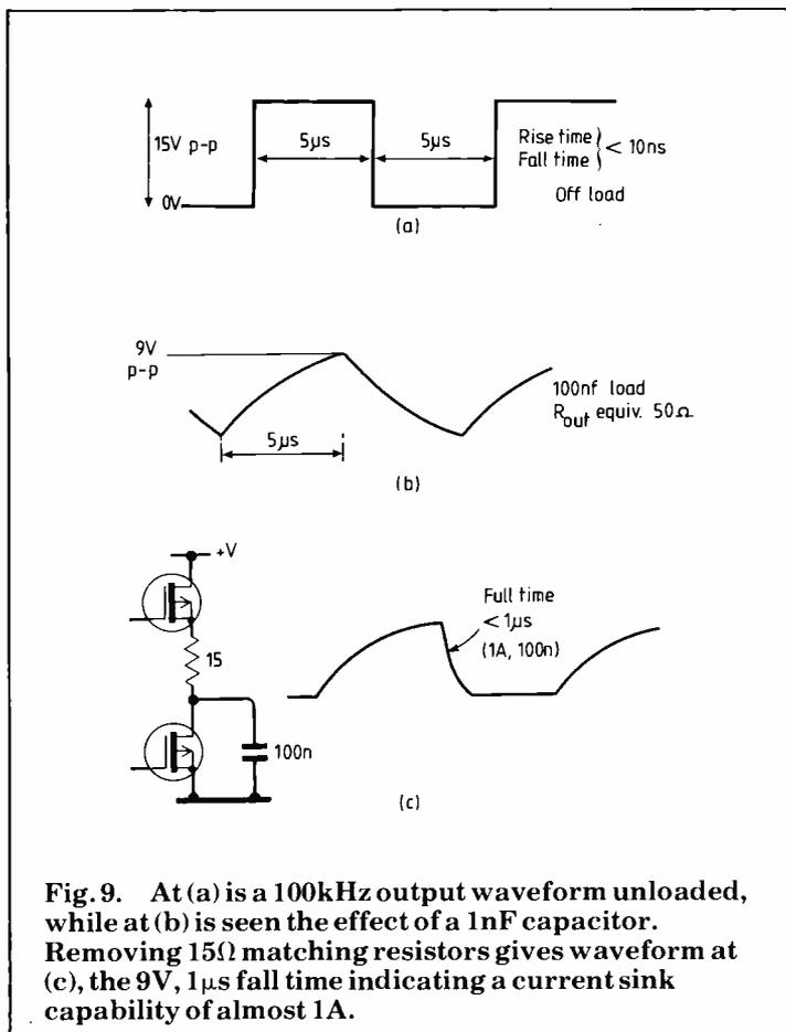
Fig. 9. At (a) is a 100kHz output waveform unloaded, while at (b) is seen the effect of a 1nF capacitor. Removing 15Ω matching resistors gives waveform at (c), the 9V, 1µs fall time indicating a current sink capability of almost 1A.
