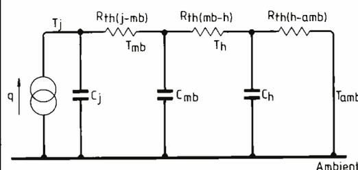
**Fig. 4.** The electrical analogue of thermal flow problem is a typical low-pass filter. Steady-state conditions corresponds to the d.c. case in the electrical circuit. If the thermal capacitances are large, a considerable time may elapse before steady conditions are reached. Designers sometimes exploit this on the assumption of intermittent loads, (in an amateur transmitter, say).
