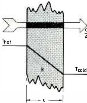
**Fig. 3.** The assumption that a linear temperature gradient occurs under steady state heat flow normal to the surface of conducting wall is illustrated. The slope of the gradient is directly related to the thermal conductivity of the wall.
