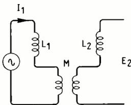
Fig. 2. Much of the inductance in Fig. 1 is leakage-uncoupled-inductance.
