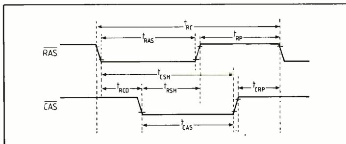
**TABLE 1. Address timing parameters of three 150ns 64K × 1 drams**
