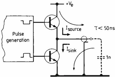
**Fig. 5. Complementary output provides high speed, but limited voltage swing.**
