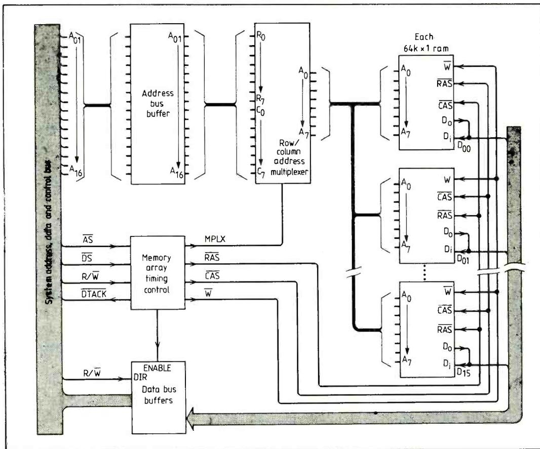
bit) addresses. The two data strobes,  $\overline{LDS}$  and  $\overline{UDS}$ , select the lower or upper or both bytes of the word addressed by  $A_{01} - A_{23}$ .
