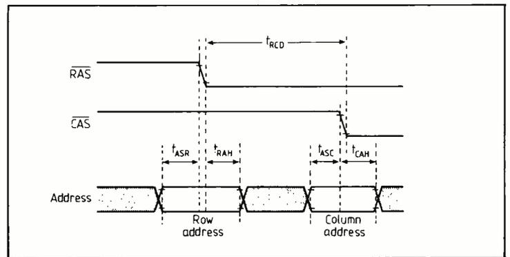
Fig. 5 is  $t_{RCD}$ , the row to column strobe lead time. For the HM4864-2 the minimum value of  $t_{RCD}$  is quoted as 20ns, and the maximum value as 50ns. These limiting values are not fundamental parameters of the memory - they are derived from other parameters. The minimum value is determined by the row address hold time plus the time taken for the address from the multiplexer to settle. The maximum value is a pseudo-maximum. It is not a maximum determined
