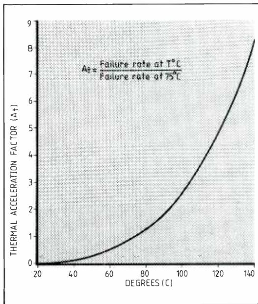
Fig. 1. There is a rapid rise in the failure rate of electronic components as the temperature goes up. This is the same as saying that the reliability worsens. Even at temperatures considerably lower than the absolute maximum allowed, the lifetimes may be much reduced.
