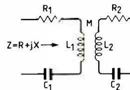
Fig. 7. Coupled circuits, series-resonant primary.  $R_1$  and  $R_2$  are the r.f. resistance of  $L_1$  and  $L_2$  respectively.
