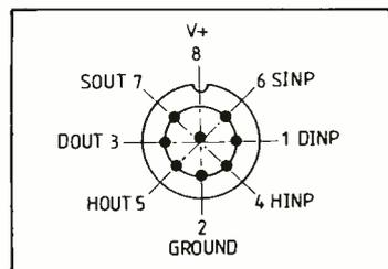
**Fig. 6. Socket contact assignment.** Poles 6 and 7 are reserved for future use.
