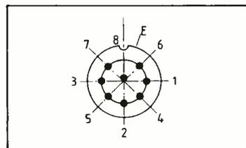
**Fig. 5. Socket pin numbering (mating face view).** S5/8 is based on an eight-pole DIN connector, but leads fitted with five-pin plugs will suit most purposes.
