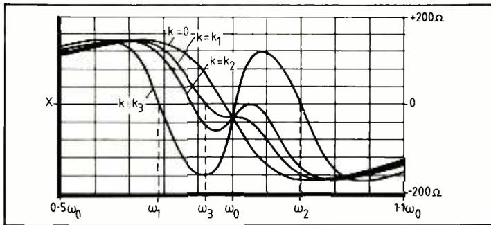
**Fig. 10. Reactive part of the impedance seen looking in at the terminals in Fig. 9. Ls, Cs and Qs as for Fig. 8.  $k_1=0.05$ ;  $k_2=0.065$ ;  $k_3=0.1$ .**
