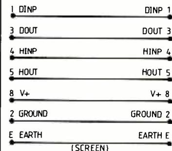
Fig. 9. Extension cable, suitable for insertion at the points labelled X in Figs 1 & 2 last month.
