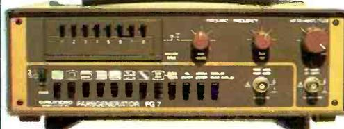
Versatile enough to check-out TV receivers, monitors and VTRs, this compact generator is at home in the field as it is in the lab or workshop. In addition to 15 monochrome and colour image signals, further picture patterns can be achieved by superimposition. Eight station frequencies can be recalled from memory for rapid test capability — even for special bands and the IF output.
