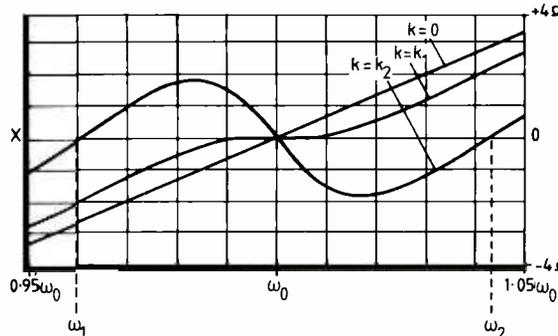
Fig. 8. Reactive part of the impedance seen looking in at the terminals in Fig. 7. In this example,  $L = 1 \mu\text{H}$ ;  $C = 1 \text{ nF}$ .  $Q_1 = 10$ ;  $Q_2 = 20$ ;  $k_1 = 0.05$ ;  $k_2 = 0.1$
