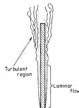
**Fig. 5. The flow along a vertical plate or fin is often complex. There is a region of laminar flow - and the building up to this at the bottom. Further up the fin, if it is long enough, the flow breaks up into turbulent region. The removal of heat per unit area of fin differs in the two regions.**
