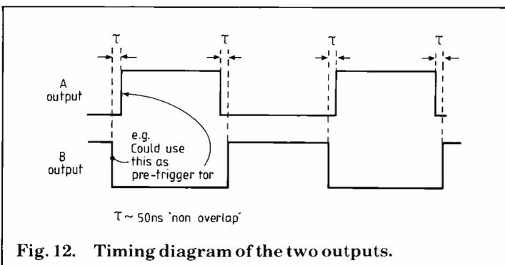
Fig. 12. Timing diagram of the two outputs.
