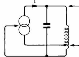
Fig. 6. Skeleton shunt-resonant self-oscillator in Hartley form.
