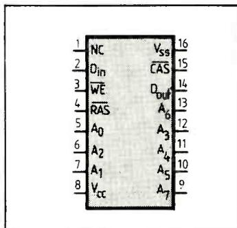
Fig. 2. Pinout of HM4864-2 64K dynamic ram.
