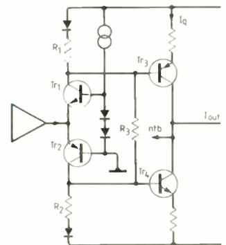
Fig.2. Skeleton circuit of the Margan amplifier. This is very similar to the Blomley design, although the Blomley system does leave each output transistor permanently conducting, while allowing the drivers to switch off.
