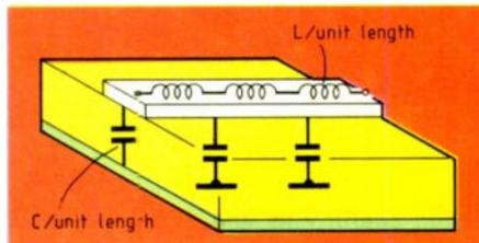
Fig.2. Analogous behaviour of a microstrip with inductance along the length and capacitance through the substrate.
