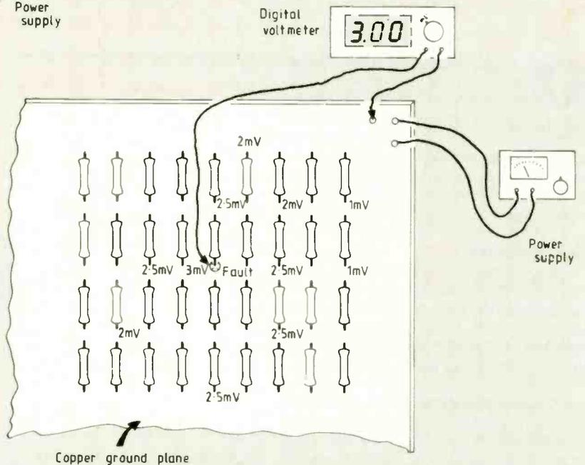
lead resistance has no effect so long as the current source is adequately good and the voltmeter input impedance is sufficiently high. There is no requirement that the lead lengths or resistances be equal in this system. Fig.1(c).
