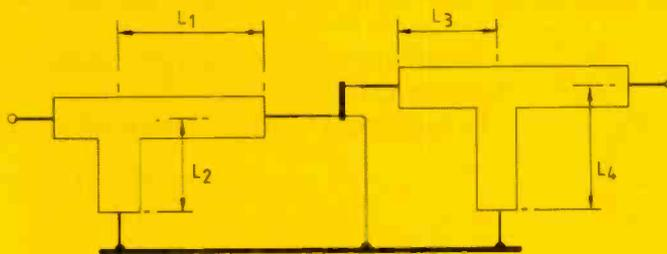
Fig.6. Basic construction of a single-stub matched amplifier.
