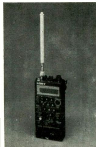
Another new radio from Sony is the ICF7600DA which offers an analogue dial in addition to the digital display, and includes a clock and timer. It offers 12 s.w. bands along with v.h.f., m.w., and l.w., with up to 15 preset stations. More details from Sony UK Ltd, South Street, Staines, Middlesex TW18 4PF. Tel: 0784 67000.
