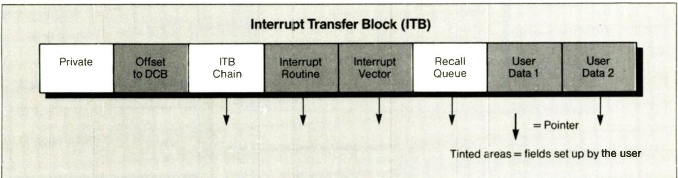
Fig.6. This structure is used by the external interrupt handler to identify the source of an external interrupt. Each block contains an interrupt routine responsible for servicing a particular kind of interrupt.
