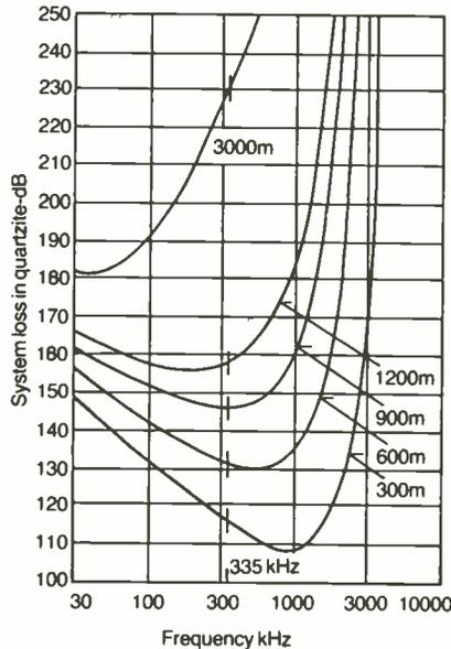
Fig.1. For any communication distance through a lossy dielectric medium like rock there is an optimum transmission frequency. Fig.1 shows, in theory, how that frequency decreases as the required range is increased. In addition, the attenuation through the rock and the inefficiency of electrically small antennas both contribute to the overall system loss.
