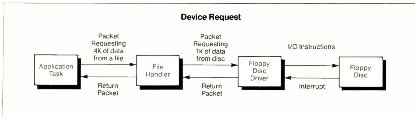
Fig.1. The file handler forms high-level interfacing between the applications task and floppy-disc driver. Low-level interfacing between the file handler and disc is carried out by the disc driver. This technique facilitates device-independent i/o.
