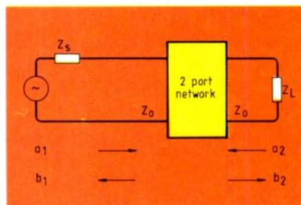
Fig.4. Incident and reflected waves in a transmission line.
