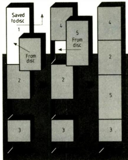
Fig.1. With segmentation, main memory needs to be reorganized when there is no room for a large segment. At (a), memory reorganization is unnecessary when a large segment in ram is swapped for a segment on disc. But at (b), memory needs to be reorganized as in (c) in order to insert the large segment in ram. This reorganization requires complex algorithms.
