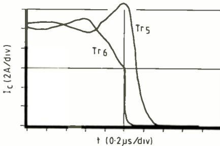
**Fig.4.** Turn-off currents for two typical transistors
