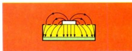
Fig.3. Electrical field surrounding a microstrip. The distribution of the field generates dispersion which varies with frequency.
