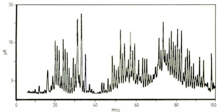
Fig.1. The sharp edges of computer clock and data waveforms couple significant common-mode currents into the mains cable over a wide frequency range. This is a major route for interference emission.
