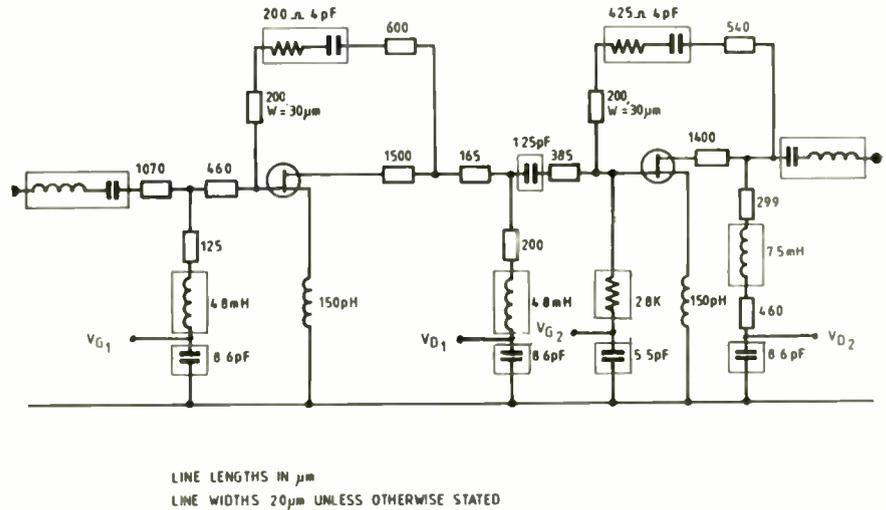
Fig.2. Circuit diagram of a wideband microwave amplifier. All components in boxes can be entered as circuit model elements in a computer-aided circuit design and simulation program.
