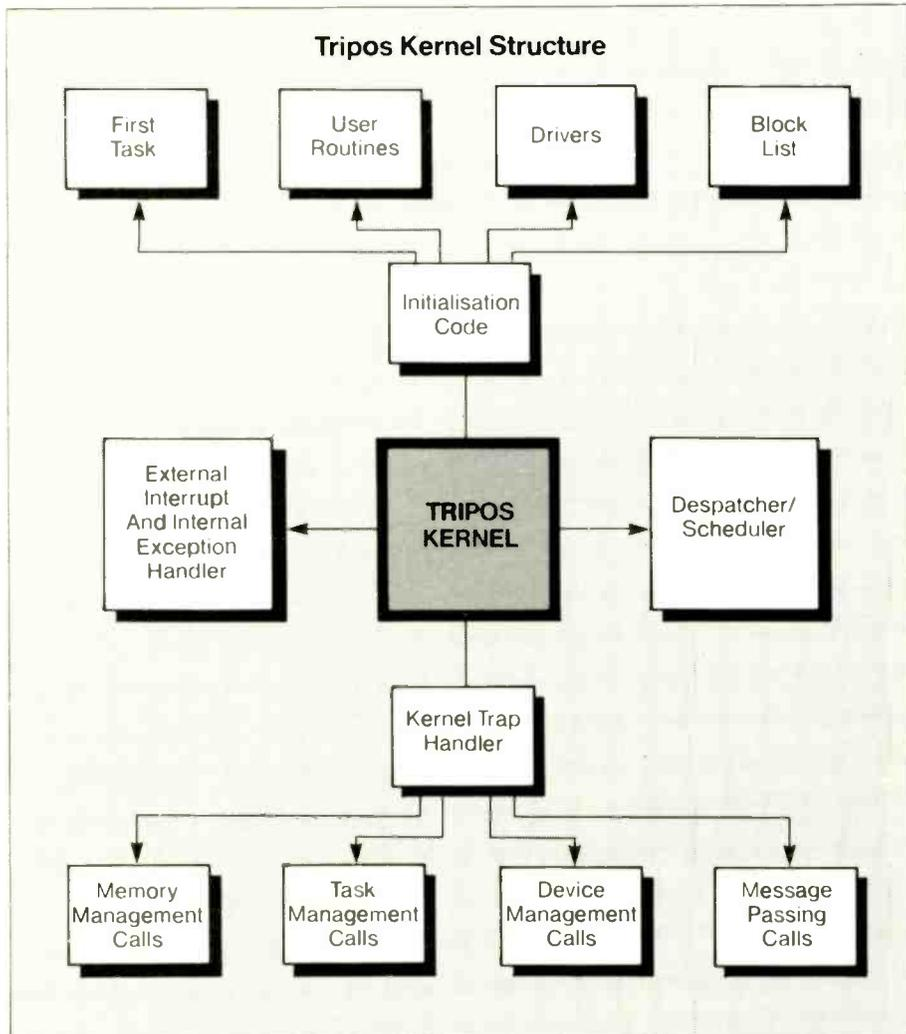
Fig.2. Tripos is structured in concentric layers. These layers become more machine dependent the nearer they are to the centre. Innermost is the kernel, 4Kbyte in size and written in assembly language.
