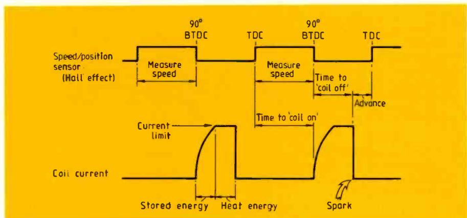
Fig.5. Time-based ignition systems normally use a Hall-effect sensor and metal vane mounted in the distributor or on the crankshaft. A current limit is required for the coil to provide variable dwell.
