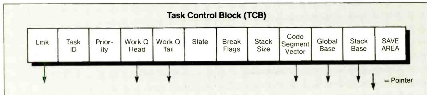
Fig.4. Each task within the system has an associated task-control block containing all information required by the system to manage the task.
