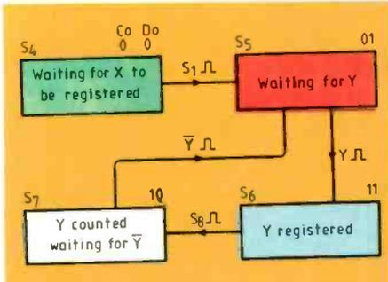
Fig.2. Y-register stores a Y pulse in a similar manner to the action of the X register. At the start of each sequence however it waits in state S4 until the X pulse has been registered before storing a Y. This synchronizes the two registers.
