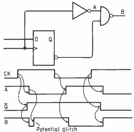
Fig.2 This Boolean equivalent of Figure 3 circuit may produce a glitch at B.
