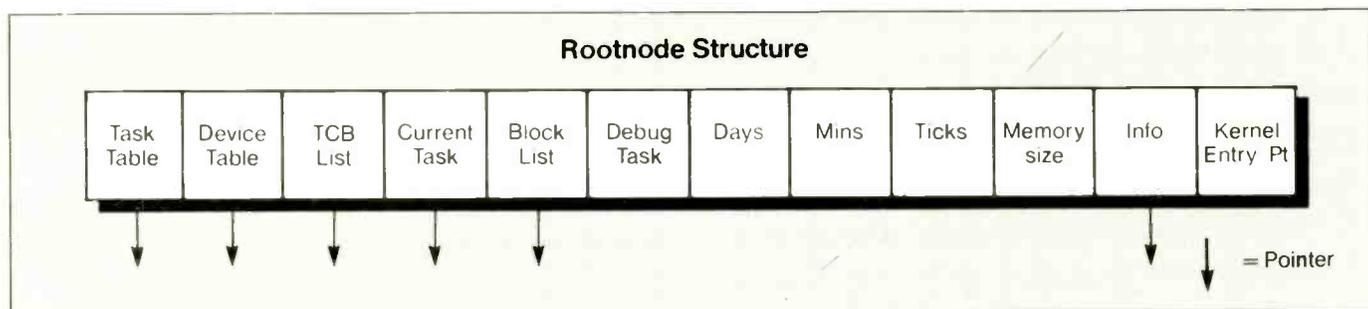
Fig.3. Root-node structure is used by Tripos to keep a record of all aspects of the system. This block is in a fixed position in memory.
