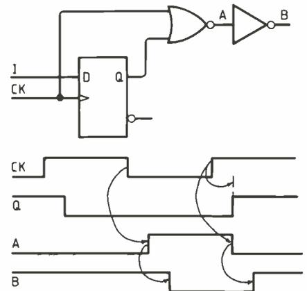
Fig.1 An example of a circuit which gives a glitch-free output at B.
