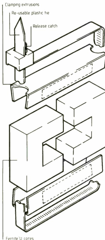
Fig.2. This demountable construction allows a ferrite anti-interference choke to be fitted without rewiring connectors.
