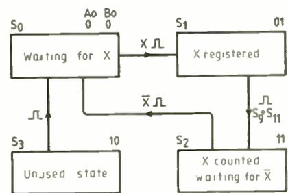
Fig.1 State diagram describes the action of the X register circuit which stores an X pulse by a state change from S0 to S1. When the difference counter enters either state S8 or S12 it counts the X pulse by moving to state S9 or S11. The difference counter then clears the X register by moving it from S1 to S2.
