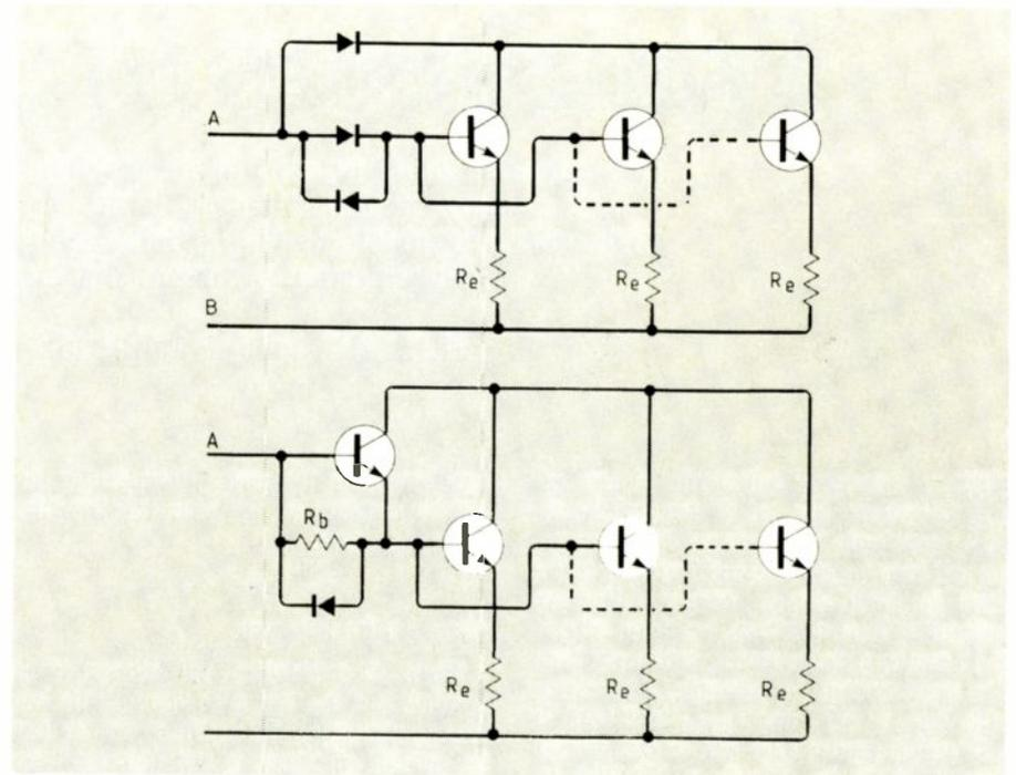
**Fig.5.** Two possible circuit precautions enabling a good sharing of current in saturation and switching conditions
