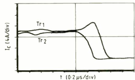
Fig.2 The behaviour of the collector currents of two transistors without (a) emitter resistors and (b) with emitter resistors
