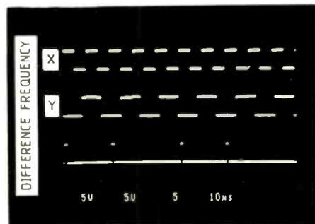
Fig.5. Oscilloscope picture shows a train of X pulses, a train of Y pulses and the resulting difference pulse train from pin 10 of the integrated circuit.
