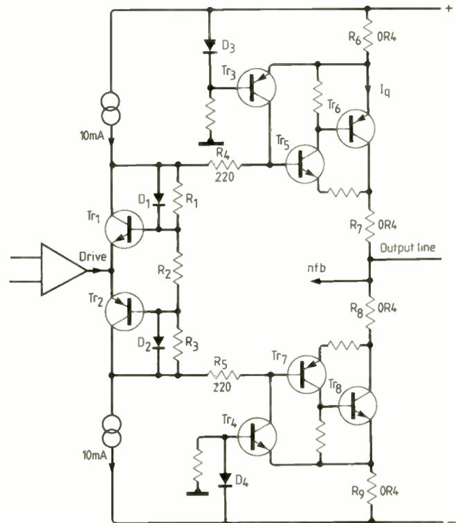
Fig.1. Simplified Blomley amplifier in which  $Tr_{1,2}$  alternately switch on and off but in which  $Tr_{3,4}$  remain conducting due to  $R_3$ . Both circuits feature a fixed voltage-source bias; hence, some part of the circuit must switch if  $I_{out}$  is to exceed  $I_q$ . A true n.s.b. system must include a dynamic variable bias working in opposite direction to the drive, giving bias voltage compliance.
