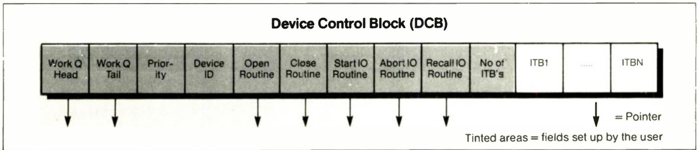
Fig.5. One of these blocks is used for each device in the system. It contains information needed by Tripos to deal with device requests from tasks within the system.
