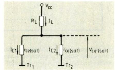
Fig.1. The behaviour of two transistors carrying an overall current  $I_L$
