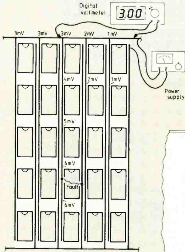
Notice that at the junctions there is a choice of which way to go. Always follow the increasing voltage as this demonstrates that current is flowing in that direction.
