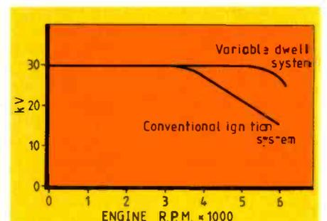
Fig.2. Variable-dwell ignition significantly improves the available ignition potential at higher engine speed and during cranking.
