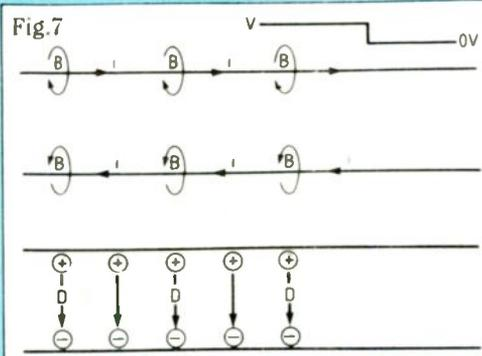
to the right. During this time, extra negative charge appears on the surface of the bottom conductor in the next one foot length, to terminate the lines (tubes) of electric flux which now exist between the top (signal) conductor and the bottom conductor.
