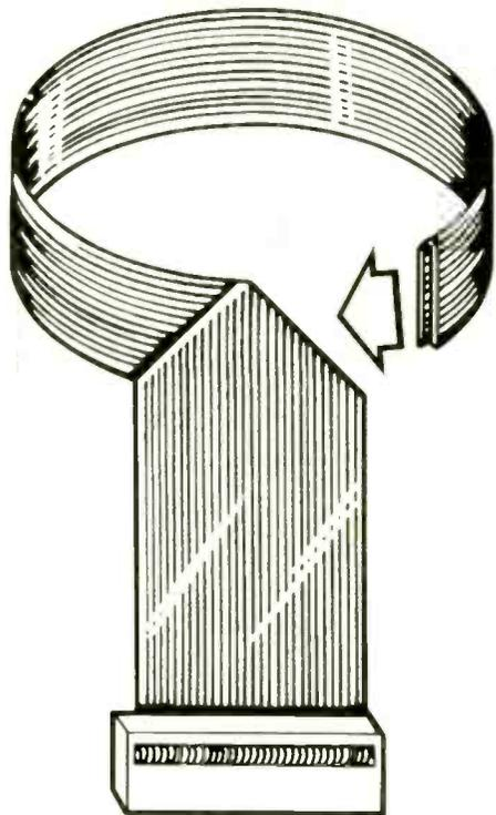
Fig.3. Wide ribbon cables can be folded in half to allow fitting within a demountable ferrite core.
