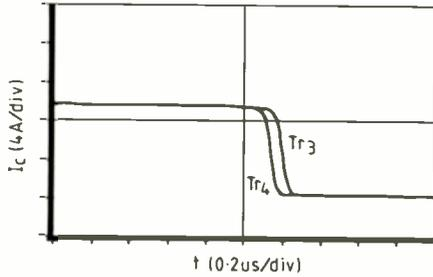
**Fig.3.** Behaviour of the collector currents at turn-off for two typical transistors with a resistive load (a) and an inductive load (b)
