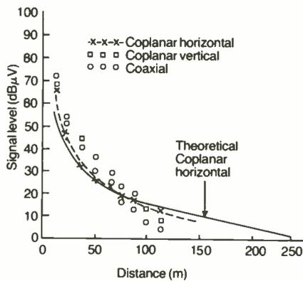
Fig.2. In a stratified medium the relative orientation of the transmit and receive antennas can have a significant effect on the received signal level. Figure 2 shows the signal passing through a near-field/far-field transition as indicated by the change in orientation from coaxial to coplanar horizontal of the loop antennas.
