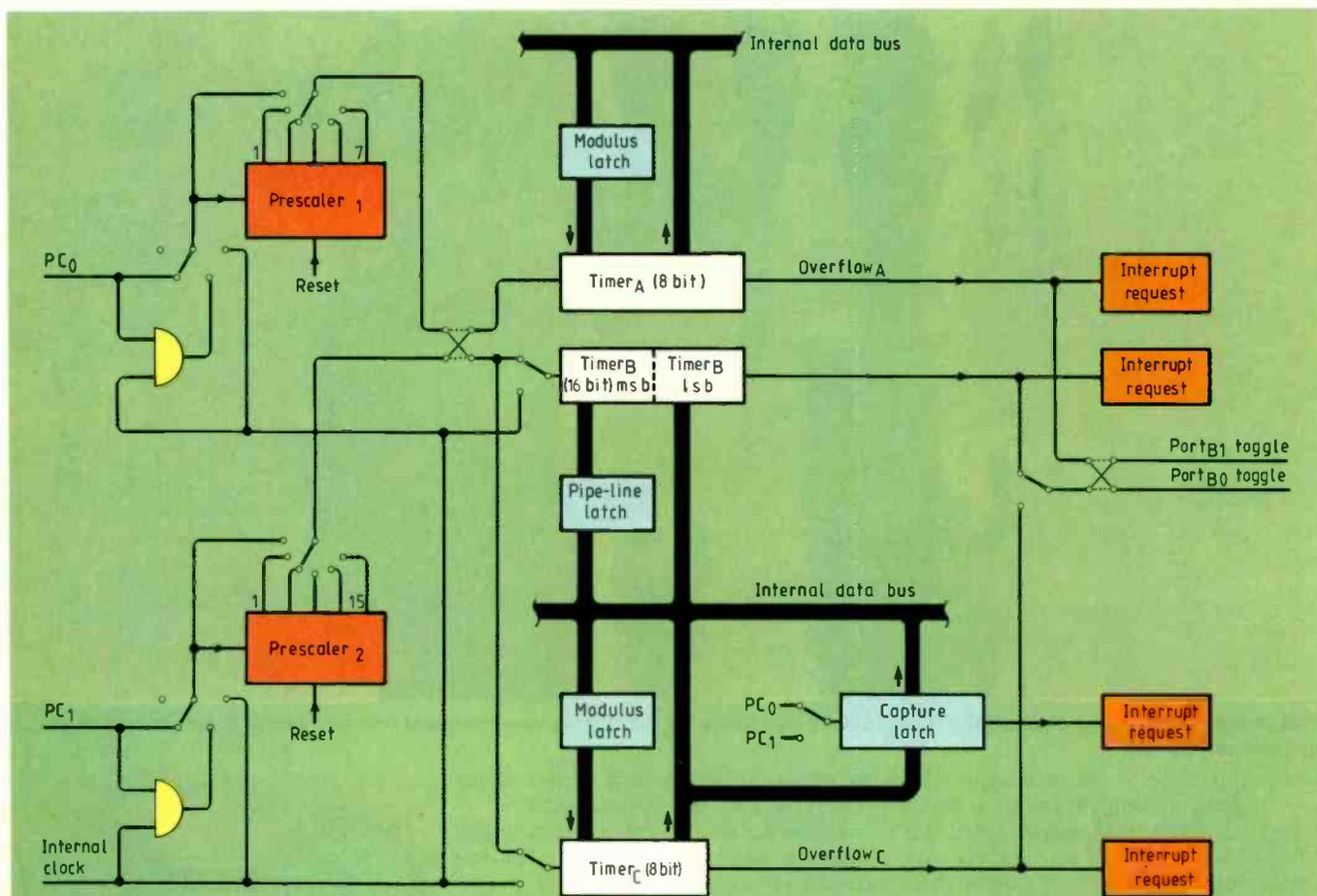
This microcontroller, designed by Motorola for automotive ignition applications, includes three timers, an a-to-d converter, rom, ram, a serial peripheral interface, i/o and a watchdog timer.
