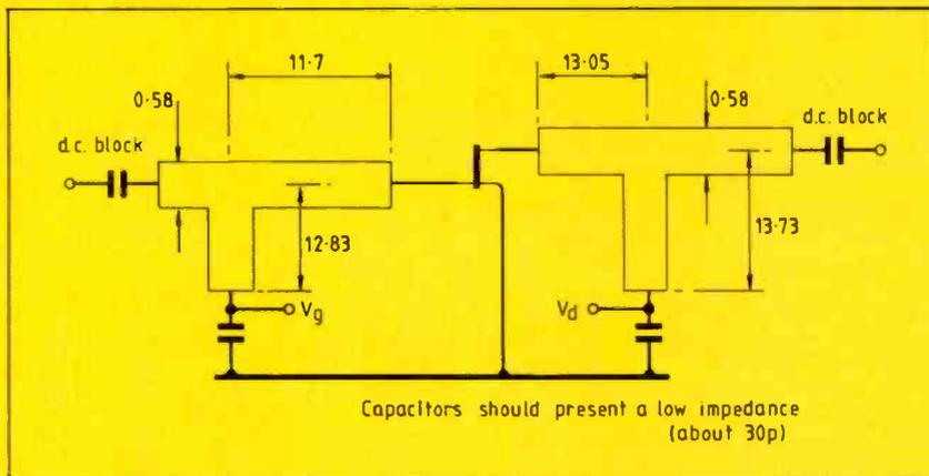
Fig.8. The completed amplifier. The NE72084 fet comes from NEC.
