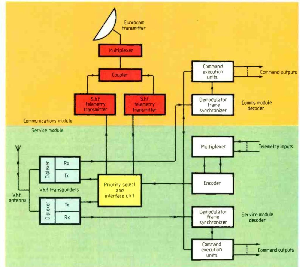
Fig. 1. Spacecraft equipment in the tracking, telemetry and command system used for remote control of the European Communications Satellite.
