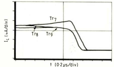
waveforms have been obtained by equalizing the collector currents with emitter resistors, but without any special precautions during the switching phase.
