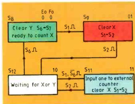
Fig.3. Difference counter counts the first X by moving from state S8 to state S9. When the X register has been cleared, counter is moved to S12 where it waits for either an X or a Y to be stored in the registers. Every X stored before a Y will cause the difference counter to move to S11 producing one difference pulse. A Y will cancel the first X and return difference counter to state S8.
