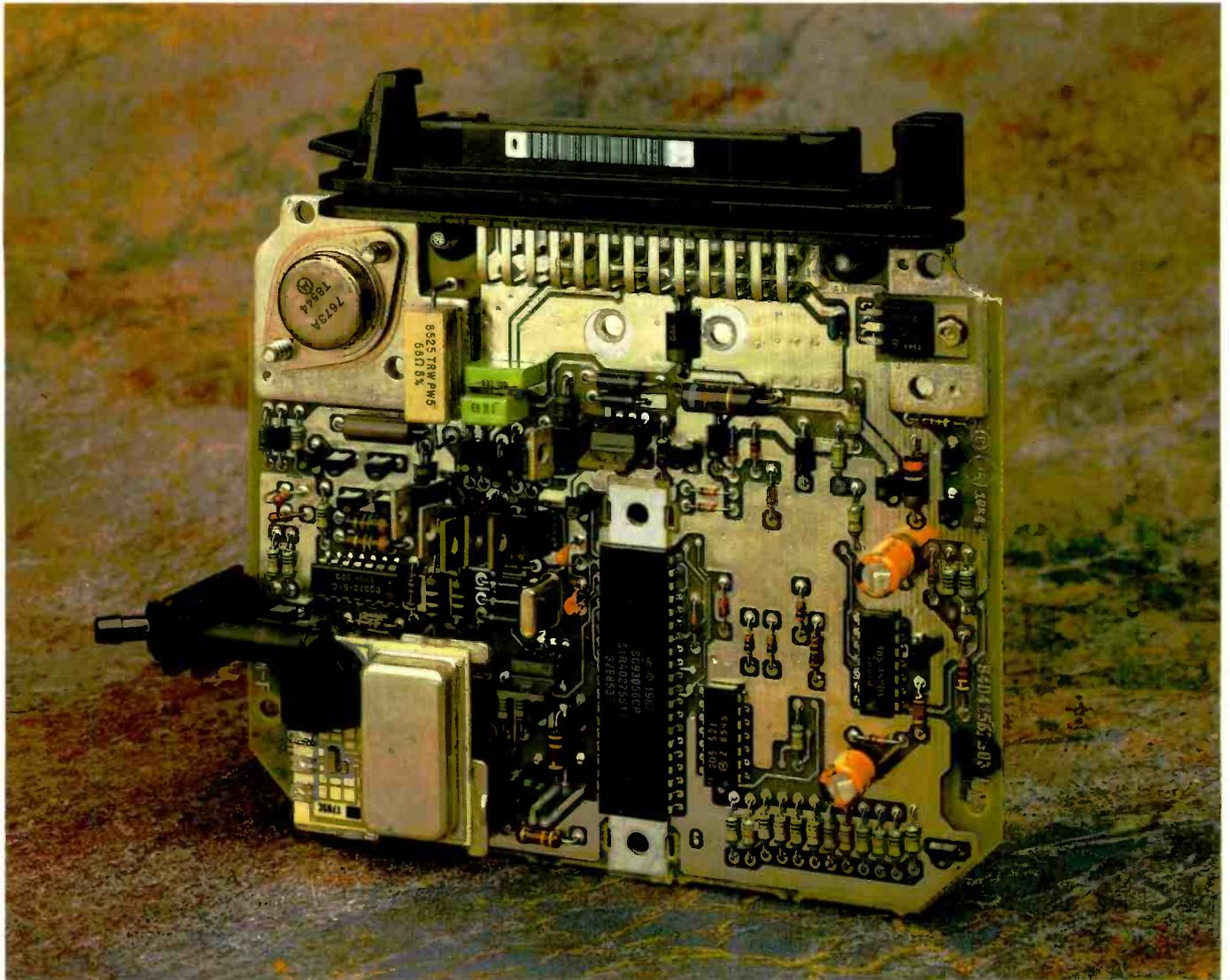
This programmable ignition controller designed for mounting in the engine compartment has an integral pressure sensor and ignition-coil drivers.
