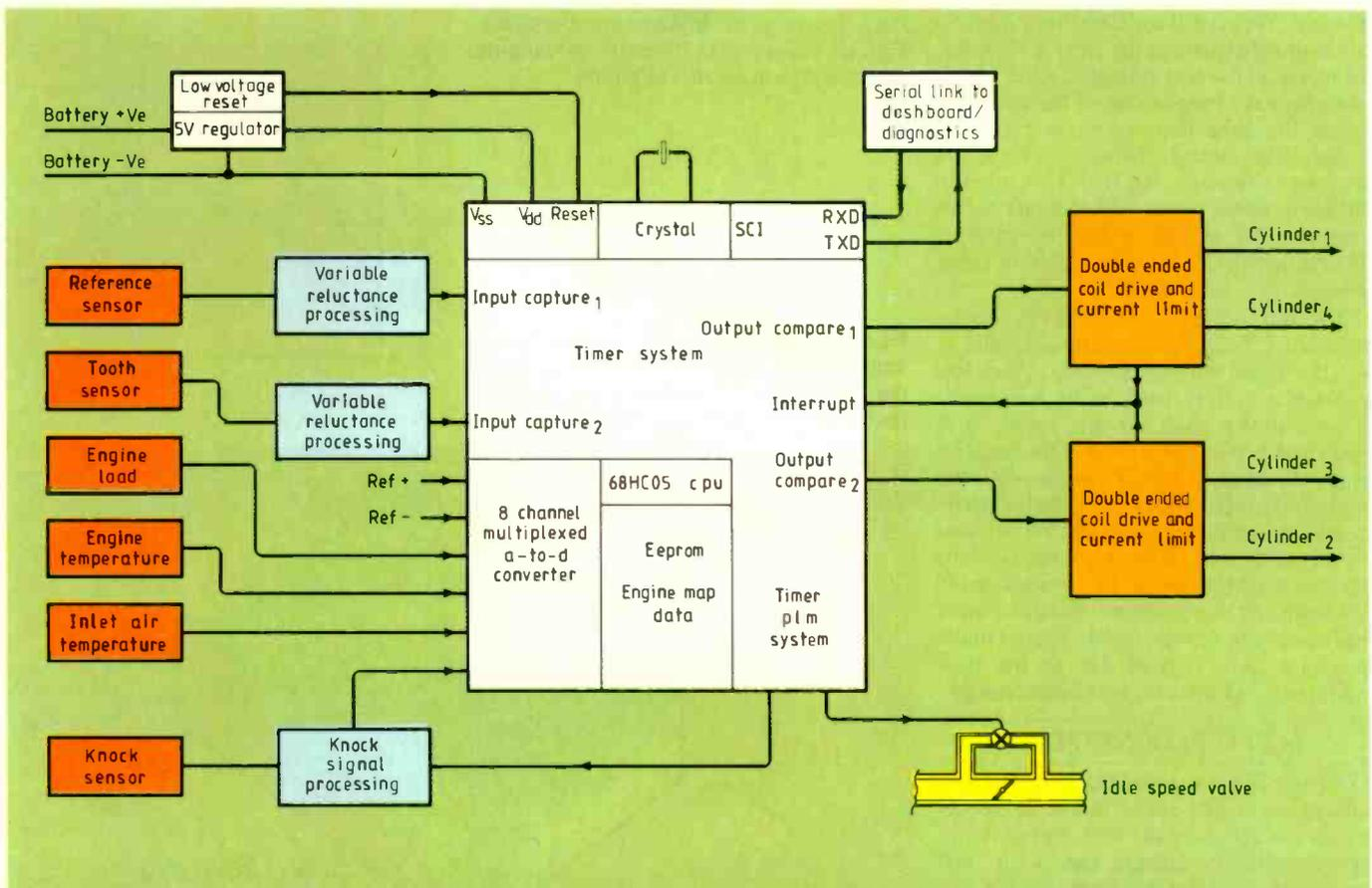
Built into another new microcontroller from Motorola is a powerful timer system which makes the device suitable for a distributorless angle-based ignition system. Included on the chip are an eight-channel multiplexed a-to-d converter, rom, ram, non-volatile eeprom, i/o and an asynchronous serial interface. In this case, the timer is a single 16-bit type, but associated with it are two capture latches and two output compared latches. The eeprom may be used to store calibration
