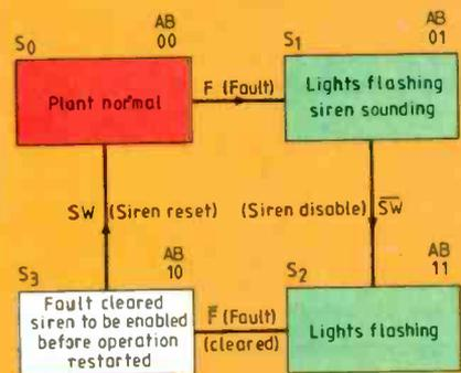
arrow. Under normal conditions the alarm system is in state S0 but when a fault F occurs the alarm moves to state S1 until the switch is operated when it moves to S2. When the fault is cleared the system moves to state S3 where it waits until the switch is returned to the on position before returning to S0.
