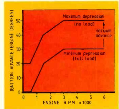
Fig.4. Complexity of a digitally-mapped engine characteristic is restricted only by the amount of available rom and the resolution of the a-to-d converter.
