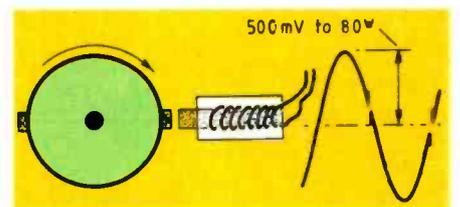
Fig.1. Variable-reluctance (magnetic) transducers are the most common type of speed/position sensors used in engine control, but they have the disadvantage of producing an output which can range from 500mV to 80V peak to peak depending on engine speed.
