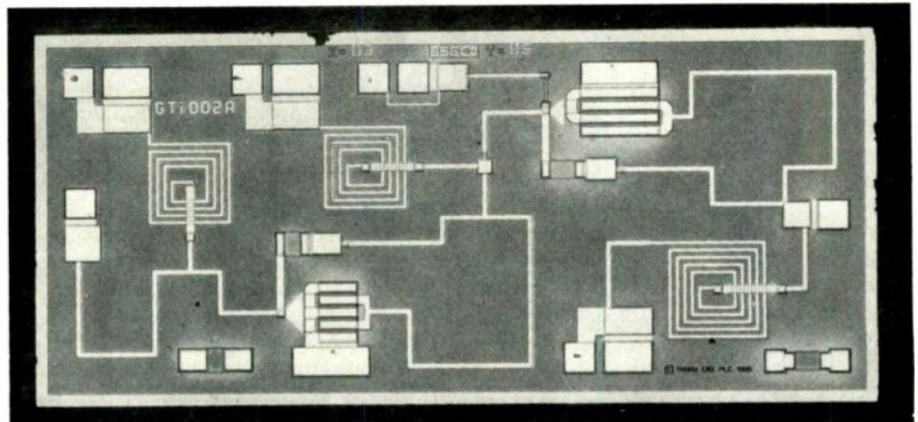
Fig.3. The completed amplifier layout. The gallium arsenide chip is only 1.4 by 3.2mm.
