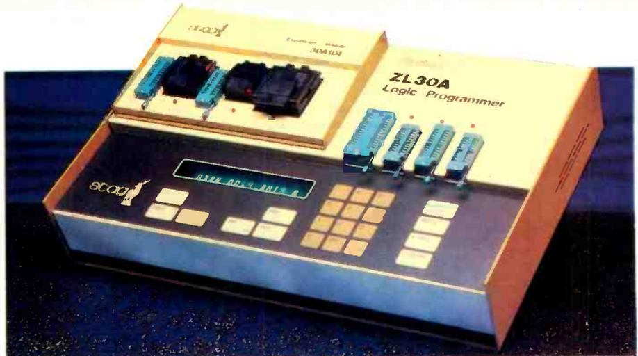
This Stag programmer together with PC and Signetics Amaze software are all that is needed to produce the a wide variety of m.s.i. chips. With an expansion module it will also cater for Mullard's new PML macro logic devices. Details of Signetics programmable logic devices and Amaze software from Paul Whicker on 01-580 6633. Stag are on 0707 332148.
