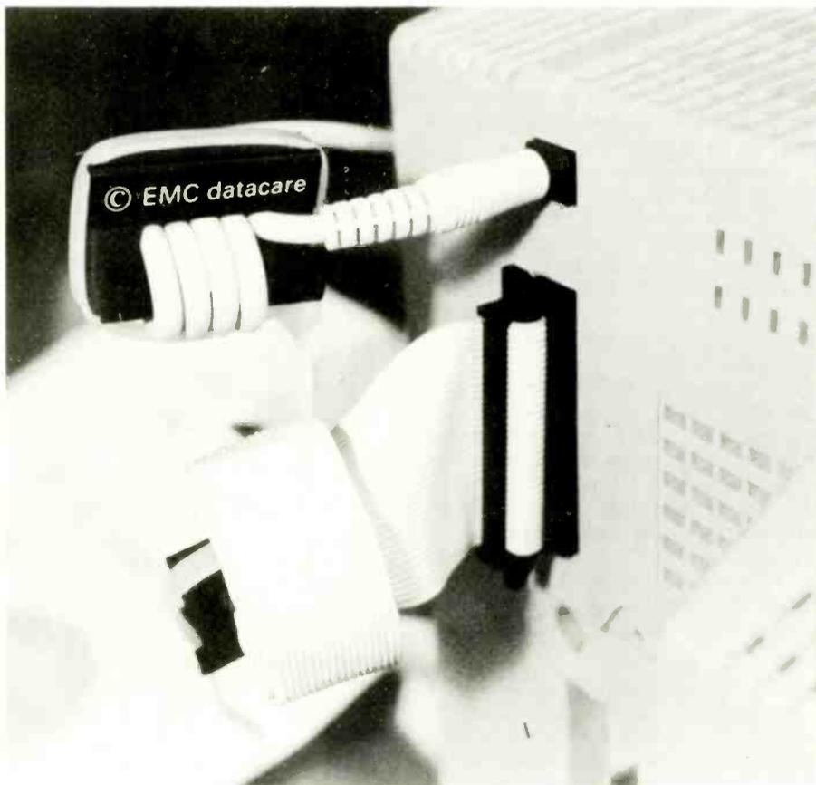
frequencies varied because of resonance in the connecting cables and emission from the computer itself. We noted only a two-fold reduction in emission at 84MHz yet a twenty-fold reduction of the relatively strong emission at 160MHz.
