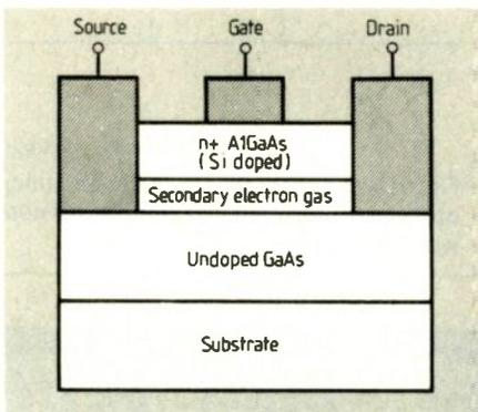
**A concentration of electrons induced in the undoped layer of the hemt becomes highly mobile.**
