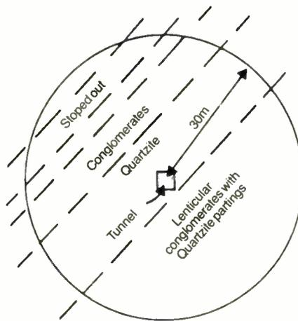
**Fig.3. The inclined strata of a particular test site are shown. A two-plate waveguide of quartzite bounded by higher conductivity conglomerates existed and confirmed a theoretical model which showed how increased range could be achieved by exploiting this natural wave-guide.**
