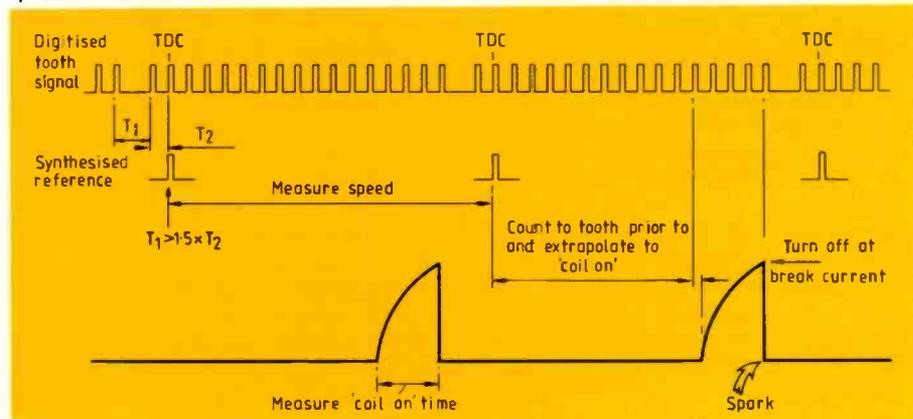
Fig.6. Angle-based ignition with missing tooth reference reduces cost of sensors and eliminates the need for current limit.
