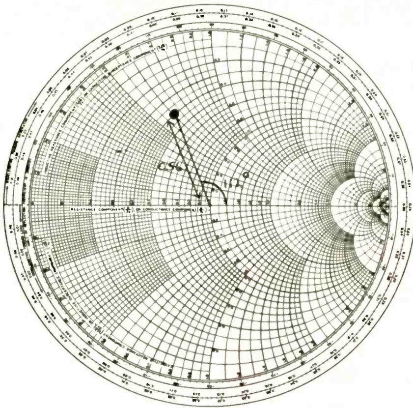
Fig.5. Smith chart is used to calculate reflection coefficients and derive the input impedance and transfer characteristics of a device.
