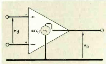
Fig.6. The op-amp, although a complex integrated circuit, has a very simple equivalent.
