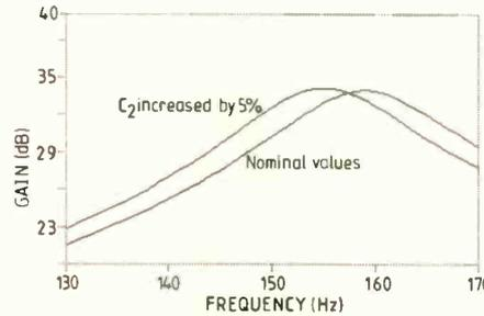
4. Program printout from Linac showing the effect on performance of a single component ( $C_2$ ) change.
