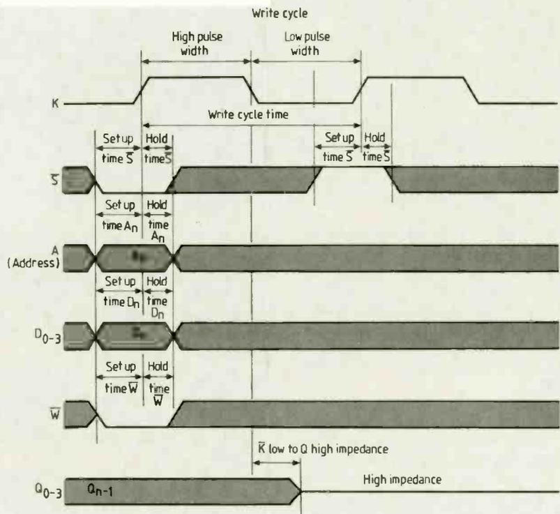
Fig.5. Synchronous static ram write cycle.
