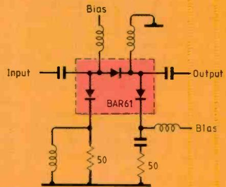
6. (above right) The use of the shunt diodes at either end of the switch produces a non-reflective device.
