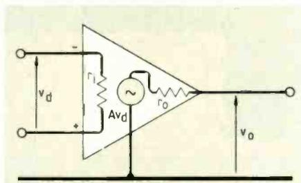
Fig.7. A real op-amp has a slightly more detailed small signal equivalent (and because of internal feedback, this applies to quite large signals also) which complicates the analysis.
