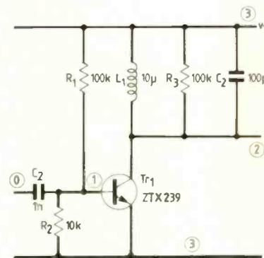
Fig.3. Simple transistor amplifier with tuned output circuit. It has a peaked band-pass response with  $F_0$  around 5MHz (analysis example in the text) Note the numbering of circuit nodes from 0 to 3, and for a.c. purposes, both supply rails are treated as ground. Capacitance and resistance could be added to simulate a more practical circuit.
