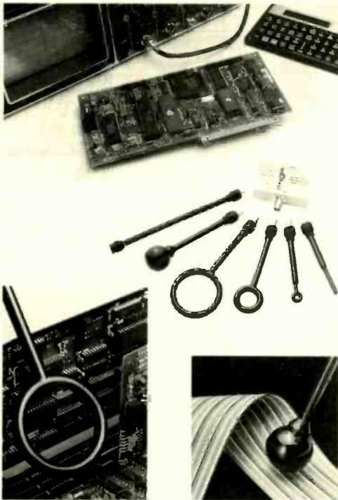
A complete, self-contained set of five probes for quick accurate detection of both magnetic (H) and electric (E) field emissions, even where access is limited. For greater versatility, the set includes a convenient probe extension handle, and is offered with an optional preamplifier.
