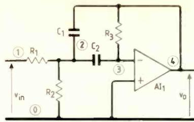
3. The designed bandpass filter with components evaluated to meet the nominal specification can be subjected to sensitivity analysis to perform the tolerancing of the design.
