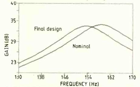
6. Comparison of the performance of the final design with the nominal response. In the final circuit all components are at their maximum excursions of tolerance. Note that the change in gain meets the specification of  $f_0$ .
