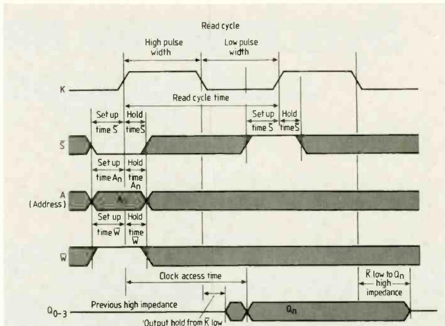
Fig.4. Read cycle of synchronous static ram.
