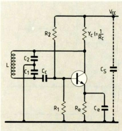
Fig.3. The well known Colpitts oscillator circuit also can yield its secrets by means of the equivalent circuit.
