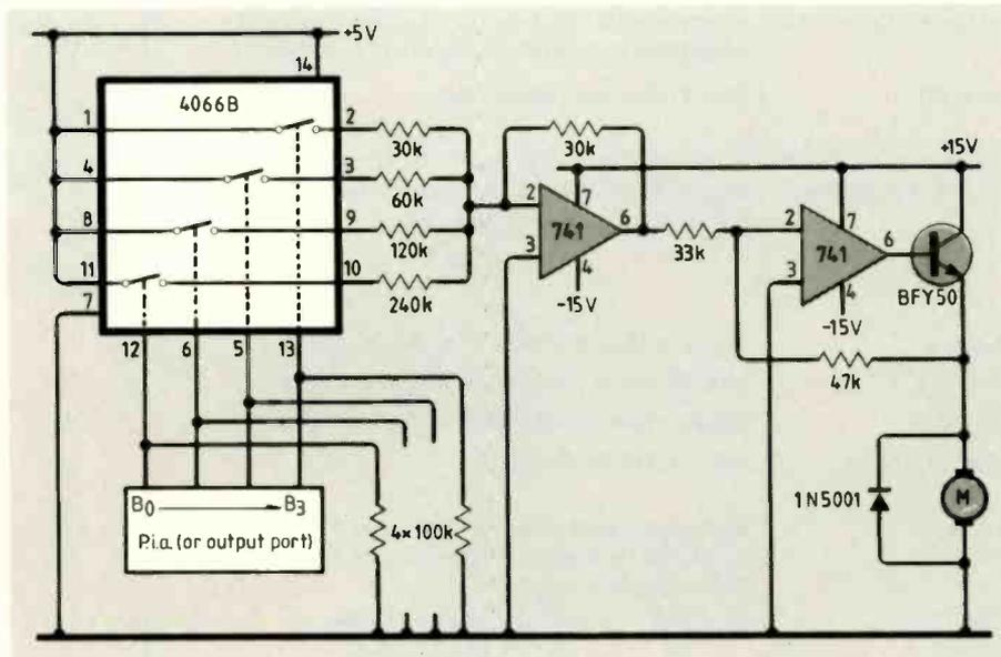
Fig. 1. Hardware for computer speed control of a d.c. motor is simple – most of the work is done by software. Diagram courtesy of Loveday, Practical interface circuits for micros, published by Pitman.
