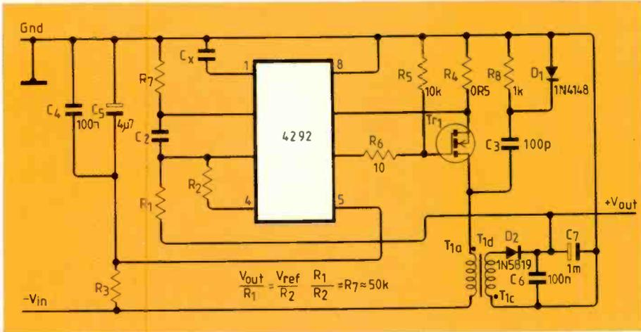
is that it operates with inputs of up to  $-120V$  so it is suitable for use in telephone line-driven supplies. At  $-48V$  input, this circuit is 60% efficient. A dual-output ( $-5.5V$  and  $+5V$ ) regulator specifically for a p.b.x. off-hook supply of  $-48V$  is one of the remaining four circuits given in the specification.
