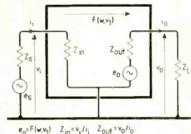
Fig.1. Block representation of circuit-transfer function. Large circuits can be broken down for analysis by chaining several such blocks, perhaps with a simpler transfer function.
