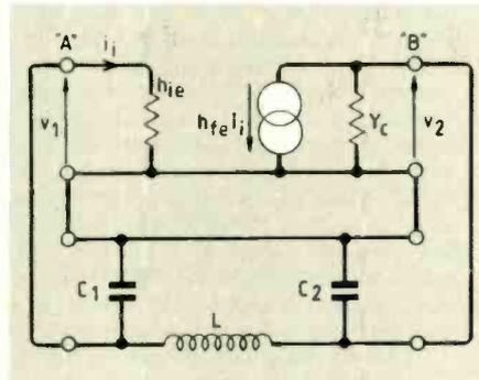
Fig.5. With the same simplifications as for the amplifier, this is the equivalent circuit finally analysed.
