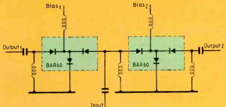
ple s.p.3.t. switch can be built using the BAR60 in the configuration shown in Fig.2.
