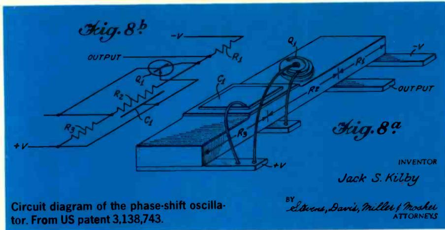
Circuit diagram of the phase-shift oscillator. From US patent 3,138,743.
