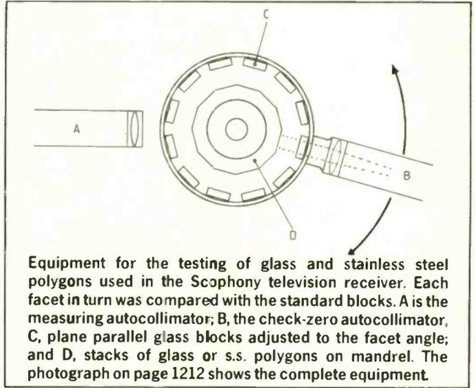
Equipment for the testing of glass and stainless steel polygons used in the Scophony television receiver. Each facet in turn was compared with the standard blocks. A is the measuring autocollimator; B, the check-zero autocollimator, C, plane parallel glass blocks adjusted to the facet angle; and D, stacks of glass or s.s. polygons on mandrel. The photograph on page 1212 shows the complete equipment.
