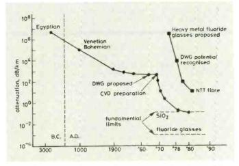
Fig. 1 Fibre attenuation over the past and projected to the future
