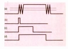
Fig.6. Trigger hold-off is used to overcome the problems of noise or contact bounce. Attempts to measure the signal shown at (a) will result either in extra counts or the short interval in (b). Trigger hold-off uses a monostable period, (c), to inhibit the signal during bounce time to produce the required measurement, (d).
