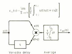
Fig.5. By making observation interval T sufficiently long and progressively varying the time shift  $\tau$ , the signal-processing diagram provides a reasonable approximation to the finite power autocorrelation function.
