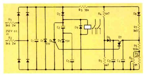
While power is on,  $C_2$  is charged through  $D_2$  and the relay is immediately energized through  $D_3$ . As  $C_3$  charges through  $D_6$  and  $C_4$
