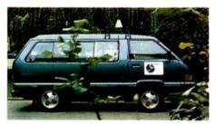
The only thing which distinguishes the Toyota Spacecruiser Van that Inmarsat uses for land mobile trials is the omnidirectional conical antenna made by Denmark's Thrane & Thrane and mounted on a roof rack. One way trials have already been conducted, and two way tests start this month in Italy, Germany, Britain and Spain.
