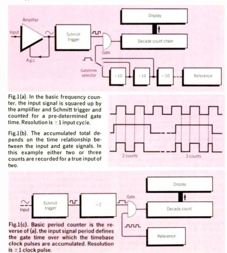
signal is counted for a fixed gate time. If the input signal is fixed, fed from a reference oscillator, the counter will display a measure of the gate pulse length, i.e. a time measurement, Fig. 1(c). For this reason, most general-purpose instruments can offer both frequency and time measurement for little increase in hardware complexity, and are known as 'universal counter-timers'.
