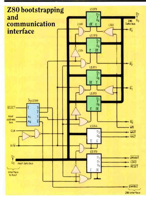
All microprocessors have some means of fetching instructions from a known address at reset. Normally, this address is in eprom, but instructions can be placed directly on the data bus at reset under control of another processor. The Z80 WAIT input makes this particularly simple.
