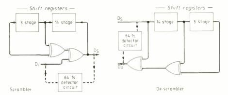
Fig.2. V.22 modems use a form of data scrambling to even out the transmitted energy spectrum.
