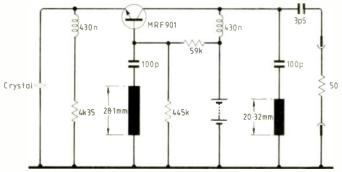
The crystal they use – an ATcut unit resonant at 843MHz – was specially made by Piezo Technology Inc. of Florida, using chemical polishing methods. Although the Q of 6200 at the fundamental frequency is promising from the point of view of phase noise, there are nevertheless spurious resonances at higher frequencies. due to the extreme difficulties of manufacture. Quantity production is therefore likely to be many years away.
