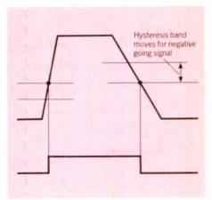
Fig.5. Hysteresis compensation is the solution to the problem in Figs. 3 & 4. By moving the hysteresis band automatically, the actual trigger level remains fixed.
