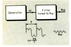
Fig. 1. Basic frequency multiplication process. Fundamental frequency with harmonics passes through a filter tuned to the desired harmonic.
