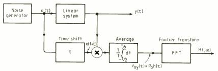
Fig.12. Signal-processing system diagram demonstrating how to obtain the time-domain impulse response h(t) and frequency-domain transfer function  $H(j\omega)$  by white-noise cross-correlation.
