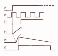
Fig.7. Analogue interpolation increases the resolution of a timing measurement to well beyond the natural limit of the timebase period. The time difference between the 'start' signal, (a), and the next active clock edge used to open the gate, (c), is converted into an analogue voltage by the integrator, (d), which is then discharged at 1% of the charge rate and the discharge time is measured, (f). The result is divided by 100 and added to the conventional measurement.
