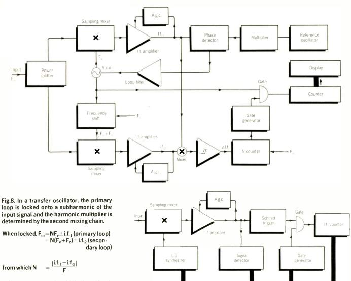
Tolerance to a.m. and multiple signal discrimination can be very good, and depend on the a.g.c.
