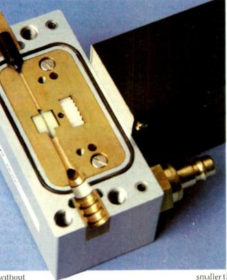
Rudimentary blowing 'head' used in the Leeds trial (below) is superseded by BT's patented design above, which enabled a spliceless link of 3.2km.
