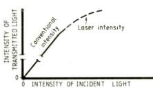
Fig. 3. At low intensity, light output from a given medium is linearly proportional to light entering the medium but when high-intensity laser light is used, transmission becomes non-linear.
