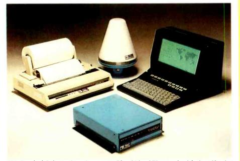
This Standard-C electronics unit measures  $73 \times 214 \times 279$ mm and weighs in at 2kg. Any computer or printer with RS232 interface can be used. Inmarsat say that the cost of equipment will be less than US \$5000; in full production it should be much less. Makers will be Racal, Danish company Thrane & Thrane, JRC in Japan and Sperry in USA.
