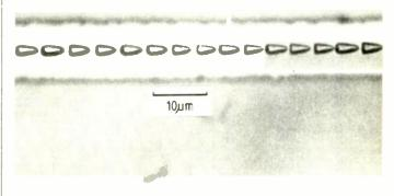
Core region of a fibre after damage, showing oxygen-filled cavities a few wavelengths across.
