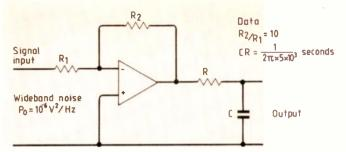
Fig.8. The linear signal processor is made up of a first order low-pass filter of 5kHz bandwidth connected in cascade with an amplifier of gain 10.
