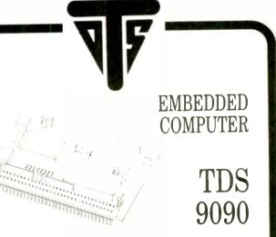
A powerful control computer based on the new Hitachi 6303Y and high level language Forth. 100mm x 72mm. 30K bytes RAM, 16K dictionary RAM/PROM, 256 bytes EEPROM, 16K Forth. You can attach 64 key keyboard, LCD and I<sup>2</sup>C bus peripherals. Built in are interrupts, multitasking, time of day clock, watchdog timer, full screen editor and symbolic assembler. 32 parallel and two serial ports. Single power supply and low power 3mA **operational mode**.
