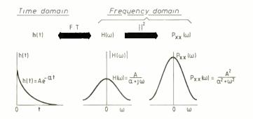
Fig.3. Transformations necessary to evaluate the power spectral density function  $P_{xx}(\omega)$  of time-domain signal h(t).
