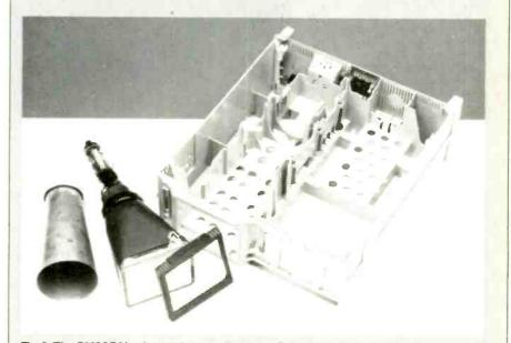
Fig.6. The PM3350's chassis is actually a one-piece injection-moulded frame made from a plastic 'alloy' of polycarbonate and ABS. The frame incorporates all 'click-fit' mountings and stops for p.c.bs and assemblies.
