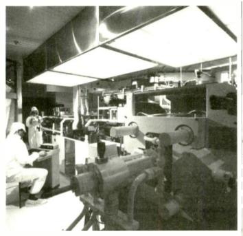
equipment and are produced at a rate of about one every ten seconds in the highly automated plant which includes the latest generation of CD-production machinery.
