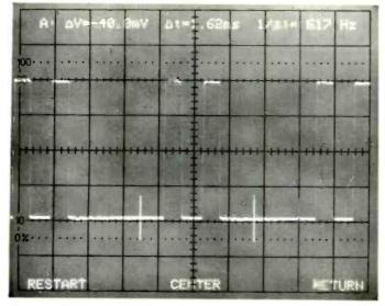
Fig.4. Pressing the 'zoom' (Restart) key automatically calculates the delay and the timebase settings, and....
