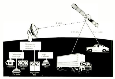
The Imarsat system consists of three basic elements: the mobile equipment consisting of transceiver, terminal, printer, a communications satellite and a fixed earth station. The earth station provides interface with the international telecommunications network.
