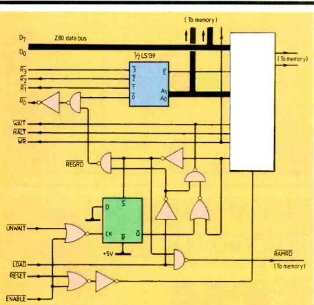
ory is not refreshed. Since it needs refreshing once every 4ms, the bootstrap loading time must be minimized. In the prototype, a simple 58byte bootstrap program that transfers in about 4ms is used. To transfer it, the HL register pair is zeroed then repeatedly used as a pointer to indirectly load immediate data into Z80 memory as follows,
