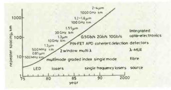
Fig.2 Key milestones for fibre-performance (spacing) projection
