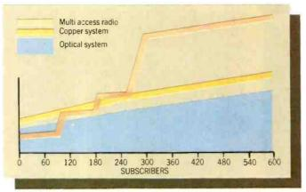
Proximity to an exchange, density of subscriber clusters and growth expectations all contribute to system choice. In general, optical cables, with their inherent bandwidth, are more costeffective where the number of subscribers is high. In a rural application using optical cables and digital multiplex, while initial cost is higher than for a radio system, incremental costs of expansion for new subscribers and new services is much lower.
