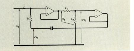
Fig. 10. Varying the effective value of R by feedback.
