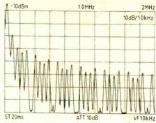
Plot 4. In the spectrum of the sampled serial data stream with the microphone switched off, regularity is caused by the constant direct voltage at the data converter's input.
