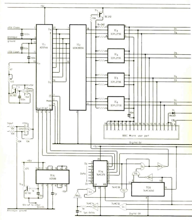
to  $IC_{16}$  sets bit 0 high. Then the user port of the computer is set up to read rather than write. At this point the a-to-d's output is feeding an open-collector buffer. The data is put on the bus by setting the control line high. Then  $IC_{20}$  clocks, the output at pin 9 goes high. Inverter 4 goes low and provides power for any bits for the opto-couplers  $IC_{3-6}$  which are zero. Next the computer reads the data, exclusive-Ors it (it is inverted) and sets
