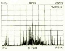
Plot 13. Switching the circuit on with the antenna mounted horizontally shows a slightly different radiation spectrum to that obtained with a vertically-mounted antenna, Plot 11.
