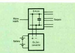
Fig. 4. While the mains supply is health it provides charging current to the battery to maintain it at its float voltage.
