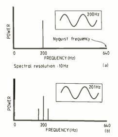
Fig.21. Results of processing synthetic data through FFT program to demonstrate the effects of spectral spreading due to signal truncation. At (a), no signal truncation results in the displayed spectrum agreeing with the anticipated result. At (b), effects of spectral spreading (leakage); 128 samples captured in 100ms. Imaginary input signal: ai[z] = 0
