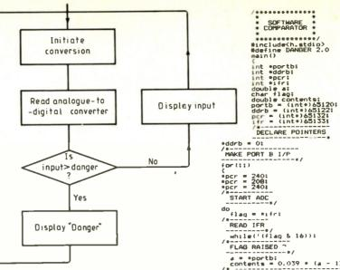
A more satisfactory approach would be to write the software to control the operation of the a-to-d in assembly language. Standard C permits this with the compiler directives #asm followed by the required assembler code and terminated with #endasm<sup>2</sup>. Unfortunately Beebug C does not yet include these directives.
