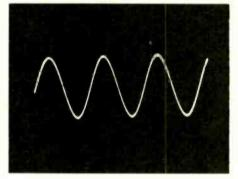
Oscilloscope display, 2V pk-pk, 10Hz.
