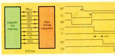
controllers. When this combination is detected by the controller, it asserts BSY. upon which the host releases SEL and the selection data bit.
