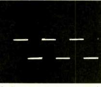
Oscilloscope display, 2V pk-pk, 10Hz (for comparison with a.c.f. display).
