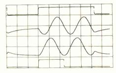
Fig. 8. Upper trace: clock output (IC<sub>4</sub>, Pin 9, 20V/div.) Second trace: phase-sensitive detector (sin)/harmonic oscillator output (IC<sub>3</sub>, Pin 7, 5V/div.) Third trace: phasesensitive detector (cos)/quadrature output (IC<sub>3</sub>, Pin 1, 5V/div.) Lower trace: flip-flop output (IC<sub>4</sub>, Pin 5, 20V/div.) (Horizontal scale 10ms/div.)
