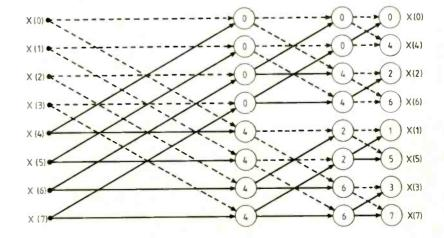
Fig.19. Graphical description of Fourier transform. The a-to-d samples the input signal, loading the real array ar[z] with data. The imaginary array ai[z] is filled with zeros.
