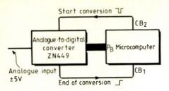
Fig.8. Interfacing an analogue-to-digital converter to the computer via the 6522 versatile interface adapter.
