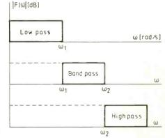
Fig.1. Modelling various filter types by use of low-pass filter.
