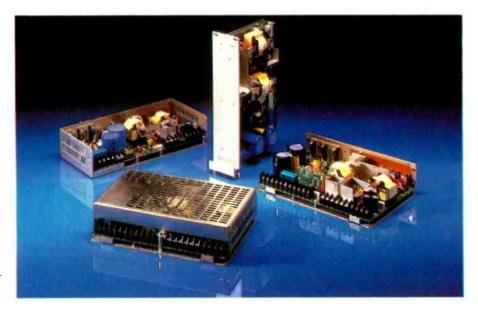
such a system is more complex in terms of component count. It has other disadvantages too such as more noise, both on the input and on the output and is more difficult and critical to design. However, it is very much smaller and lighter than a linear. It is also very much more efficient, and because of these savings it is of lower cost above a few hundred watts.
