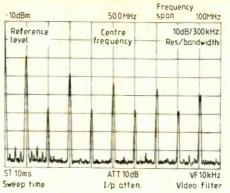
Plot 1. Spectrum of the 10MHz crystal oscillator reveals many harmonics.
