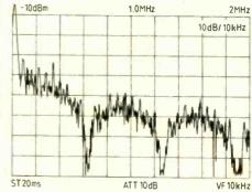
Plot 5. With a 'random' input at the microphone, the serial data-stream spectrum shows rapidly changing data.
