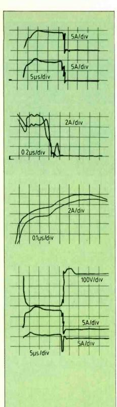
Both bipolar transistors shared the load current equally without selecting matched devices. Top diagram shows collector current while the middle curves are of rising and falling edges with an expanded timebase. Traces in lower diagram are collector voltage and current and base current (bottom). This paralleling technique can be extended using additional parallel b.j.ts, each of which requires a further base drive current transformer; as shown schematically in Fig.3.
