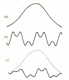
Fig.14. The Hanning function. At (a), the Hanning data window.  $W[i] = 0.5(1 - \cos(2\pi i/N))$ , where i is the sample point number and N the total number of samples. At (b), truncated data to be transformed; and at (c), the effect of multiplying by the Hanning data window.
