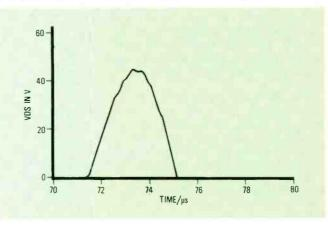
Fig.3. Theoretical waveform using Spice of drain source voltage across a mosfet feeding two-element tank circuit.
