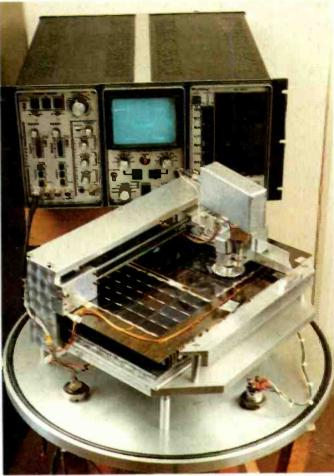
Fig.2. ERA Technology's laboratory equipoment for investigating discharges in solar arrays. The portion of an array is charged up by electron bombardment in a vacuum. Circular table is the base of the vacuum chamber.
