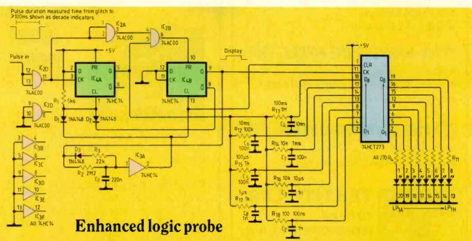
Most existing logic-probe designs indicate that a pulse has occurred, but this one also indicates the duration of the pulse. Having an idea of the pulse width greatly simplifies fault finding. In a microprocessor system for example healthy strobe pulses are typically from 200ns to 1 $\mu$ s wide. Any strobe of less than 100ns or greater than 10 $\mu$ s therefore requires further investigation. Without the probe, a fast oscilloscope would be needed.
