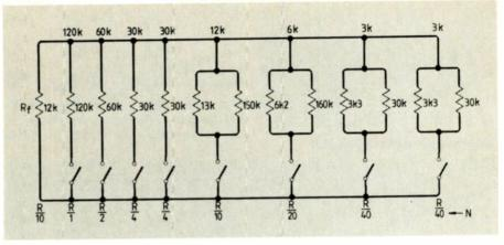
Fig.9. 1,2,4,4 switching combination for frequency control.
