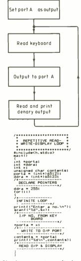
Fig.2. Simple program to monitor keyboard continuously and to write to port A.
