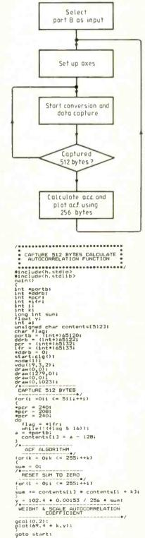
Fig.12. Program to calculate and plot the autocorrelation function.
