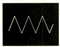
Oscilloscope display, 2V pk-pk, 10Hz.
