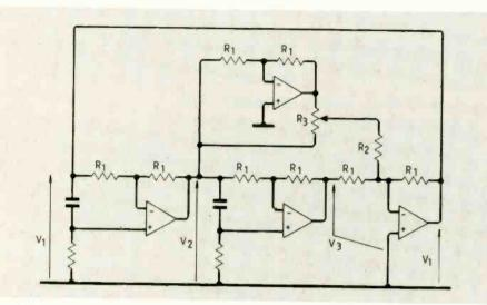
Fig.12. Wide-range frequency control, one variable resistor.
