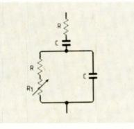
Fig.1. The variable resistor gives a large shift in frequency when R is small and vice versa.
