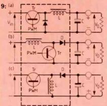
(a) Step-down circuit (buck), (b) step-up circuit (boost), (c) inverting buck-boost circuit.
