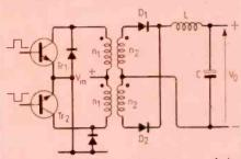
The transistors alternately turn on and the voltage across the secondary will be  $V_{in}$  multiplied by the turns ratio of the transformer. Frequency of the secondary waveform will be twice the switching frequency which means simple filtering on the output can be designed for. Each device must be rated for twice the supply voltage as this is the voltage seen by one transistor when the other is conducting.
