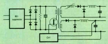
Fig.3. Keeping the input d.c. capacitor charged can be achieved in an alternative u.p.s. by using a d.c. converter to step up the voltage and using this output to keep the capacitor charged.
