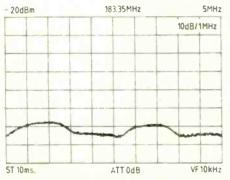
Plot 8. A closer look at one of the spectral peaks from Plot 7 with no audio input.
