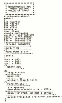
Fig.9. Program to synchronize a-to-d and print decimal value of input signal.
