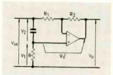
Therefore  $V_3 = V_1/180^\circ - 2\tan^{-1}\omega CR$
