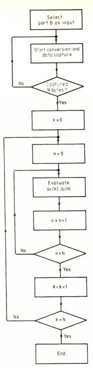
Fig.15. DFT and Hanning window: flow-chart for the program of Fig.16.
