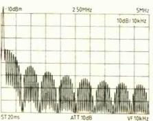
Plot 3. Spectrum of the analogue-to-digital converter start-conversion pulse-train.
