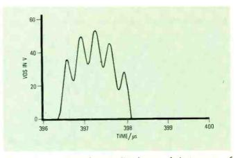
Fig.4. Theoretical waveform predicted across drain to source of mosfet when a modified tank circuit used.
