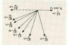
Fig.14. Phasor diagram for V<sub>1</sub> and V<sub>4</sub>  $(-V_3)$  in Fig.12, showing that as exceeds 1/CR, phase angle nears 180 degrees.
