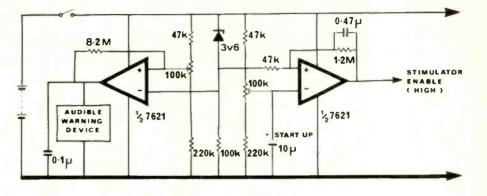
Fig.3. Possible design of battery-discharge manager. During discharge, with the stimulator operating, the battery current is typically 250 mA. At the end of discharge, with the stimulator disabled and the audible warning operating, the remanant battery current is 130  $\mu$ A.
