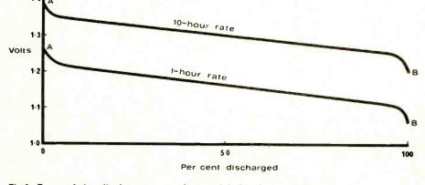
Fig.1. Form of the discharge curve for a nickel-cadmium cell.
