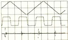
Fig. 7. Upper trace: sensor excitation ( $Tr_1$ ,  $Tr_2$  emmitters, 10V/div.) Middle trace: phase-sensitive detector reference ( $IC_1$ , Pin6, 20V/div.) Lower trace: typical sensor output (500 mV/div.) (Horizontal scale 0.1ms/div.)
