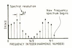
Fig.13b. Discrete Fourier transform. The spectral resolution  $\Delta f$  equals 1/N.T hertz, where N is the number of samples and T the time increment between samples. For example, if the time between samples is 6.5ms and we decide to process 16 points, then the spectral resolution will be 10Hz. Therefore a digitized 50Hz sinewave would ideally be observed as a single ordinate at the sixth sample point.
