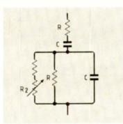
Fig.2. In this arrangement, R<sub>1</sub> gives a small frequency shift when R is small.
