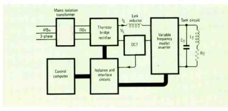
induction heating power supplies to achieve more sophisticated power control, increased reliability and improved system efficiency refs 2,3. The microprocessor control system could also monitor the performance of the supply unit and carry out general supervisory tasks such as the continuous control of the temperature and flow rate of the cooling water.
