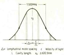
where c is the velocity of light. These are the laser's longitudinal modes.
