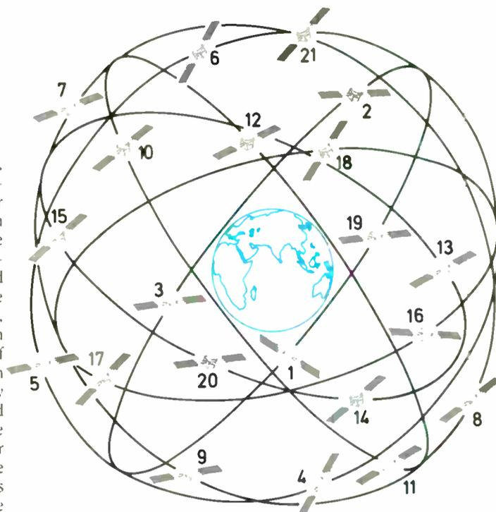
Fig. 1. GPS satellites are not geostationary — they have inclined orbits that take them over any point on their ground track or ce every 12 hours. (Diagram from Ref. 1.)
