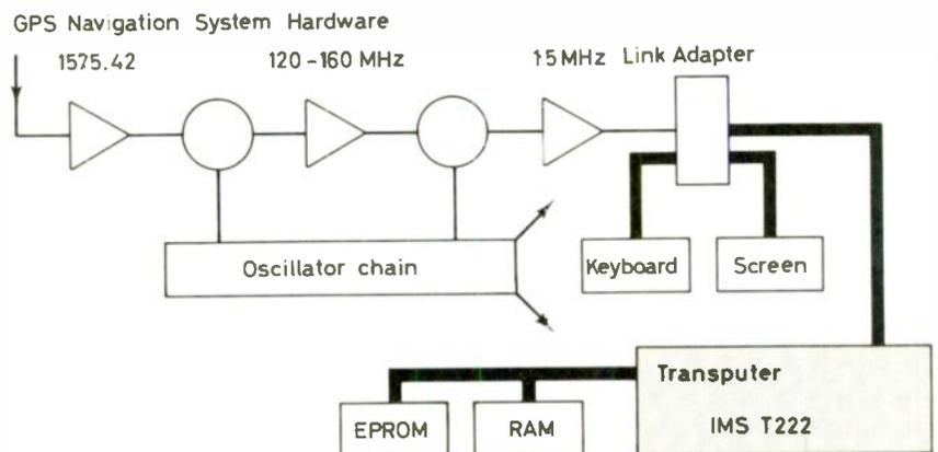
Fig. 5. GPS navigation system hardware. This new system uses the same r.f. section as a traditional system, but conversion is to a lower frequency of 1.5MHz — the lowest frequency that can handle the bandwidth.
