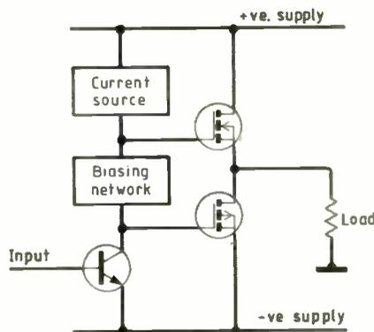
Fig. 1. With this configuration, maximum output power is severely restricted due to the fet's high gate-to-source voltage.
