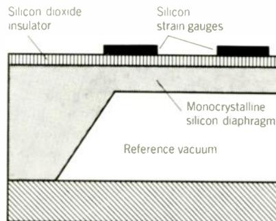
**Diaphragms etched into silicon wafer will be cut into pressure sensors less than 4mm square (Novasensor).**
