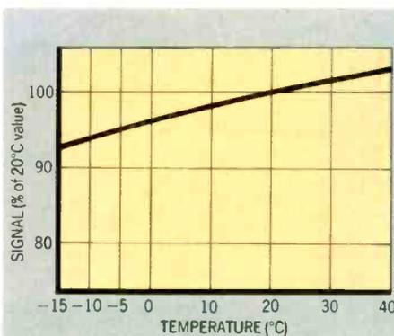
The oxygen sensor has a low temperature coefficient over the range  $-15$  to  $+40^{\circ}\text{C}$ . Curve shows the signal as a percentage of the  $20^{\circ}\text{C}$  value.
