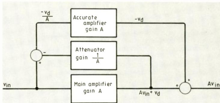
**Fig. 3. Feed-forward amplifiers are inherently stable, so they do not need bandwidth limiting. But addition of the inverted error signal to the output of the main amplifier is not easy to arrange.**
