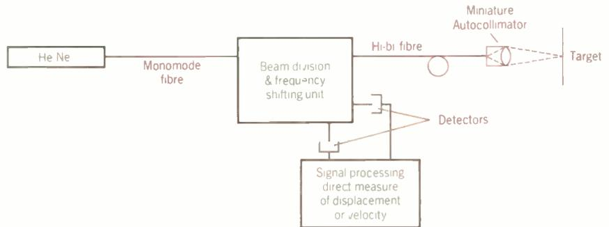
**Non-contact vibration sensor using heterodyne signal processing will be marketed by Cogent Ltd of Ascot later this year.**
