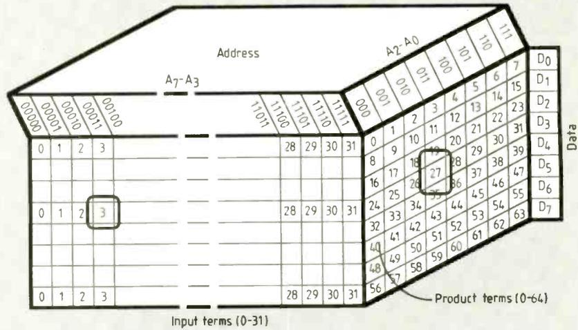
Fig.2. PLD address mapping. For example, (Product Term 27, Input Term 3) (Address 00011011, Data 00001000).
