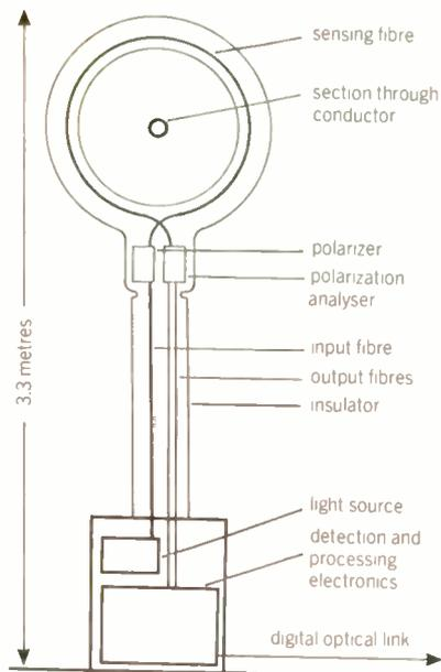
**Prototypes of the Faraday current sensor developed in conjunction with Sifam will be undergoing field trials later this year. One of the unique features of this system is that the polarizer is made in situ on the fibre. The polarization analyser developed especially: it can determine both the ellipticity and the azimuth of the optical beam transmitted through the sensing fibre.**
