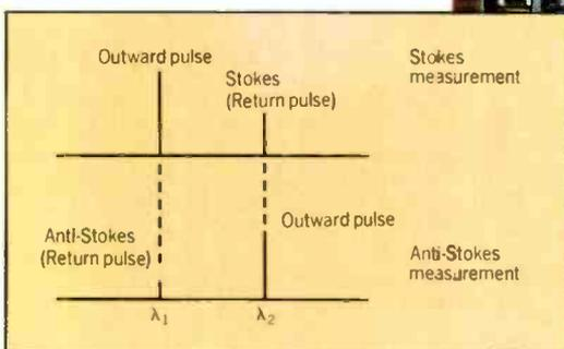
distance through the fibre at each wavelength; outward at one wavelength and returning at the other. The total attenuation is therefore the same for both measurements, irrespective of the spectral attenuation properties of the fibre. A major advantage that results from this is that the Cossor system requires access to only one end of the sensing fibre and will remain accurate irrespective of any changes in cable characteristics.
