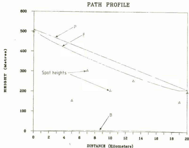
Fig.2. Typical "rough" path profile for a 20km path. This profile is drawn using a K factor of 4/3 and a radio frequency of 950MHz.
