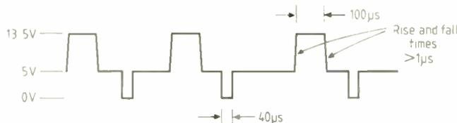
Fig.4. Pin 11 of device under control of pulser test routine.
