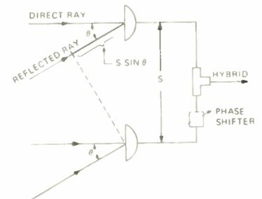
Fig.11. Reception of direct and reflected rays.
