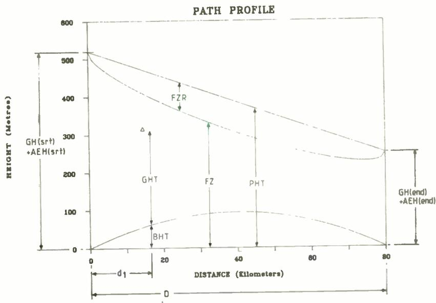
Fig.1. Parameters needed for path profiles.
