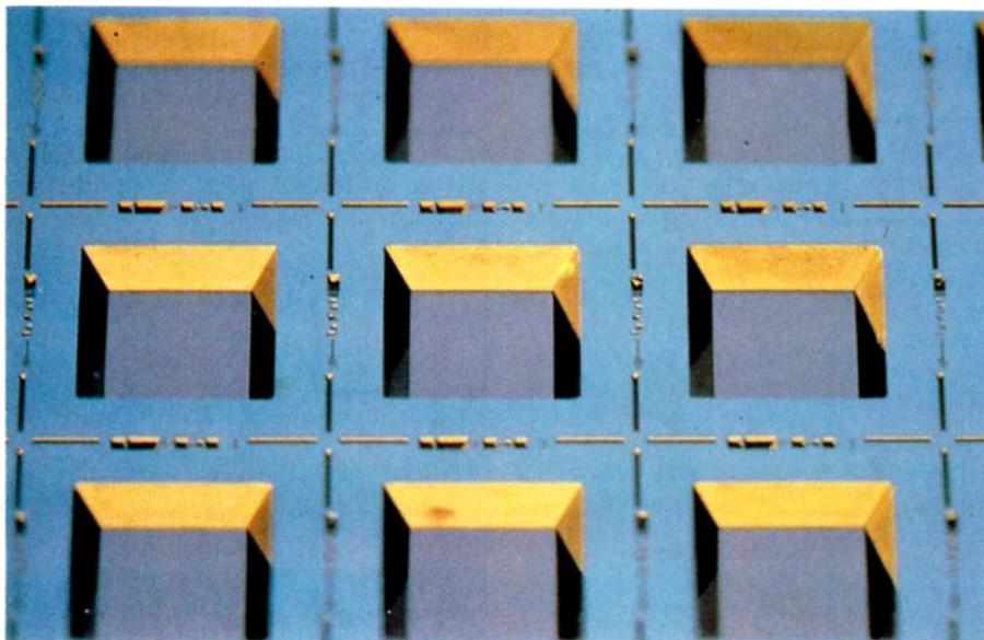
silicon version of this resonant sensor (below) incorporates a resonant structure bonded at both ends to bridge supports formed in the surface of the diaphragm. The diaphragm encloses a reference vacuum maintained on the resonator side of the diaphragm while gas for pressure measurement is applied to the other side.
