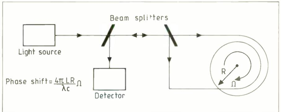
*The basic concept of the fibre optic gyro relies on an effect first described by Sagnac in the 1920's in which a differential phase shift is induced in light that travels clockwise and anti-clockwise around a rotating optical system.*
