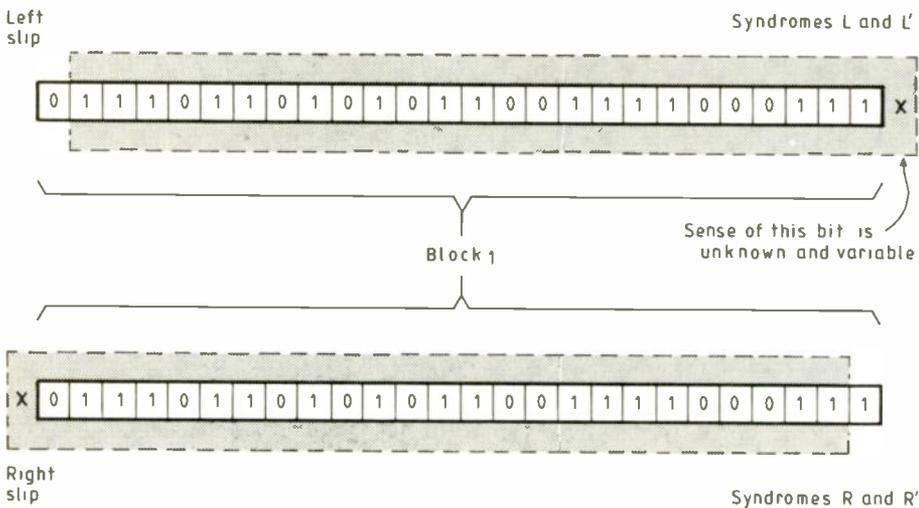
Fig.6. Locking to the RDS bit-stream: block 1 bit-slip syndromes.
