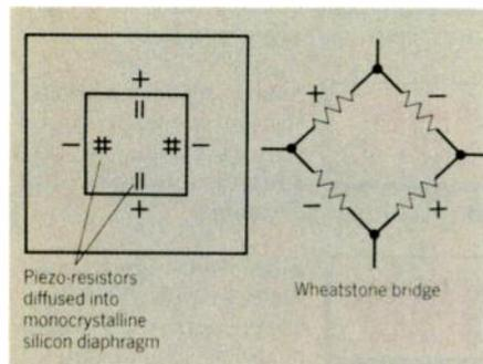
**Conventional semiconductor silicon pressure sensor has four piezo resistive strain gauges diffused into the surface of the pressure diaphragm and connected in a Wheatstone bridge.**
