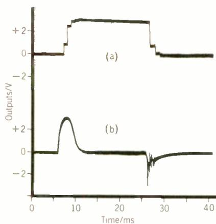
**The conventional current transformer cannot be used for transient measurements because its output is proportional to the rate of change of current with time ( $Ldi/dt$ ), whereas the output of the fibre optic system is linearly related to current, making it suitable for both direct and transient currents.**
