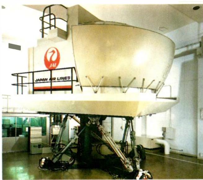
**Simulator by Rediffusion Simulation for JAL, showing the curved, wrap-around screen for the WIDE image display. The jacks impart the motion sensation.**
