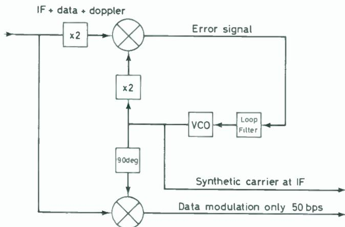
Fig. 3. Traditional GPS receivers require one of these hardware tracking channels per satellite (a). Sections (b) and (c) are a traditional code tracking loop and a hardware carrier tracking loop respectively.
