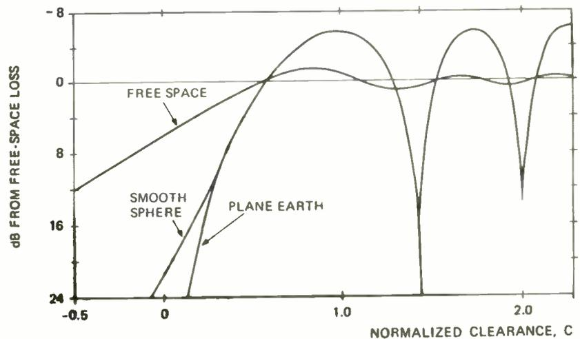
Fig.5. Loss versus normalized clearance.
