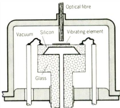
**A bridge structure incorporated into the surface of the silicon diaphragm is made to resonate at its natural frequency with electro-static excitation. Pressure applied to the diaphragm bows and stretches the resonator, causing its frequency to change.**
