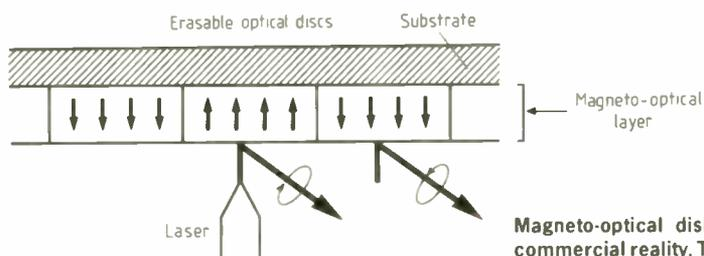
Magneto-optical disks are not yet a commercial reality. The laser heat written magnetic domains in the magnetic layer produce a polarisation twist in the optical layer of just a few degrees.
