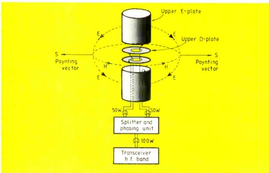
Fig.6. The "barrel-shaped" crossed-field-antenna (CFA).
