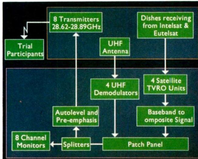
Fig.5. BT M<sup>3</sup>VDS system parameters.
