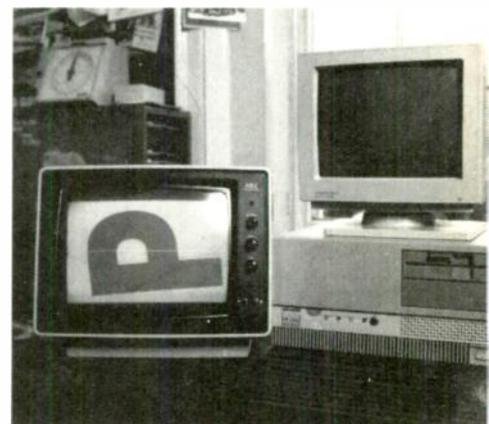
Left is a plot of light intensity against xy axis of image scanned through Fairchild Weston CCD camera and processed by CCUM board. Image on display screen is letter 'P' transfer. Middle picture is computer screen showing 8-bit numbers for each pixel built up against time. It is possible to measure edges to accuracy of 0.1 pixel (one micron). Computer screen in right-hand picture shows analogue information from line-scan camera. Intensity of light across P shown by cursor on computer monitor.
