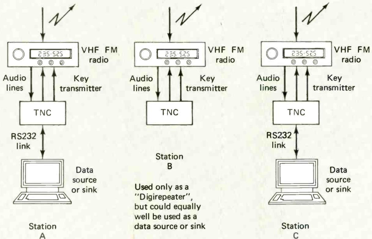
Packet radio on VHF: station B acts as an unattended relay point, making communication possible between A and C.
