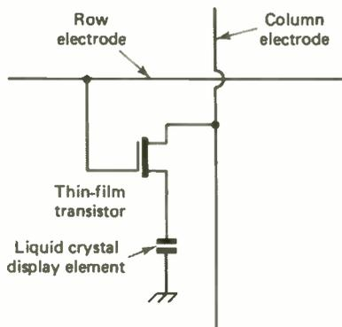
Earlier thin-film transistors used to switch liquid-crystal picture elements in this way were leaky and required an extra capacitor across the liquid-crystal display.
