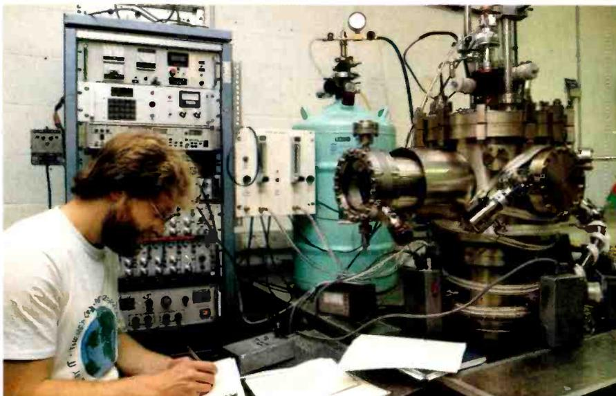
**VG Scientific HB501 scanning transmission electron microscope.** Specimens are mounted within the ultra-high vacuum stainless-steel column to the right of the control console (right). A coherent electron ray, the electrical equivalent of a laser beam, can be focussed onto a spot only half a millionth of a millimetre in diameter.
