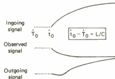
Now that we have dealt with this (previously-induced) signal leaving the oscilloscope, let us deal with the signals entering it when the above relay is operated as above. [The reason for dealing with these outgoing and incoming signals separately is because they overlap (time-wise) hence the trace is composite.]
