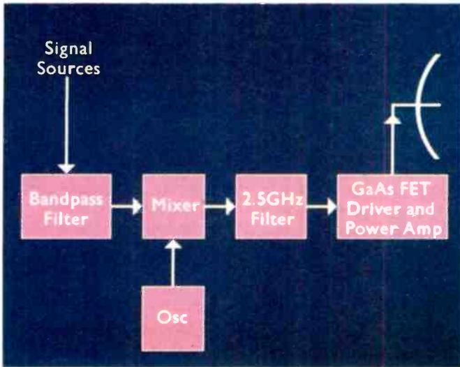
Fig.1. The basic MVDS transmitting system.
