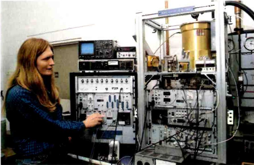
**460-490GHz radio-astronomical receiver** (above) being assembled and tested. When completed it will be installed in the 15m diameter James Clerk Maxwell telescope on top of the 4260m high Mauna Kea, Hawaii.
