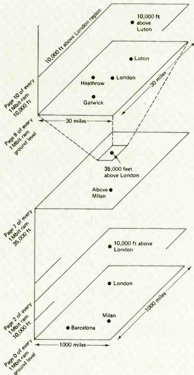
velocity of all aircraft, to be transferred to an identical machine (in the higher pages of the 1 Mbit rams) which will be accelerated into the future by (in effect) increasing clock rate. Potential hazards between a pair of aircraft will then be flagged up because of actual collision between two of the growing (future tense) amoebae in this accelerated machine, one representing each aircraft that is at risk.
