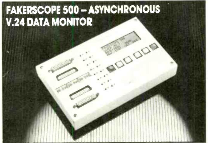
Easily operated by soft keys, with user prompts displayed on an 80 character LCD, the Fakerscope includes an RS 232 breakout box, plus a data monitor and message generator. The message generator can output both canned and pre-programmed data, while output flow control can be Xon/Xoff or level control. Each Fakerscope 500 includes 8kbyte of capture RAM. Data can be reviewed on the LCD or a separate terminal and is displayed in ASC11, HEX or baudot. The Fakerscope 500 costs only £495.00.
