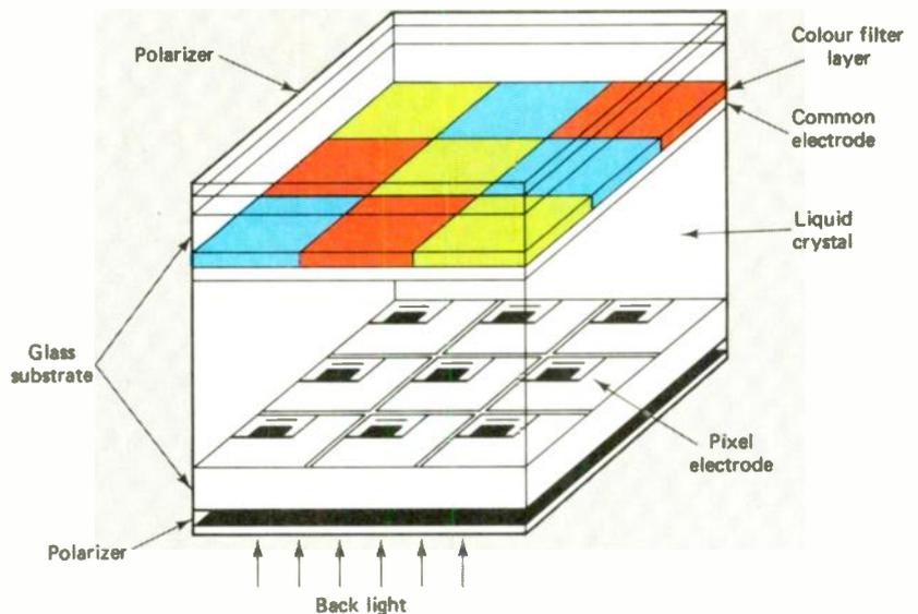
Colour pixels in the prototype display, and probably in the final product, are staggered by one-and-a-half dots to give a better picture. The polarizer absorbs about 50% of light and there are other losses, hence the need for backlighting.
