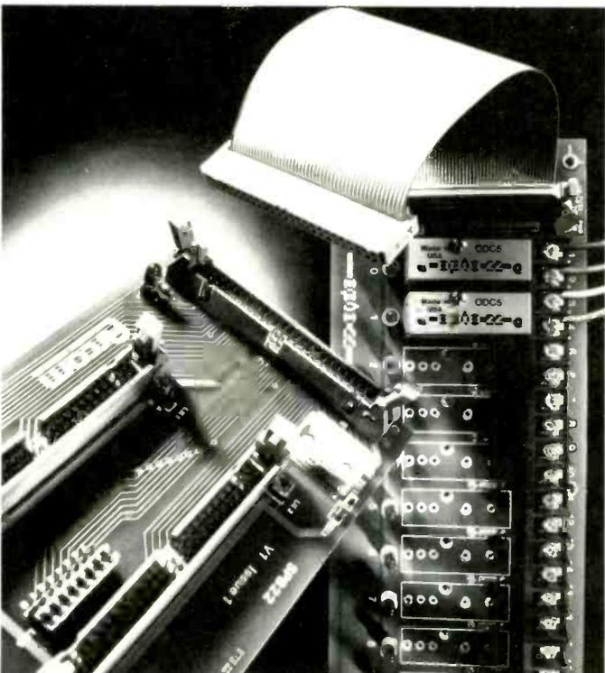
conversion. Data rates up to 64Kbits/s are supported. The asynchronous character lengths can be from 8 to 11 bits including start, stop and parity bits. Micro Call Ltd 084 421 5405
