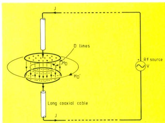
Fig.1. Circular capacitor plates showing the surrounding magnetic fields when applied with a sinusoidal voltage  $V$ .
