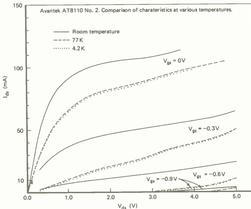
Fig. 6. Characteristics of a AT8110 at room temperature (full line), 77K (dashes) and 4.2K (dots). Note the remarkable agreement between the two sets of low temperature curves which suggests that even when the device is immersed in liquid helium, the effective channel temperature is probably of order 80K or above.
