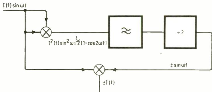
Fig. 6. Carrier regeneration: signal extraction system based on a narrow-band filter.
