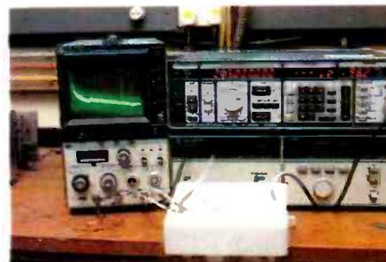
A spectrum analyser displaying the noise spectrum (between 20kHz and 350MHz) of a UHF amplifier constructed using GaAs mesfets. In the first photograph, the amplifier is operating at ambient temperature, while in the second it has been cooled by immersion in liquid nitrogen.
