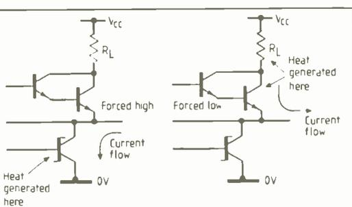
Left: normally low output driven high; right, normally high output driven low.
