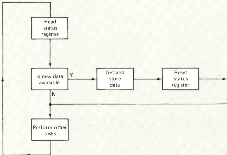
Fig.2. Polling provides an attractively simple method of signalling to the host that data is available.
