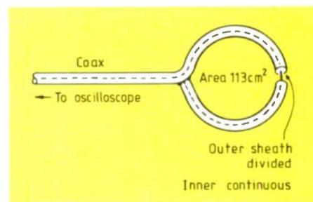
Fig. 4. Balanced Faraday screened loop.
