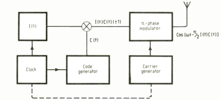
Fig. 2. Transmitter essentials in a typical direct sequence spread system.
