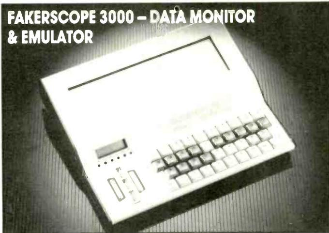
A high contrast, 840 character LCD, permanent user status messages and qwerty keyboard contribute to the user friendliness of the Fakerscope 3000. It includes 10 non-volatile set up files, is fully compatible with asynchronous, synchronous and bit synchronous systems and can monitor at up to 72kbps for synchronous protocols. Each instrument supports SNA and X.25 decoding at levels 2 and 3. The Fakerscope 3000 can be supplied with up to 64kbyte of capture RAM and costs from £1495.00.
