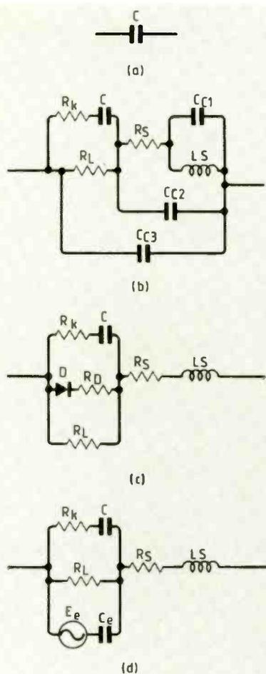
Fig. 1. At (a) is a "pure" capacitance, which is more nearly represented by the equivalent circuit at (b). The diode in (c) represents the unidirectional conductive path in an electrolytic capacitor, while (d) shows a generator and resistor to indicate the stored charge and dielectric hysteresis exhibited by film dielectrics.
