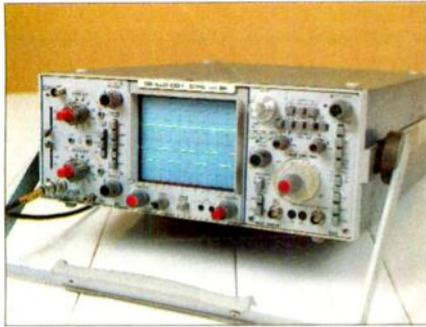
Telequipment D755 Dual Beam 50MHz
