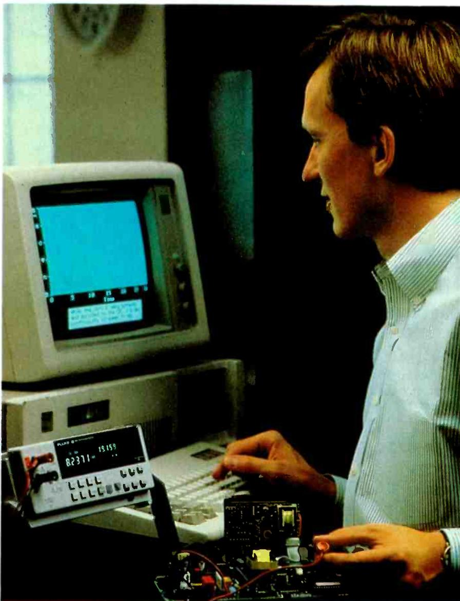
*In the "interact window", the selection of functions and values is made by pull-down menus, and when applicable, editable fields. When the Enter key is pressed, the command and values are sent to the instrument. This type of user interface all but eliminates the need to type in command strings, although they can still be entered at any time on the command line.*
