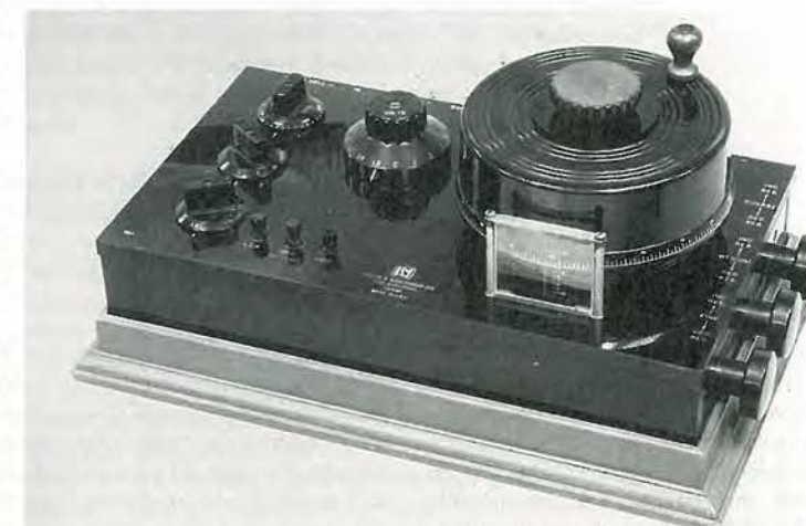
This Leeds and Northrup version of the potentiometer is an adaptation of the Crompton arrangement, one of a series (K1 through K5) sold as recently as the 1980s. This one is a K2, dating about from the 1940s. It has three ranges, with full-scale readings of 1.6V, 0.16V and, believe it or not, 0.016V.
