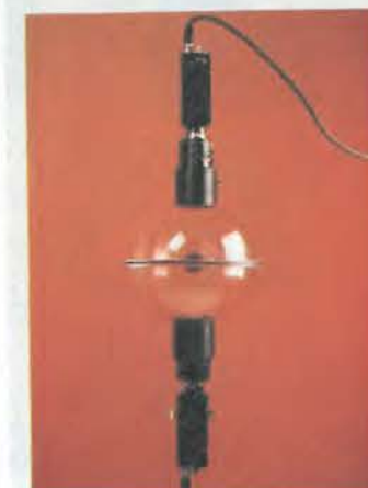
Using a spherical mirror, this camera can see in all directions at once - see page 186.
