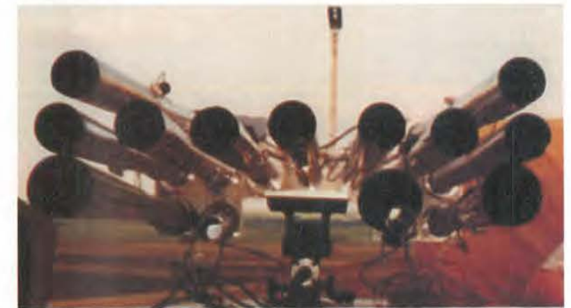
Stanford's Fly's Eye is an array of photomultiplier tubes designed to time-resolve the horizontal development of intense sub-millisecond ionospheric flashes that have come to be known as 'elves'.
