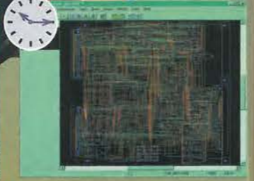
Now the SPECCTRA Autorouter is employed to finish the routing of the design at high speed and with high-grade quality. All design rules are fully respected. (45 min.)
