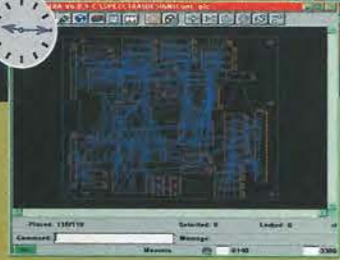
AutoPlace rapidly and conveniently places the remaining components with algorithms that approach the interactive method of expert designers. On-line changes are possible. (5 min.)
