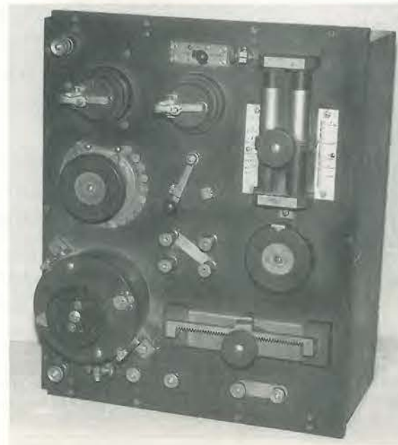
Photo 1. This Marconi Company receiver from circa 1915 was designed for reception between 250 to 1300m. It represented a standard in coastal and marine communications.
