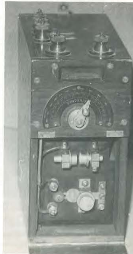
Photo 3. Transmitter for aeroplane wireless station from circa 1915 – one of the first transmitters designed specifically for aviation.
