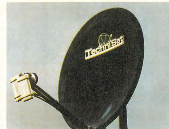
Fig. 1. One of the earliest dual-lnb satellite installations in the UK, as installed in December 1990. Both the original Marconi 1.3dB noise lnb's continue in daily use.
