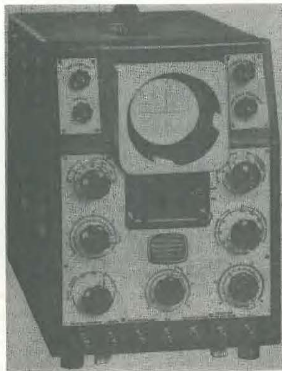
Fig. 4. An advanced oscilloscope of the forties. The Cossor 1035 Mk IIA was a true dual-beam oscilloscope with a maximum bandwidth of 7MHz (Y1 amplifier), 100kHz (Y2 amplifier) and a fastest sweep rate of 15us/scan, with repetitive, triggered and single-stroke operation.
