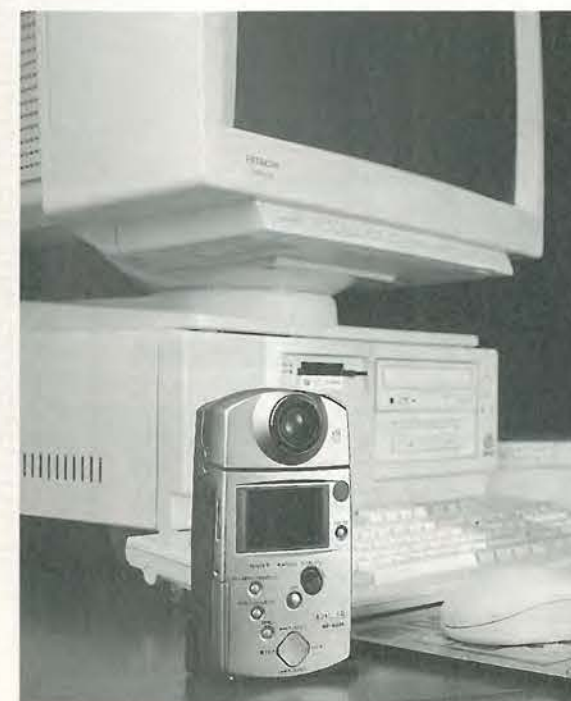
Incorporating a single chip carrying the 300 000 components necessary to handle all camera functions – including real-time MPEG-1 coding/decoding – Hitachi's disk camera has a 260MB disk expected to give 20 minutes of MPEG-1 video and audio recording.
