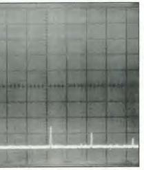
Fig. 6. Spectrum of the 10V peak to peak output of the circuit of Fig. 5. Spectrum analyser settings as for Fig. 4, but with video filter set to 'medium'.
