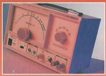
AG2601 is a portable mains-powered instrument covering 10Hz to 1MHz in five overlapping decades. Sinewave distortion between 500Hz and 50kHz is just
