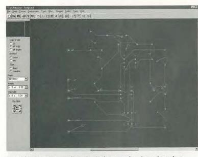
Fig. 4. Ultimate Rat's nest of test circuit after manual sorting and transfer to Windows. Note the force vectors which can aid component placement.
