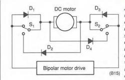
A reliable (and cheap) method of stopping a dc servo motor very quickly without recourse to electronic sensing
