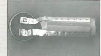
Fig. 11. Photograph of a dismantled and partially unwound capacitor shows a good example of the stitched technique used to connect both anode and cathode foils to their respective tab foils central tabbed in this example. Also the cold pressure welded joints connecting anode and cathode tabs to the external tag rivets are clearly visible. This excellent joint results from the tool pattern which, by compressing and displacing metal, removes the oxide layers allowing direct metal to metal bonds.
