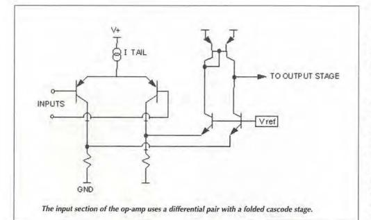
Both op-amps and comparators have been announced, in single, dual and quad form. Part numbers are LMV321, 358, 324 for op-amps and LMV331, 393 and 339 for comparators. These devices are drop in replacements for their LM ancestors. "Very often when we introduce a new product, designers have to relearn how to use it - not with the LMV," said Claustres.
