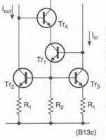
Fig. 3. Practical circuit of the wider bandwidth current mirror with uncompromis ed accuracy.
