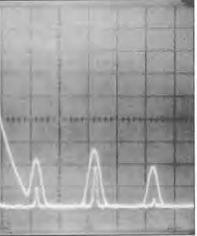
Fig. 2. Upper trace, output of the circuit of Fig. 1. Span 0-5kHz, 100Hz resolution (IF) bandwidth, video (post detection) filter off. Lower trace, as above, but with component values in brackets, resolution bandwidth 30Hz.
