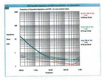
Fig. 9. As for Fig. 8 but this time using 47µF values. Due to the larger size and foil area, the Panasonic bi-polar style easily outperforms the smaller alternatives.
