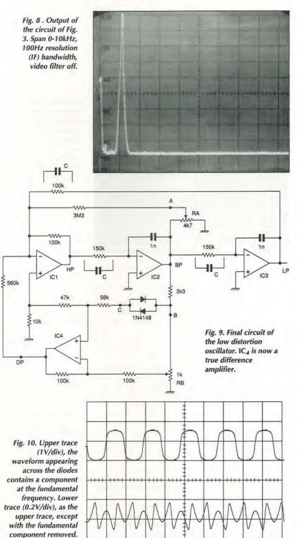
Resistor  $R_{\rm B}$  in Fig. 9 allows this to be adjusted to equal the amplitude of the fundamental component of the negative feedback signal shown in the lower trace of Fig. 11. The result is that the output of the difference amplifier  $IC_4$  then contains the harmonic components only, as shown in Fig. 10, lower trace.
