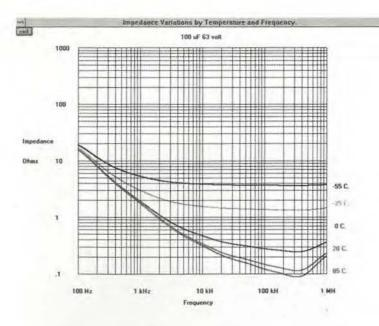
Fig. 13. Plot showing how impedance versus frequency characteristics change with ambient temperature, for a typical 100µF 63V capacitor.
