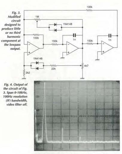
filter - was larger than at the output of the second integrator - the low-pass output. Its feedback resistor was therefore raised by  $4.7k\Omega$ , the integrators between them now providing a gain of 4.7% less than unity.
