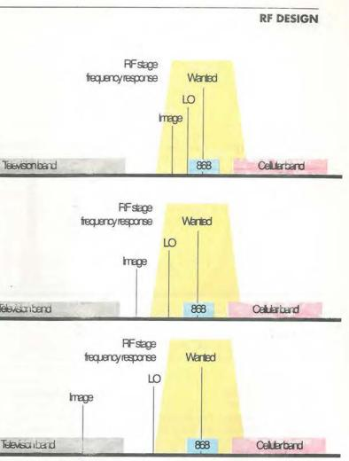
Impact of intermediate frequency and front-end filtering choices.
