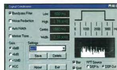
The DSP applet provided with the WR3000 spectrum monitor ISA card (£995+VAT) allows continuous control of audio bandwidth and other signal conditioning functions
