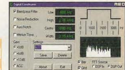
The DSP applet provided with the WR3000 spectrum monitor ISA card (£995+VAT) allows continuous control of audio bandwidth and other signal conditioning functions
