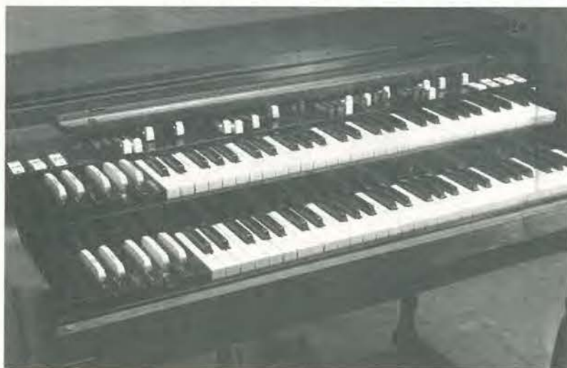
Fig. 5. Developed before solid-state electronics, Hammond's B3 organ has no oscillators. It uses electromechanics instead.
