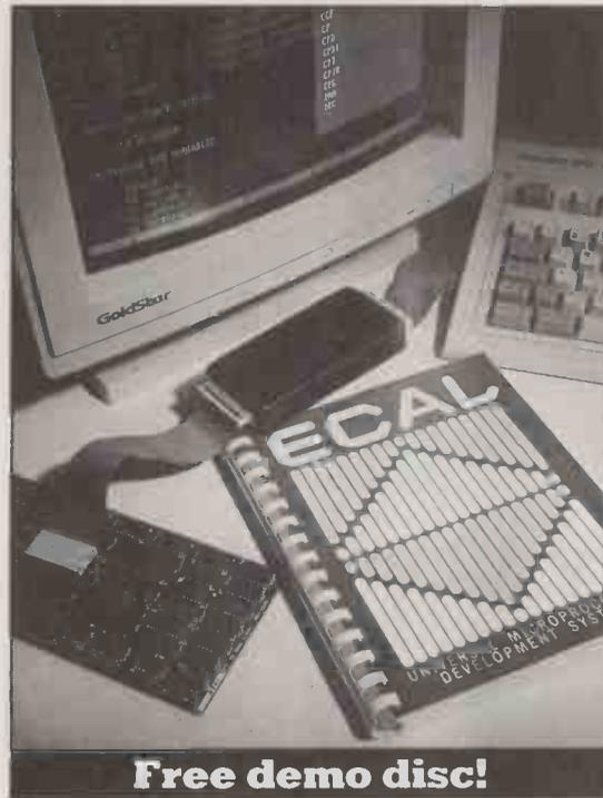
The PC based ECAL hardware emulator is fully integrated with the assembler. Connection is made to the target through the eprom socket so a **single** pod can support **all** processors. Facilities include windows for the inspection or change of registers or memory. You can even watch your program executing at source level!
