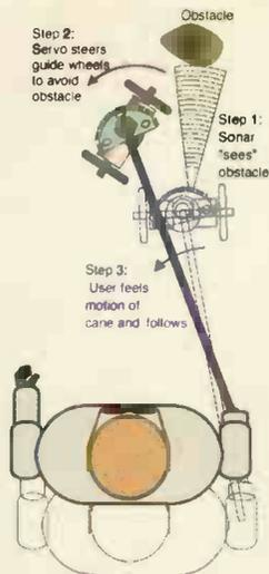
The 3.5kg *GuideCane* consists of a long handle with a thumb-operated joystick for direction control, an array of ultrasonic sensors and a small on-board computer mounted on a two-wheeled steering axle. Users push it ahead with one hand. When the device's ultrasonic sensors detect an obstacle in its path, the computer automatically turns the wheels to steer around the obstacle and resume the original direction of travel.
