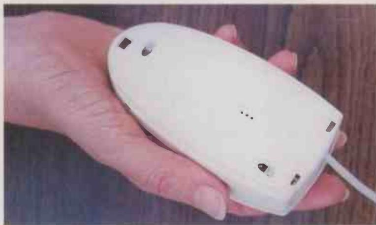
*Look underneath and you will see no rubber ball. The two fibre optic sensor points can be seen at the bottom and top.*
