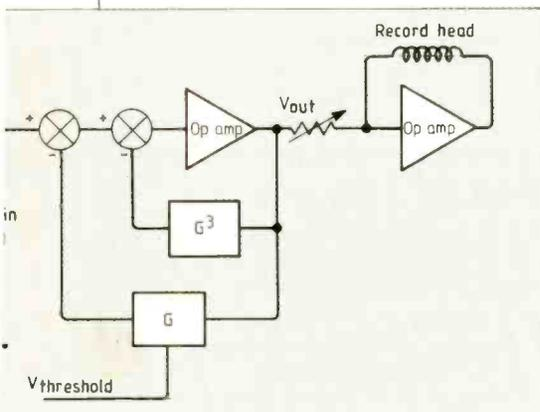
linear relationship, using a diode-pair function generator ( $G^3$ ) whose conductance increases as the cube of the input voltage. Output is the cube root of the input.
