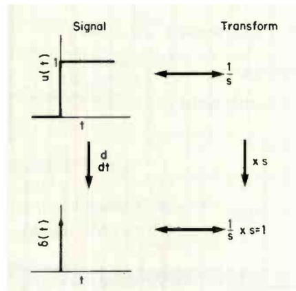
**Fig. 4.10. Laplace transform of the unit impulse.**
