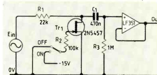
Fig. 10. Shunt connected fet switch, which exhibits higher on resistance and provides less attenuation. Distortion occurs at lower input levels.
