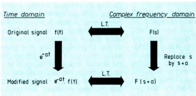
Fig. 4.3. Frequency shifting rule.
