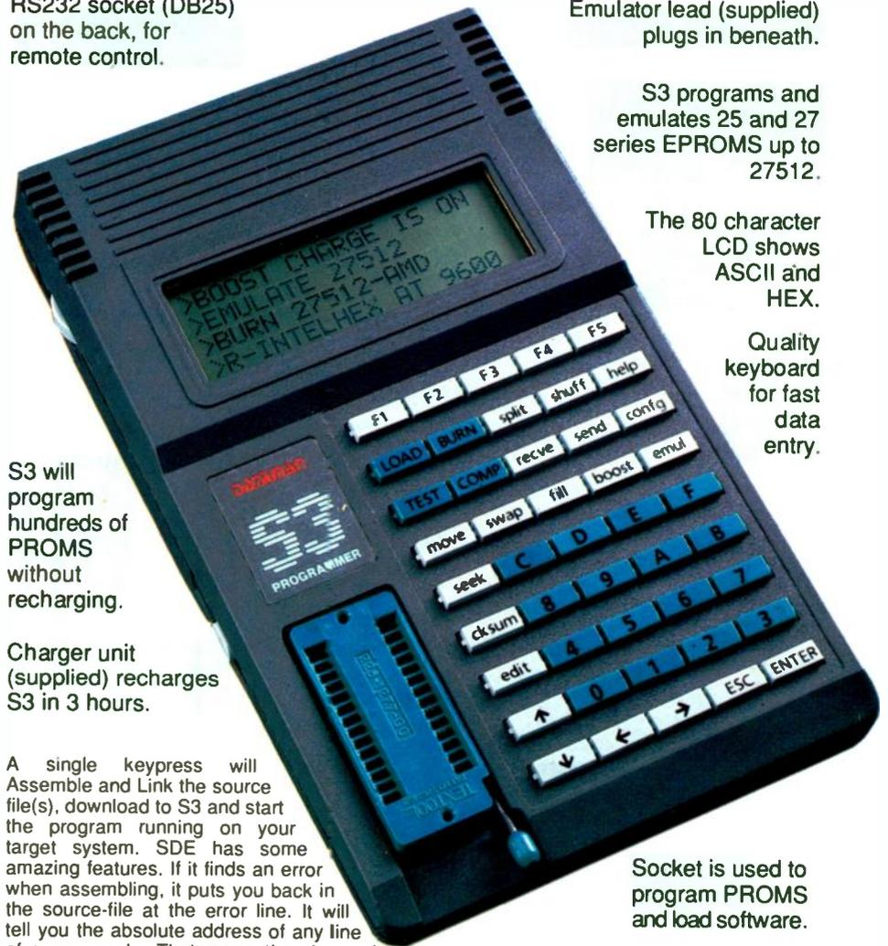
Socket is used to program PROMS and load software.
