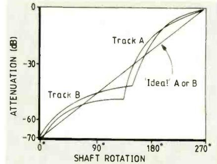
Fig. 3. Ideal logarithmic gain-control response and that given by ganged controls in a stereo system, which may not be well matched.
