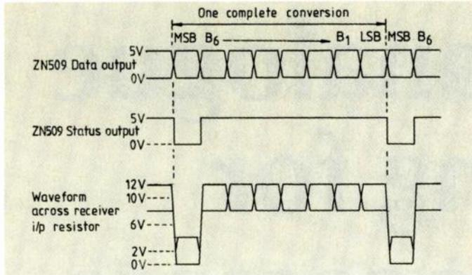
Fig. 3. Receiver input waveforms. Clock period is 196µs.
