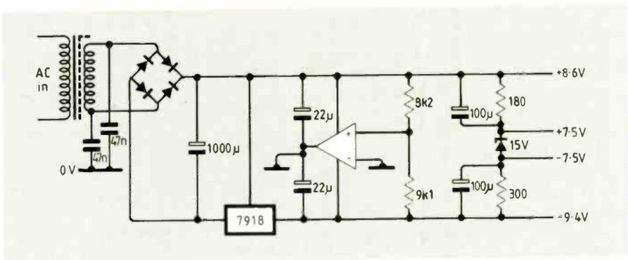
Fig 14. Stabilised power supply for Quad preamplifier.
