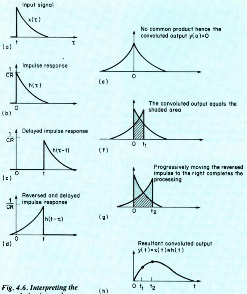
**Fig. 4.6. Interpreting the convolution integral graphically.**
