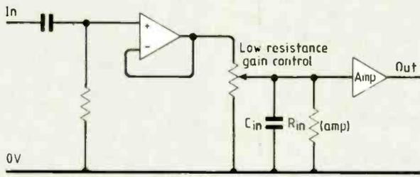
Fig. 2. Buffer stage eliminates effect of variable impedance and allows use of low-value control.
