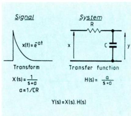
Fig. 4.2. Signal and system are matched in the sense that the system impulse response is identical to the characteristics of the signal.
