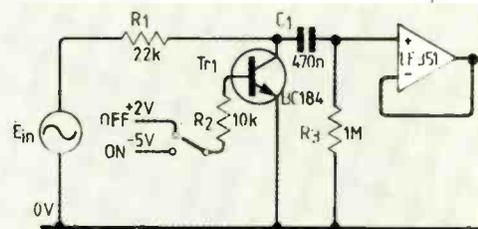
Fig. 9. Small-signal bipolar transistor switch, shunt connected, for low-impedance sources, which can offer THD of less than 0.005%.
