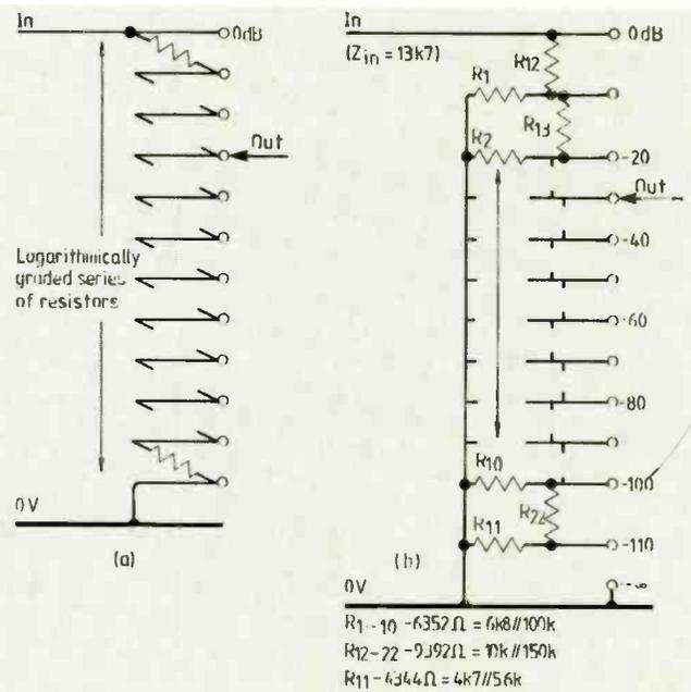
Fig. 6. Log-law switched gain control used by Quad (a), in which graded resistors are switched by c-mos elements. At (b) is alternative type by author which uses non-graded resistor values.
