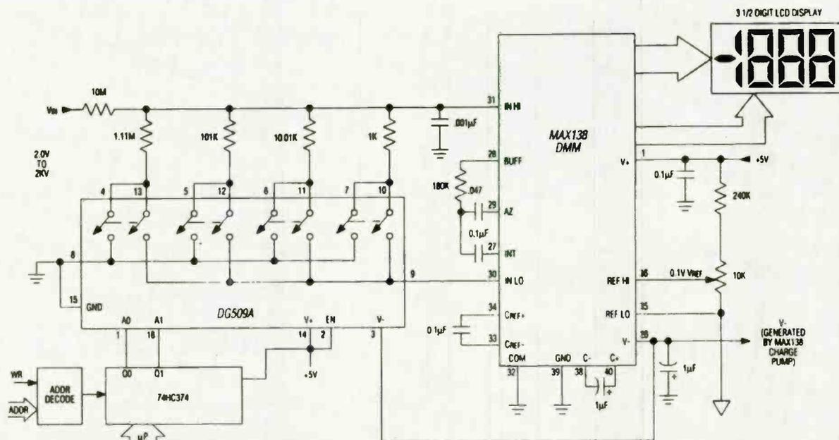
Although many low-cost digital panel meter chips now exist, they are commonly designed for a single range and have no provision for different voltage ranges. When input switching is needed, one solution is to use solid-state devices in a divider arrangement, but this does mean that the switch resistance has to be taken into account when designing the divider. Since the resistance is not accurately known and varies with temperature and power supply voltage, the method is not ideal.
