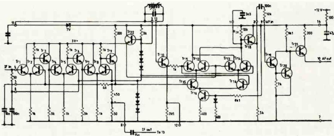
Fig.9. MC1351 FM IF strip and demodulator.
