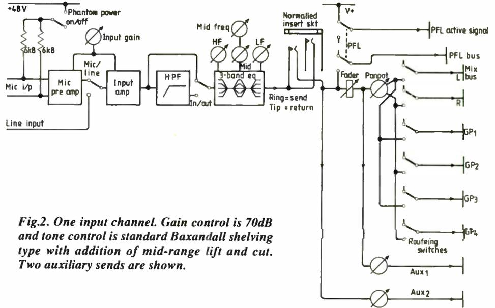
**Fig.2. One input channel. Gain control is 70dB and tone control is standard Baxandall shelving type with addition of mid-range lift and cut. Two auxiliary sends are shown.**
