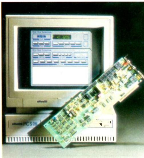
a full-sized 8-bit bus PC expansion card, which employs a mixture of surface-mounted and standard technology. The card is fitted with two standard 4mm banana sockets (for signal input) on the industry-standard 0.75in pitch, together with a male 9-way D-type connector for control of an optional external scanner. Board layout is uncluttered and, in many cases, users will not need to change the settings of the configuration jumpers fitted.
