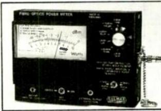
dBm and  $\mu W$  scale; battery life 500 hours.
