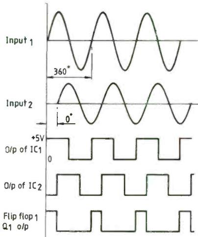
0-199.9. For the range set by resistors R<sub>1,2</sub>, measurement resolution is 1° over 0-360°. Measurement accuracy is better than 0.2% over 1kHz to 250kHz, falling off at lower frequencies.
