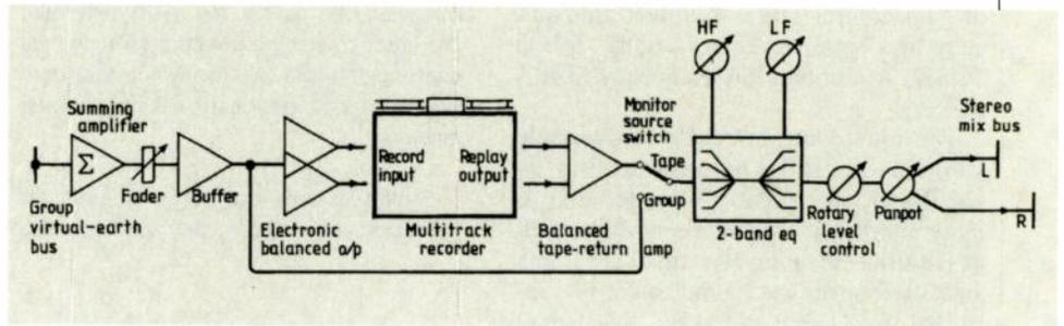
**Fig.3. Block diagram of typical group module, showing switching between direct output and tape replay for monitoring purposes.**
