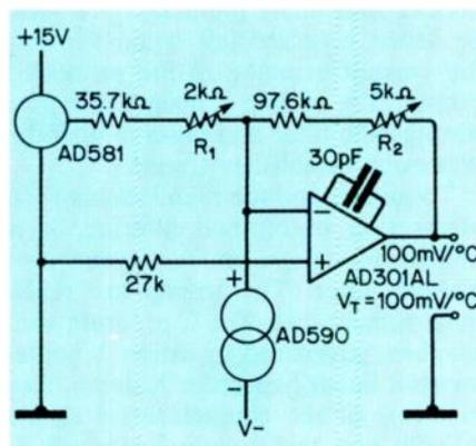
Fig. 8.6. Measurement of temperature using the AD590.
