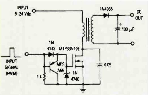
Fig.1. Common mosfet drive arrangement.
