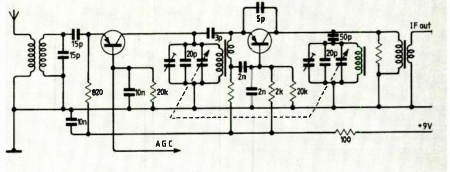
Fig.5. Low-cost tuner-head design of 1967, using self-oscillating mixer.
