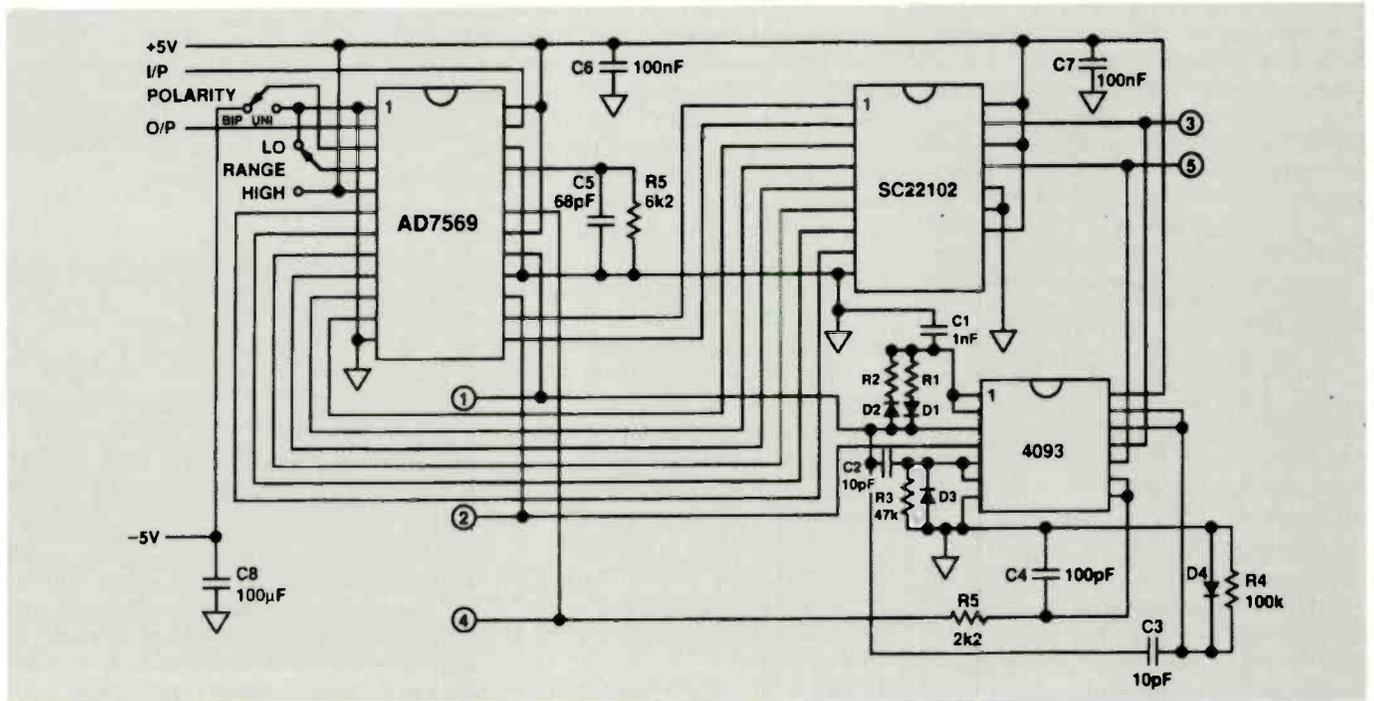
Fig.1. Three-chip function generator.
