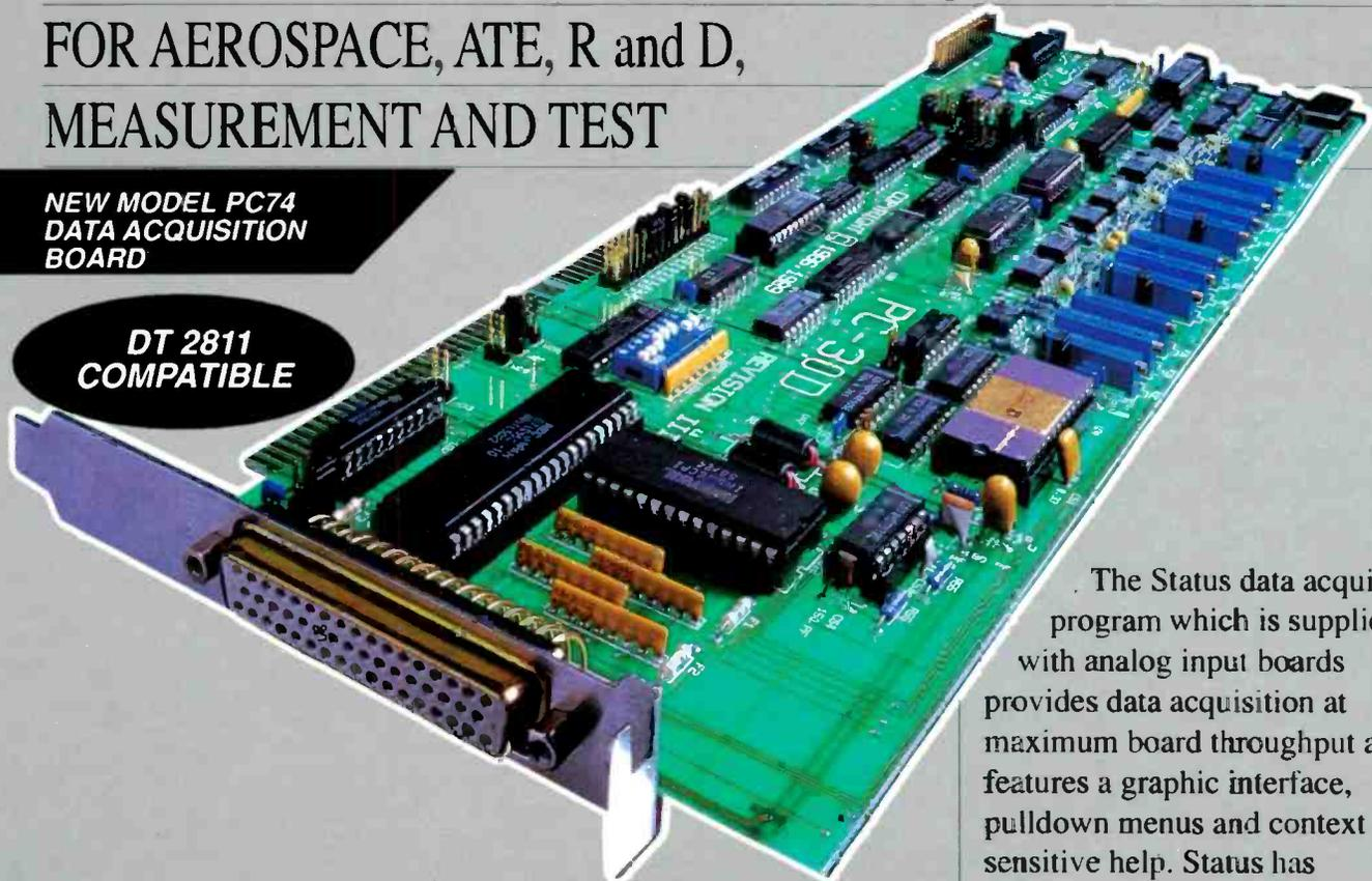
We market high performance multifunction data acquisition boards for laboratory test, measurement and control applications. The multi-channel analog input may be used for signal analysis, data logging, sensor and transducer interfacing and voltage measurement.
