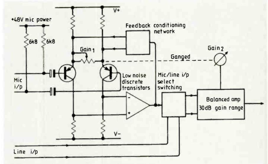
Fig.5. Low-noise microphone amplifier with wide gain range and balanced line output. Transistors in first stage avoid noise problem of op-amps.
