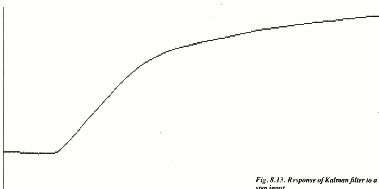
*Fig. 8.13. Response of Kalman filter to a step input.*
