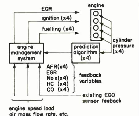
Fig. 4. Ricardo engine management system based DSP using the results of
