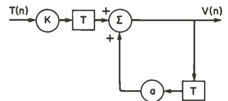
Fig. 8.15. Characteristics of the filter modelled as recursive digital filter.
