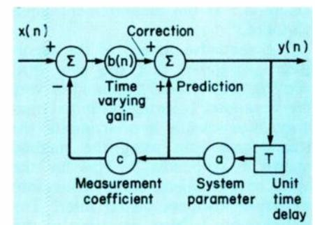
Fig. 8.9. System block diagram of the Kalman filter representing the recursive relationship  $\hat{y}(n) = a\hat{y}(n-1) + b(n)x(n) - ac\hat{y}(n-1)$ .
