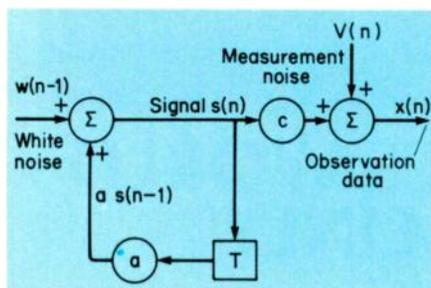
Fig. 8.17. Models of signal and observation process (a) and optimum recursive estimator — Kalman filter (b).
