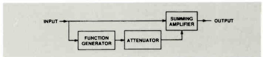
signal is 2% and the correction applied to the signal from the function generator's A-to-D is 2%, then the resolution to which correction is applied is the 0.4% of the function generator multiplied by 2%,
