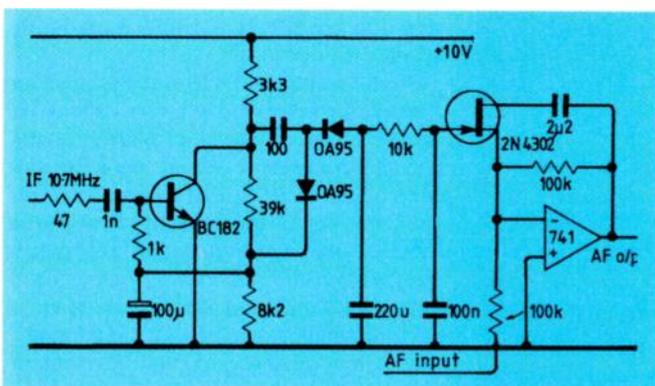
Fig.2. Automatic noise muting circuit operated by IF output signal strength.
