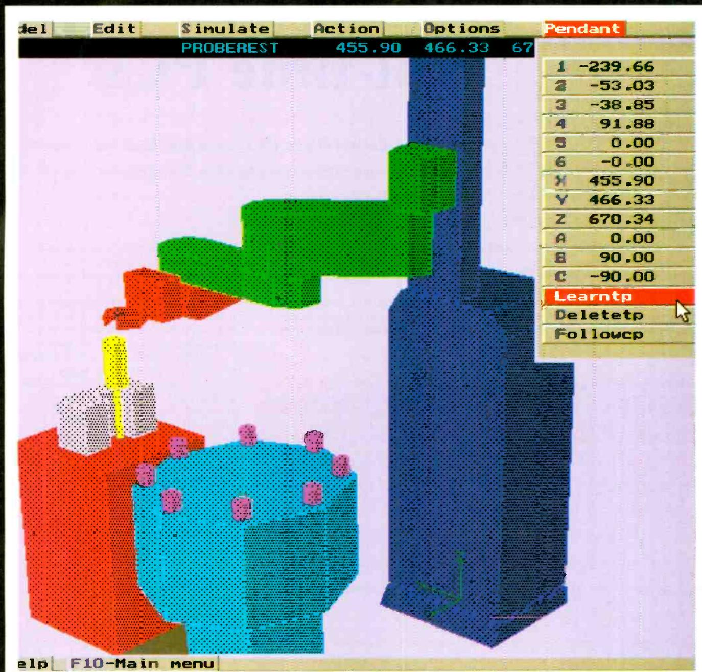
Simulation is an indispensable tool for planning all manner of systems, and Robotics is no exception. Workspace from Robot Simulations of Newcastle runs on a PC and allowing engineers to evaluate different robots, experiment with designs of factory workcells or calculate cycle times.
