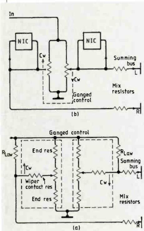
Fig.7. Standard panpot circuit at (a) showing how pull-up resistor draws current through wiper contact resistance, which is usually greater than the end resistance of the pot., limiting maximum attenuation. Arrangement at (b) uses NICs to replace pull-up to modulate law with panpot setting. Left/right isolation increased from -65dB to -90dB.
