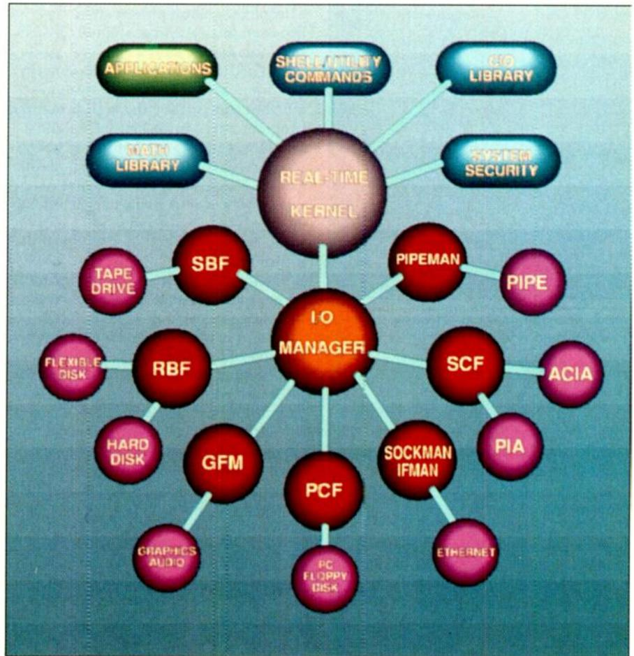
Fig.1. Modular architecture of the OS-9000 operating system
