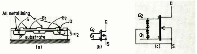
Fig.6. Structure and circuit symbol of dual-gate depletion-type mosfet.
