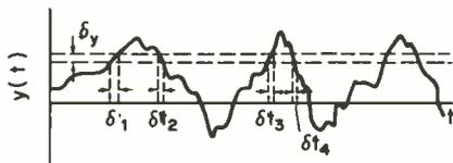
Fig. 8.1. Quantifying random signals using the probability density function.
