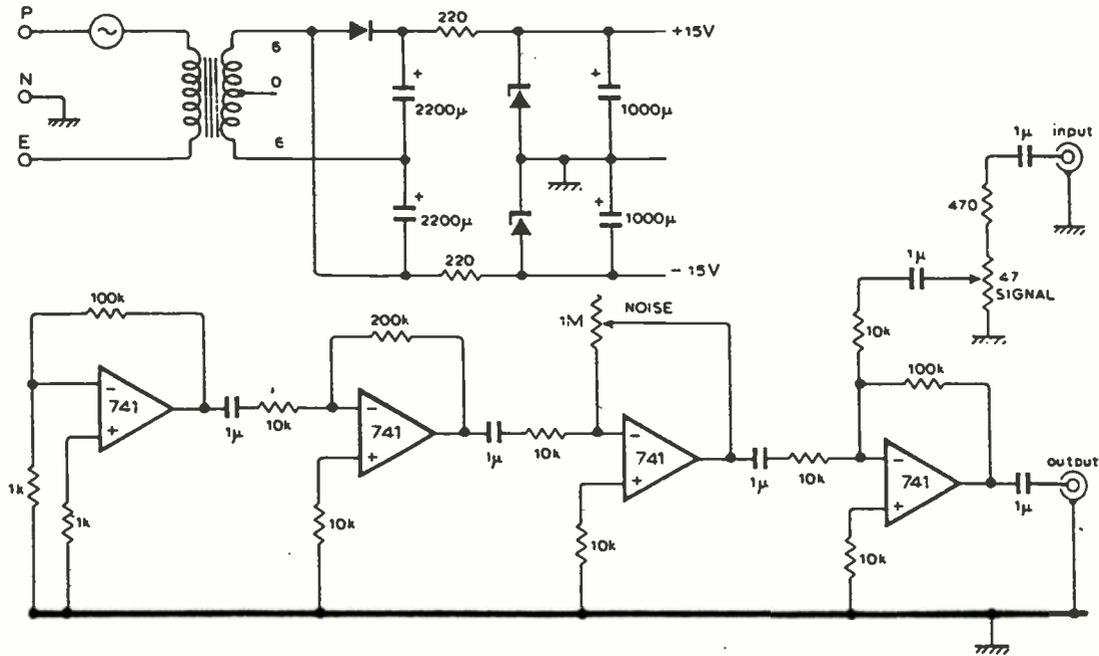
50-5000 Hz WHITE NOISE—Both signal and noise levels are continuously and independently variable from zero to maximum in simple noise generator developed to demonstrate re-
