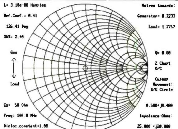
Z-MATCH II takes the drudgery out of RF matching problems and includes many more features than the standard Smith Chart. Provides solutions to matching problems using transmission line transformers, stubs, discrete components etc.etc.. Supplied with comprehensive user instructions including many worked examples
