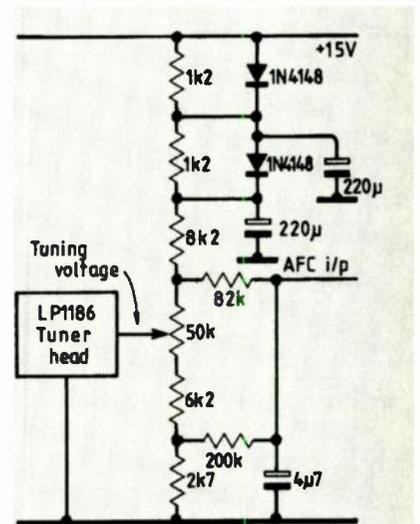
Fig.7. Skingley and Thompson Varicap-diode thermal compensation.
