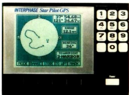
*Navico's Star Pilot GPS costs £2395 and has a 128 X 160 pixel display, which is responsible for the elevated price. Vessel's track is displayed.*
