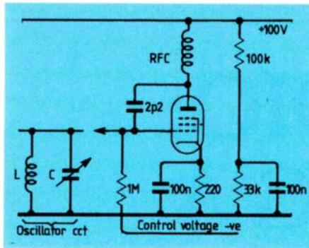
Fig.1. Vari-mu pentode used as Miller-capacitance stage for AFC purposes.
