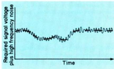
Fig. 8.5. Elementary first-order low-pass digital filter removes HF noise, allowing output to follow slowly changing input signal.
