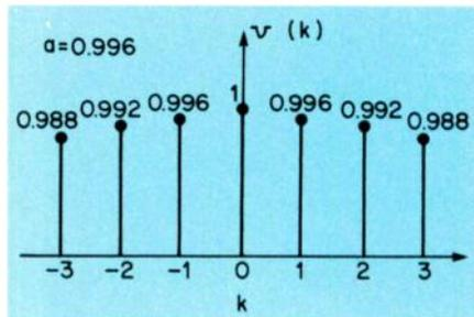
Fig. 8.16. Effect of digital filter on a random input may be determined by autocorrelating the processed output. Notice mean-square value is given by  $r_{vv}(0)$ .
