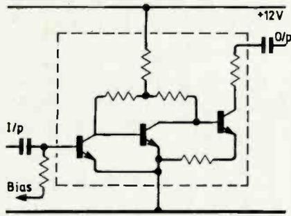
Fig.8. Motorola MFC4010 IC RF gain block.
