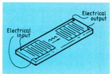
Fig.3. Basic construction of surface acoustic wave filter.
