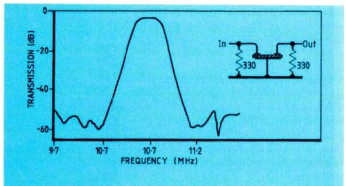
Fig.4. Transmission characteristic of FM IF ceramic filter.
