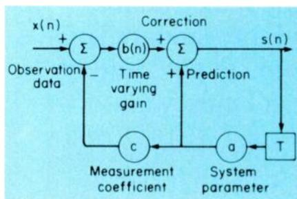
Assume the linear observation model  $x(n) = cs(n) + v(n)$  and the dynamic signal model  $s(n) = as(n-1) + w(n-1)$ . Then substitute and express the mean-squared error as:
