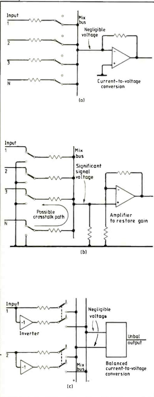
**Fig.8.** Virtual-earth summer at (a) effectively eliminates cross-talk, since there is almost no signal at the summing point. Voltage-mode circuit at (b) allows cross-talk. Balanced virtual-earth summing circuit at (c) requires a separate inverter for each channel to provide the anti-phase signal.
