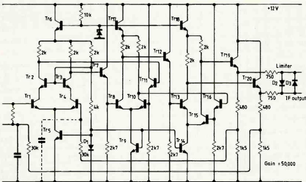
Fig.10. Limiting IF amplifier gain block used in RCA CA3089E.
