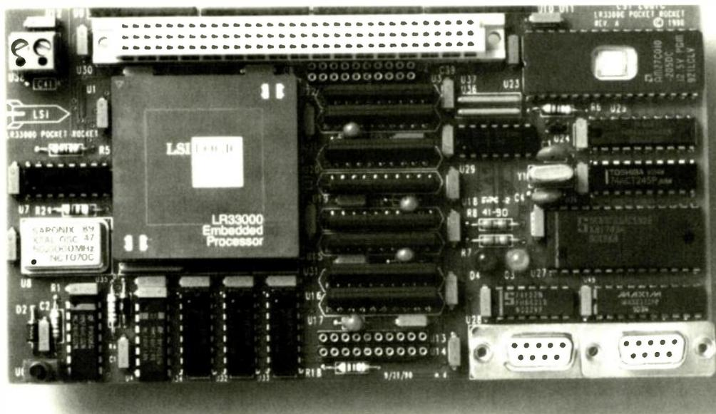
**Pocket Rocket from LSI Logic, an evaluation board for the LR33000**
