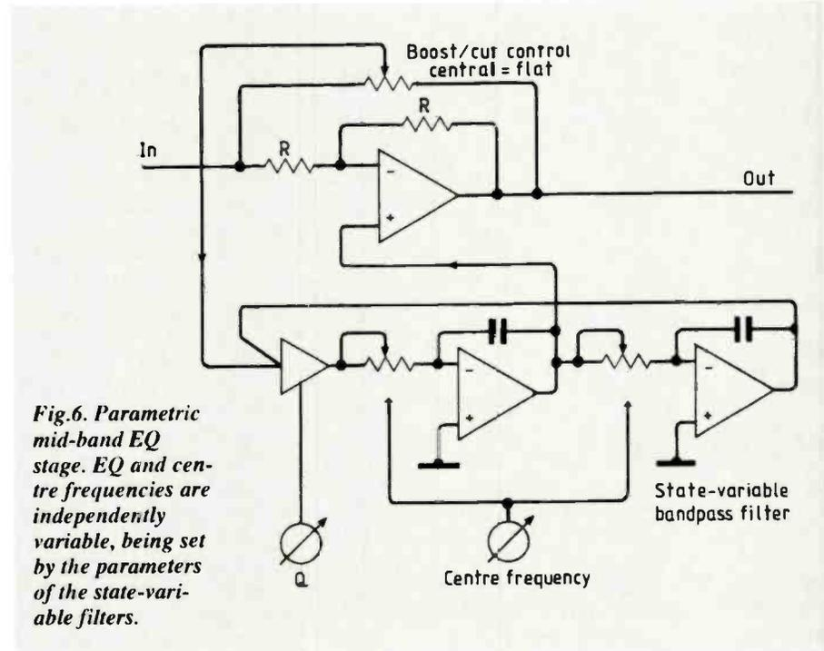
Fig.6. Parametric mid-band EQ stage. EQ and centre frequencies are independently variable, being set by the parameters of the state-variable filters.
