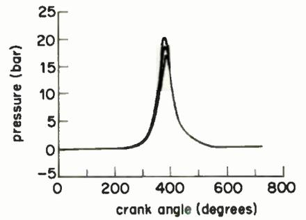
Fig. 1. Measurement of cylinder pressure during combustion cycle for a typical
