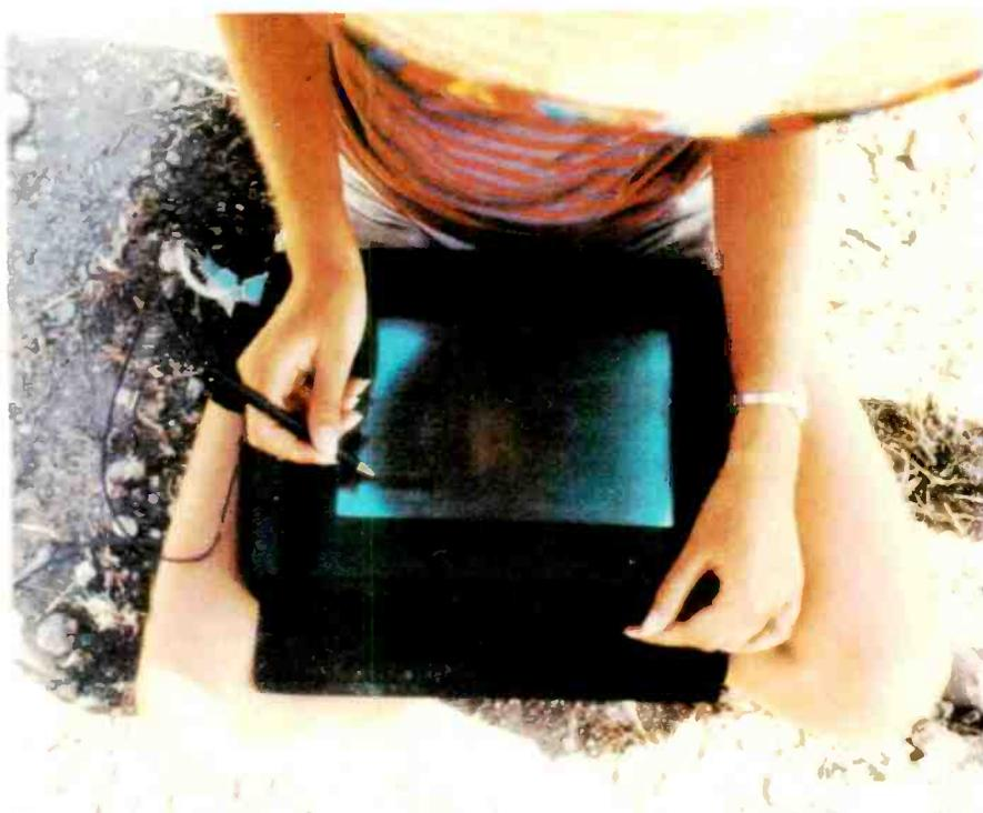
*Raw data is entered by means of a stylus and is then digitised as the work proceeds. GRiDPad then plots a map of the dig on screen.*
