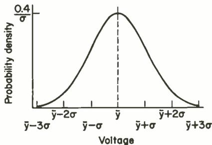
Fig. 8.2. Theoretical Gaussian curve for random signals normalised in terms of mean and standard deviation.
