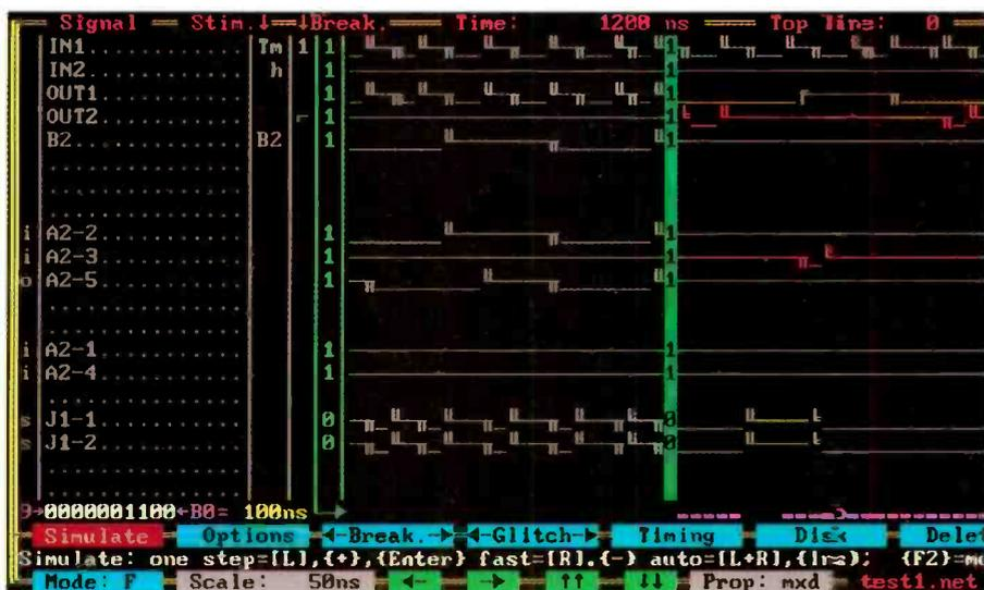
Susie PC-based logic simulation program simplifies digital design.
