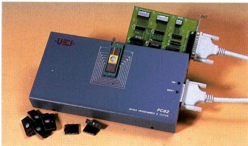
**UNIVERSAL PROGRAMMER.** The complete designer's kit. This will program EPROMS, FLASH EPROMS, EEPROMS, BPPROMS, PALS, GALs, EPLD's, and large range of microcontrollers. A unique feature is the testing of any TTL/CMOS logic chip, DRAM & SRAM.
