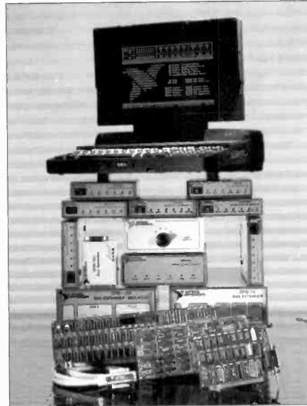
Simple solutions for the integration of IEEE-488, SCSI, RS-232, RS-422, and Centronics parallel devices
