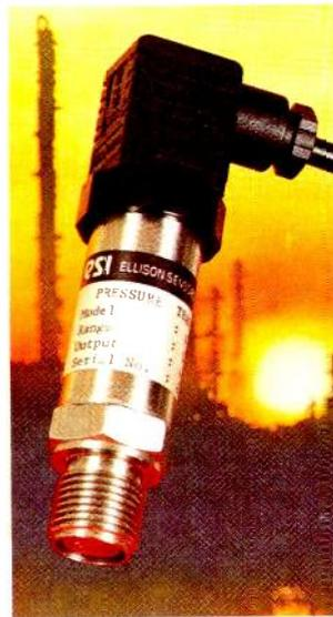
**Pressure transmitter.** A British-designed and manufactured pressure transmitter from Ellison, the *PR3100* is said to be so versatile that it meets virtually all requirements in industry and science, also meeting European standards. It is a strain-gauge instrument with a two-wire 4-20mA output and is built in stainless steel with temperature compensation from -20°C to 80°C. Pressure range is from 250mbar to 1000mbar. Ellison Sensors International, 0978 846434.
