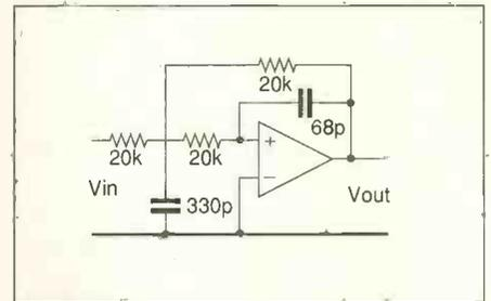
Fig. 8. 2nd order low pass antialiasing filter ( $F_{3\text{dB}}=5\text{kHz}$ ) that can be built with the *Max293* uncommitted op amp
