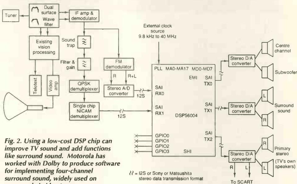
**Fig. 2. Using a low-cost DSP chip can improve TV sound and add functions like surround sound. Motorola has worked with Dolby to produce software for implementing four-channel surround sound, widely used on prerecorded video tapes.**
