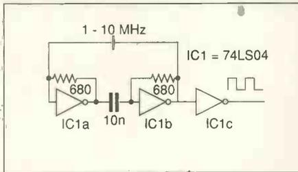
Fig. 5. Simple crystal oscillator consisting of two inverters connected in a ring via a capacitor and a crystal.
