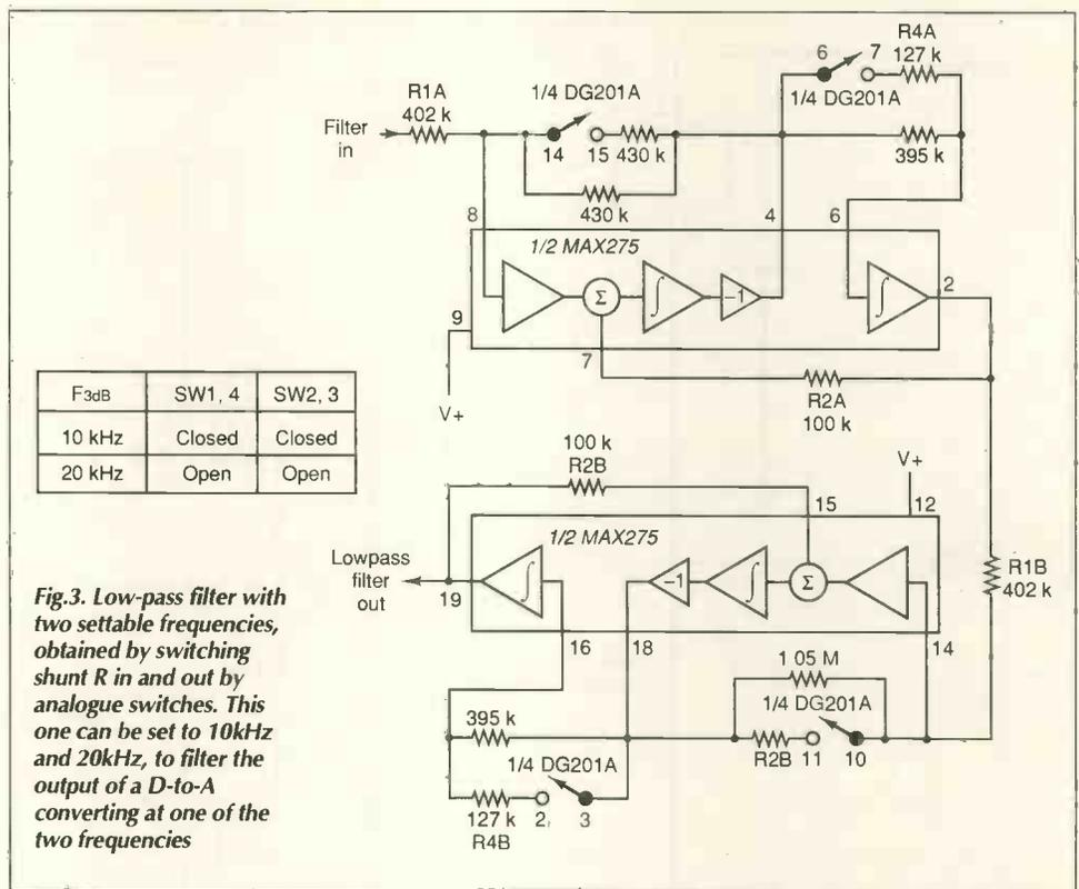
Fig. 3. Low-pass filter with two settable frequencies, obtained by switching shunt R in and out by analogue switches. This one can be set to  $10\text{kHz}$  and  $20\text{kHz}$ , to filter the output of a D-to-A converting at one of the two frequencies
