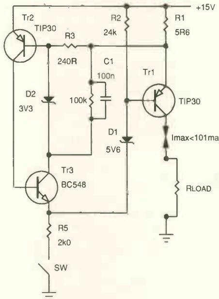
*Overcurrent protection circuit prevents power-supply damage caused by switch-on surges and acts as a circuit breaker in the presence of a short-circuit.*
