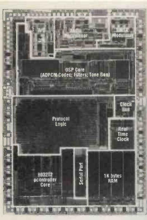
Chip layout of AMD's Am 79C410 telephone circuit
