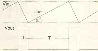
**Fig. 1. Positive feedback from the comparator output to initiate flyback reduces jitter in this voltage-to-period converter.**
