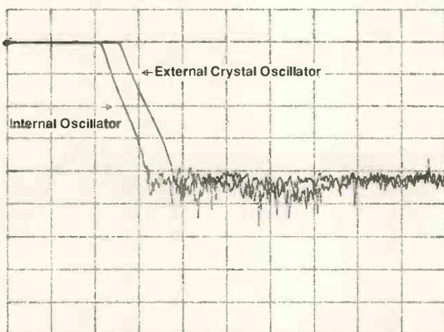
Fig. 3. 5kHz SC filter amplitude response with the internal and an external oscillator.
