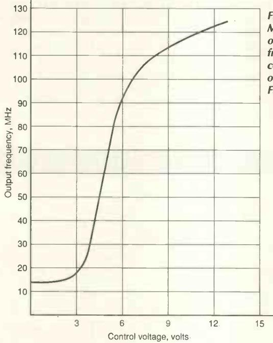
Fig. 6. Measured output frequency vs control voltage of circuit in Fig. 5.
