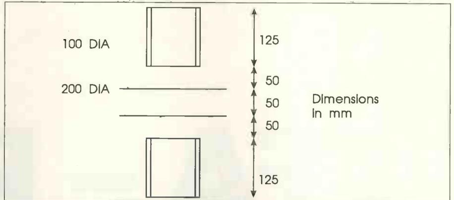
Test CFA. The steel conductors were supported with insulating Perspex parts. The dimensions represent a 50% scaling on the author's original figures..
