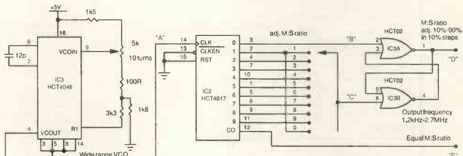
Three ICs form a 1.2kHz-2.7MHz pulse and square-wave generator having a mark-to-space ratio adjustable in 10% steps from 10% to 90%.
