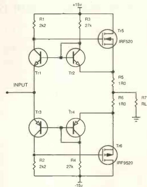
**Current mirrors in this power output stage, which sources and sinks current, allow accurate setting of standing current.**
