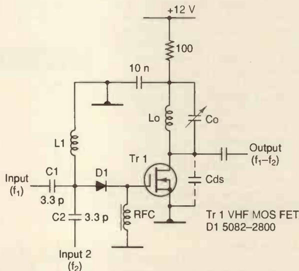
Fig. 17. Diode mixer for up to 2GHz input. Tuned amplifier reduces input-to-output signal feedthrough.
