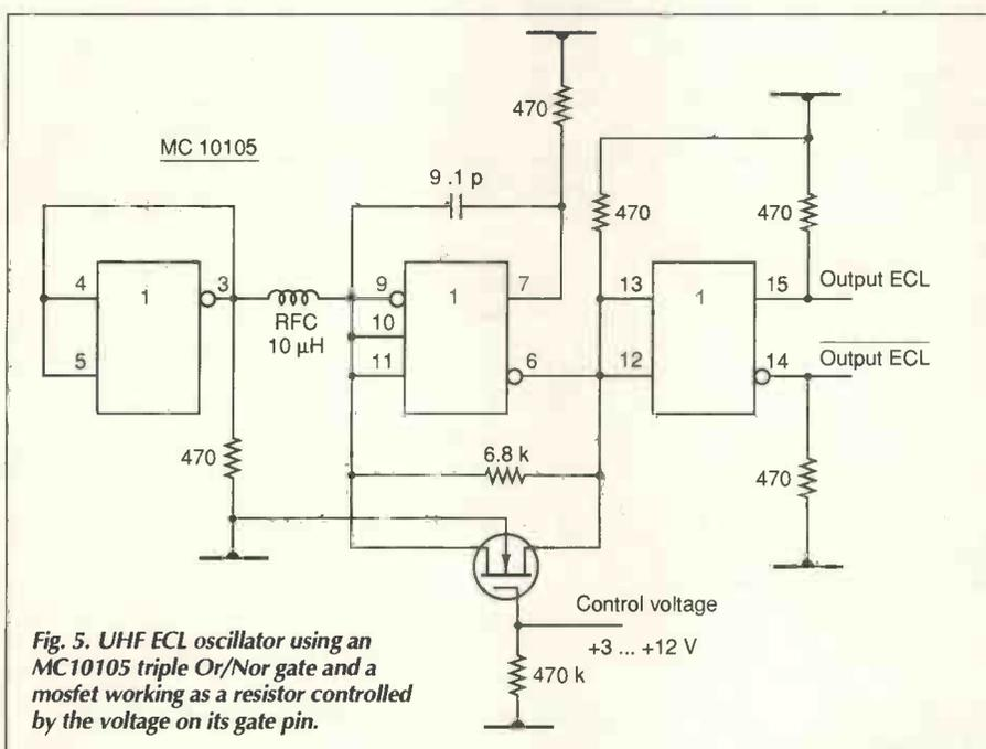
Fig. 5. UHF ECL oscillator using an MC10105 triple Or/Nor gate and a mosfet working as a resistor controlled by the voltage on its gate pin.
