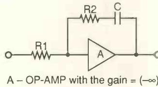
Fig. 2. Loop filter for second-order PLL.
