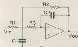
feedback filter<sup>5</sup>, because there are two feedback paths from the output of the amplifier to the RC network. Design equations of the filter are:
