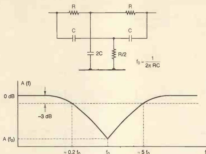
Fig. 14. To avoid coil in Cauer filter, this twin-T preceded by a lag-lead filter produces good results, the trough being better than 60dB with 2% components.
