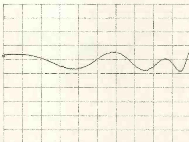
Fig. 4. Pass band ripple of the 5kHz SC filter with external crystal clock.
