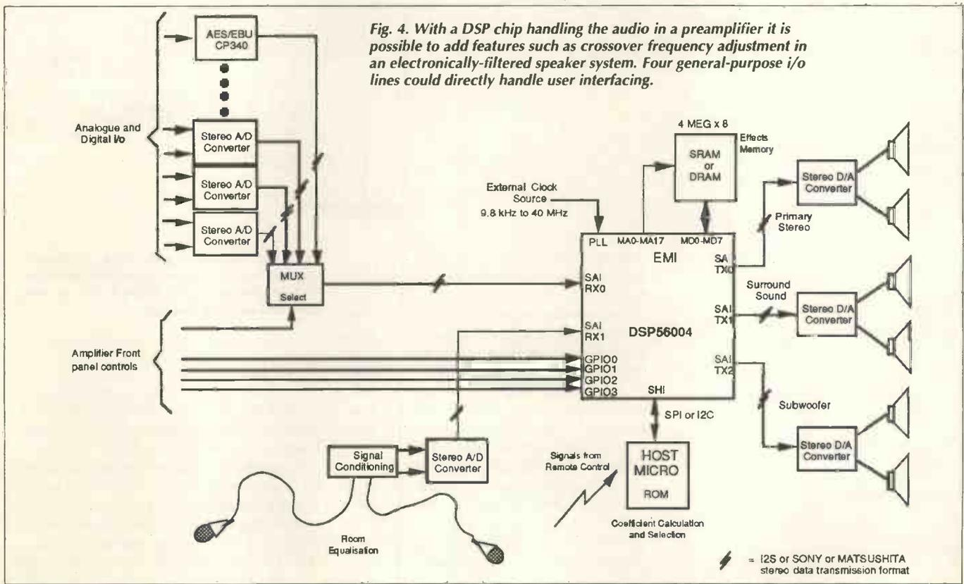
Fig. 4. With a DSP chip handling the audio in a preamplifier it is possible to add features such as crossover frequency adjustment in an electronically-filtered speaker system. Four general-purpose i/o lines could directly handle user interfacing.
