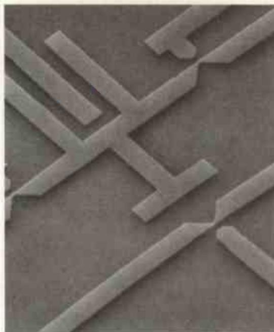
A memory cell consists of one gate-capacitor and one multiple tunnel junction (MTJ).
