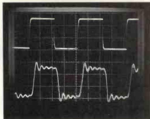
Fig. 10. Effect of non-linear delay versus frequency characteristics on a square waveform. Top trace, input 500Hz square waveform; bottom trace, output 5kHz elliptic filter  $v(X=0.5ms, Y=2v)$ .
