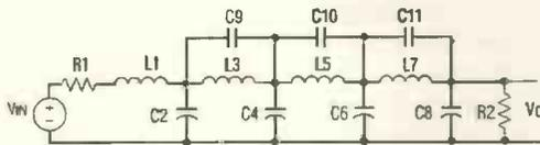
Fig. 5b. The MAX29X series filter structure emulates a passive eight pole lowpass filter. In the case of the elliptic types, this results in ripples in both the pass- and stopbands.
