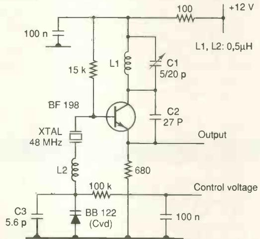
Fig. 7. Crystal oscillator capable of frequency variation of less than 1% by varicap diode in series with the crystal.
