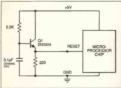
Fig. 1. This was a popular circuit for the reset function until engineers discovered how badly it oscillated.
