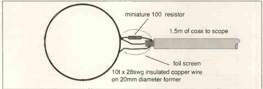
Fig.2. Electromagnetic probe.
