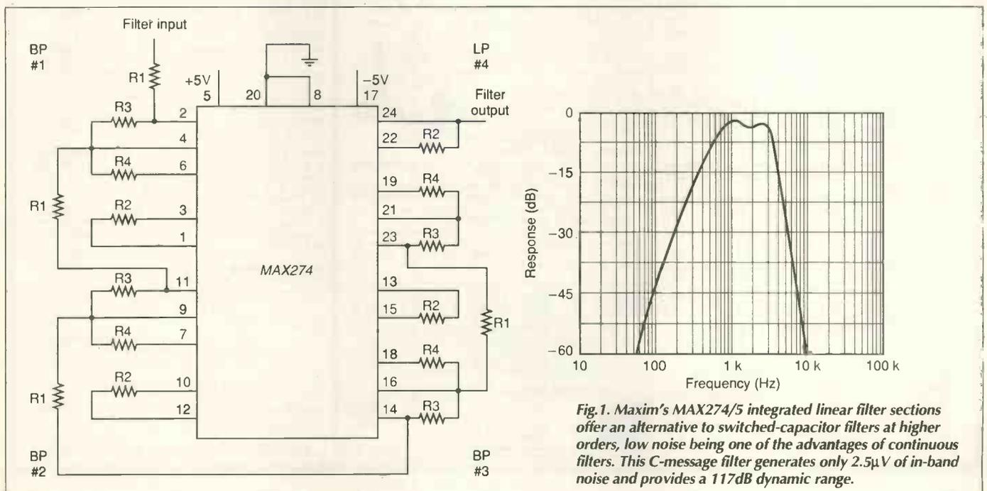
Fig.1. Maxim's MAX274/5 integrated linear filter sections offer an alternative to switched-capacitor filters at higher orders, low noise being one of the advantages of continuous filters. This C-message filter generates only 2.5µV of in-band noise and provides a 117dB dynamic range.
