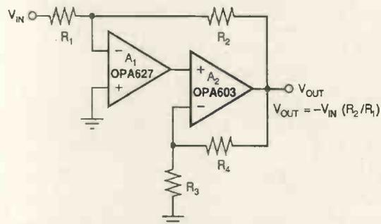
Fig. 1. Composite amplifier is better than the sum of its parts. DC and high-frequency performance are both enhanced and relatively unaffected by gain setting.
