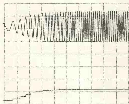
Fig. 1b. Using a small value of C, the swept oscillator output was applied direct to the detector circuit. The detected output (lower trace) follows faithfully the peak amplitude of the sweeper output (upper trace) over the partial scan shown, covering about 30Hz to 650Hz.
