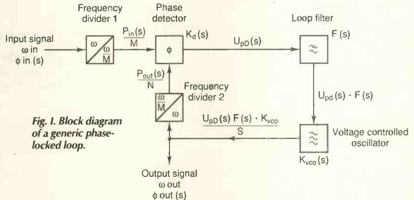
Fig. 1. Block diagram of a generic phase-locked loop.
