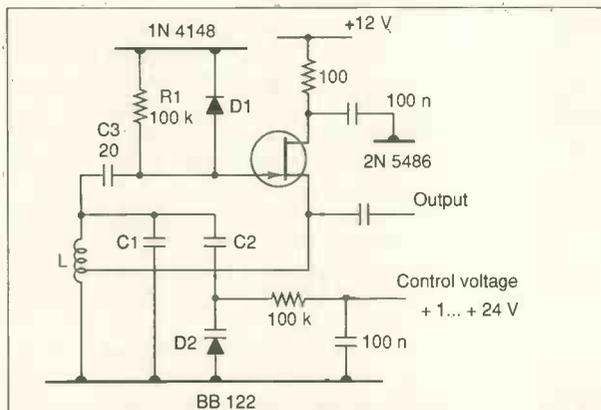
Fig. 1. Voltage-controlled oscillator using a fet for low-noise performance. Loose coupling via transformer tap and low-value capacitors assists frequency stability.
