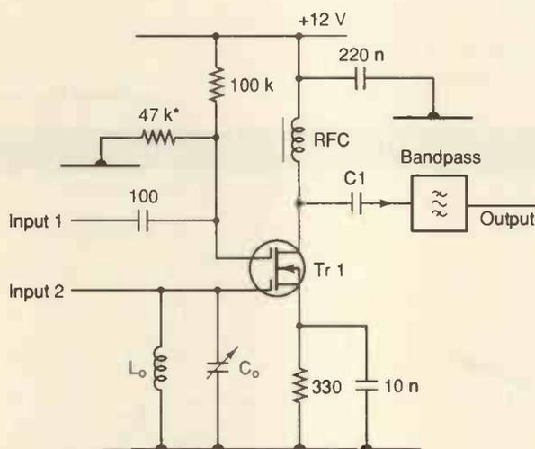
Fig. 16. Mixer based on a dual-gate fet. Both inputs may be wide-band if required.
