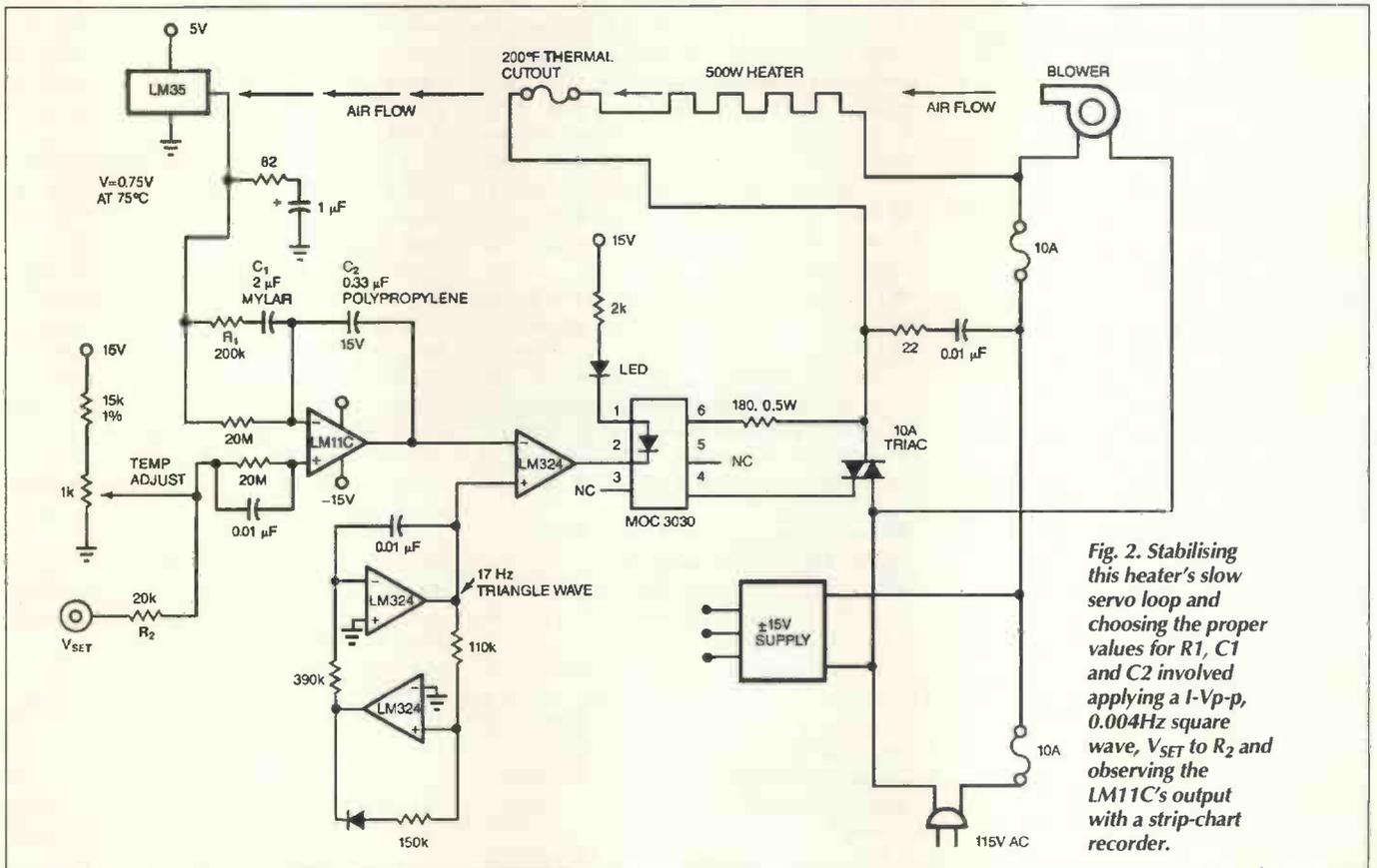
Fig. 2. Stabilising this heater's slow servo loop and choosing the proper values for R1, C1 and C2 involved applying a 1-Vp-p, 0.004Hz square wave, V<sub>SET</sub> to R<sub>2</sub> and observing the LM11C's output with a strip-chart recorder.
