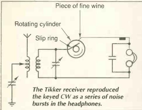
Even so this potential was generally much greater than that of the RF current at the antenna terminals. Fortunately, damping of the tuned circuit was minimal. Headphones presented an impedance approaching  $30k\Omega$  at 1.0kHz, so tuner resonance and transformation resulted in some voltage gain.
