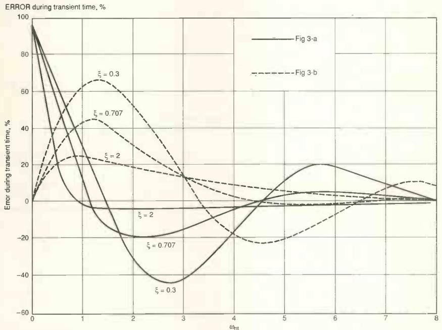
Fig. 3. Phase errors in response to stepped change of input phase (a) and frequency (b) for varying values of x.
