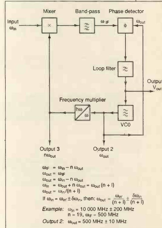
Fig. IV. PLL in use as a frequency divider.
