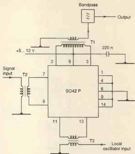
Fig. 15. SO42P used as a mixer up to 200MHz. Input frequency is rejected by 30dB on the mixed output level.
