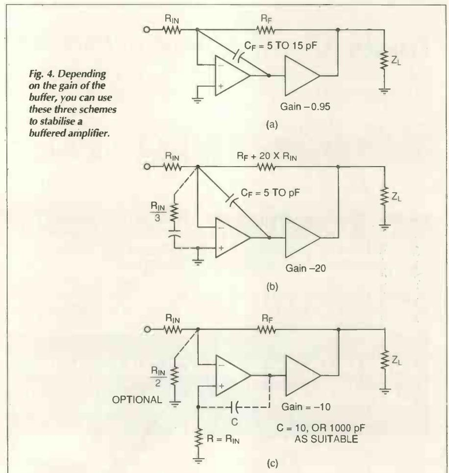
Fig. 4. Depending on the gain of the buffer, you can use these three schemes to stabilise a buffered amplifier.
