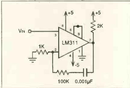
Fig. 3. This zero-crossing detector has no DC hysteresis but 50mV of AC-coupled hysteresis.
