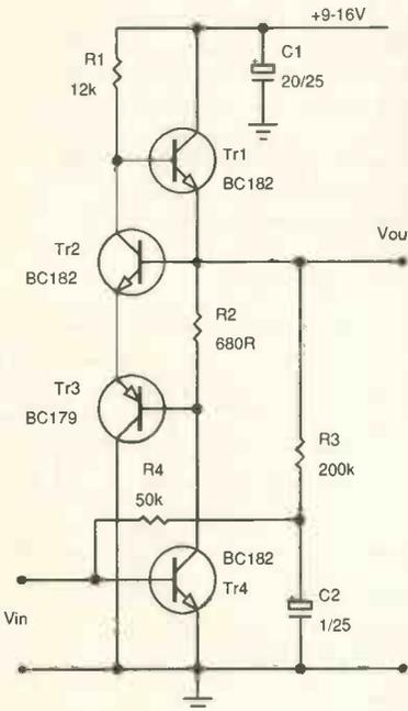
Since the  $Tr_{1,2,3}$  amplifier's frequency response is wide-band, the resulting amplifier exhibits a gain of over 60dB over a bandwidth of 850kHz into 50Ω, using BC182 and BC179 transistors. Feedback through  $R_2$  gives an output impedance of only a few ohms. Capacitor  $C_2$  across the bias resistors for the input stage removes AC feedback.
