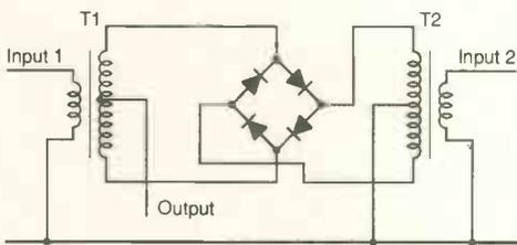
Fig. 8. Early type of double-balanced mixer used as a phase detector, the transformer ratios fixing the tuning range.
