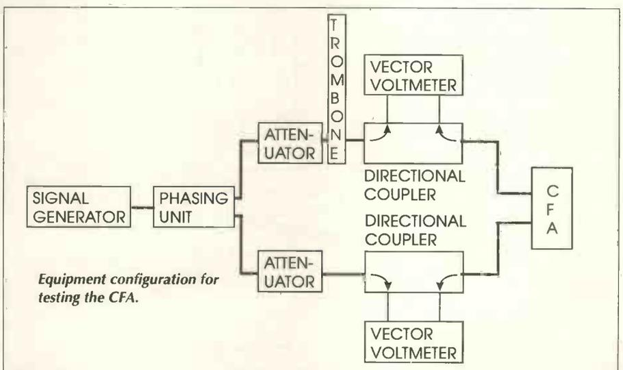
Equipment configuration for testing the CFA.
