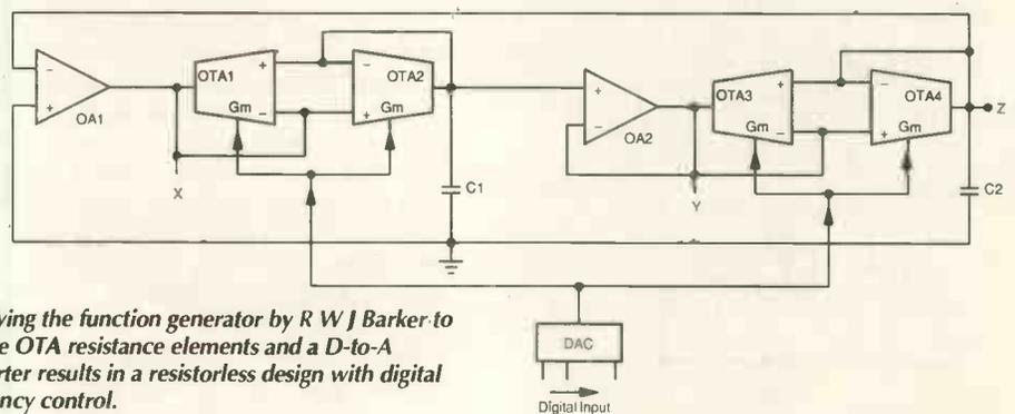
*Modifying the function generator by R W J Barker to include OTA resistance elements and a D-to-A converter results in a resistorless design with digital frequency control.*
