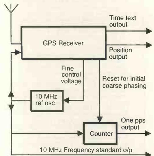
Fig. 5. Timing Receiver. A standard GPS receiver with an external clock generator and divider chain can equal any atomic clock in long term timing accuracy. Short term is degraded to tens of nanoseconds by Selective Availability.
