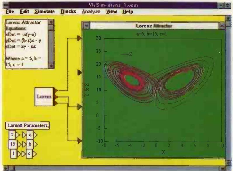
Fig. 2. A model of a Lorenz Attractor used to illustrate VisSim's features.
