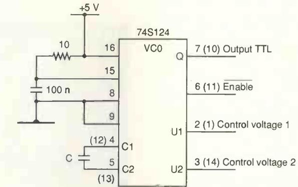
Fig. 4. Dual VCO, giving an output frequency of  $5 \times 10^{-4}/C$  (where C is in farads) up to about 60MHz. Tuning range is determined by voltage applied to pin 3.
