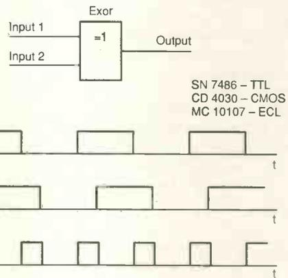
Above Fig. 10. Logical exclusive-OR phase detector. Output is a pulse-width-modulated pulse train - zero output when inputs in-phase. A low-pass filter on the output removes the pulses to leave DC.
