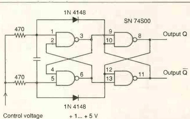
Fig. 2. Very simple, but linear oscillator, usable up to about 30MHz.
