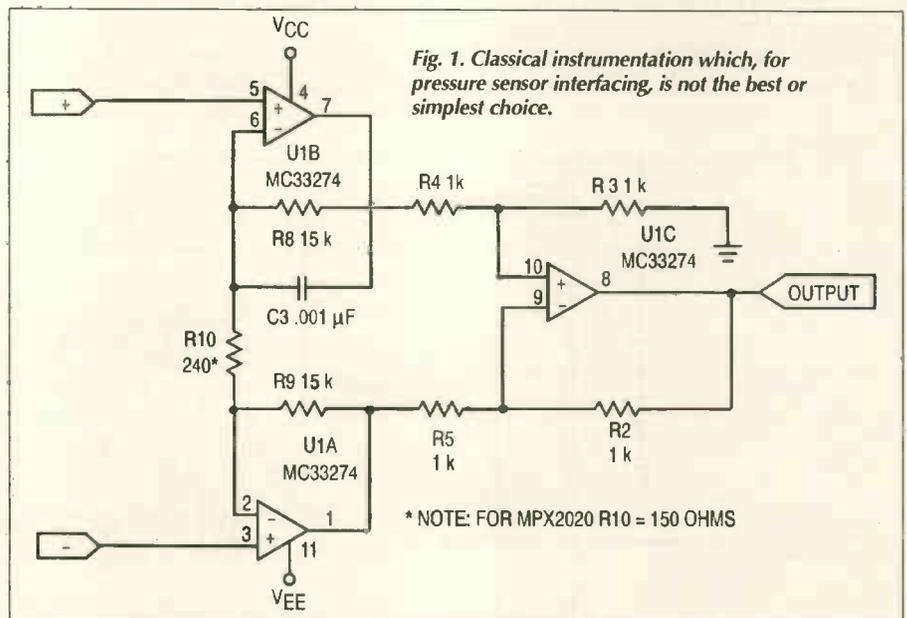
Fig. 1. Classical instrumentation which, for pressure sensor interfacing, is not the best or simplest choice.
