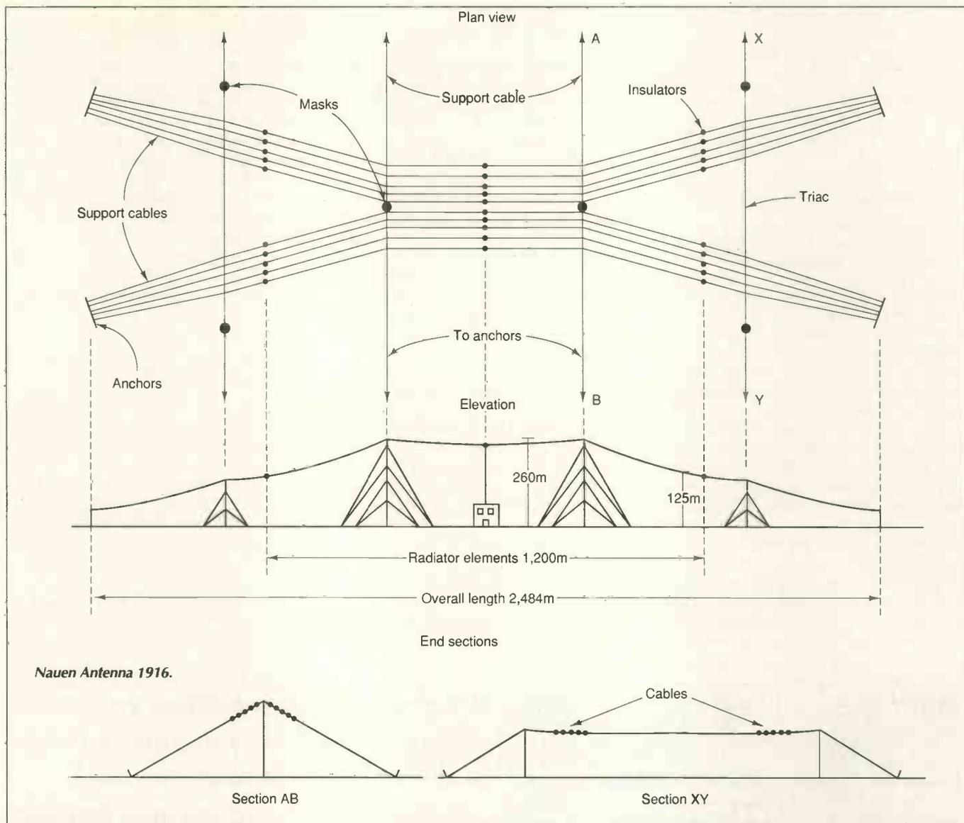
relay stations and it was from these that the Nauen very-long-wave antennas evolved. The original mast at Nauen was 100m tall with a 400m diameter umbrella. But in 1909, diameter was increased to 600m, and in 1911, one side of the umbrella was lengthed to give an overall length of 1626m, with the height of the main mast increased to 260m.
