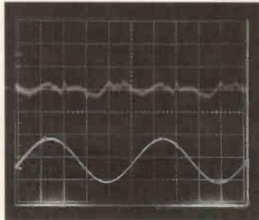
Fig. 4b. The circuit's output at 1kHz (lower trace) and the residual signal after filtering out the fundamental, representing the total harmonic distortion (upper trace).
