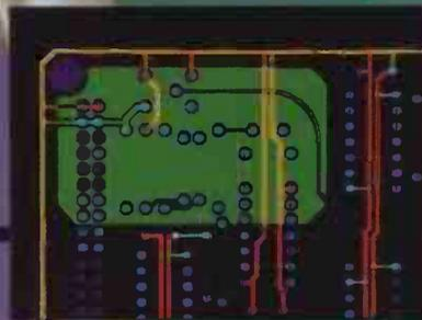
If you need partial ground planes then with the Dos extended board systems you can automatically create copper polygons simply by drawing the outline. The polygon is then filled with copper of the desired net, all correct pins are connected to the polygon with thermal relief connections and user defined gaps are respected around all other pads and tracks.
