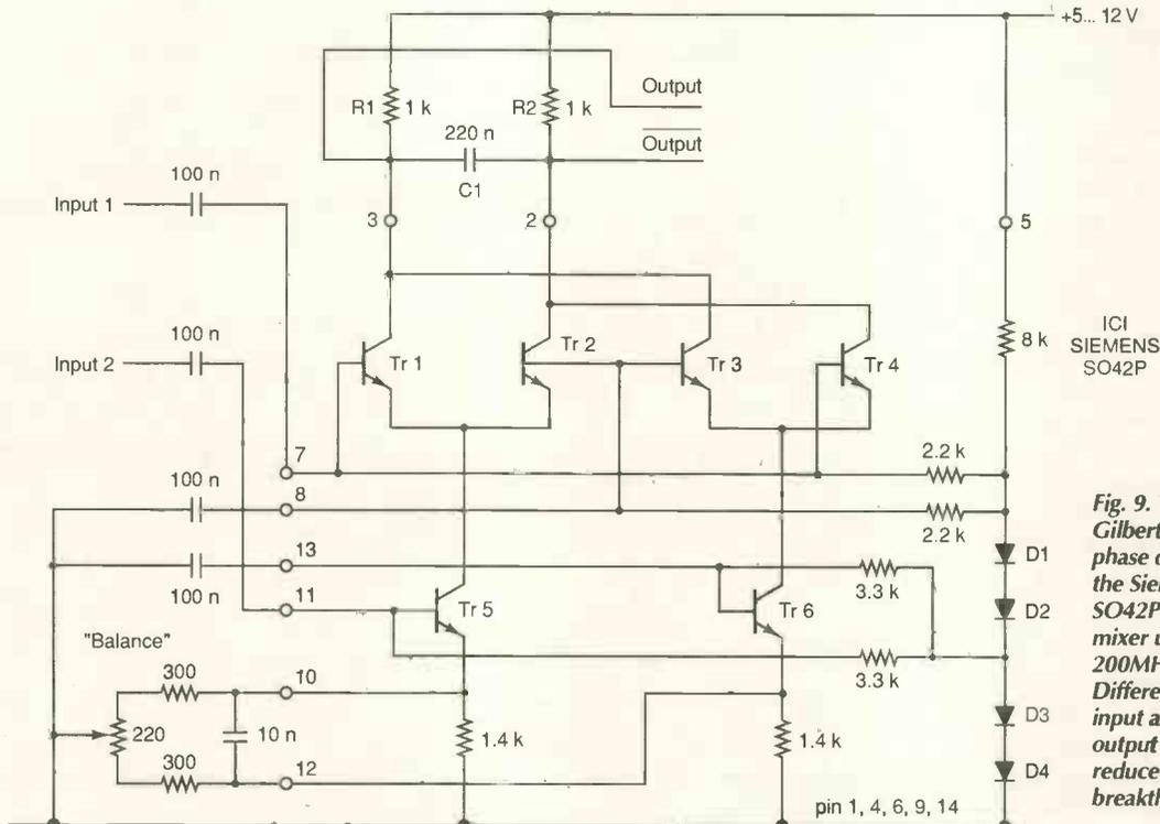
Fig. 9. Typical Gilbert Cell phase detector, the Siemens SO42P balanced mixer up to 200MHz. Differential input and output make for reduced breakthrough
