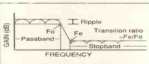
Fig. 2. Corner frequency of the elliptic filters is defined as the point where the filter output attenuation falls just below the pass band ripple.
