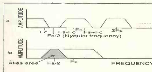
Fig. 1a. Frequency spectrum of continuous time signal sampled at  $F_s$ .
