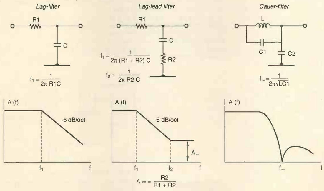
Below Fig. 13. Three types of filter used as loop filters in PLLs. Cauer type works well, but needs a coil.
