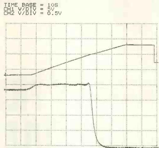
Fig. 2b. As 2a, but using the MAX293 elliptic filter with its 1.5:1 ratio of  $F_s$  to  $F_o$ .
