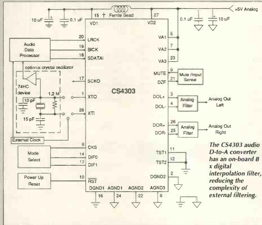
The CS4303 audio D-to-A converter has an on-board 8 x digital interpolation filter, reducing the complexity of external filtering.
