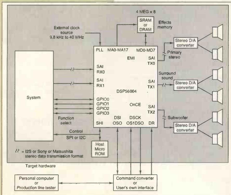
*Fig. 1. Implementing the audio DSP chip is not as difficult as might be expected. The system shown represents components not directly related to audio processing such as video circuits.*
