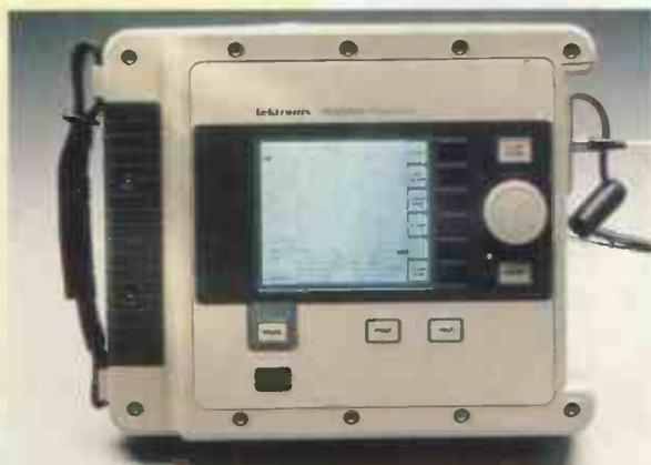
**Optical reflectometer.** Tek's *TFS3030 FiberMini* optical time-domain reflectometer offers single or dual wavelength analysis, automated fibre analysis, multiple measurements, control over measurement parameters and a display with infinite zoom. Basic model gives 18dB measurement for a 0.5dB loss up to 55km from the front panel. Tektronix UK Ltd, 0628 486000.
