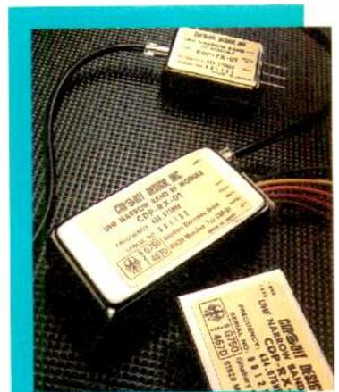
**Narrowband radio modules.** A matched transmitter/receiver pair by Circuit Design for the pan-European ETS-300-220 frequency of 434MHz is a now available. *CDP-TX-01* is a narrowband transmitter using a crystal oscillator with a  $\pm 4$ ppm stability and direct fsk modulation to allow 12.5kHz channel spacing. The *CDP-RX-01* receiver is a crystal-controlled double superhet with 120dBm sensitivity and  $\pm 5$ kHz selectivity. Low Power Radio Solutions Ltd. Tel., 0993 709418; fax 0993 708575.
