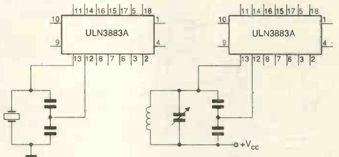
capacitance of about 7pF, and has to be taken into account when designing the external oscillator circuitry.
