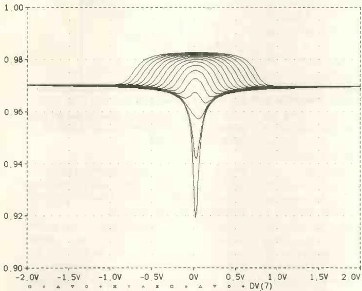
Left are curves for a bipolar complementary feedback pair, crossover region  $\pm 2V$ ,  $V_{bias}$  as a parameter. Fourth curve up provides good optimal setting – compare with curves on the right, for a fet source follower crossover region with  $\pm 15V$  range.
