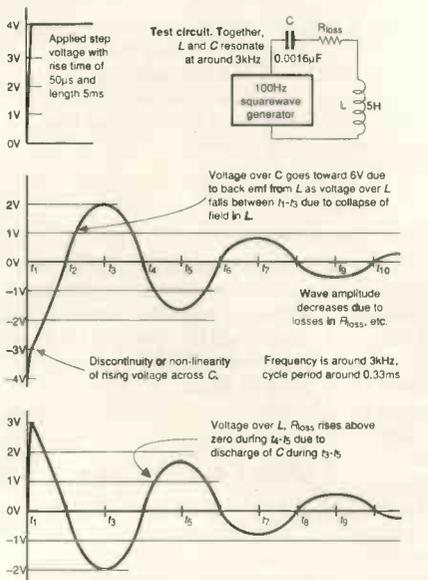
"Apart from the initiation waveform, which is non-linear and has a discontinuity, this waveform is explained by the mathematical analysis shown."
