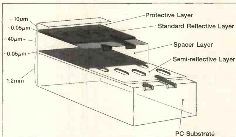
*Dual layer construction of Philips high-density CD system, whose complexity indicates initial take-up by the computer, not consumer, industry. Light beams will need to be focused separately on the two layers; each layer offers different read-out characteristics.*
