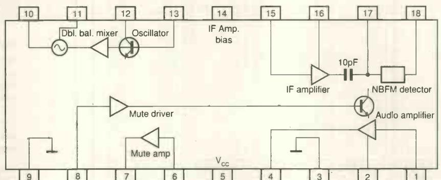
Fig. 2. The ULN3883A has an automatic standby mode which switches off the audio stage, making it particularly suited to battery applications such as a cordless telephone receiver.
