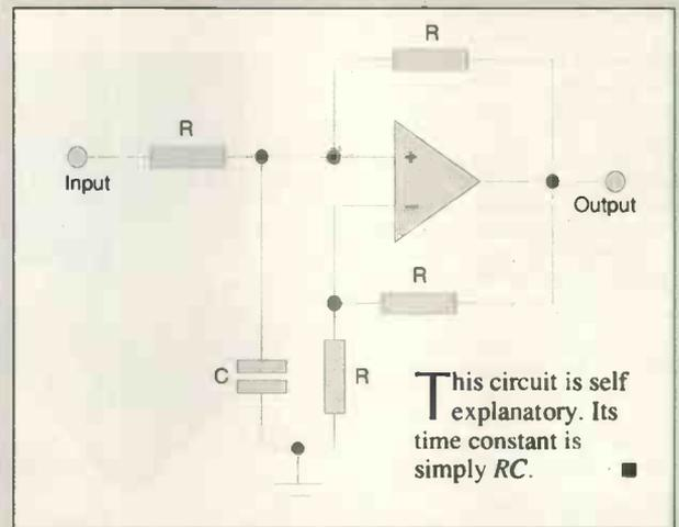
This circuit is self explanatory. Its time constant is simply  $RC$ .
