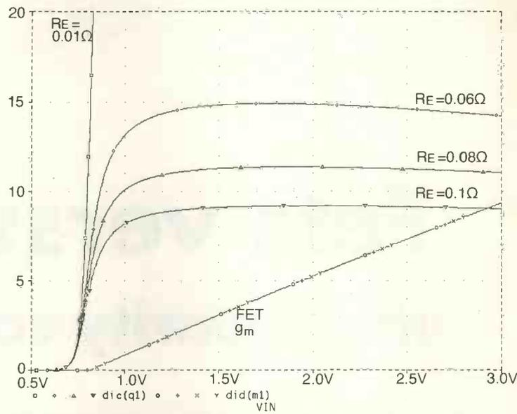
Fig. 3. Graph of transconductance versus input voltage for bjt and fet. The near-horizontal lines are bjt  $g_m$  for various  $R_E$  values.
