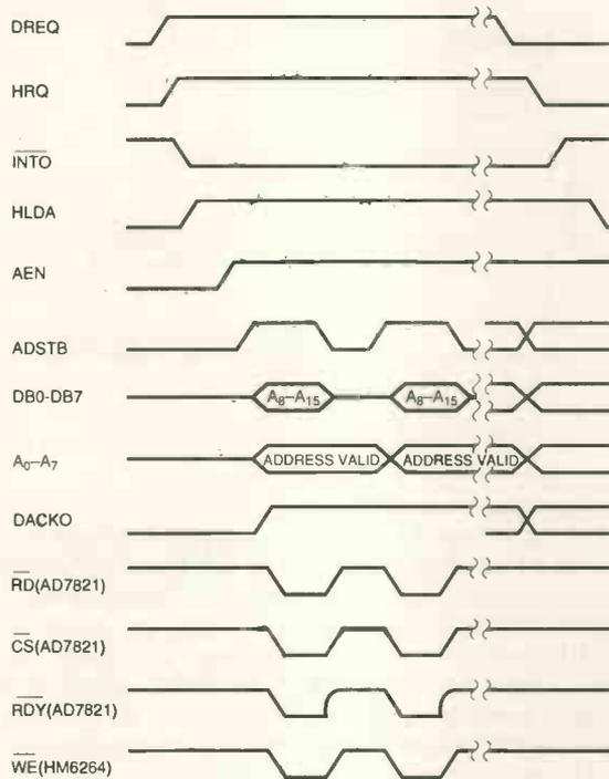
Fig. 6. 'Fake dma', used because the 8052 does not support true dma, allows rapid data transfer to memory.
