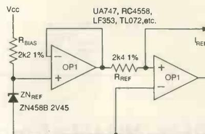
*Current source provides very high thermal stability. Output current is determined by value of  $R_{ref}$  and diode voltage.*
