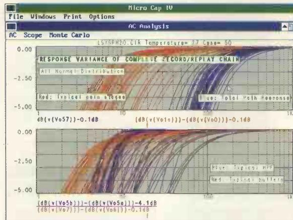
**Fig. 2. Unequalised frequency responses of a possible complete consumer-grade audio reproduction path (upper panel, blue plots). Upper panel red plots, and blue and red lower panel plots, show typical responses of constituent gain stages, high-pass filters and buffers. Each Monte Carlo run represents myriad design differences, as nearly all audio chains are made from effectively random equipment assemblies. There are no standards for  $f_{3L}$ . Y axis is decibels.**
