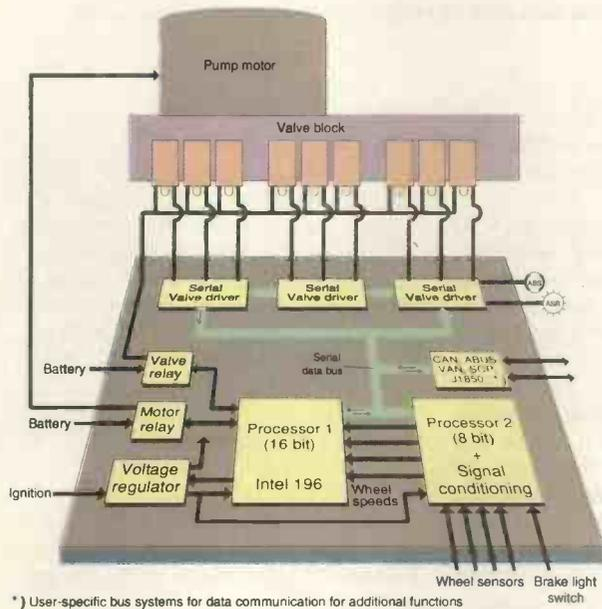
Fig. 5. In ITT's Teves Mk 20 ABS module, two processors – one of them 16 bits – work together, monitoring each other to eliminate the chance of a total loss of braking.
