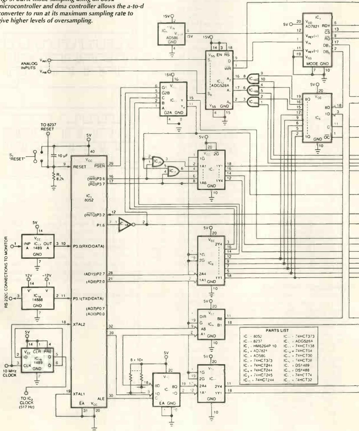
IC<sub>15a</sub>, this and IC<sub>15b</sub> ensuring that the CS\ line of IC<sub>4</sub> goes low only when an input/output read operation of IC<sub>2</sub> occurs. IC<sub>15c</sub> provides the correct polarity for the RD\ input and equalises the delay paths for the CS\ and RD\ lines, ensuring that the circuit obeys the CS\ to-RD\ setup time.
