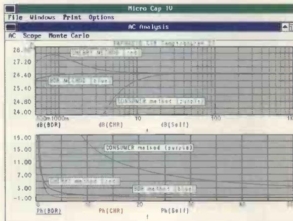
Fig. II. Frequency responses (upper panel) of the three contrasted circuits all provide negligible roll-off in the audio band >20Hz, but with true, frequency-dependent phase shift visible for a change (lower panel), the consumer/Self circuitry commits phase crime well within the ear's most sensitive domain.
