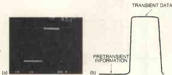
transient data; when playback mode starts, the first output from the counter will correspond to the memory location of the first pre-transient sample. To alter the ratio of transient to pre-transient samples, simply alter the connections from counter 1 to IC<sub>10</sub> and IC<sub>11</sub>.
