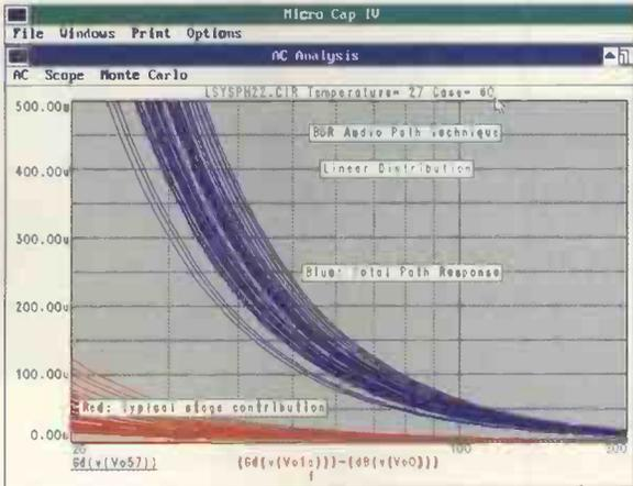
**Fig. 7. Phase disaster at path output. With consumer values, the phase response of the whole path is truly non-linear, and the rate of phase shift changes at hundreds of degrees every few Hz around 40Hz. In the lower panel, the phase change rate (enlarged x30) isn't even linear by 1kHz. Note also the wild singleton - a disparate of excess phase. Y-axis is degrees.**
