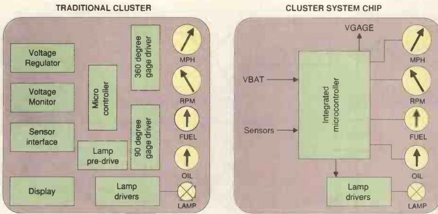
Fig. 4. Increasing microprocessor integration makes car electronics more reliable while improving compactness and maintainability.
