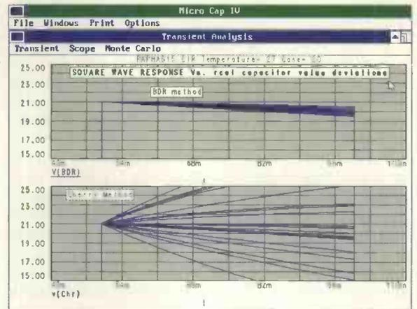
Fig. VII. Effect on the two square waves shown in the lower panel of Fig. IV when capacitor values are stepped over real world tolerances. The lower set of plots shows how - with most variations - Cherry's method fails to achieve the flat top that is its goal. The bdr method is clearly much less sensitive to part tolerance, though with more than 20 plots (a limit imposed for visual clarity) a few 'wild' plots will occur. Y-axis is volts.
