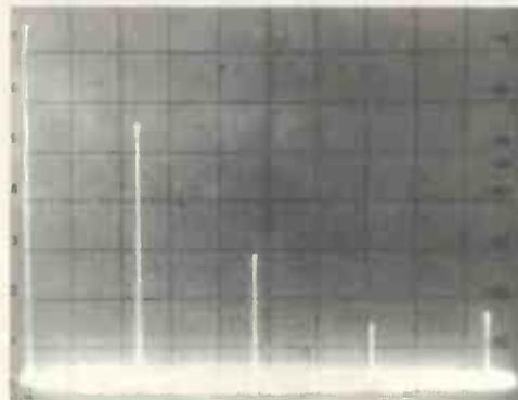
Fig. 6. Simple and fairly crude line-stabilised oscillator (a) gives output at (b); span 0-1000MHz, 10dB/div vertical, ref. level (top of screen) -10dBm. Fundamental component of (b) shown in (c), with centre frequency 235MHz and horizontal scale 5kHz/div, IF bandwidth 1kHz, video filter at max. (giving a post-detector bandwidth of 1.5Hz), 10dB/div. vertical, ref. level -30dBm.
