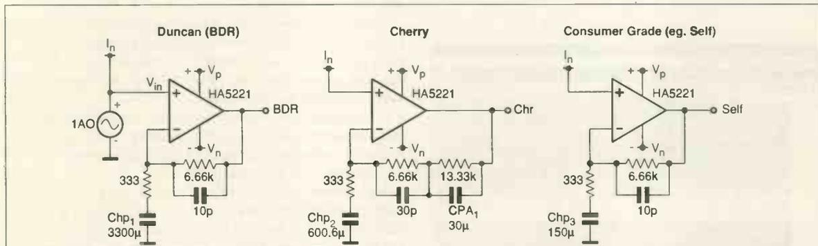
Fig. I. Three bass response approaches compared. Centre is Prof Cherry's "phase compensation" scheme. Note ac test source (left) drives all three. Measurements are referred to node labels; nodal numbering in MicroCap is automatic and transparent. Left and right circuits vary only in their elcap size. The Harris HA5221 IC model parameters are Level 1 for speed, and have been over tweaked but these factors have no appreciable effect on simulation accuracy or validity in our strictly If arena.
