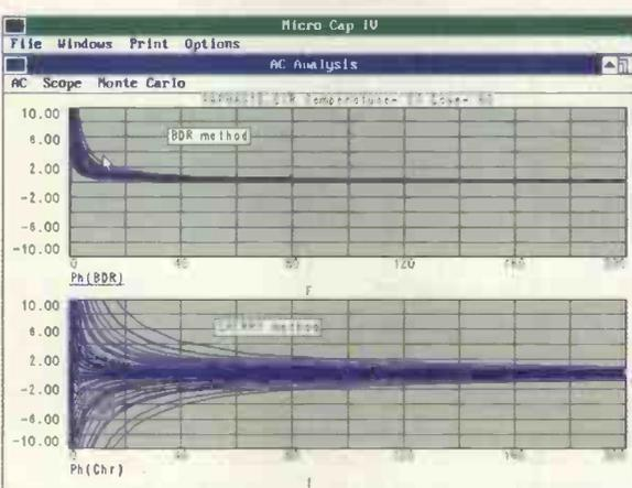
revealing true phase linearity so that a straight line on this linear scale, whether sloping or level, indicates absence of waveform distortion. Anything bending is slurring the signal with respect to frequency.
