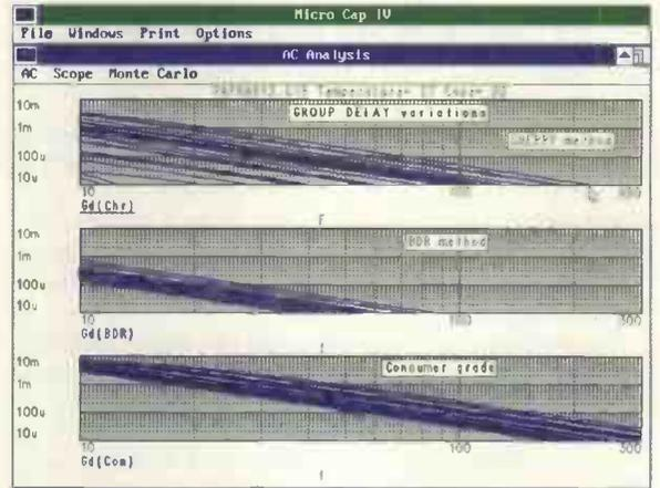
Fig. VIII. Three signal delay patterns. Group delay is plotted with the 'Gd' operator. For clarity with the three, smaller scales and because smooth Gd plotting demands slower runs than phase or amplitude, the number of Monte Carlo runs has been reduced from 60 to 30.
