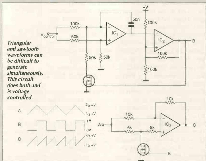
Triangular and sawtooth waveforms can be difficult to generate simultaneously. This circuit does both and is voltage controlled.
