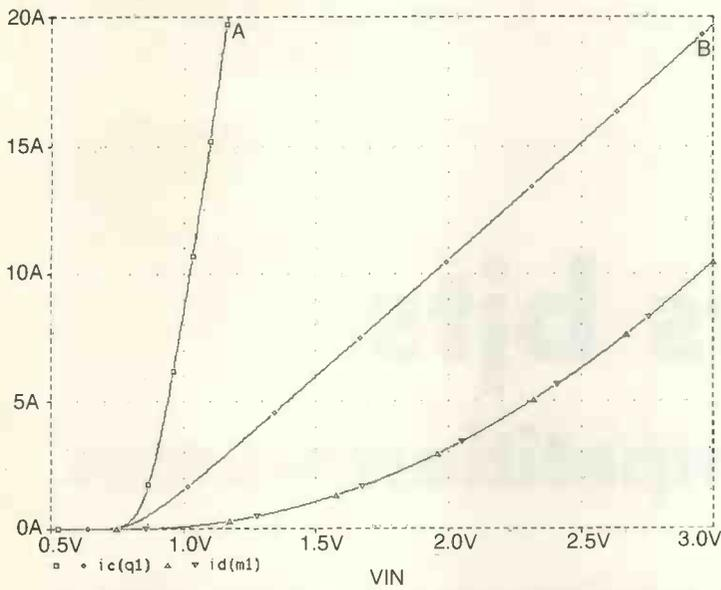
Fig. 2. Graph of  $I_C$  and  $I_D$  for the bjt and the FET. Curve A shows  $I_C$  for the bjt alone, while Curve B is the result for  $R_E=100m\Omega$ . The curved line is the  $I_D$  result for a power fet without any degeneration.
