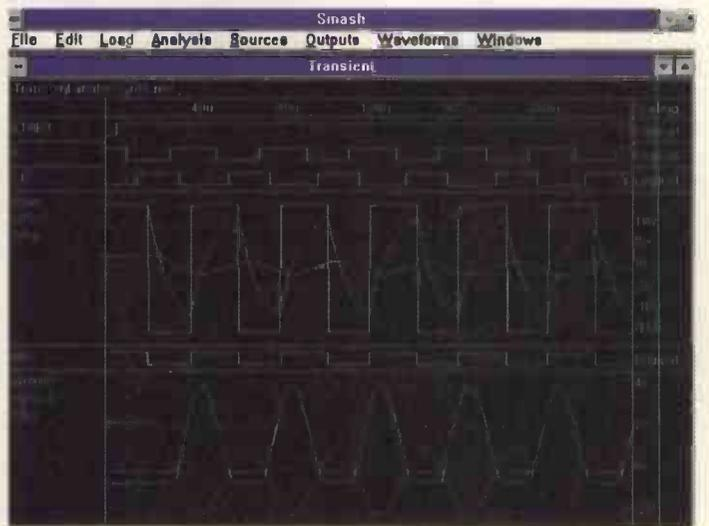
F: An example of running the transient analysis routine for a mixed analogue and digital circuit. In this case, *Smash* has to deal with both analogue voltages and logic levels. Whenever a node connects to both analogue and digital components, it becomes an interface node.
