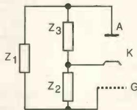
**Fig. 1. O'Connor's universal oscillator circuit.**  $Z_1$  is a reactance of one sign while  $Z_2$  and  $Z_3$  are both of the other. For 'valve' read n-p-n bipolar, n-channel fet, hemt etc, as appropriate.
