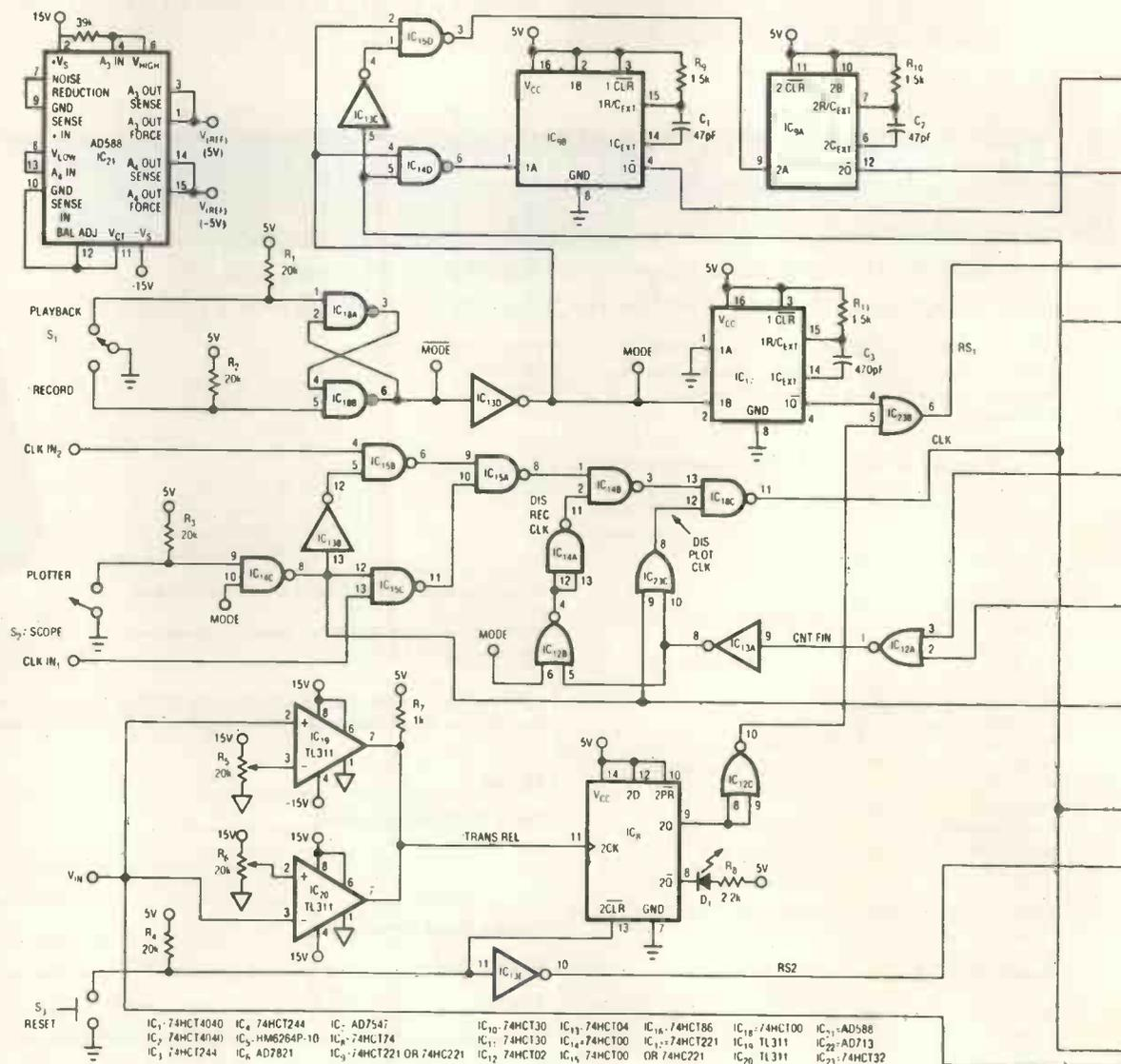
fast clock input, CLK IN<sub>1</sub>, for the clock source in record mode or when displaying stored data on an oscilloscope. A slower clock input, CLK IN<sub>2</sub>, is for use when printing data on an X-Y plotter.
