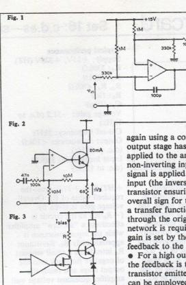
again using a common emitter output stage has the feedback applied to the amplifier non-inverting input, while the signal is applied to the inverting input (the inversion in the transistor ensuring the correct overall sign for the gain). For a transfer function that passes through the origin a pre-biasing network is required. Again the gain is set by the ratio of the feedback to the input resistor. For a high output-impedance,
