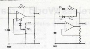
• An unequal mark-to-space ratio may be obtained by using the circuit shown right. The two resistors R<sub>18</sub> and R<sub>1b</sub> are selected by the switching action of diodes D<sub>1</sub> and D<sub>2</sub>, D<sub>1</sub> conducting when the output is negative, and D<sub>2</sub> when the output is positive.
