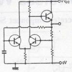
Addition of Tr<sub>3</sub>, as shown middle, allows the timing of the output square wave to be more nearly controlled by the R<sub>1</sub>C<sub>1</sub> time constant. Tr<sub>1</sub> and Tr<sub>3</sub> form a long-tailed pair so that the junction of C1 and R1 are effectively connected to one intput of a differential operational amplifier.
