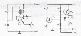
• The  $R_1C_1$  timing components may be connected to the base of  $Tr_1$  as shown in the middle right circuit with a potentiometer  $R_2$  fixing the emitter voltage and hence the time taken for  $Tr_1$  to switch on as  $C_1$  charges through  $R_1$ .
