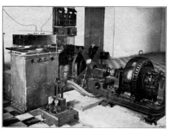
The Transmitting Apparatus, showing Rotary Spark Gap, with H.T. Signalling Key in foreground. Pipes convey the air blast to the contact.
