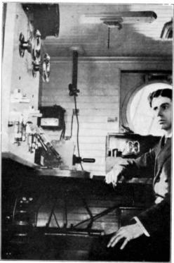
Marconi Apparatus in a Revenue Cutter in the Arctic.
