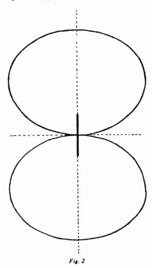
such a diagram in the case of  $d = \frac{\lambda}{2}$ . It is formed by two flat tangent curves. But when d diminishes with regard to  $\lambda$  these curves tend to become circles, so that from  $d = \frac{\lambda}{6}$  downwards these curves are practically circular. Fig. 3 shows this case.
