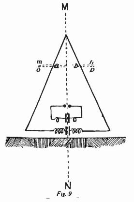
of the looped aerial) will be the sum of the actions of all the pairs of elements, and if the maximum width of the aerial does not exceed  $\frac{\lambda}{6}$ , the diagram of the intensity of electromagnetic field generated by these aerials will be formed by the two tangent circumferences, like those of Fig. 3. The looped aerials are therefore directive aerials, having the direction of maximum radiation contained in their own plane; perpendicularly to their plane the radiation is nil.
