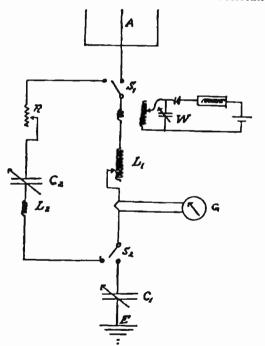
Fig. 1. Diagram of Apparatus for measuring Antenna Resistance
