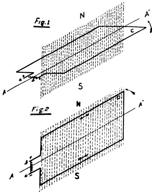
maximum speed. In this case *b* will be *plus* (Positive) and *a* *minus* (Negative). If *a* and *b* are connected together so a current can flow, it will flow from *b* to *a* indicated by the arrow along side the loop. The E. M. F. has passed through all values from zero to its maximum, that is, the E. M. F. has had a different value for every change in position of the loop. These values are called instantaneous values, and will be discussed later.
