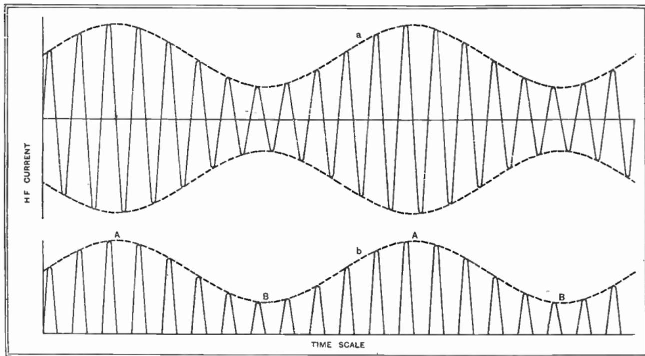
Fig. 75 : Modulated R.F. current (diagram a). Over any period of time appreciably greater than an R.F. cycle, the average current is zero, and so is inaudible in earphones. The same current, rectified, is shown in diagram b. The average current now rises and falls at modulation-frequency and can now be heard in earphones
