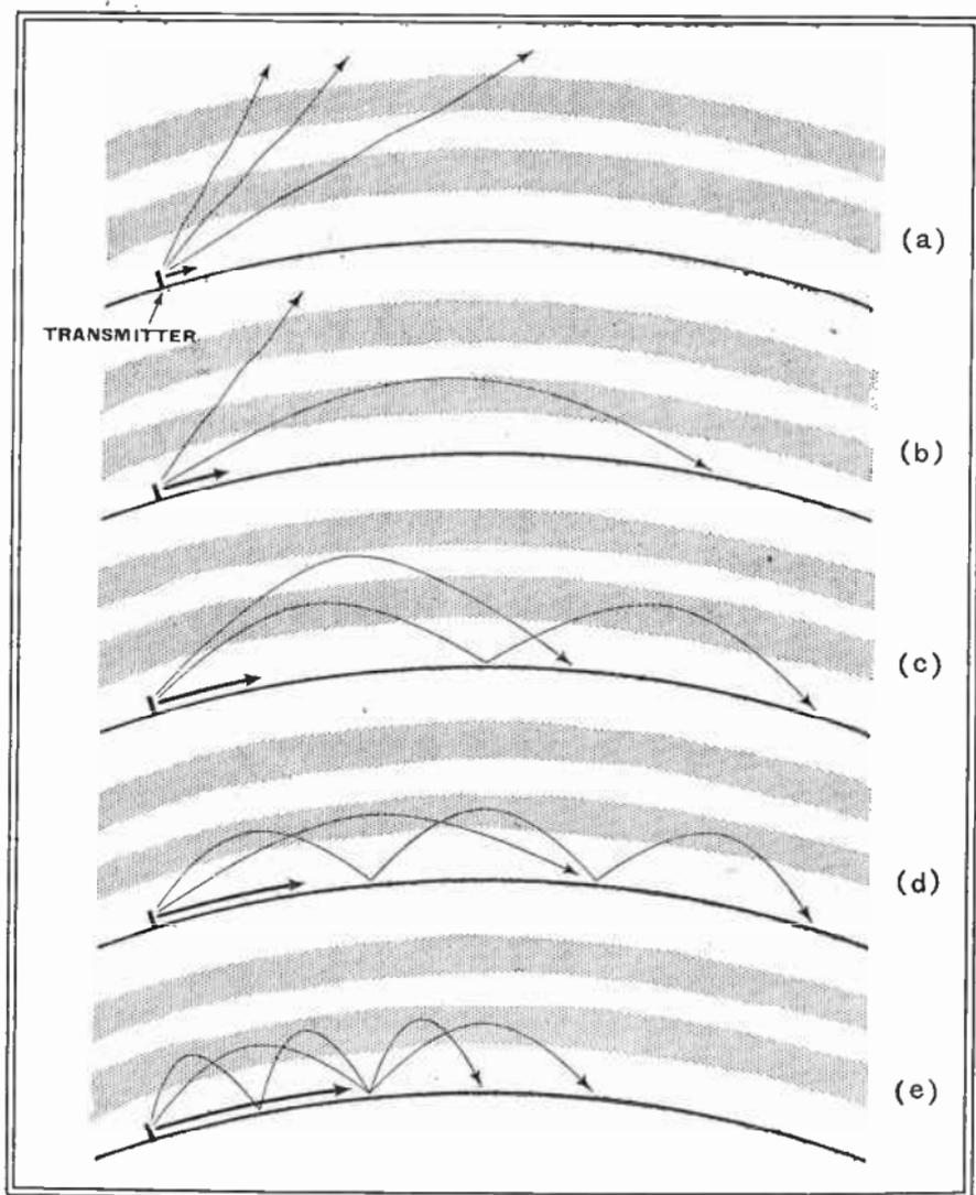
Fig. 168 : Showing (not to scale) the relative ranges of ground wave and reflected wave from very high frequencies (a) to very low (e)
