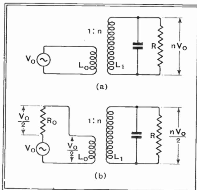
Fig. 94: (a) R.F. transformer. The tuned secondary, of dynamic resistance  $R$ , is shown as a loss-free circuit shunted by  $R$  as load-resistance. (b) Where the source (aerial, valve, etc.) has resistance, maximum volts on  $R$  are obtained when  $n$  is so chosen as to make the apparent resistance of the primary equal to that of the source. For this,  $n = \sqrt{\frac{R}{R_0}}$ , and the voltage distribution is as shown
