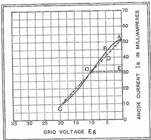
Fig. 125 : Dynamic curve of pentode with 10,000-ohm load. Ideal characteristic giving zero second and third harmonics is shown dotted. Percentage third harmonic =  $\frac{BD}{AE} \times 67$  approximately
