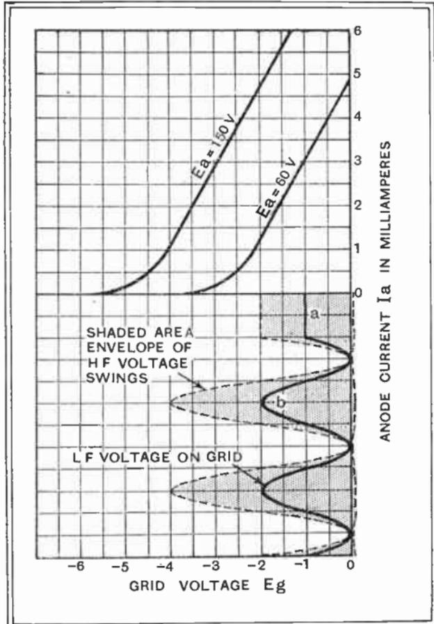
Fig. 87 : Curves showing reason for overload of grid detector. Even though the rectified voltage  $b$  on the grid may not overrun the straight part of the characteristic, the R.F. voltage accompanying it may cause anode-bend detection
