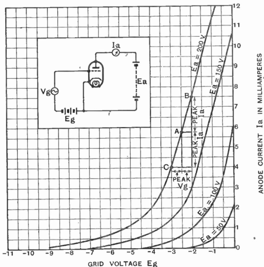
Fig. 65 : Anode-current grid-voltage curves of a medium-impedance indirectly heated triode. The alternating anode current caused by an alternating grid-voltage  $V_g$  can be read from the curves
