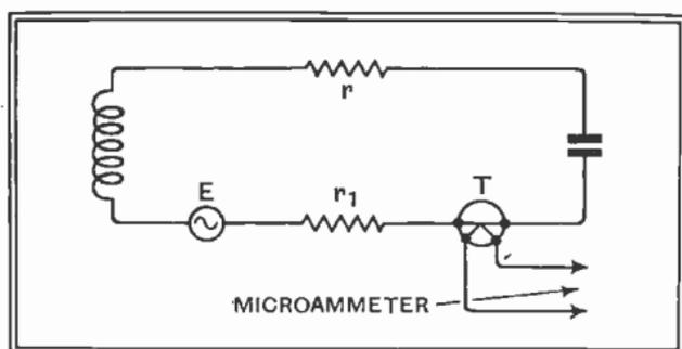
Fig. 58 : Simple method of determining series resistance  $r$ . If the current is noted when  $r_1 = 0$ , and then reduced to half this value by introducing and adjusting  $r_1$ , the necessary value of  $r_1$  is  $r$ . The resistance of the H.F. milliammeter (thermo-junction T) is included in  $r$ , and must be allowed for.
