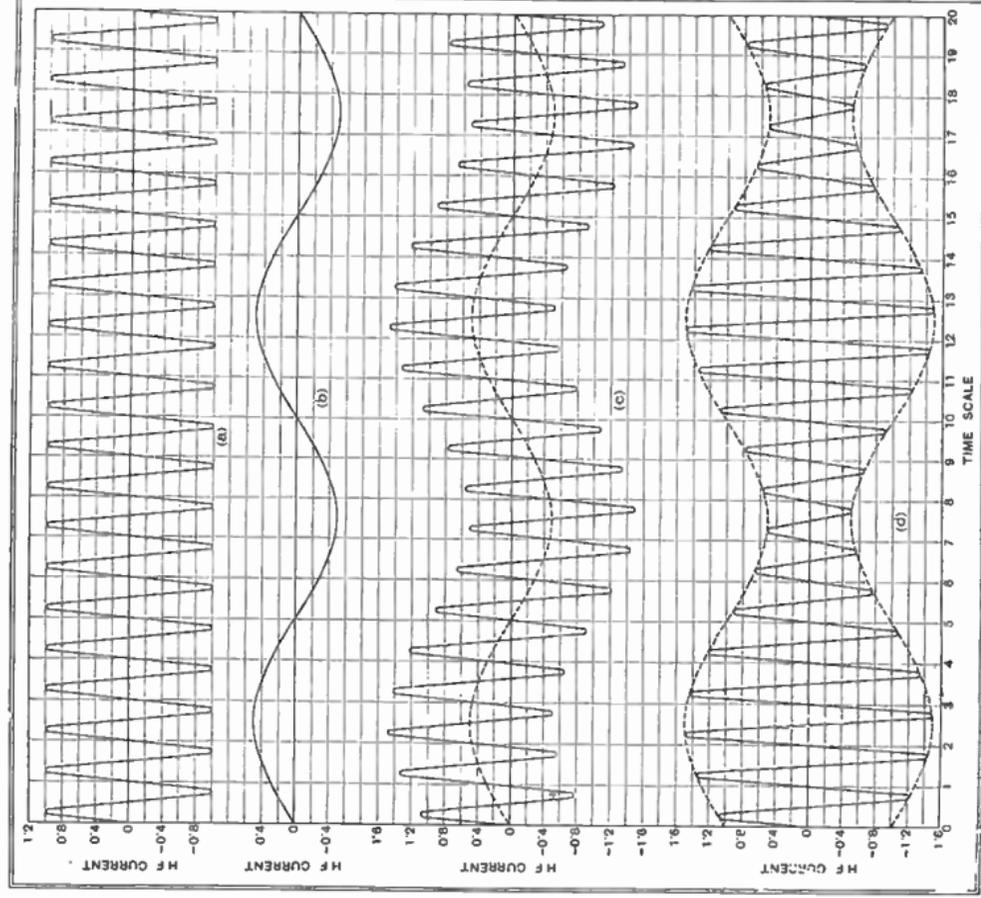
Fig. 72: Diagrams *a* and *b* show a radio-frequency current and a musical note to be combined with it for transmission. Mere addition of the currents results in *c*, in which the currents remain separate so that only the R.F. component would be radiated. Diagram *d* shows the modulated carrier resulting from multiplying the curves as described in the text: it is radiated complete from the aerial
