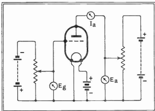
Fig. 62 : Circuit for taking characteristic curves, as in Fig. 63 or 64, of triode valves
