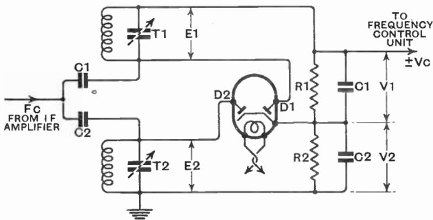
Fig. 152 : The circuits  $T_1$  and  $T_2$ , tuned one on either side of the correct intermediate frequency, pass to the double diode voltages which, when rectified, can be made to control oscillator-frequency
