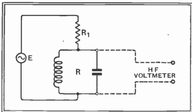
Fig. 57: Simple method of determining dynamic resistance for a parallel-tuned circuit. If  $R_1$  is adjusted until the R.F. voltmeter reads  $E/2$  volts, we know that  $R_1 = R$
