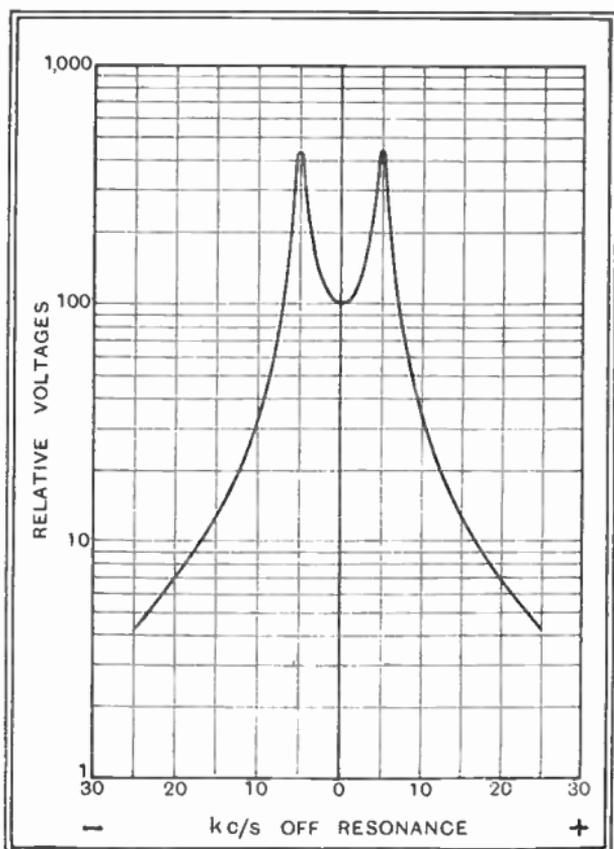
Fig. 145: Showing how "rabbit's ears" develop when an attempt is made to broaden the peak by closely coupling coils of high  $L/r$ .  $L/r = 140$ .  $X/r = 79$  (formula 3)
