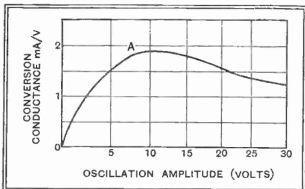
Fig. 138 : Type of relationship between oscillation amplitude and conversion conductance of frequency-changer. The oscillation amplitude is not critical so long as it exceeds a certain value in the neighbourhood of A
