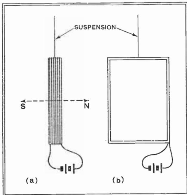
Fig. 18 : A coil, free to rotate, sets itself in the orientation indicated, when a current is passed through the winding
