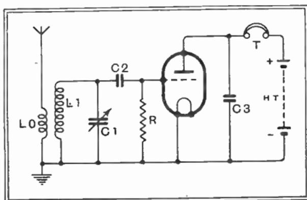
Fig. 93: Circuit of single-valve set in which a triode valve is used as grid detector and amplifier of the detected signals
