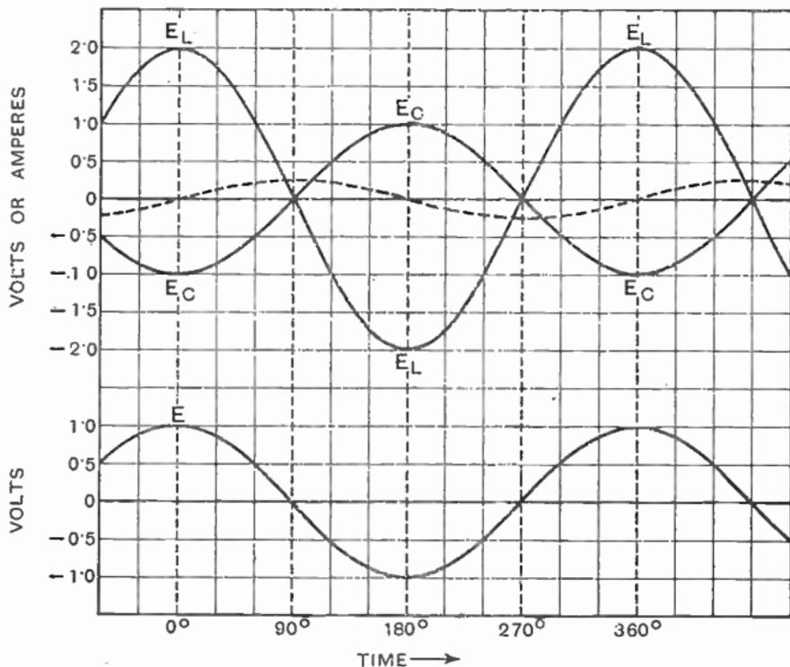
Fig. 47 :  $E_C$  and  $E_L$  represent the voltages across C and L of Fig. 46 when the current shown by the dotted curve is flowing. These voltages are at every instant in opposition and together make up to the voltage E
