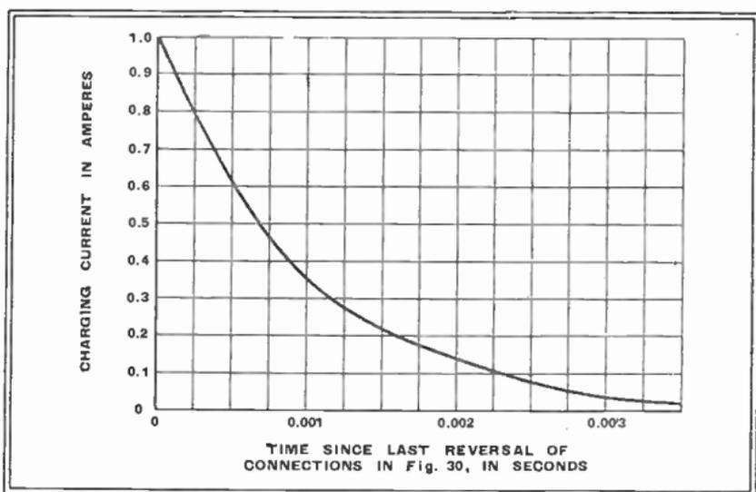
Fig. 31 : Showing the rapidity of the decay of the current after each reversal of direction
