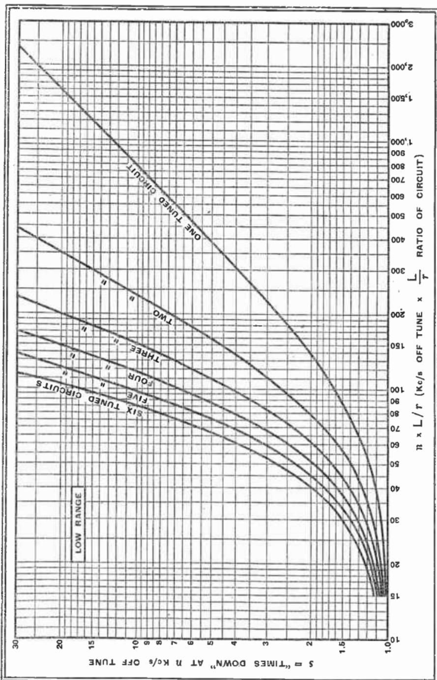
Fig. 115 a : General data-curves showing relationship between  $n \times L/T$  and  $s$  for 1 to 6 tuned circuits in cascade. Where value of  $s$  exceeds 10, use the continuation of these curves in Fig. 115 b
