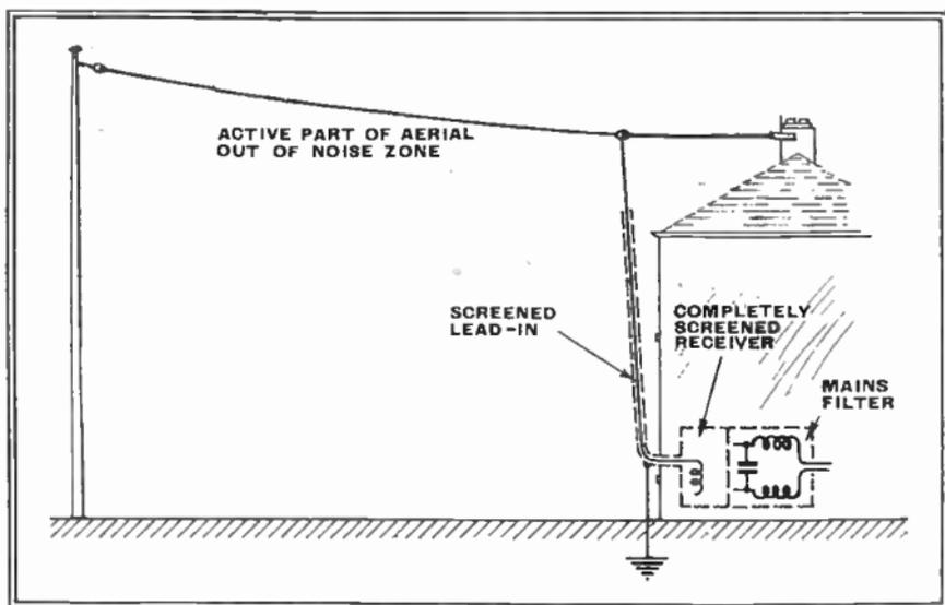
Fig. 173. Diagram of a screened-downlead anti-interference aerial
