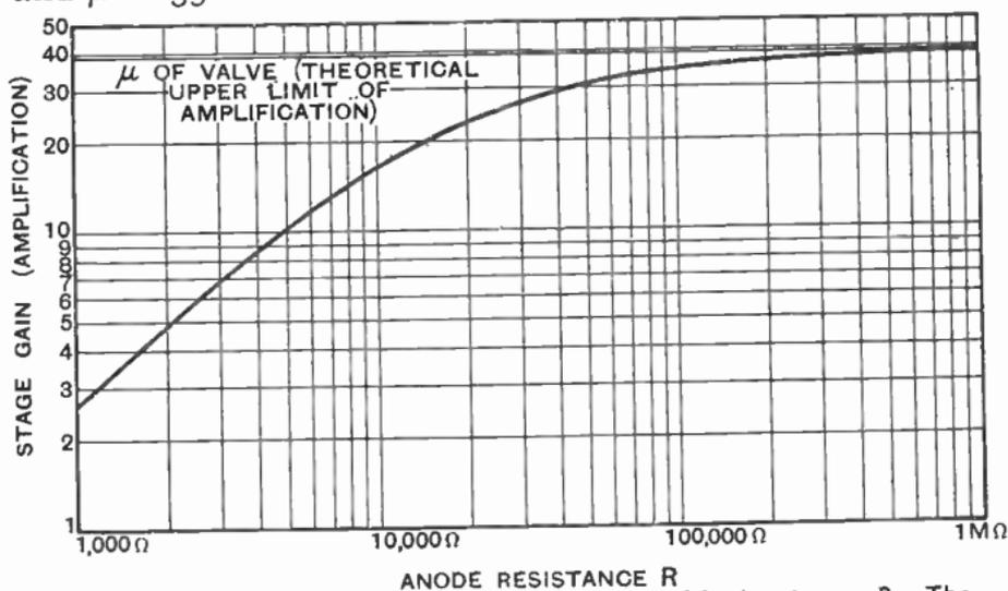
Fig. 68: Amplification of stage with different values of load resistance  $R$ . The valve, throughout, is supposed to have  $\mu = 39$ ,  $r_a = 14,400$  ohms
