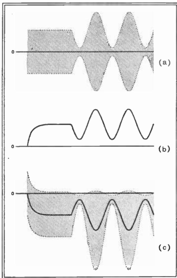
Fig. 84 : When a radio-frequency wave *a* (shown first unmodulated and then modulated) is applied to a diode detector having a time constant intermediate between the periods of the modulation frequency and the radio frequency, the voltage across condenser is as at *b*, and across diode as at *c*, where the full line is the average of the R.F.
