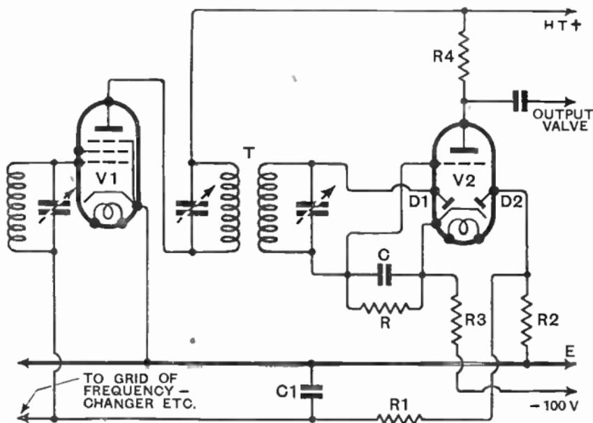
Fig. 151 : Amplified A.V.C., with delay. Initially positive, the cathode of  $V_2$  is driven down to earth potential by the grid bias generated by rectification at  $D_1$ . At this point  $D_2$  begins to draw current, and A.V.C. starts work
