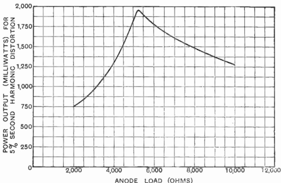
Fig. 122 : Relation between anode load and available power, allowing 5 % second-harmonic distortion, for the valve of Fig. 121 worked at point A
