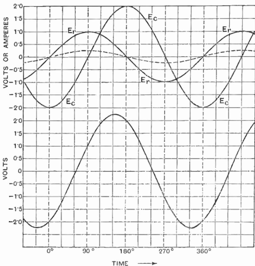
Fig. 42 : In the upper curve,  $E_r$  represents voltage across the resistance, and  $E_c$  voltage across the condenser, of Fig. 41. The lower curve shows the resultant total voltage; that which the generator must have to drive 0.25 amp. through the circuit
