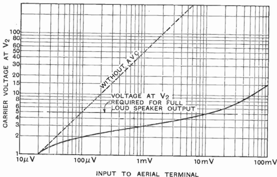
Fig. 148 : A.V.C. curve for system of Fig. 147. Note that if 5 v. at  $V_2$  is wanted for full output, the A.V.C. is unnecessarily limiting output on all inputs from  $20\mu\text{V}$ . to  $10\text{ mV}$
