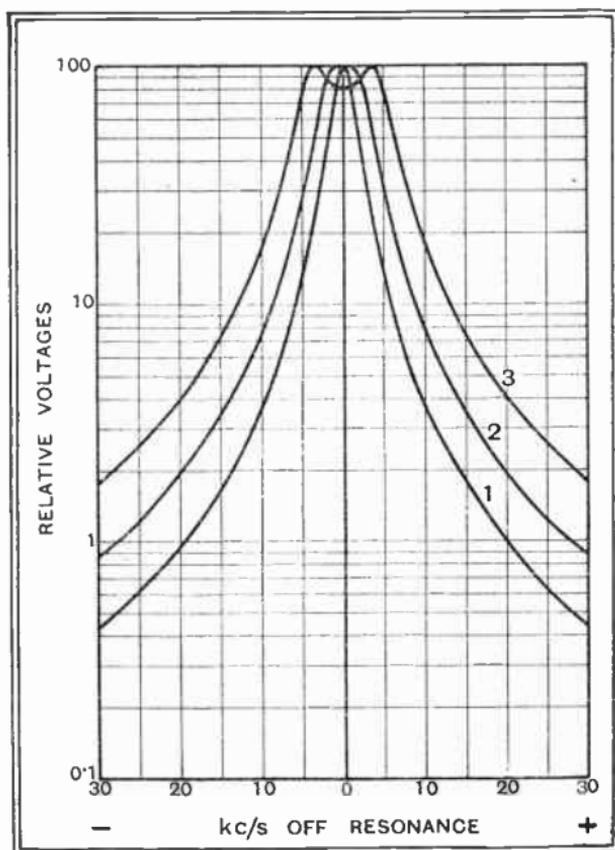
Fig. 143: Resonance curves of two tuned circuits, each  $L/r = 40$ . (1) Cascaded:  $X/r = 0$ . (2) Critically coupled  $X/r = 1$ . (3) Coupled to give overall band-width  $\pm 5$  kc/s.  $X/r = 2.04$ . (See formula 6)
