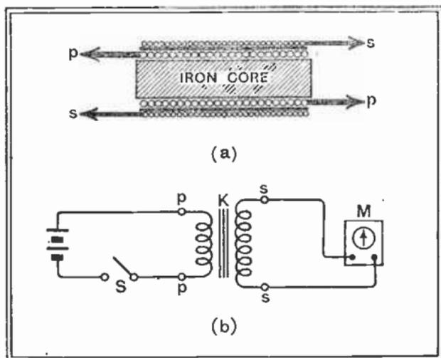
switch, M registers the momentary flow of a current in the opposite direction to that observed on closing it, while the current in the primary can be shown to drop practically instantaneously to zero.
