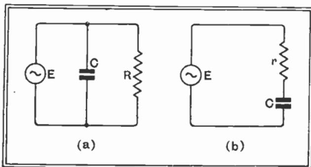
Fig. 33 : A condenser which absorbs energy when a current flows through it can be represented as a perfect condenser with a resistance either in parallel (a) or in series (b). Watts lost are (a)  $E^2/R$  or (b)  $I^2r$ . R and r are related by the equation  $\frac{1}{2\pi f C R} = 2\pi f C r$
