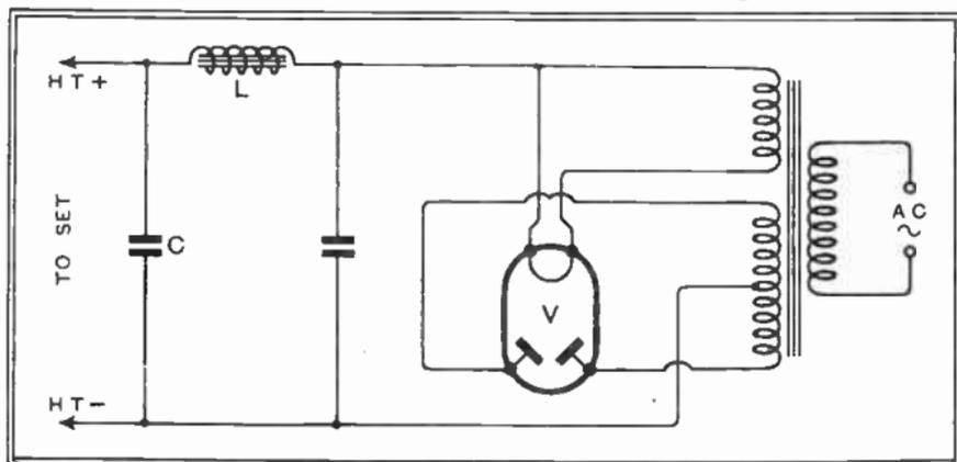
Fig. 157: Complete H.T. supply system for A.C. set. (Note that the set itself replaces the load resistance R of Fig. 155)
