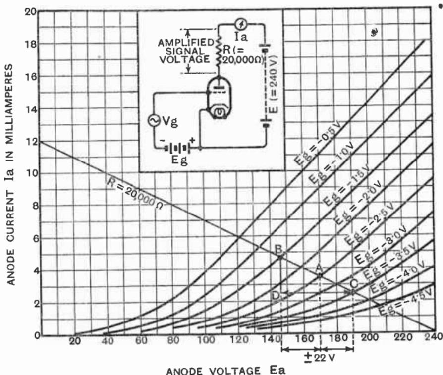
Fig 66 :  $E_a-I_a$  curves of the valve of Fig. 65. The line " $R = 20,000 \Omega$ " drawn across the curves gives, in conjunction with the curves themselves, full data as to the performance of the valve with this value of load resistance and an anode battery of 240 v.
