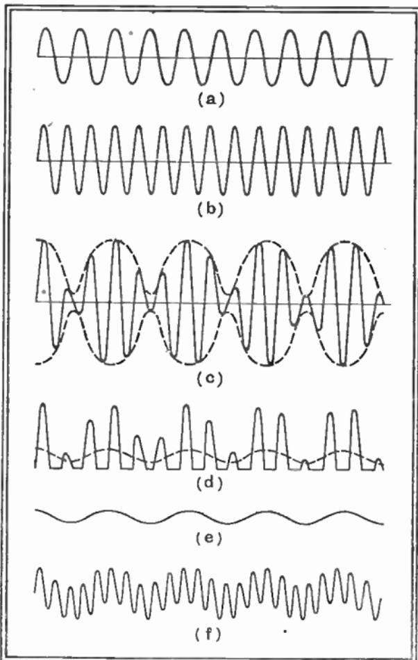
Fig. 134 : A sample of incoming carrier wave, of ten millionths of a second duration, is represented at a. To the same scale b is the local oscillator signal. When the two are added (in a "first detector") the result is c, which must be rectified (d) to yield a difference frequency (e). But if a and b are multiplied together (f), the difference frequency comes directly
