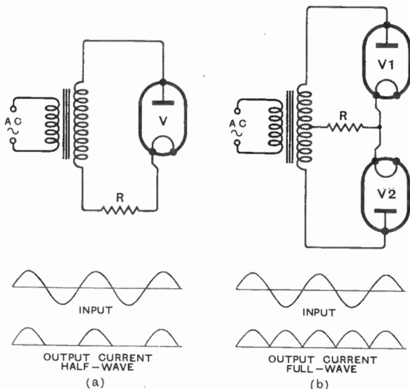
Fig. 155 : Half-wave and full-wave rectification. In *a* *V* acts literally as a valve, suppressing alternate half-waves ; in *b* there are in effect two transformer secondaries, phased so that the pulses through *V*<sub>1</sub> come between those through *V*<sub>2</sub>
