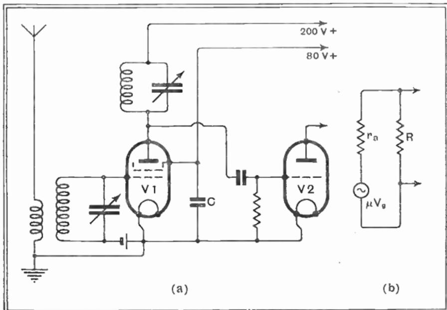
Fig. 106 a: A simple R.F. stage employing a screened valve with tuned-anode coupling; b equivalent anode circuit of the valve. If  $R$  is small compared with  $r_a$ , gain of stage is approximately  $gmR$
