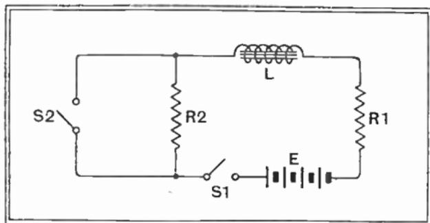
Fig. 14 : Current in inductive circuit. L, electro-magnet (inductance);  $R_1$ , represents resistance of L;  $R_2$ , high resistance switched into circuit by opening  $S_2$ ;  $S_1$ , main circuit switch
