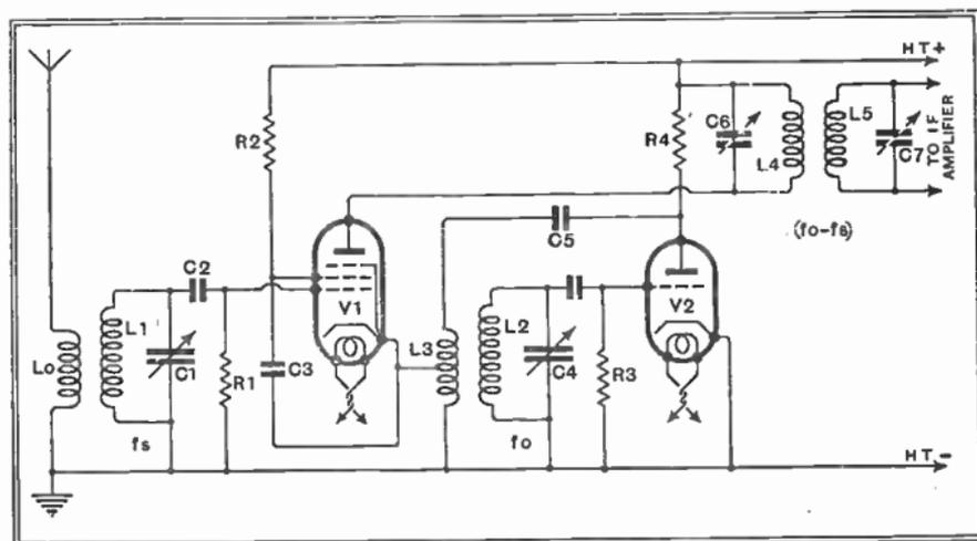
Fig. 135 : Circuit of simple two-valve frequency-changer. The signal-frequency  $f_s$  is applied to the grid of  $V_1$ , and the oscillator  $V_2$  is tuned to  $f_o$ . Currents at the intermediate frequency  $(f_o - f_s)$  appear in the anode circuit of  $V_1$
