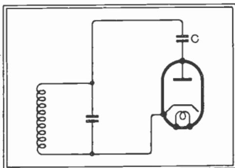
Fig. 82 : Diode detector with infinite load resistance
