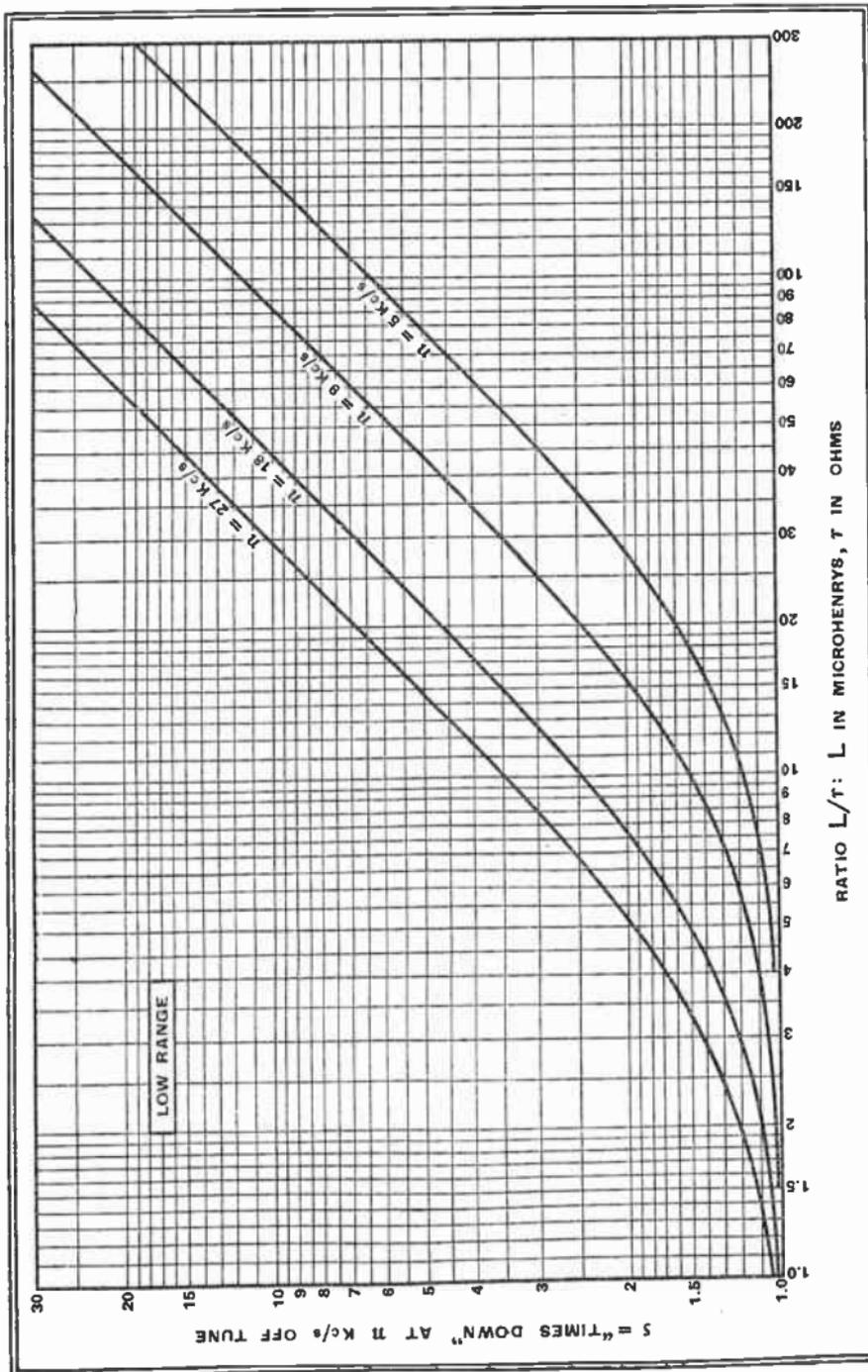
Fig. 114a : Showing relationship for one tuned circuit between  $L/r$  and  $s$  at 5, 9, 18, and 27 kc s off tune. Where value of  $s$  is greater than 10, use the continuation of these curves in Fig. 114 b
