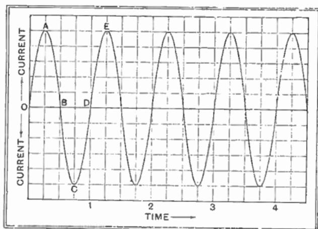
the left of the diagram, while magnitude and direction of current are shown by vertical distance from the line OBD, the height of which indicates zero current. Distance *above* the line is regarded as positive, in-
