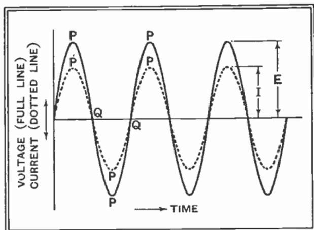
Fig. 29: Voltage and current relationships in the circuit of Fig. 28. The average power over one complete cycle is  $\frac{1}{2}EI$ , or half the power developed when  $E$  and  $I$  both have maximum values
