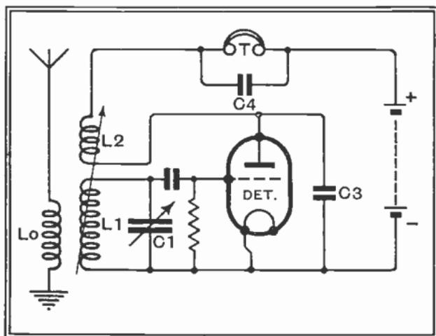
Fig. 96 : Conventional single-valve set with adjustable reaction
