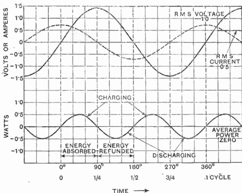
Fig. 39 : Relation of voltage, current and power in a purely capacitive circuit. Note that the average power is zero, and compare Figs. 38 and 40
