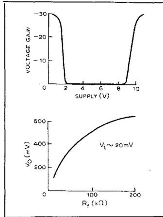
which is  $< V/2$  the supply voltage has to be  $> 8V$  in this circuit.
