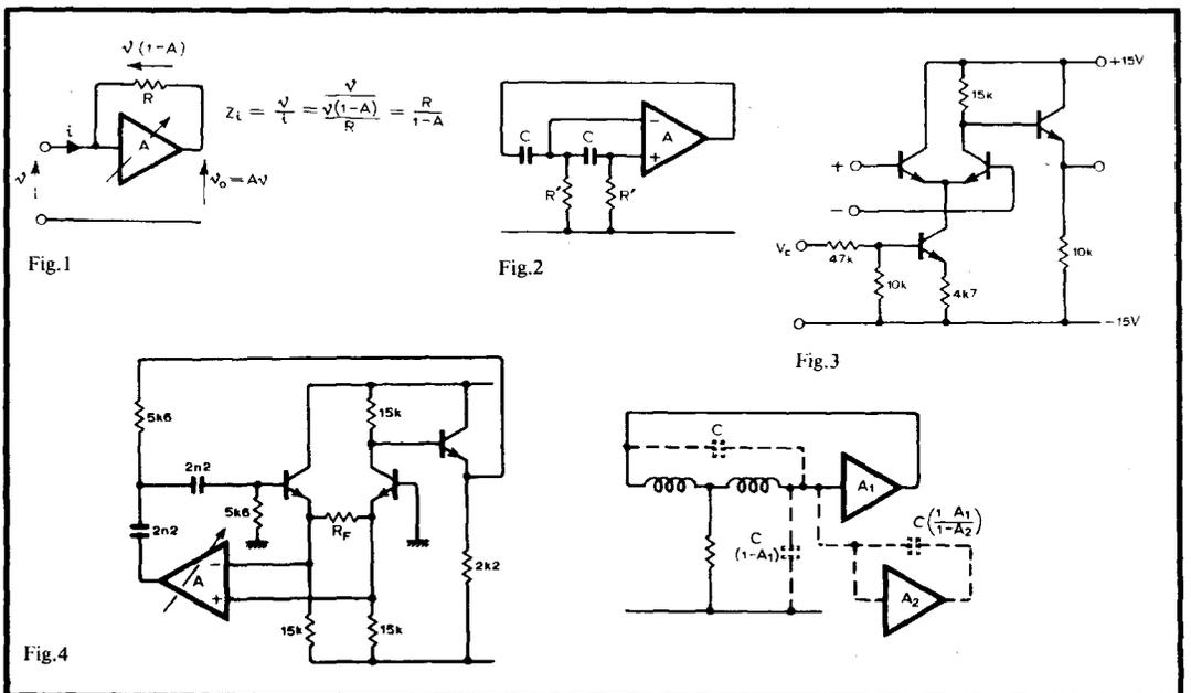
effect can be applied to LC oscillators to replace a capacitor that normally appears in a feedback path by either a grounded capacitor or one connected across a separate amplifier. If  $A_1$  is fixed to sustain oscillations, then  $A_2$  varies the effective
