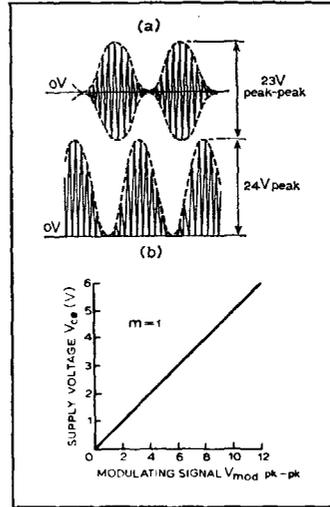
$R_E$  permits balancing of transistor characteristics to cancel carrier. Circuit right is one in which modulation is applied both to collector and emitter<sup>5</sup>.
