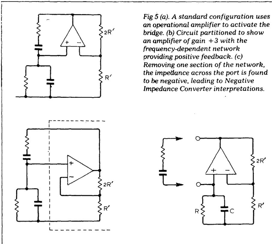
Fig 5 (a). A standard configuration uses an operational amplifier to activate the bridge. (b) Circuit partitioned to show an amplifier of gain +3 with the frequency-dependent network providing positive feedback. (c) Removing one section of the network, the impedance across the port is found to be negative, leading to Negative Impedance Converter interpretations.
