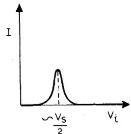
Fig. 4. Variation of inverter current with input voltage.
