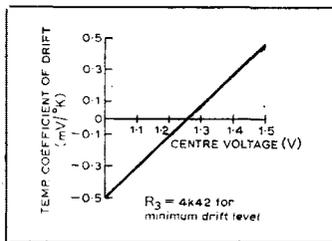
of operating from a single-ended supply and provides the facility of strobing such that a pulsed output is clamped between 0V (due to the c.m.o.s. output stage) and the temperature independent reference level. Centre voltage is the value at ambient, adjusted by R<sub>3</sub>. Temperature range imposed on transistor package was +70° to -30°. Minimum drift obtained at V<sub>out</sub> ≈ 1.25V.
