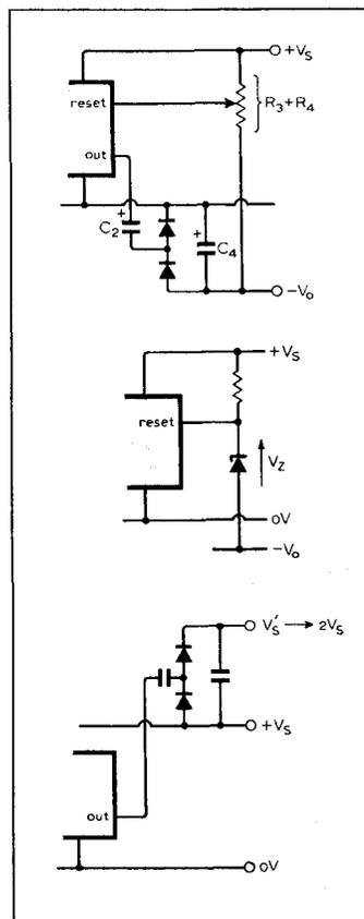
pair is significantly better than for the voltage doubler, loads down to 100Ω being tolerated
