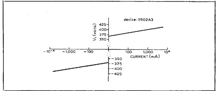
1. Asymmetric voltage dependent resistors—low voltage
