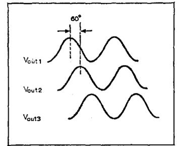
and maintaining as close a ratio as possible between the R values. Frequency is approximately 1/3RC. Note that with the CR values necessary for 60° phase shift at a specific frequency, the output of each buffer stage is attenuated by about one half and hence the minimum gain of each stage must be > 2.
