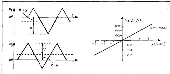
inverted sum of e<sub>1</sub>, e<sub>2</sub> and y. With x and y both at 1V and varying the frequency of the triangular wave the output accuracy was maintained within 1% up to 6kHz. The device is a 4-quadrant multiplier.
