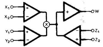
circuit design. To avoid the inconvenience of the scaling factor when devising new configurations it is helpful to write the variables in normalized from  $x, y, z:$
