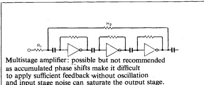
Multistage amplifier: possible but not recommended as accumulated phase shifts make it difficult to apply sufficient feedback without oscillation and input stage noise can saturate the output stage.
