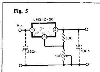
on the internal resistor  $R_1$ . LM109/309 are earlier versions on the same principle, but designed specifically for +5V logic levels. Fig. 5 is an adjustable output circuit. Capacitors are optional depending on transient response requirement and distance from supply. Another advantage of this i.c. is the internal circuitry which provides shutdown of the regulator if the die temperature reaches 175°C, thus providing virtually absolute protection.
