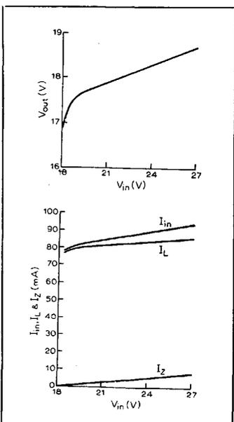
D<sub>1</sub> cathode and V<sub>OUT</sub>. Note that V<sub>OUT</sub> is now adjustable over a wide range, for a given zener voltage by choice of the ratio R<sub>2</sub>:R<sub>3</sub>.
