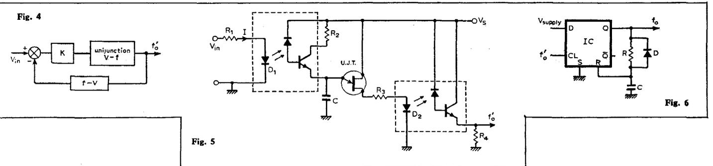
Linear voltage-to-frequency converters
