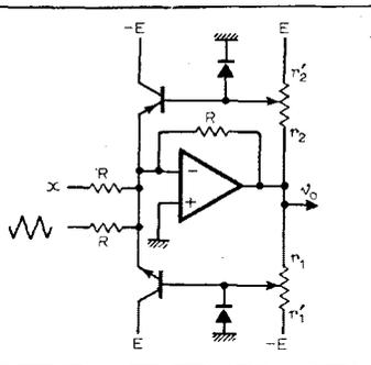
shown above; this arises from the fact that the product xy is obtained by biasing a triangular wave by x and limiting the resultant at ±y. A suitable high speed limiter is shown above. The output is limited at r<sub>1</sub>E/r' for negative inputs and at -r<sub>2</sub>E/r'<sub>2</sub> for positive inputs. These would be set to ±y respectively. Note that r<sub>1,2</sub> ≪ R for good limiting.
