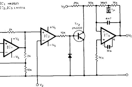
constant, then an analogue divider is implemented. Input levels should be less than  $+10V$  (all signals must be positive) and
