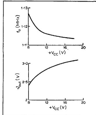
output waveform. The more the gain exceeds the critical value the more distorted will the output waveform become and the lower will be the frequency of oscillation. (See graphs for effect of increasing supply voltage, for example, after setting the critical condition at a lower value of +V<sub>CC</sub>.)
