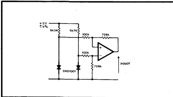
One special device that has been reported, contains a pair of silicon p-n junctions. One is so heavily doped that its band-gap voltage is reduced to that of germanium. The voltage difference is then temperature stable at around 0.41V, the difference between silicon and germanium band-gap voltages. The configuration of the circuit is not particularly novel, but the temperature coefficient is  $< 10\text{p.p.m. K}^{-1}$ , over the full military temperature range.
