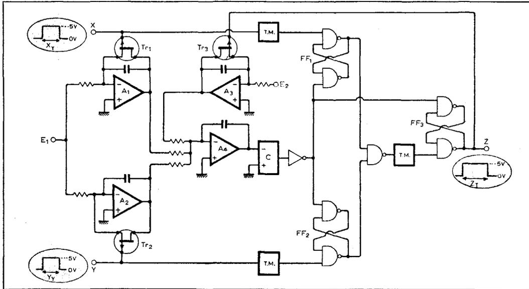
Analogue information  $x$  and  $y$  is contained in the input pulse widths  $x_T$  and  $y_T$  respectively. On the occurrence of the pulse  $x$ , the f.e.t. switch  $Tr_1$  opened and integrator  $A_1$ , fed from the d.c. signal  $E$ , ramps down and integrator  $A_4$  rises in a parabolic manner to a voltage
