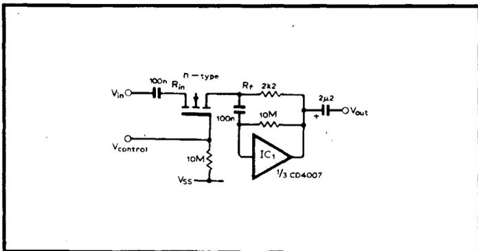
This voltage controlled amplifier is derived from a CD4007 package. IC<sub>1</sub> inverter is biased into its linear region by the 10MΩ resistor, and one of the n-type f.e.t. is used as a voltage variable resistor. Control voltage range is dependent on |V<sub>DD</sub> - V<sub>SS</sub>|. With above network gain is claimed variable from zero to just over unity.
