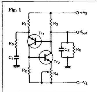
appropriate phase angle to the make the loop phase shift zero. The Fig. 1 circuit is of similar form to Fig. 2 for which an approximate analysis is given. Assume the base-emitter voltages are negligible. Then the signal  $v_{in}$  will appear as  $v_{out}$ . The input signal current  $i_{in}$  comprises  $v_{in}/R_1$  and  $i_{in} - v_{in}/R_1$  up through  $Tr_1$ . The voltage across  $R_1$  is then  $i_{in}R_1 - v_{in}$  which must be that
