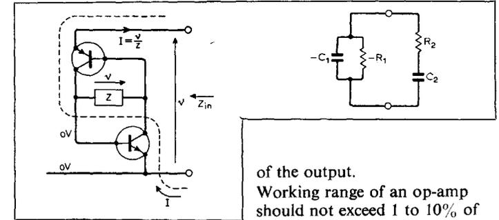
of the output. Working range of an op-amp should not exceed 1 to 10% of the unity gain frequency to avoid severe unbalance at the bridge input, i.e. at  $I_{set} = 1\mu A$ , gain-bandwidth product is 70kHz. If oscillator frequency is 700Hz, amplifier gain is 100, and hence input required is 1% of output. If set current is reduced to 0.1 $\mu A$ , then for same frequency gain is only 10. Hence for the same output greater unbalance required at the input.
