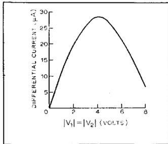
within ±0.4% full-scale. Over the range of control voltages used above (V<sub>1</sub>=V<sub>2</sub>=0 to 10V) the differential current is acceptably sinusoidal over half the range.
