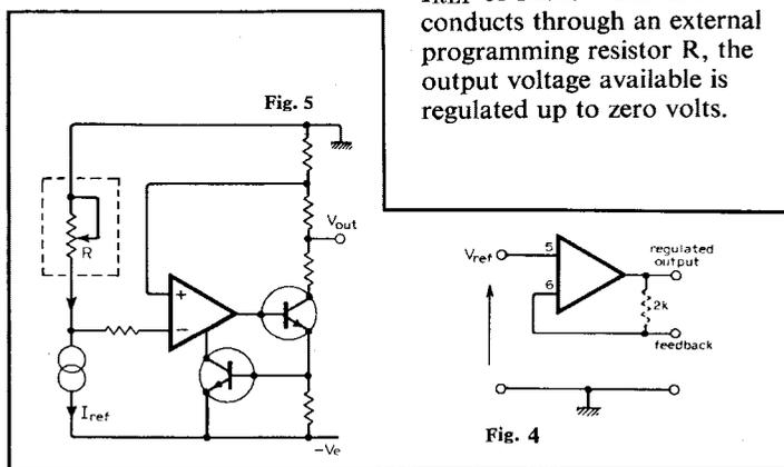
resistor provides a current  $I_{REF}$  of 1mA. When this conducts through an external programming resistor  $R$ , the output voltage available is regulated up to zero volts.
