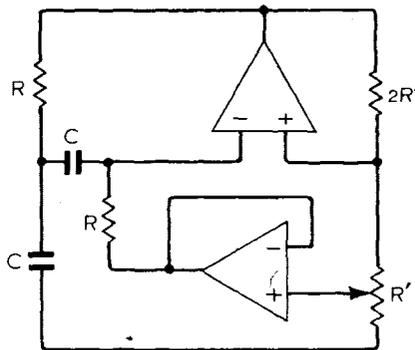
Fig. 6. Adding another amplifier at appropriate points in various oscillators allows a single control to change the frequency without varying loop gain.
