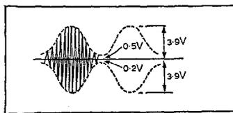
Also, since  $i_d = g_{DS} v_{mod}$  and  $i_c = \alpha(I_E + i_d)$  then  $v_o = V_{CC} - \alpha I_E R_L - \alpha g_{DS} R_L v_{carrier}$ . This provides, an a.c. product of  $2\alpha R_L I_{DSS} / V_P^2 \times (v_{carrier}) (v_{mod})$ . Similar limitations to levels apply in this circuit ( $\alpha$  common base current gain).
