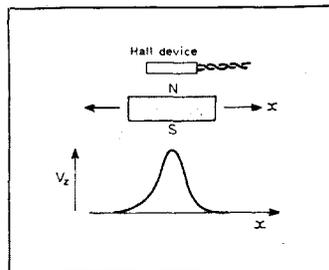
between the device and a stationary magnetic field. Displacement laterally between the magnets will produce an output voltage when the device is moved from the mid-position. An alternative arrangement will provide a linear output proportional to the displacement direction shown. In this case the magnetic field strength varies along a central plane.
