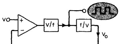
Fig. 8. In this "charge-dispersing" system, a constant amount of charge for each output pulse is fed back so that pulse rate can be proportional to the control signal.
