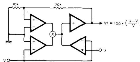
An even simpler configuration has, in normalized form,
