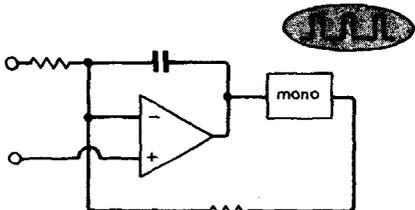
Fig. 10. An alternative arrangement is to dispense charge into a summing integrator. Output pulse rate is a linear function of control voltage or current.
