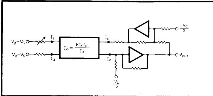
The analogue multiplier/divider is assumed to have a characteristic given by  $I_0 = K I_1 I_2 / I_3$  where  $I_1, I_2, I_3$  are input currents,  $I_0$  is the output current and where  $K$  is a parameter dependent on temperature, device ageing etc. Such a circuit is suitable as a precision modulator, where a product term should be generated to an accuracy of
