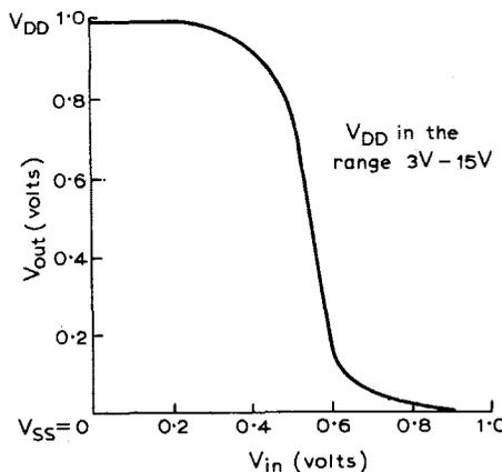
Fig. 3. Transfer function of c.m.o.s. inverter.
