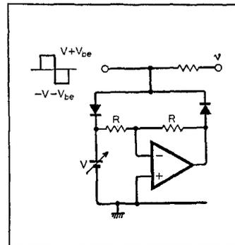
sinusoidal negative feedback and limited positive feedback can be obtained as shown above. It can be shown<sup>1</sup> that for this circuit the output is given by  $2qE\sqrt{2}/\pi$  volts r.m.s. A possible voltage-controlled limiter is shown above
