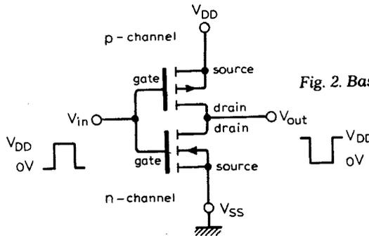
Fig. 2. Basic c.m.o.s. inverter.
