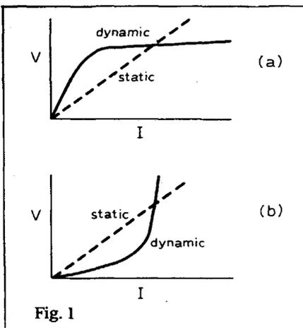
Zener breakdown is a field effect which dominates for heavily-doped narrow junctions, where even small p.d.s of three or four volts can provide a sufficiently intense field for the direct production of hole-electron pairs. The observed characteristics are that the current increases steadily as the operating region is approached, with a rounded knee, and with a temperature
