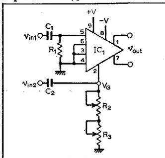
V<sub>out</sub> (pin 1 or 7) 800mV pk-pk unmodulated, see waveform opposite.
