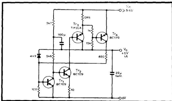
As the performance/cost ratio of integrated-circuit voltage regulators continues to improve it is tempting to ignore discrete-component designs altogether. This is dangerous because the constraints of i.c. processing, for example absence of high performance p-n-p transistors, can bring limitations. In particular for highest efficiency the output transistor has to operate in common emitter, and if a separate power device has to be
