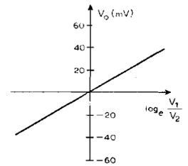
range of  $V_1$  two decades, from 0.03V to 4.0V. Linearity better than 1%.
