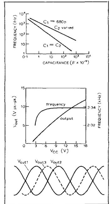
t.h.d. 1.2%. For 470kΩ, V<sub>out</sub> 4.4V pk-pk, t.h.d. 0.3%. R<sub>2</sub> 7.8MΩ V<sub>out</sub> 6.8V pk-pk, t.h.d. 0.6%. For 4.7MΩ, V<sub>out</sub> 4.1V pk-pk, t.h.d. 0.2%. For all above alterations, frequency does not change more than 0.2%. Variation with supply C<sub>1</sub>, C<sub>2</sub> shown on graphs.
