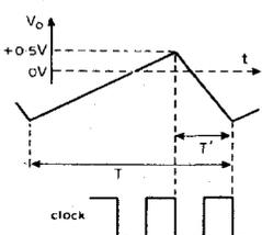
Clearly in a complete period T the charge put in by V<sub>2</sub> is cancelled by the charge withdrawn by V<sub>1</sub> as the starting and finishing voltages are the same.
