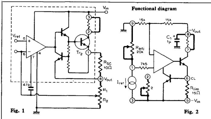
The schematic diagram of the LM105/205/305 group is within the dashed box. External components provide a basic low current positive regulator circuit.
