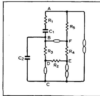
since  $f \propto 1/\sqrt{R_3}$ . Typically  $R_3$  may range from 100 $\Omega$  to >1M $\Omega$ .
