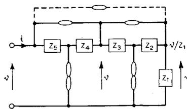
produce sustained oscillation. For  $Z_1 = Z_2 = Z_3 = Z_5 = R$  and  $Z_4 = 1/j\omega C$ ,  $Z_1 = j\omega CR^2$ .
