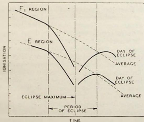
Fig. 7 : Effect of an eclipse of the sun on the ionisation of the F<sub>1</sub> and E layer
