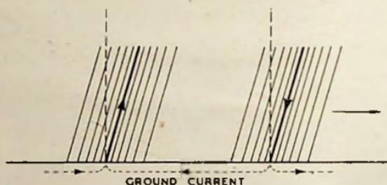
Fig. 4 : Showing forward tilt in the ground wave front
