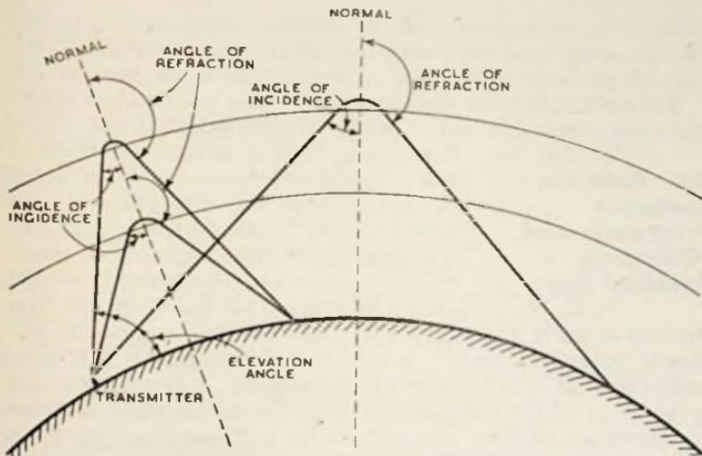
Fig. 20 : Showing how the angle of incidence varies with transmission distance and with layer height
