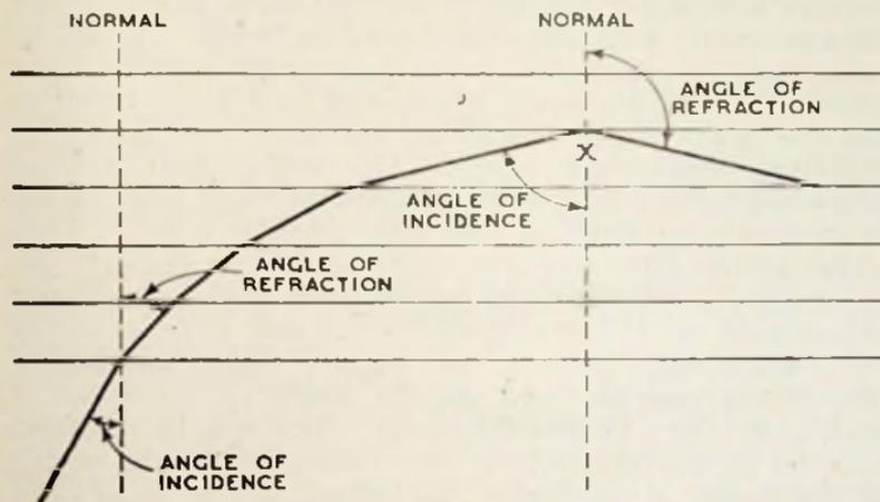
Fig. 22 : Showing successive refractions at imaginary thin layers of constant electronic density, each layer having greater electronic density than that next below it
