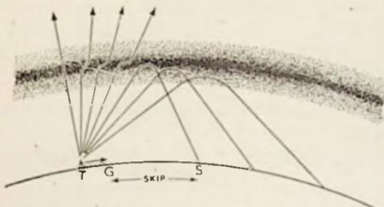
Fig. 24 : Showing the reason for the existence of a skip zone
