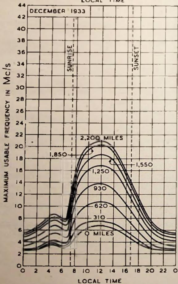
Fig. 23 : MUF's for various distances, obtained by the use of
