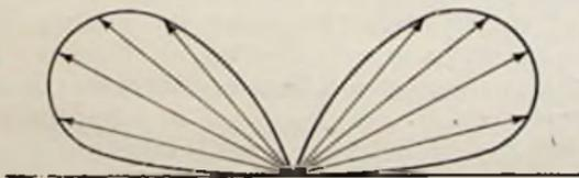
Fig. 21 : Section of radiated energy when using aerial directive in the vertical plane
