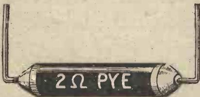
*Pye grid leaks are fitted with stout wires which are very useful when soldering the leak in position.*
