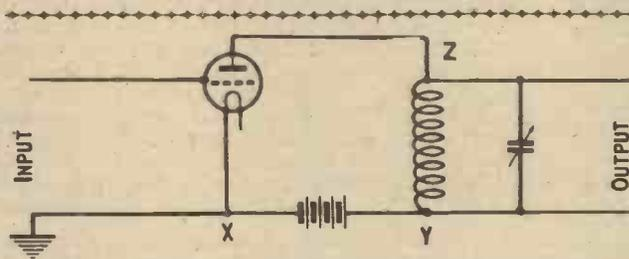
Fig. 1.—The simplest form of tuned-anode circuit.
