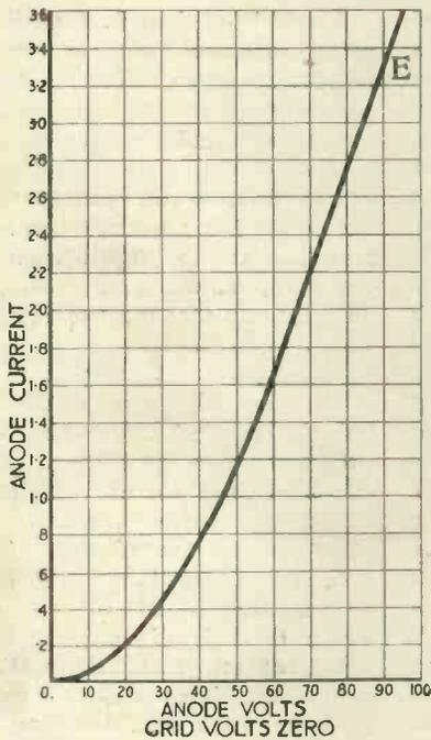
Fig. 5.—Showing the characteristic curve for a P.1 valve.
