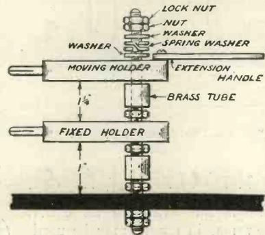
Fig. 9.—The arrangement of spindle.
