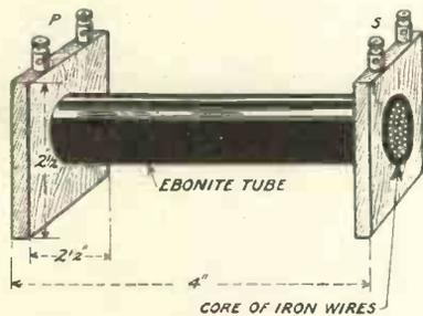
Fig. 1.—The bobbin and core of the transformer.
