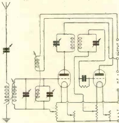
Fig. 7.—One of the most successful circuits for reducing interference.
