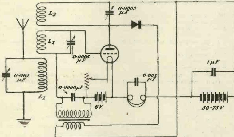
A modified arrangement of the circuit appearing in "Modern Wireless" No. 2, page 88, Fig. 4.
