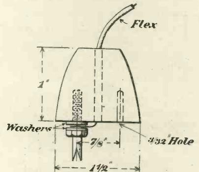
Fig. 8.—Details for contact pin.
