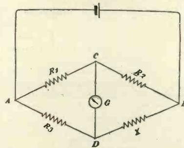
Fig. 3.—Wheatstone's bridge for accurate determination of resistance.
