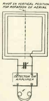
Fig. 3.—Frame arranged for rotation about vertical axis
