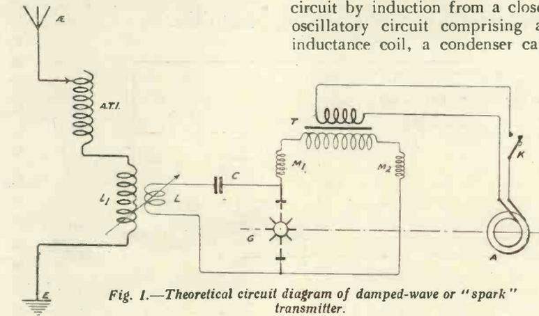
Fig. 1.—Theoretical circuit diagram of damped-wave or "spark" transmitter.
