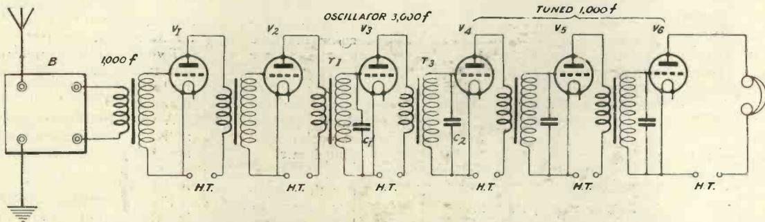
Illustrating the principle of the eliminating circuit; B being the usual receiving apparatus.
