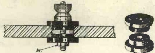
Fig. 3.—Ebonite bushes for insulating terminals fitted to wood panels.
