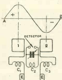
Fig. 4.—Principle of the Weagant arrangement.
