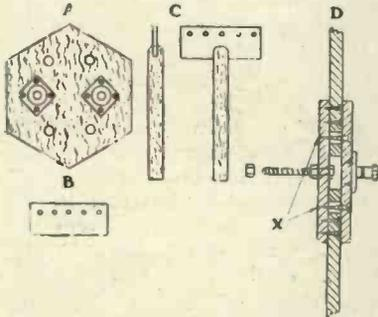
Fig. 3.—Parts required for constructing frame aerial.
