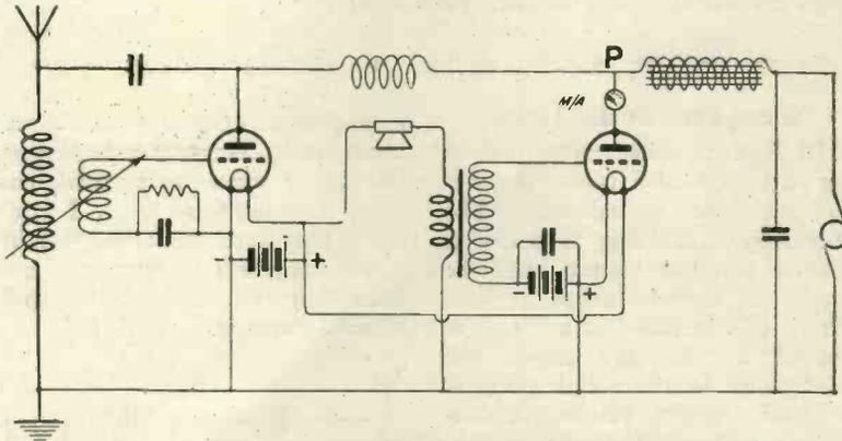
Fig. 3.—Showing arrangement of circuit for choke control.
