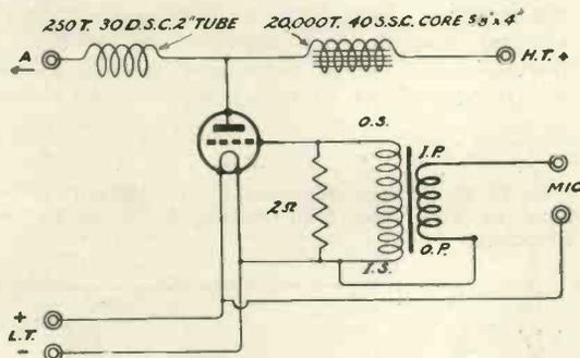
Microphone transformer: core  $\frac{1}{2}$  in. diameter  $\times$  4 in. iron wire.
