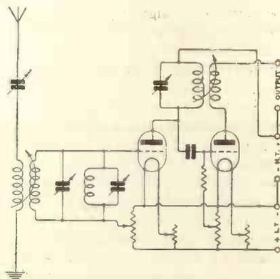
Fig. 8.—Circuit with retractor arrangement.
