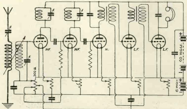
Fig. 2.—One method of using the three-slider potentiometer.
