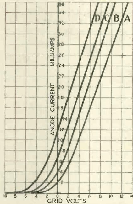
Fig. 6.—Curves illustrating the effects of various anode voltages with 4 volts on the filament. A, 20 volts; B, 30 volts; C, 40 volts; D, 50 volts.
