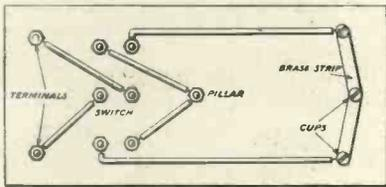
Fig. 10.—The underside of the panel.
