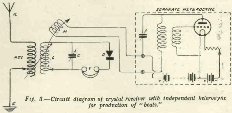
Fig. 3.—Circuit diagram of crystal receiver with independent heterodyne for production of "beats."
