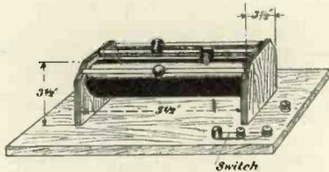
Fig. 1.—The three-slider potentiometer.
