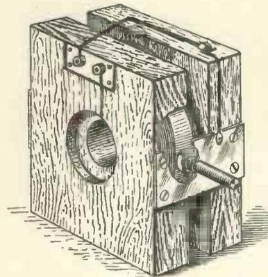
Fig. 6.—A completed variometer.
