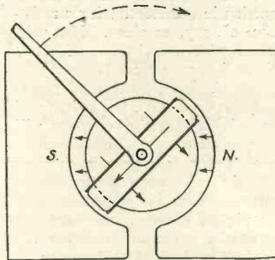
Fig. 4.—Showing the moving coil.
