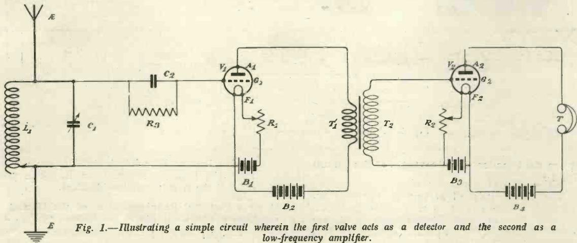
Fig. 1.—Illustrating a simple circuit wherein the first valve acts as a detector and the second as a low-frequency amplifier.
