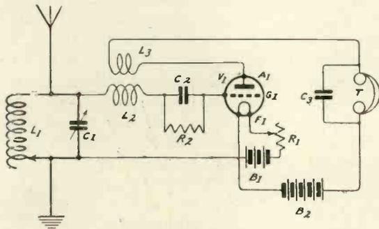
Fig. 1.—An uncommon method of reaction.
