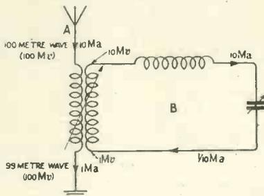
Fig. 5.—Distribution of current and potential in receiving oscillatory circuits.
