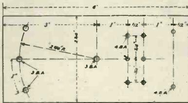
Fig. 7.—Layout of the panel.
