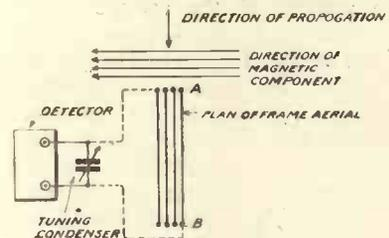
Fig. 2.—Illustrating phase-effect in a frame edge-on to advancing waves.
