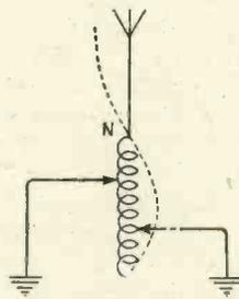
Fig. 1.—Potential nodes in aerial system.
