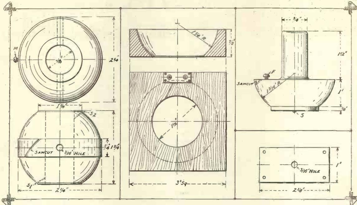
Fig. 5.—Details of the aerial variometer.
