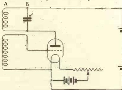
Fig. 6.—Reacting valve for reducing the effective resistance of the grid circuit.
