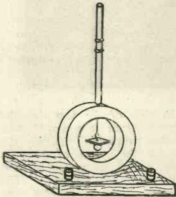
Fig. 1.—Illustrating principle of electromagnetic ammeters and voltmeters.
