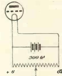
Fig. 4.—Potentiometer connections.
