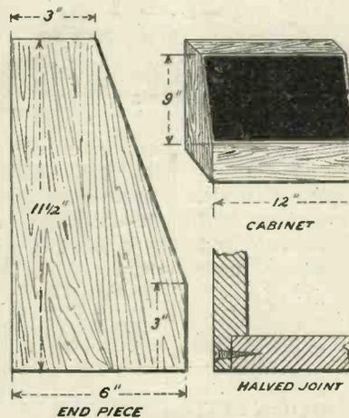
Fig. 4.—Illustrating the different sections of the cabinet.
