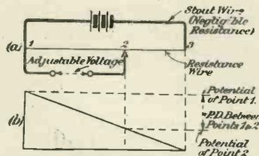
Fig. 1.—(A) Arrangement of potentiometer. (B) Graphical representation of uniform potential-gradient along potentiometer wire.
