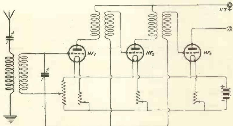
Fig. 5.—Arrangement of the potentiometer in circuit.
