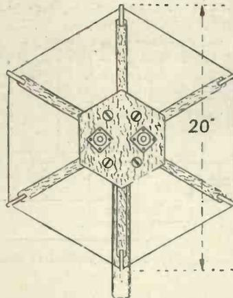
Fig. 4.—Illustrating the position of the arms.
