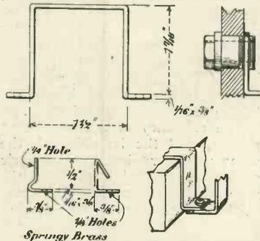
Fig. 4.—Giving dimensions of clips for holding the grid cells.
