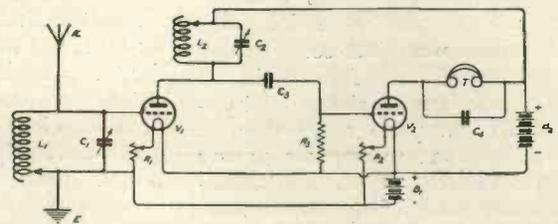
Fig. 4.—The circuit shown in Fig. 3, but using single L.T. and H.T. batteries.
