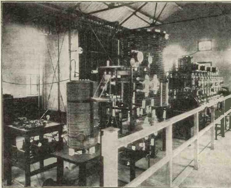
*Continuous wave transmitter, showing, from left to right: (1) high-speed signalling relays; (2) independent drive; (3) rectifier and oscillator valve panel.*
