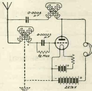
We give above a novel circuit for which good results are claimed in America. If an earth connection is used with the aerial it should be connected as indi-
