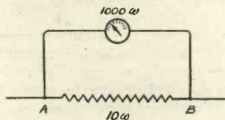
Fig. 5.—The voltmeter circuit must not take sufficient current to upset the circuit conditions.
