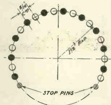
Fig. 11.—Suggested method for fitting studs.
