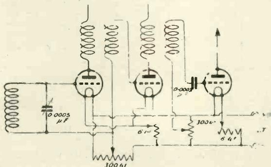
(1) The aerial circuit condenser is there for the purpose of controlling the wavelength of the receiver. (2) There is no definite ratio between the sizes of the coils you mention; it is more a matter of experiment than anything else. (3) The potentiometer should control the high-frequency valves alone, but under certain circumstances an additional potentiometer is useful to control the grid of the rectifying valve. See Fig. above.
