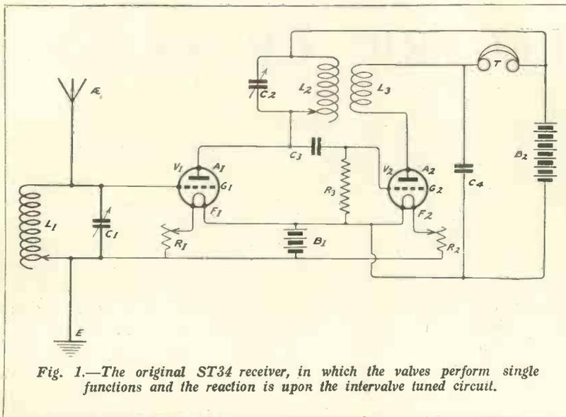
Fig. 1.—The original ST34 receiver, in which the valves perform single functions and the reaction is upon the intervalve tuned circuit.
