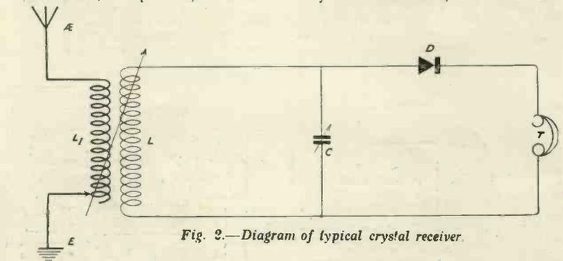
Fig. 2.—Diagram of typical crystal receiver.
