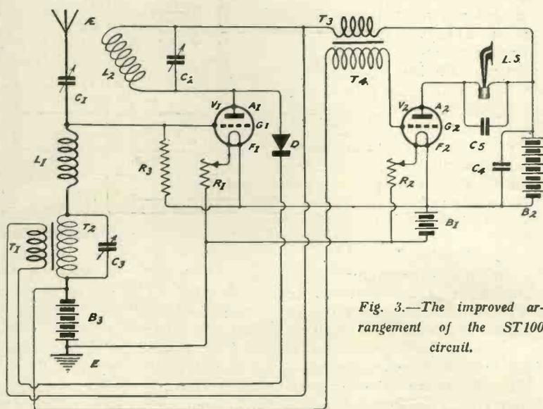
Fig. 3.—The improved arrangement of the ST100 circuit.
