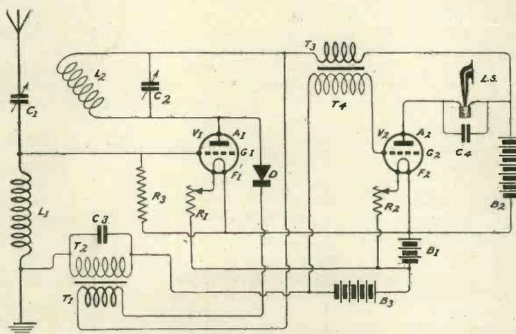
Fig. 1.—The original ST100 circuit with grid cells added at  $B_3$ .
