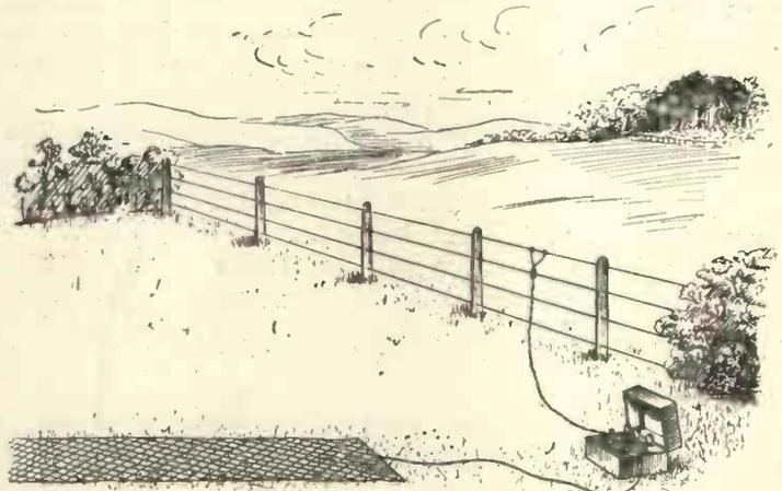
Fig. 2.—Using a fence as an aerial.
