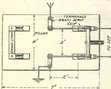
Fig. 6.—A double-pole earthing switch.
