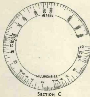
With these charts, which may be cut, pasted on cardboard and assembled, it becomes easy to find the dimensions of a coil for a given wavelength or inversely find up to what wavelength a coil and condenser will tune. Other operations are also possible.
