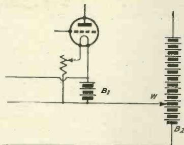
Fig. 2.—Method showing how the H.T. battery may be used for providing negative potential to the grid.
