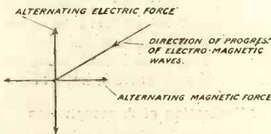
Fig. 1.—Perspective view, showing the direction of the components in electro-magnetic waves.
