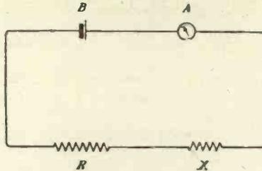
Fig. 2.—Rough method of measuring a resistance.
