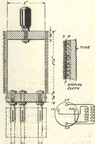
Fig. 8.—Details of the H.F. transformers.
