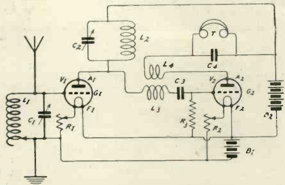
Fig. 2.—The same method of reaction applied to a high-frequency valve.
