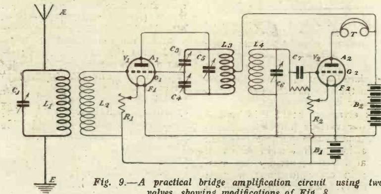
Fig. 9.—A practical bridge amplification circuit using two valves, showing modifications of Fig. 8.
