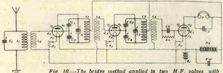
Fig. 10.—The bridge method applied to two H.F. valves with a third, acting as a detector.
