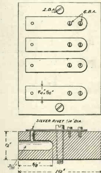
Fig. 6.—Plug block for H.T. and L.T. connections.
