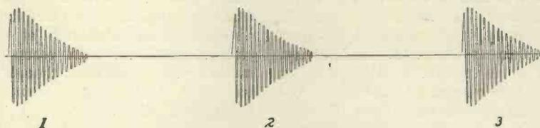
Fig. 3.—Groups of damped oscillations.
