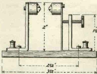
Fig. 5.—The detector assembled for use.
