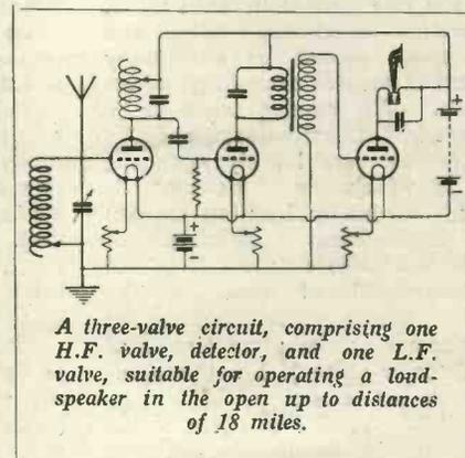
A three-valve circuit, comprising one H.F. valve, detector, and one L.F. valve, suitable for operating a loud-speaker in the open up to distances of 18 miles.
