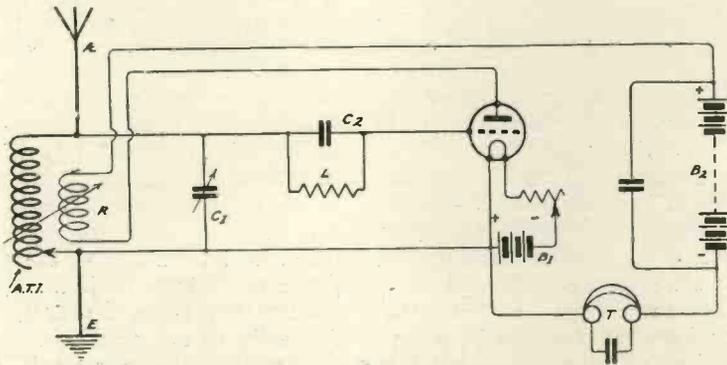
Fig. 4.—Circuit diagram of modern self-oscillating valve receiver.
