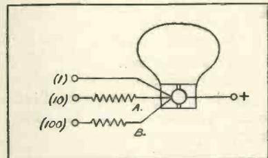
Fig. 7.—The principle of Fig. 6 incorporated in voltmeter instrument.
