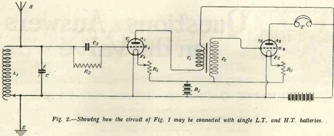
Fig. 2.—Showing how the circuit of Fig. 1 may be connected with single L.T. and H.T. batteries.
