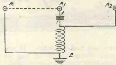
Fig. 5.—The suggested arrangement for series-parallel capacity switching.
