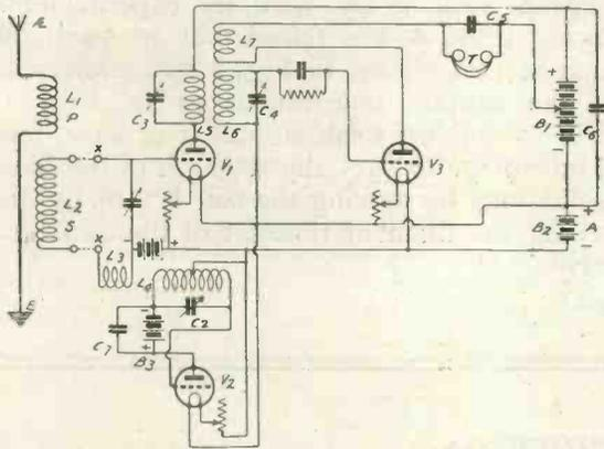
Fig. 1.—Three-valve Super-Heterodyne circuit.
