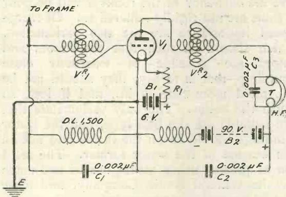
Fig. 1.—The Circuit "A," a modification of the original Armstrong Super.
