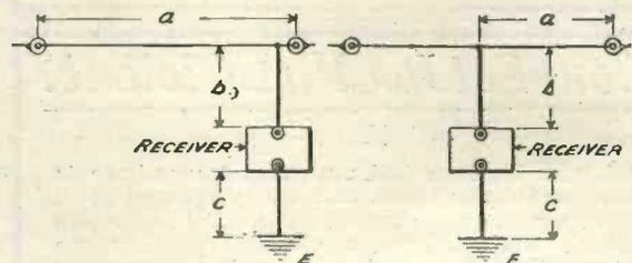
+c), the length "a" being that of the horizontal part of the aerial. In the right-hand figure the natural wave length will be four times ( $a+b+c$ ), but note that in this case "a" represents only half of the horizontal length of the aerial.
