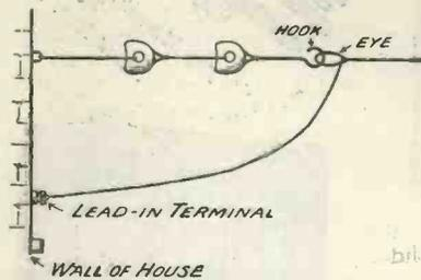
Fig. 2.—Arrangement for fixing counterpoise at house end.
