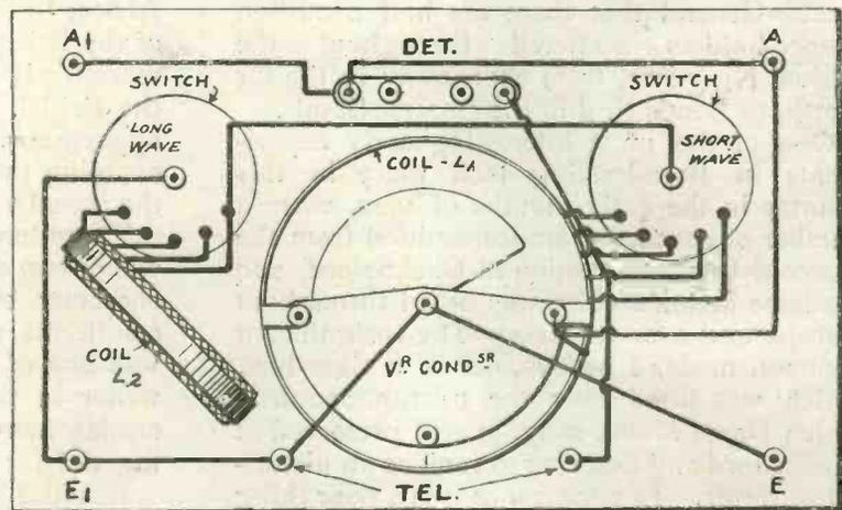
Fig. 6.—A “back-of-panel” wiring diagram.
