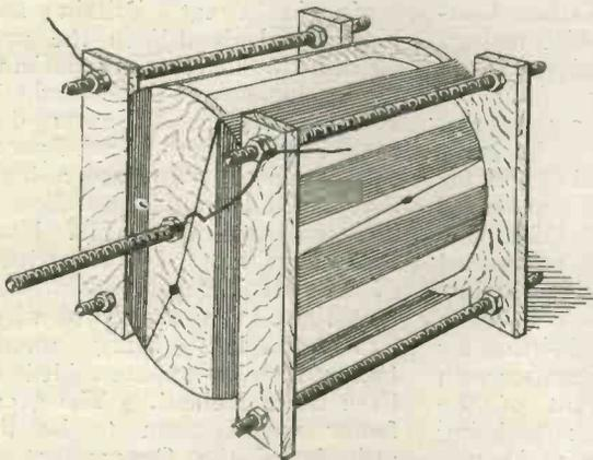
Fig. 1.—The completed variometer.
