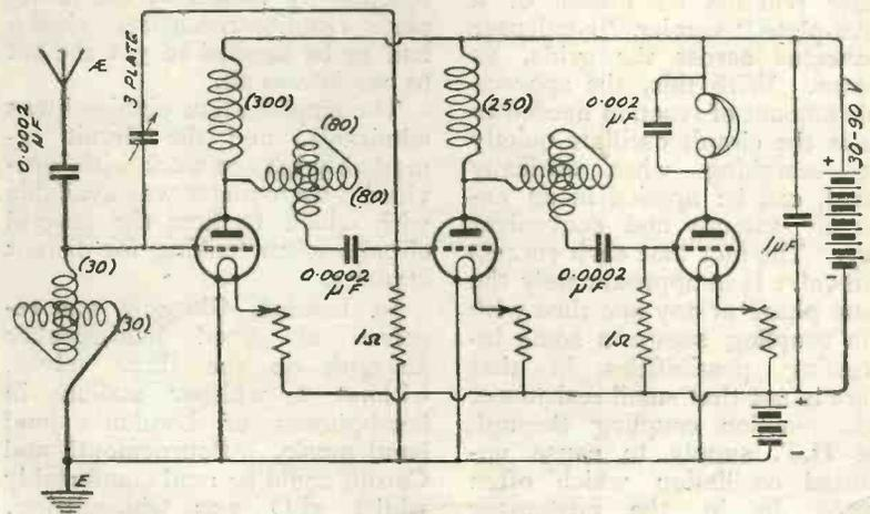
Fig. 2.—The series-tuned-anode method applied to 2 H.F. valves.
