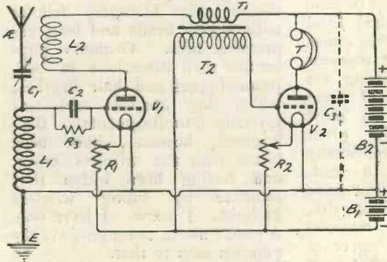
Fig. 4.—The circuit arrangement of the receiver. The condenser  $C_3$ , shown dotted and connected across the H.T. battery, may be found desirable, though the writer has omitted it without any disadvantage. When used this condenser should be of not less than 0.02  $\mu$ F.
