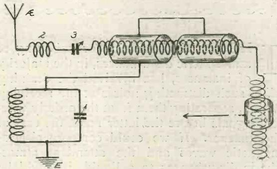
Fig. 4.—Duplicate resonance coils and guard rings may be used as shown.
