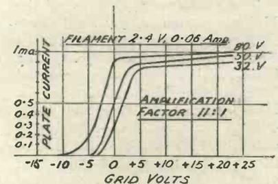
Fig. 3.—Curves obtained with the AR06 type valve.
