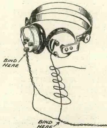
Fig. 4.—Illustrating the method of connecting the 'phones.
