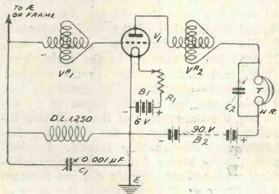
Fig. 3.—The Circuit "C," illustrating a further development.
