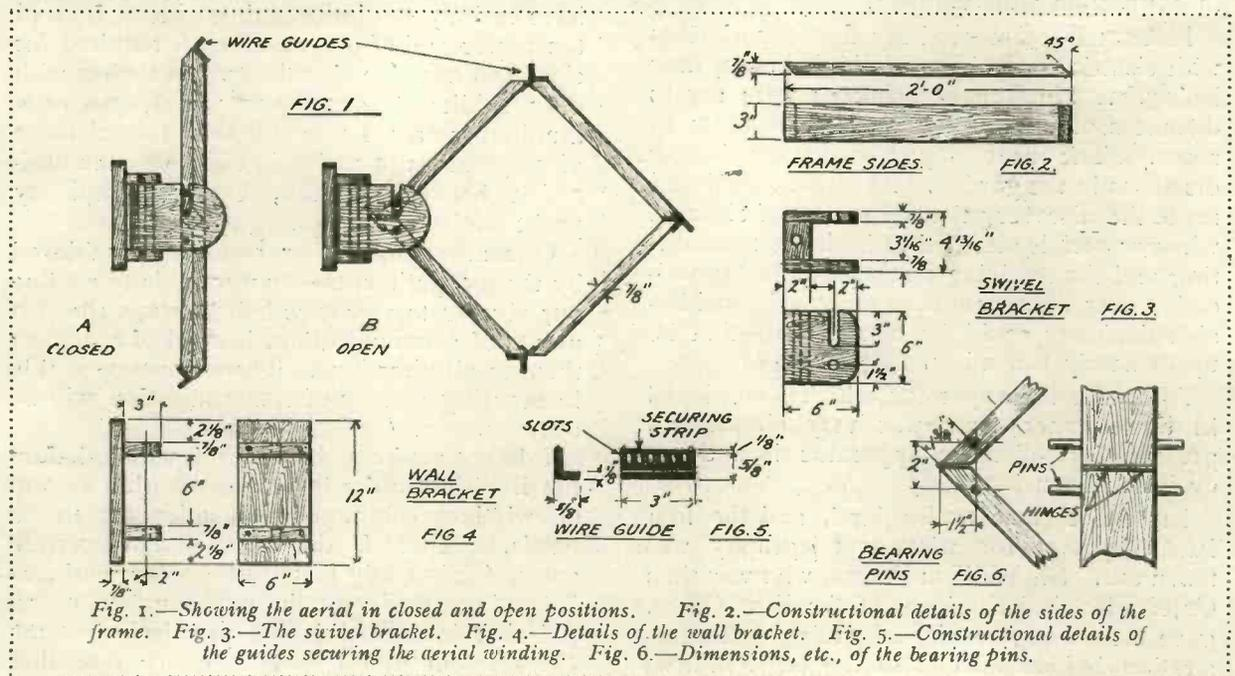
Fig. 1.—Showing the aerial in closed and open positions. Fig. 2.—Constructional details of the sides of the frame. Fig. 3.—The swivel bracket. Fig. 4.—Details of the wall bracket. Fig. 5.—Constructional details of the guides securing the aerial winding. Fig. 6.—Dimensions, etc., of the bearing pins.
