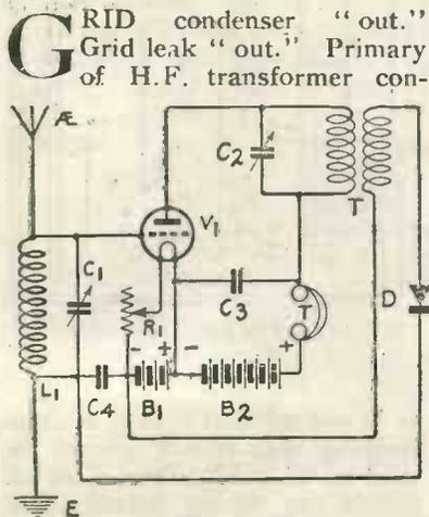
Fig. 9A.—A Simple Reflex Receiver.
