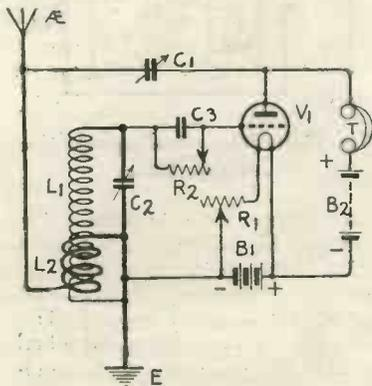
Fig. 14A.—An improved Reinartz Receiver.
