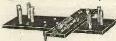
Fig. 1.—The double valve holder.
