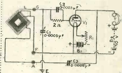
Fig. 3. The Circuit.
