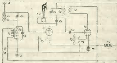
Fig. 27.—The ST75 Circuit.
