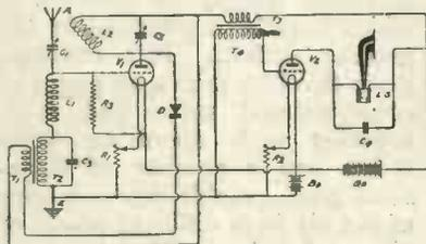
Fig. 19.—The ST100 circuit.
