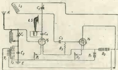
Fig. 25.—The ST150 Circuit.
