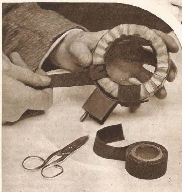
Figs. 9 and 10.—This is a good method of attachment (covered by Burndy patents) employing a binding of adhesive tape and a segment of fibre.
