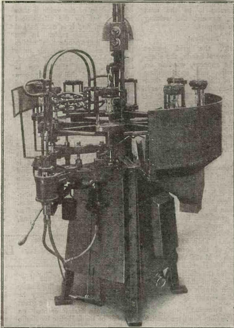
A "sealing-in" machine for small valves.
