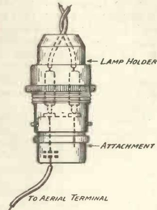
Fig. 2.—Principle of the plug-in attachment.
