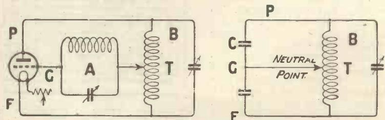
Fig. 2.—“Neutral-grid” connections.
