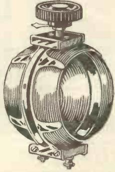
Well-known spherical type, Self-supporting winding, Aluminium skeleton frame, wound green D.C.C. wire, approx. wave-length 300-800 metres, very close coupling.
