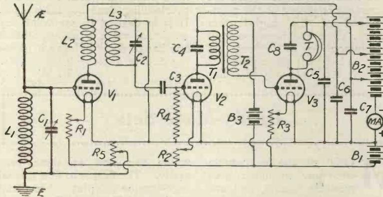
Fig. 2.—Showing position in which milliammeter should be used when employing three separate H.T. tapplings.
