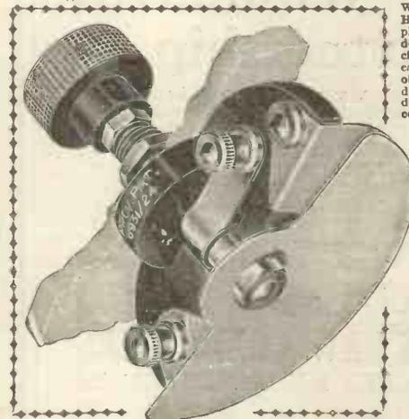
Where more than one stage of H.F. amplification is employed the necessity for the dead accurate balancing of circuits is well known. Large capacity condensers are obviously unable to tune to dead accuracy. A small condenser of very low maximum connected in parallel with the main condenser, gives just the required amount of delicate control.
