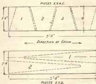
Fig. 3.—Cutting out the parts.
