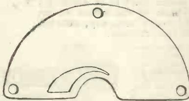
Note the novel design of the special Peto-Scott Square Law Plate (registered design No. 707587). Actual tests have proved that the Peto-Scott Square Law Condenser gives absolute straight line reading over the whole of the Dial.
