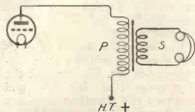
Fig. 1.—Connections of a telephone transformer.
