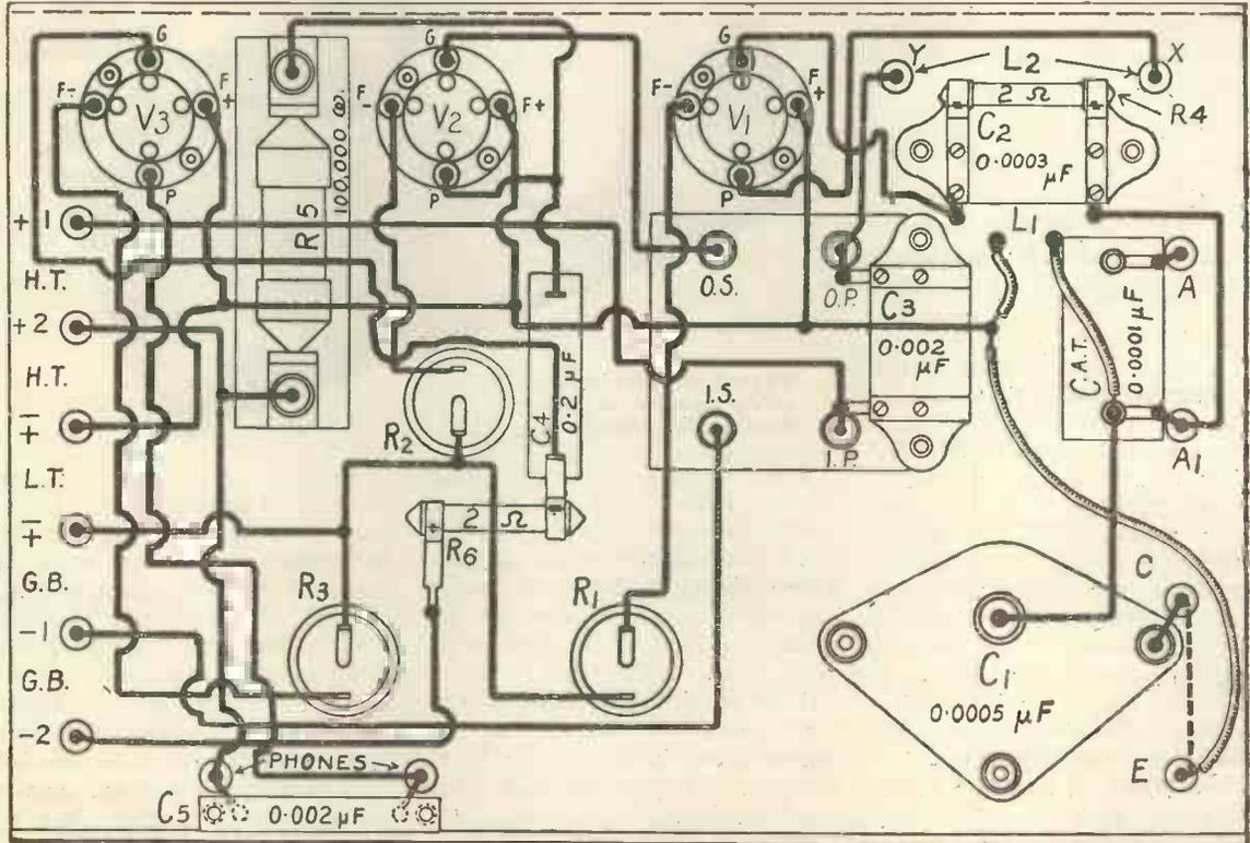
Owing to an error in the photogravure process the wiring diagram which appeared on page 25 of our photogravure supplement was shown incorrectly, the grid and anode of the second valve being joined together. The corrected diagram appears above.
