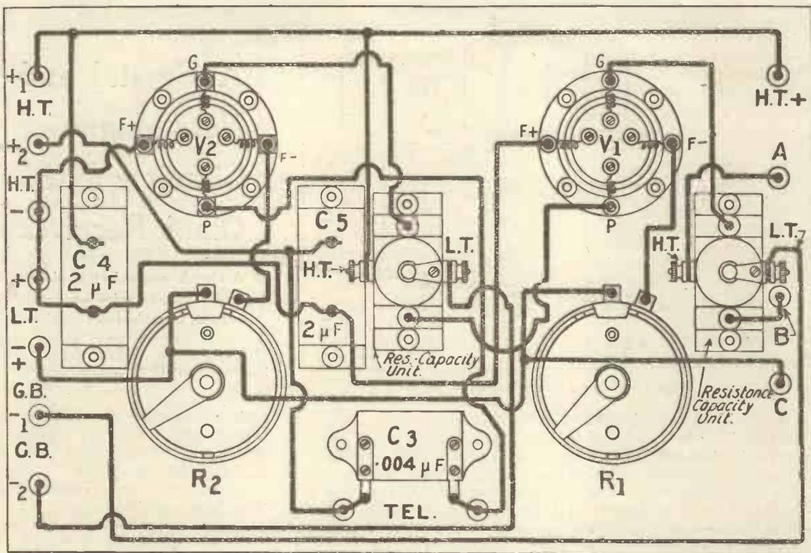
Fig. 6.—Practical wiring diagram.
