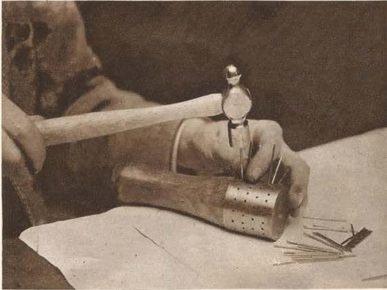
Fig. 1.—Preparing the former for use. The one illustrated is a commercial product known as the "E.C."
