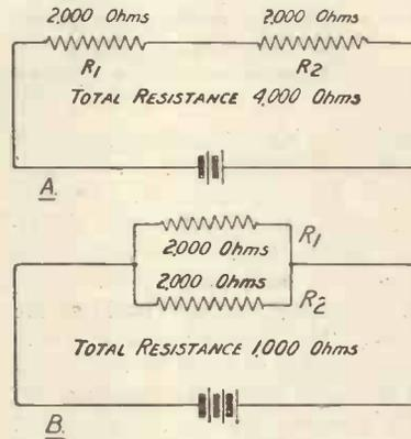
Fig. 5.—Illustrates the effect of resistances in series or parallel.
