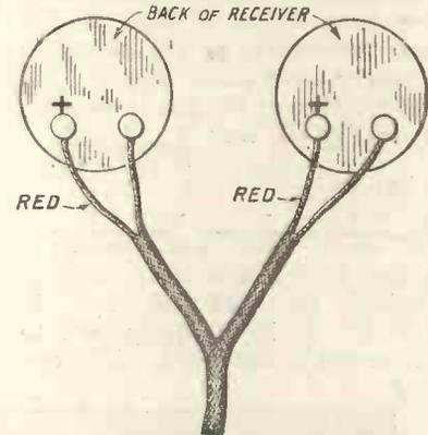
Fig. 3.—The cord lead marked red should be joined to the + terminal of the receivers.
