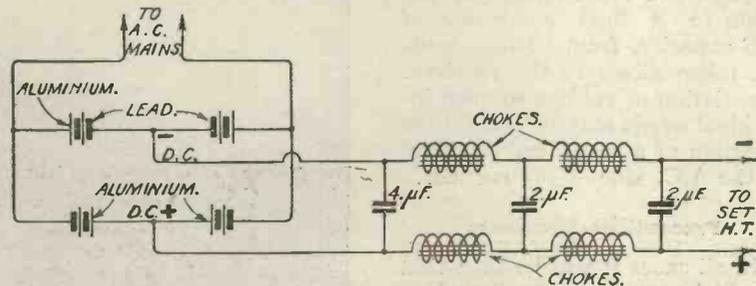
Fig. 4.—The complete arrangement of rectifier and smoothing circuit is shown here.
