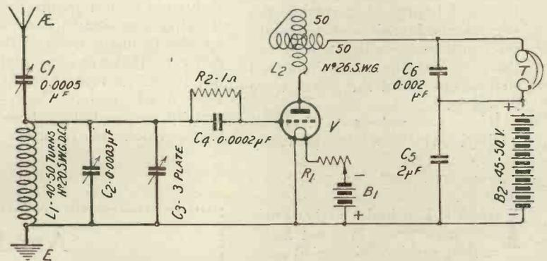
Fig. 2.—A circuit which will tune all short-wave B.B.C. stations on one inductance. The variometer may be loaded with a 0.0003 μF fixed condenser for higher ranges.
