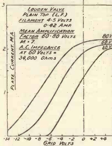
80 volts H.T. In these circumstances very good and distortionless amplification resulted, again showing appreciable gain on our standard R valve. A considerable amount of L.F. energy could be handled successfully, particularly by
