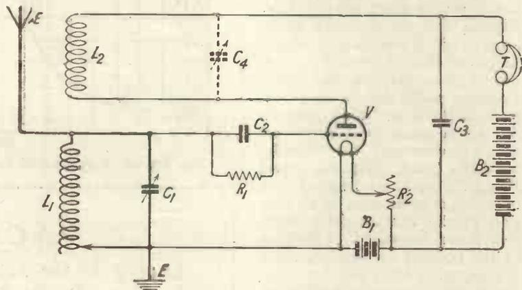
Fig. 9.—A self-heterodyne circuit.
