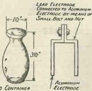
Figs. 1 and 2.—Illustrating the jar and method of connecting the electrodes.
