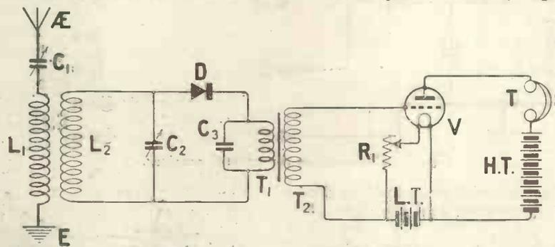
Fig. 2.—The circuit arrangements.
