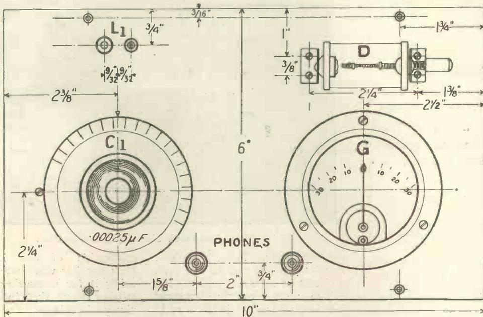
Fig. 4.—Half scale drawing of top of panel.
