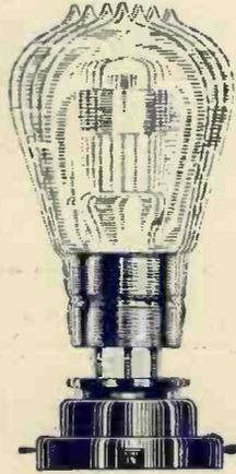
The illustration shows how a valve in the Anti-Phonic Holder vibrates when tapped. Normally, the springs in the base protect the filament from shocks.
