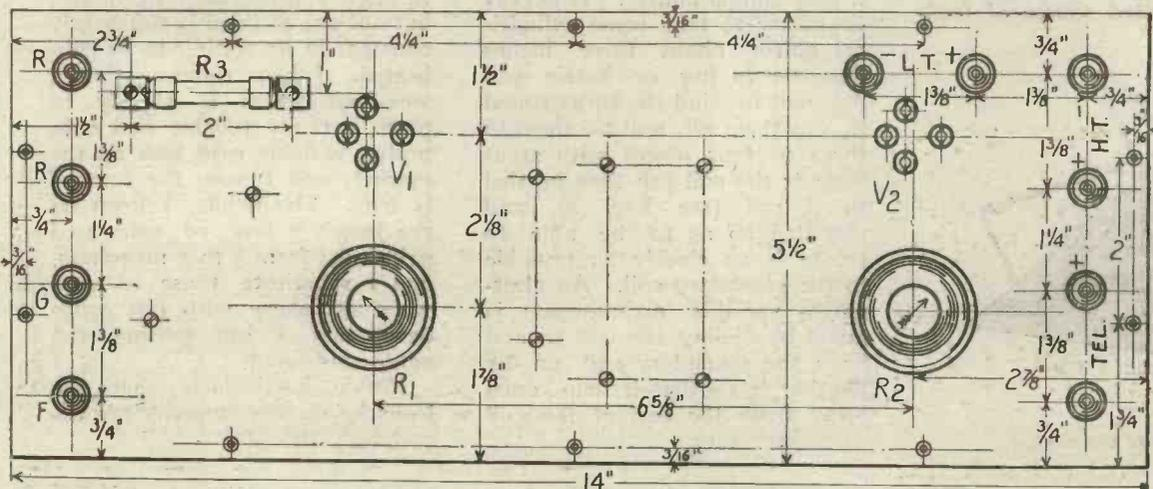
Fig. 7.—The layout of the panel and drilling dimensions.
