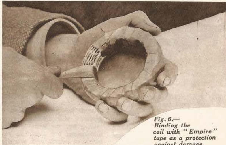
*Fig. 6.—Binding the coil with "Empire" tape as a protection against damage.*
