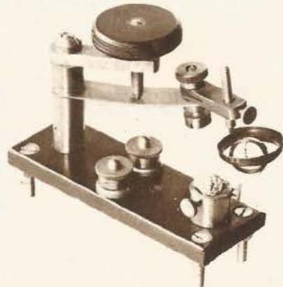
Fig. 13.—The crystal-detector stand.
