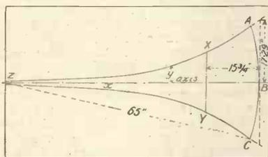
Fig. 2.—Dimensions of the horn.
