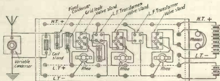
Fig. 17. A detector and two note magnifiers wired up on the layout board.
