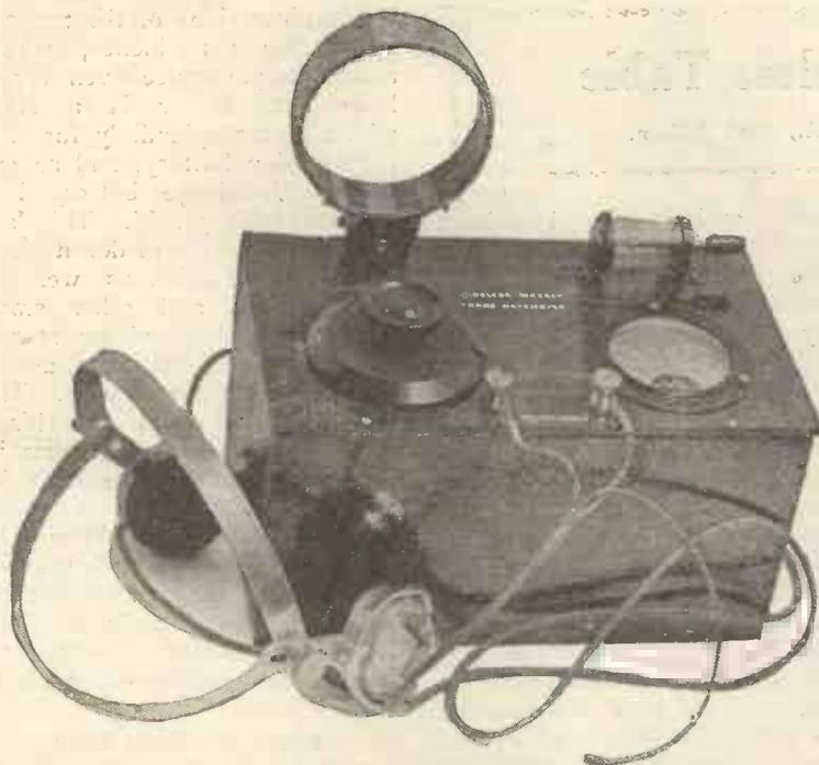
The telephones are used for calibration. Indications of resonance are visual.
