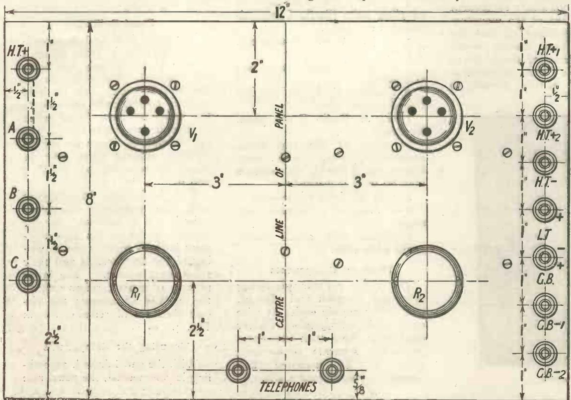
Fig. 5.—Drilling plan to half scale.
