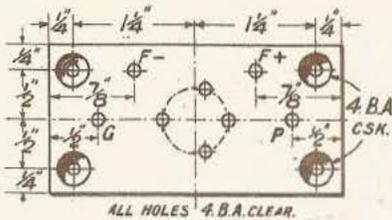
Fig. 9.—Drilling details of valve panel.
