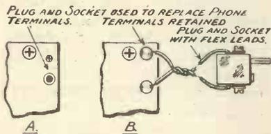
Fig. 1.—Adapting the set for plug-in leads.
