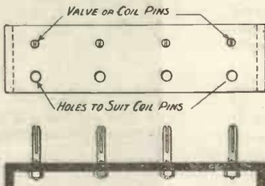
Fig. 1.—How the rack for plug-in coils is made.
