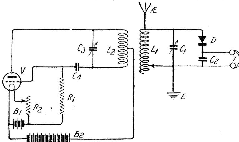
Fig. 3.—A crystal receiver using a valve oscillator to produce beats for c.w. reception.
