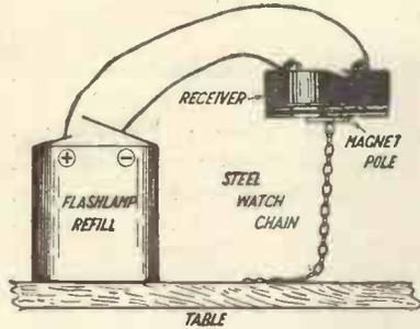
Fig. 4.—A polarity test for telephone connections.
