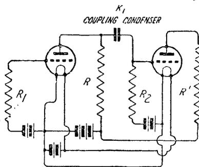
Fig. 2.—How units are coupled.
