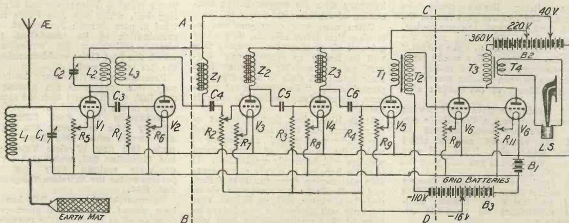
Fig. 1.—Showing the general principle of the circuit used by the B.B.C. for demonstration purposes at the exhibition.
