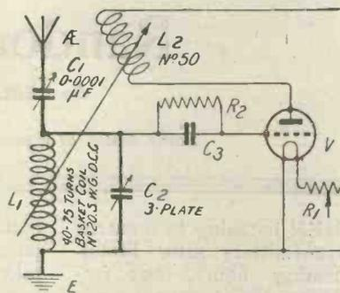
Fig. 3.—A combined series-parallel aerial tuning condenser circuit.
