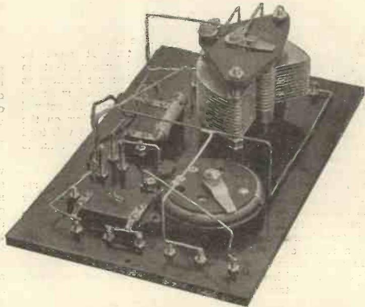
Fig. 2.—Back of panel wiring.
