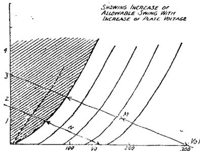
Fig. 8.—Relation of allowable swing and plate voltage.
