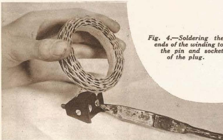
Fig. 4.—Soldering the ends of the winding to the pin and socket of the plug.
