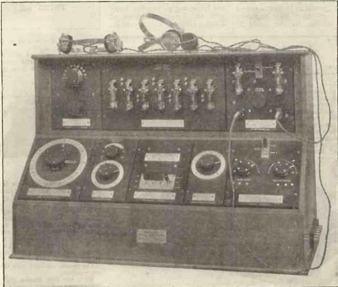
*A Marconi exhibit at Wembley. A complete D.F. equipment with a seven valve receiver incorporated in the same cabinet.*
