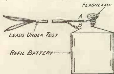
Fig. 2.—Variations of the lamp indicate the condition of the leads.
