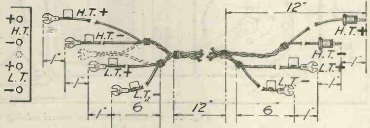
*Constructional details and dimensions of the battery connector.*
