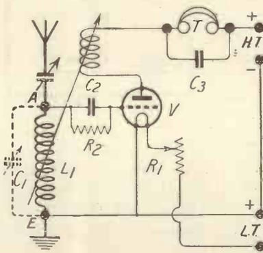
Fig. 3.—The theoretical circuit.
