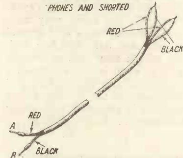
Fig. 1.—The leads arranged for a continuity test.
