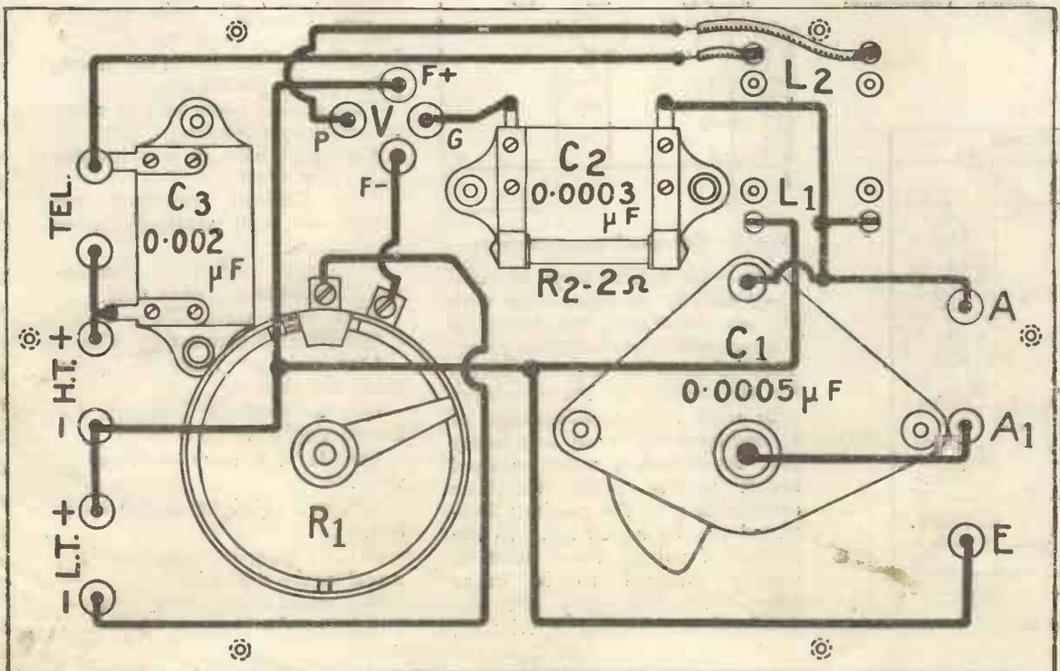
Fig. 6.—Practical wiring diagram of the instrument.
