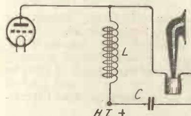
Fig. 2.—The use of a choke coil to by-pass the steady anode current.
