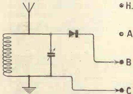
Fig. 7.—Connections for crystal receiver.
