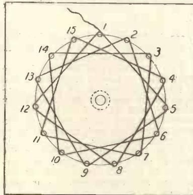
Fig. 1.—One complete "layer" of the coil.
