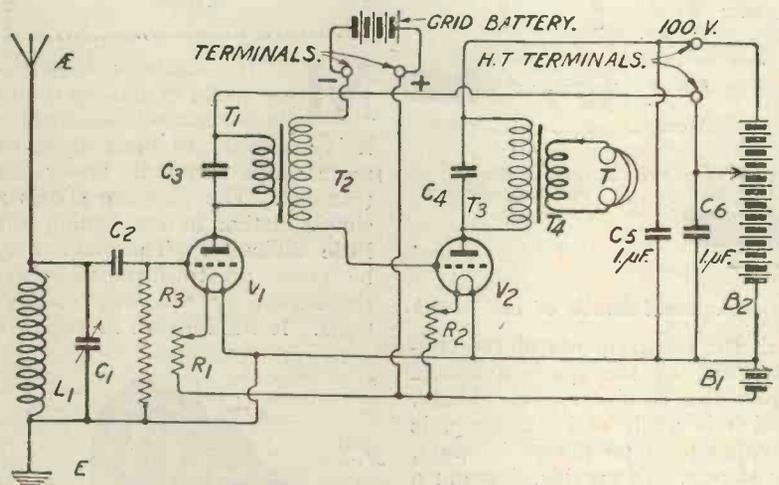
Fig. 1.—An ordinary detector and note-magnifier circuit adapted for applying negative grid bias and separate anode voltage to the last valve.
