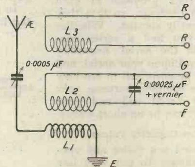
Fig. 6.—Three coil tuner for the Fig. 5 circuit.
