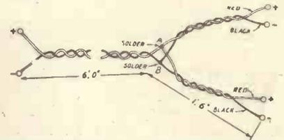
Fig. 6.—Method of connecting leads to put earpieces in parallel.
