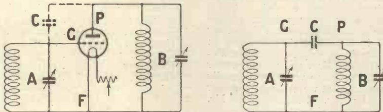
Fig. 1.—The oscillating circuit in a tuned H.F. amplifier.
