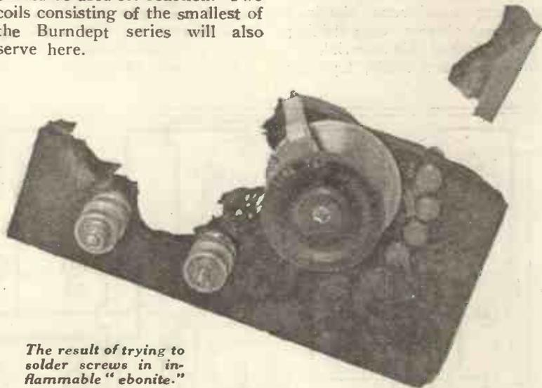
The result of trying to solder screws in inflammable "ebonite."
