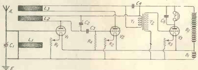
Fig. 2—A double reaction circuit for the "Omni."
