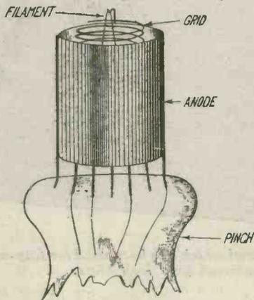
Fig. 2.—The electrodes of a power valve.
