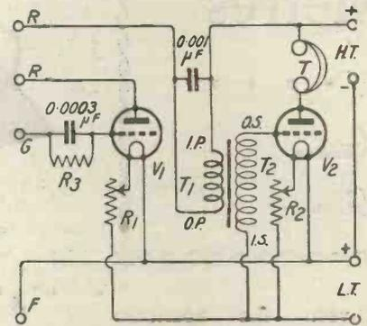
Fig. 5.—Circuit of the detector and note magnifier panel.
