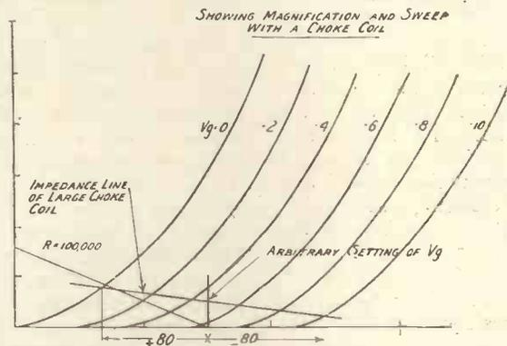
Fig. 10.—Showing magnification and sweep with a choke coil.
