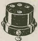
Is fixed by a single screw in centre, the holder itself acts as a jig for drilling the holes for panel wiring. For surface wiring clamp the wires under the heads of screws. Has safety insulated plate socket. (Prov. Prot'd.)
