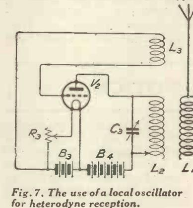
Fig. 7. The use of a local oscillator for heterodyne reception.
