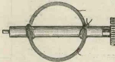
Fig. 2.—Method of securing the hank coil.
