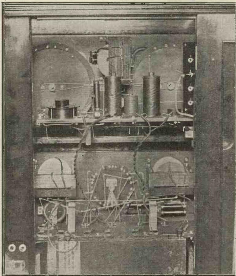
A close up of the interior of a Marconiphone four valve receiver embodying the new Marconi transformer.
