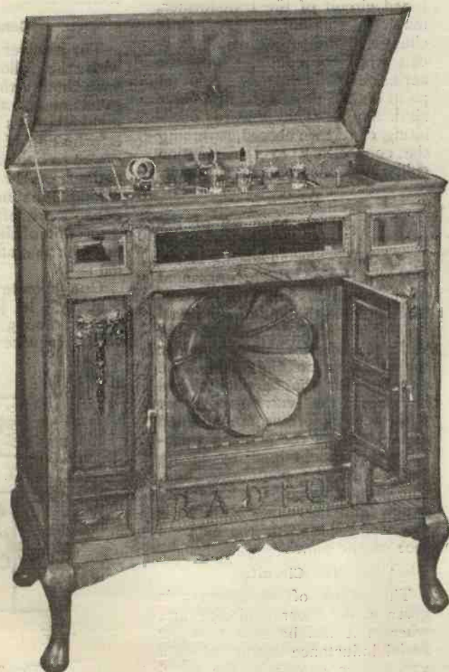
The luxurious 4-valve T.A.T. receiver, made by Mr. Lester, of which another photograph appears elsewhere.
