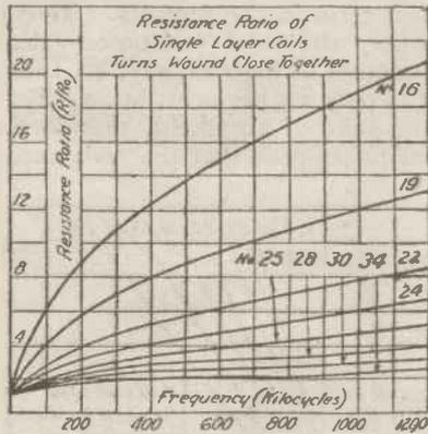
Fig. 4.—Relation of resistance ratio to frequency in single-layer coils.
