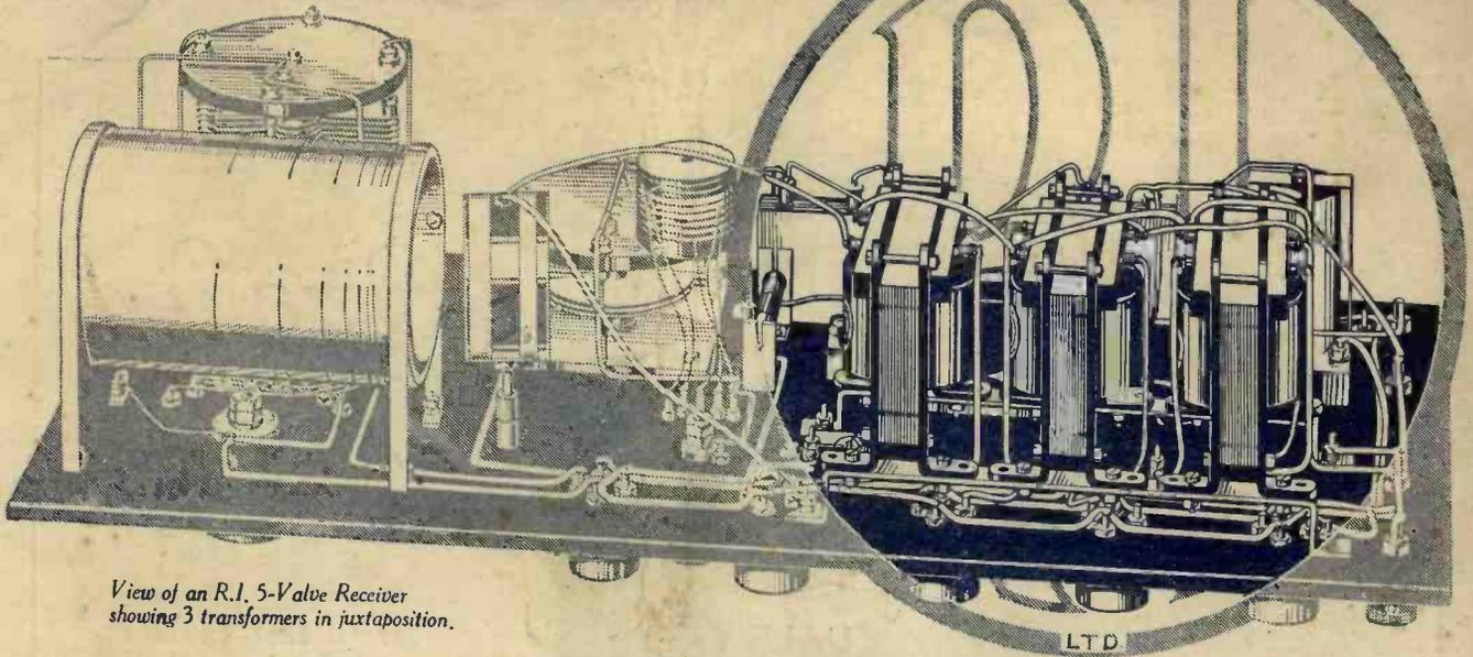
View of an R.I. 5-Valve Receiver showing 3 transformers in juxtaposition.
