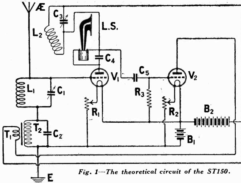
Fig. 1—The theoretical circuit of the ST150.
