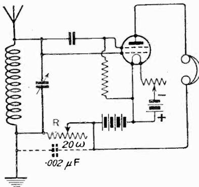
Fig. 3.—An alternative method of control.
