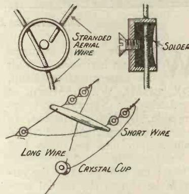
Diagram illustrating how the join is made.
