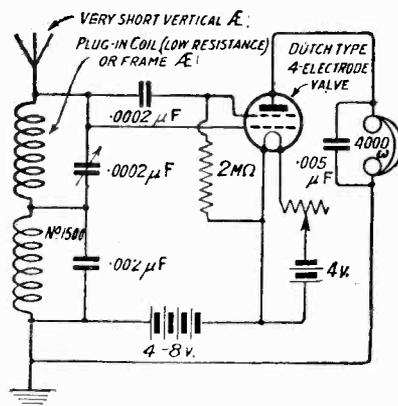
Fig. 4.—A single-control super-regenerative receiver.
