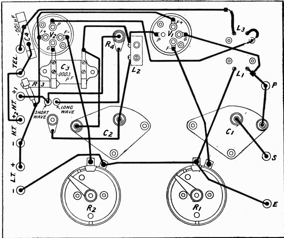
Fig. 3.—The wiring diagram, showing the necessary connections. Blueprint No. 90 b.
