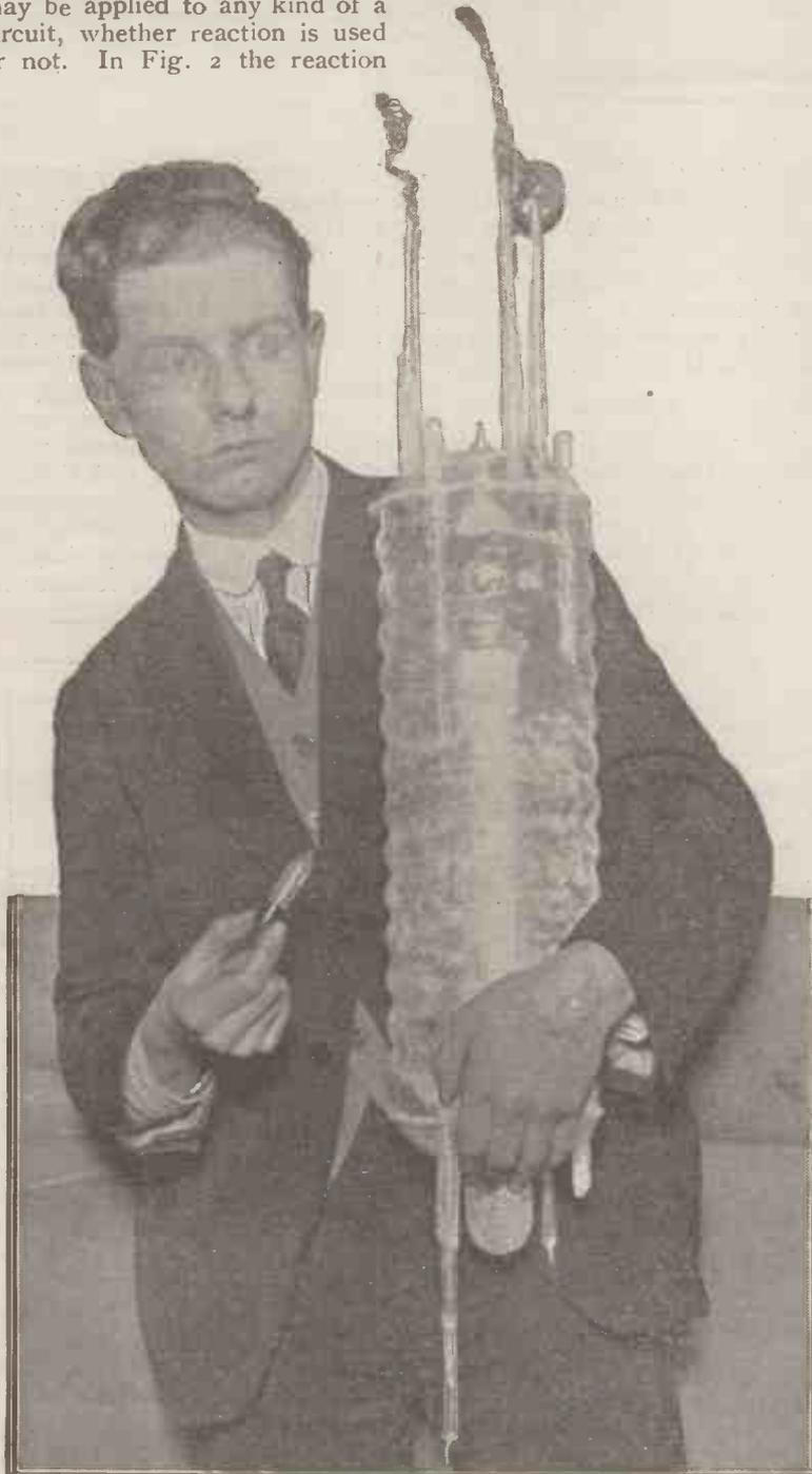
Our photograph shows a 30 Kilowatt Silica Transmitting Valve, made for the Admiralty, compared with the peanut valve held alongside.
