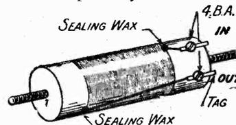
Fig. 5.—Showing method of securing the wire in the choke coil.
