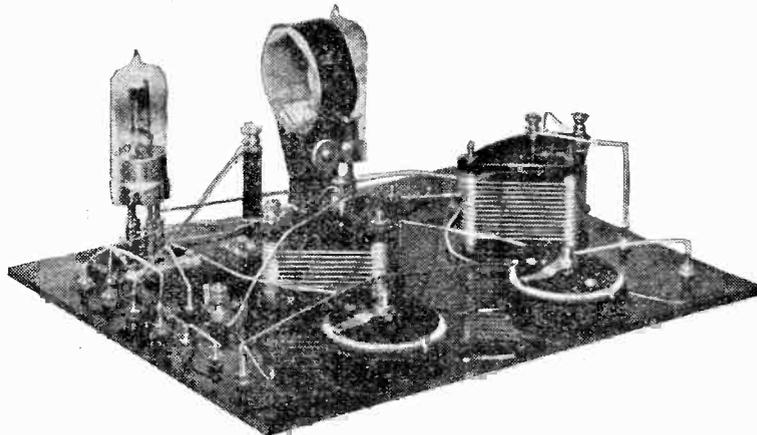
Showing the valves and anode coil.
