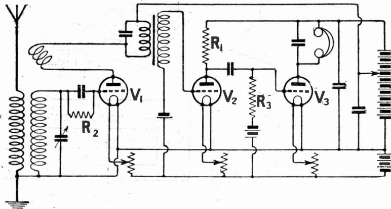
Fig. 1.—One transformer coupled, and one resistance coupled note magnifier form a good combination.
