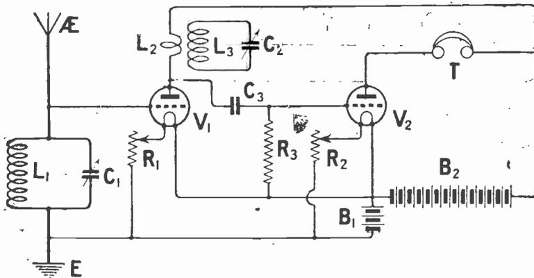
Fig. 1.—Illustrating the arrangement of the anode trap.
