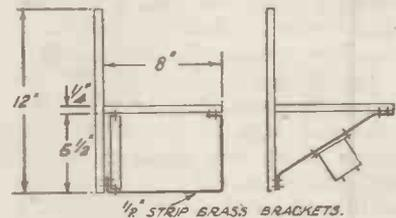
Fig. 5.—Details of the panel supporting brackets, showing manner in which the condenser C10 and grid cells are mounted.
