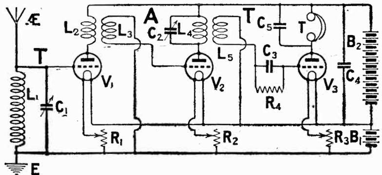
Fig. 2.—A T.A.T. circuit in which H.F. transformer coupling is employed.
