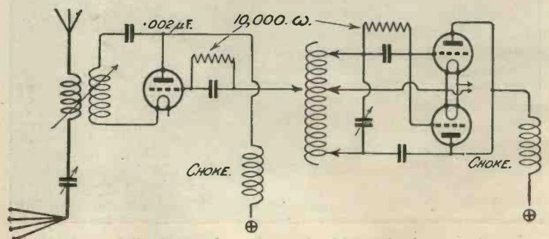
The Master Oscillator circuit used at 2DX.
