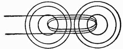
Fig. 7.—This arrangement of turns gives the highest self-induction.
