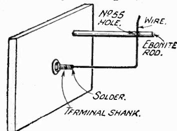
Fig. 5.—Secure the wire in the manner shown.
