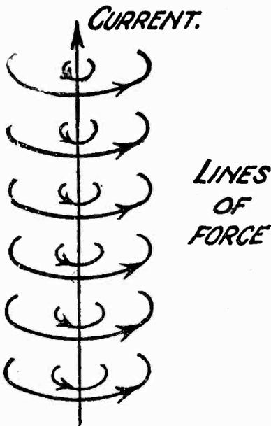
Fig. 1.—Distribution of field around a straight conductor.
