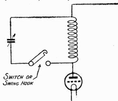
Fig. 4.—A suggested arrangement for cutting out the variable condenser in a tuned anode circuit.
