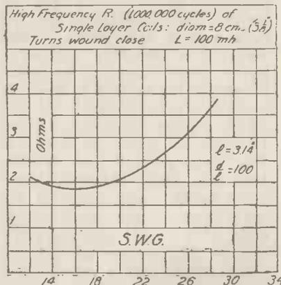
Fig. 6.—Curve produced under the same conditions as in Fig. 5, but using a coil of 100 microhenries.
