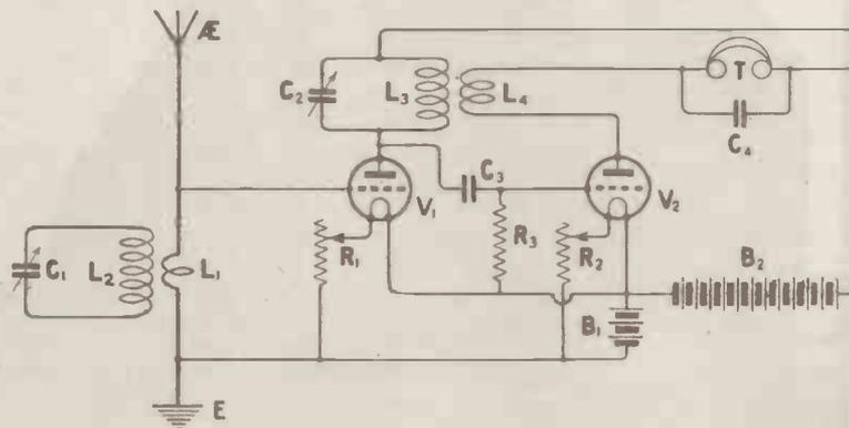
Fig. 3.—Trap aerial tuning applied to the ST34 circuit.
