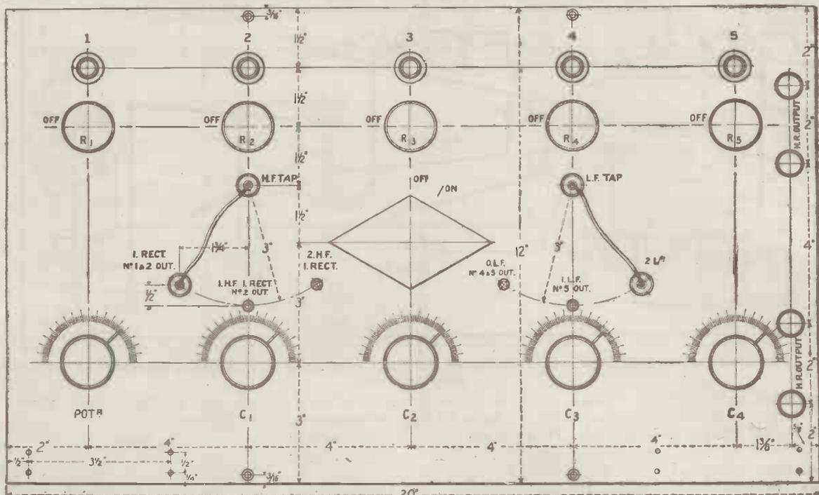
Fig. 1.—The layout of the panel and drilling dimensions. Blue print No. 94a.
