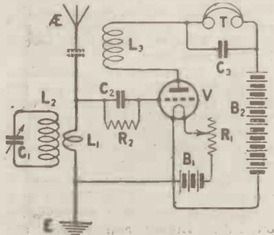
Fig. 2.—In the case of a single valve the reaction coil  $L_3$  may be coupled to either  $L_1$  or  $L_2$ .
