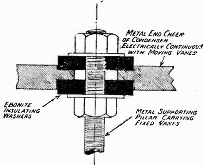
This diagram shows the method of clamping the fixed plates of Burn-dept condensers.
