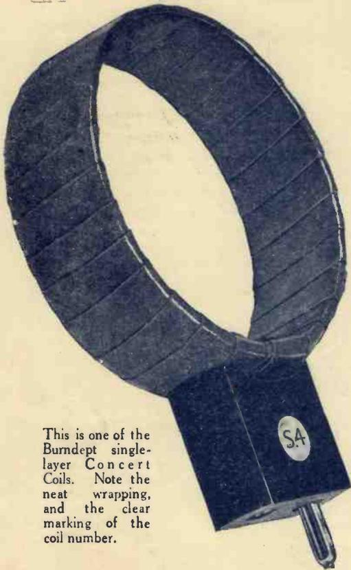
This is one of the Burndept single-layer Concert Coils. Note the neat wrapping, and the clear marking of the coil number.
