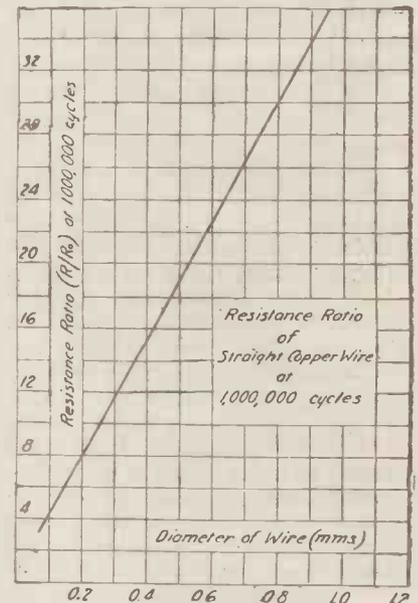
Fig. 3.—Curve of resistance ratios of straight copper wire plotted against diameter.
