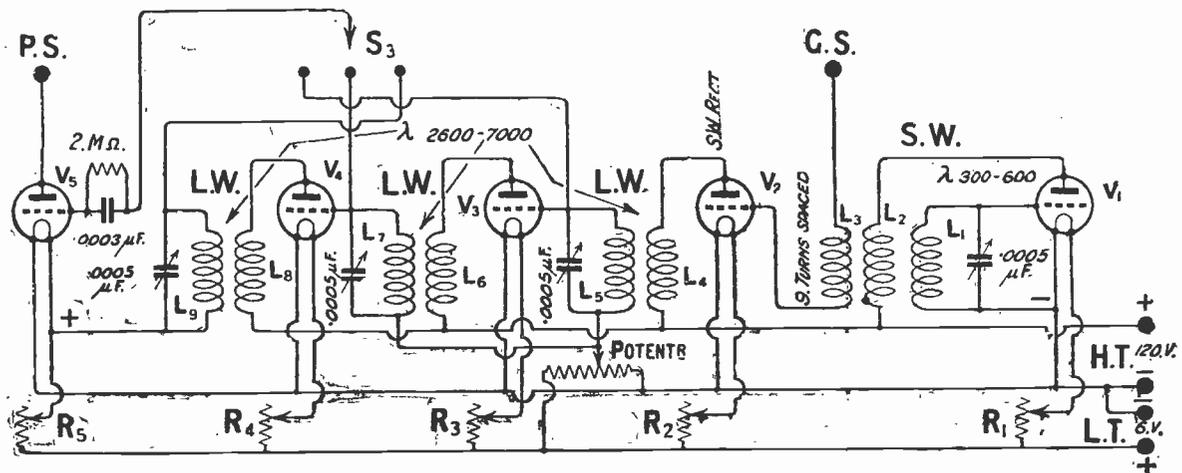
Fig. 6.—Theoretical circuit arrangement of the super-heterodyne unit.
