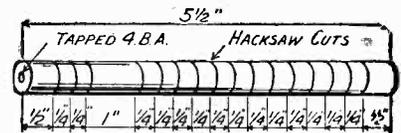
Fig. 4.—How the rods are grooved.
