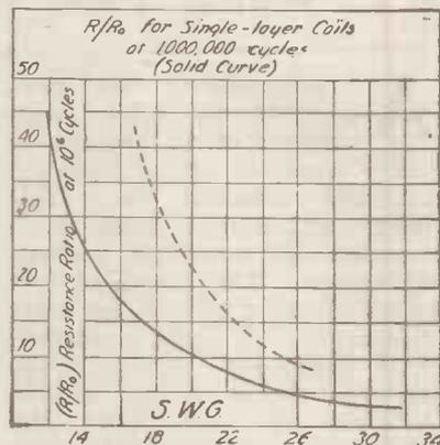
Fig. 10.—Showing the variation in  $R/R_0$  for single-layer coils at 1,000,000 cycles.
