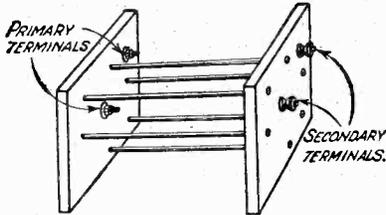
Fig. 1.—Details of the coil former.
