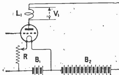
Fig. 2.—When H.F. potentials are applied to the grid the E.M.F.'s across L<sub>1</sub> will be small.
