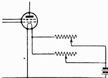
Fig. 2.—The reaction control.
