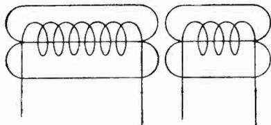
Fig. 8.—Separating the turns reduces the self-induction.
