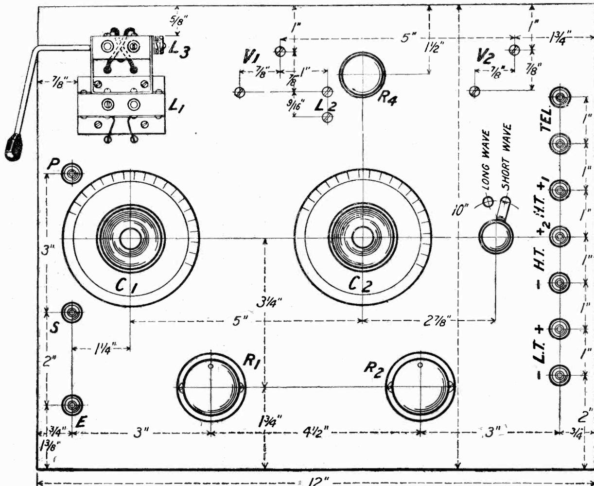
Fig. 2.—A half-size drawing of the panel, giving all necessary dimensions. Blue print No. 90a.
