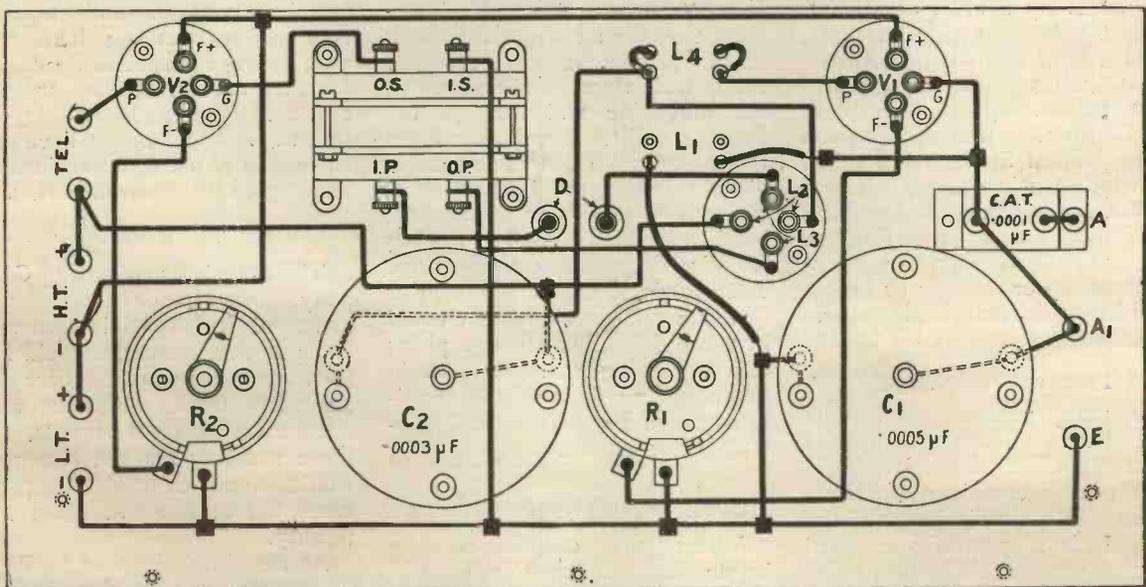
Fig. 6.—Practical back-of-panel wiring, of which full-sized drawings may be obtained upon quoting Blueprint No. 95b.
