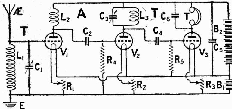
Fig. 1.—A three valve T.A.T. circuit using tuned anode coupling.
