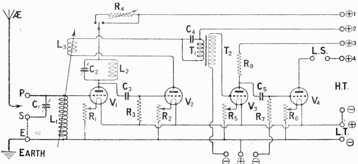
Fig. 4.—Showing the connections necessary when a two-valve amplifier is added, the last stage of L.F. being resistance coupled.
