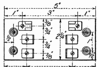
Fig. 4.—Drilling dimensions.
