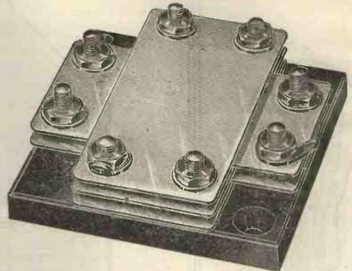
For sharp tuning and to shorten the wavelength, thus facilitating self-oscillation by the reduction of capacity in the aerial circuit, a small fixed capacity series condenser having an air dielectric must be used.
