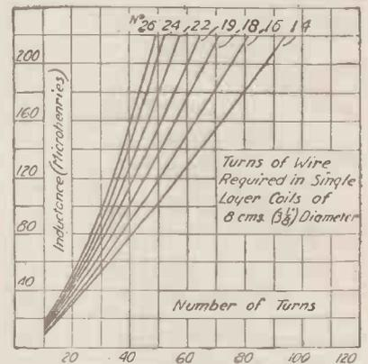
Fig. 8.—Showing number of turns required in single-layer coils of the same diameter to give different values of inductance.
