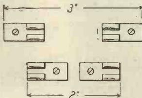
The lower diagram shows how fixed condenser clips may be mounted to economise in space.
