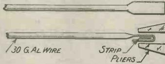
Fig. 5.—Details of the pointer.
