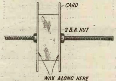
Fig. 4.—How the side supports for the coil-former are mounted.
