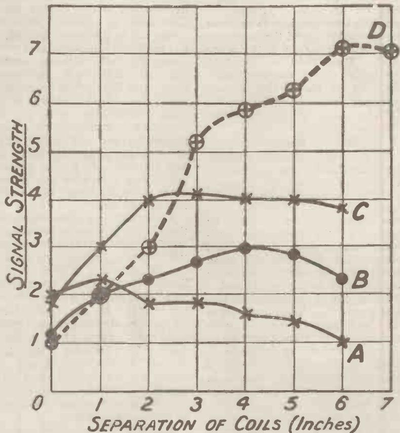
Fig. 1.—The curve D is a good example of the errors which may be introduced by concealed reaction effects.
