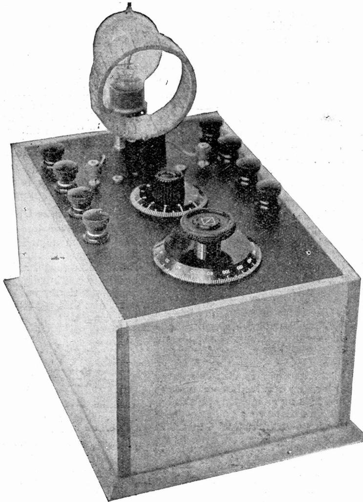
A graduated dial upon the filament rheostat is a desirable refinement.
