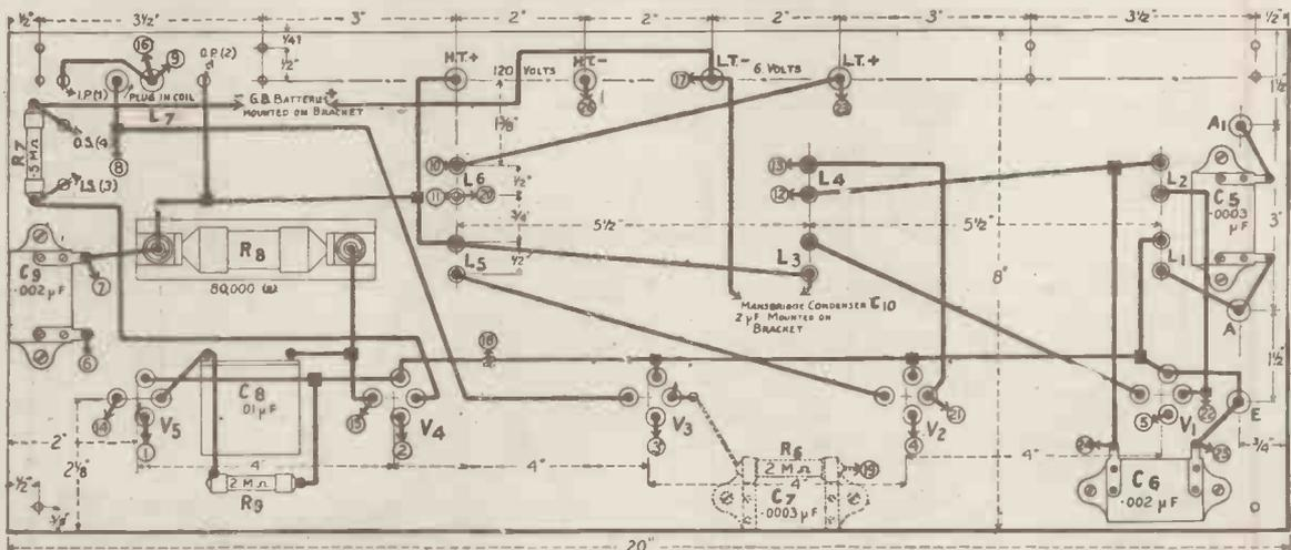
Fig. 3.—The wiring of the underside of the valve panel, the lower edge being that which fits against the front panel. Blue print 94c.
