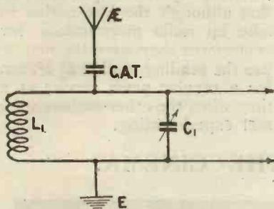
Fig. 1.—The C.A.T. method of increasing sharpness of tuning.
