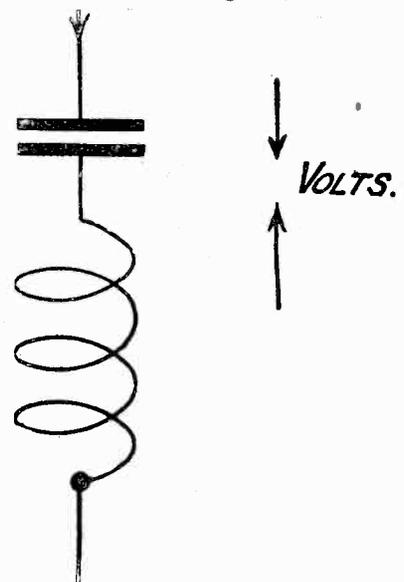
Fig. 3.—Relation of voltages produced across a coil and a condenser.
